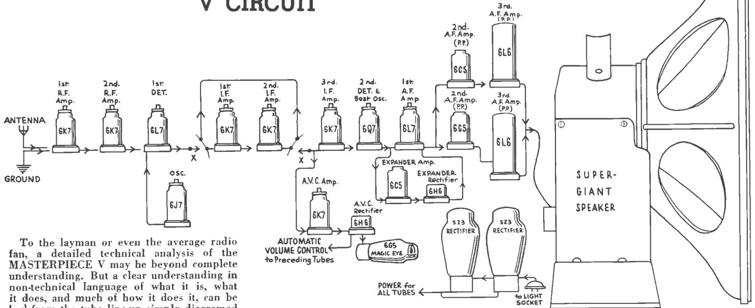
To the layman or even the average radio fan, a detailed technical analysis of the MASTERPIECE V may be beyond complete understanding. But a clear understanding in non-technical language of what it is, what it does, and much of how it does it, can be had from the tube line-up simply diagramed above.
