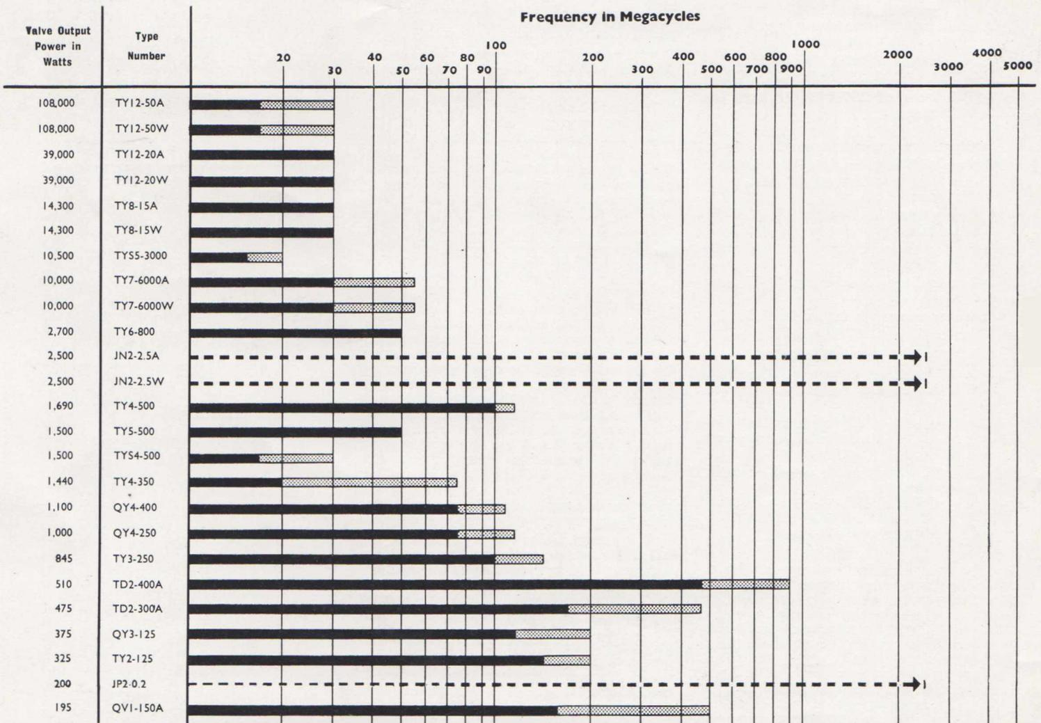
**Increased Ratings** The ratings shown here are for continuous operation. In many industrial applications where valves are operated intermittently ratings may be considerably increased. Details are available on request.
