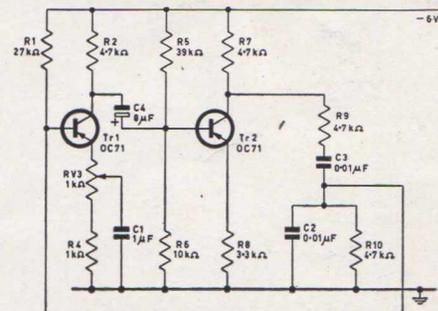
This simple two-stage R-C oscillator will provide an audio output of reasonable waveform at a frequency of approximately 2.5kc/s. Temperature stability is good and supply voltages from -3V to -9V can be used, providing RV3 is suitably adjusted. This control provides a convenient means of adjusting the circuit for optimum performance and compensates for changes of ambient temperature. The audio output may be taken from R7 or R8.
