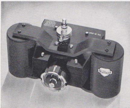
The JN2 - 2.5A Magnetron which is shown on the cover of this issue is primarily designed for microwave heating. The power output is 2.5kW c.w. at a fixed frequency of  $2.45 \pm 0.025$  Gc/s. More detailed information may be found on Pages 30 and 31.
