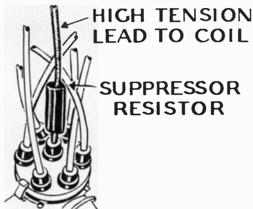
Figure 14. Distributor Suppressor Resistor
