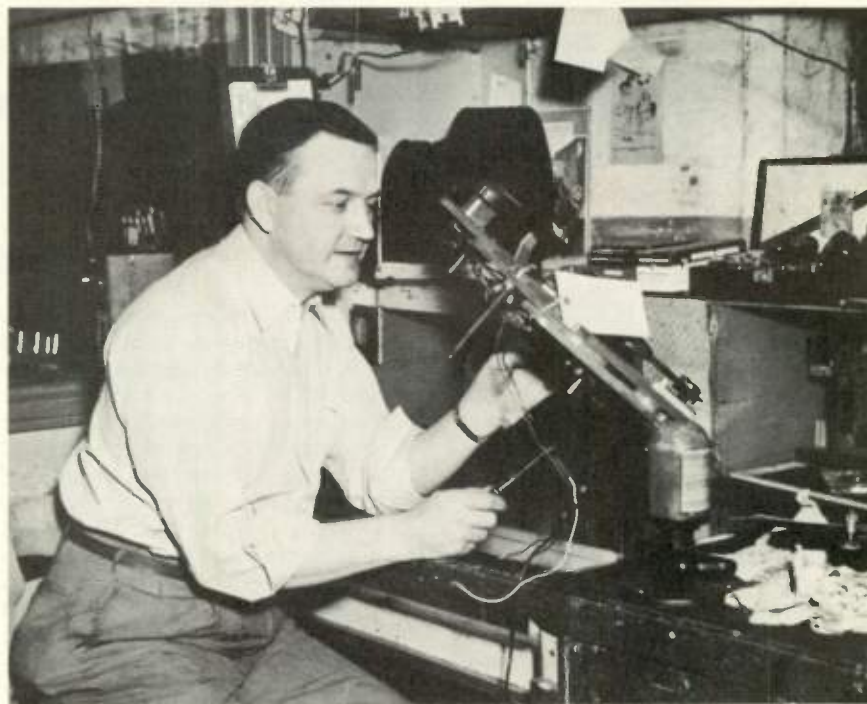
Harold Simmons, Phono Specialist, has both hands free because of the ball jointed turntable holder and the plate glass bench top that provides full illumination in those hard to see places.
