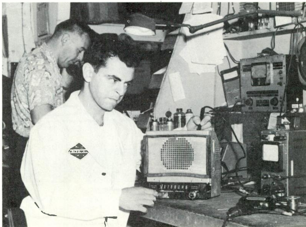
Richard Hajian tests a tube while making an auto radio repair. Regardless of the reason the radio was brought in, a complete check is made of the entire radio before it is returned to the customer.
