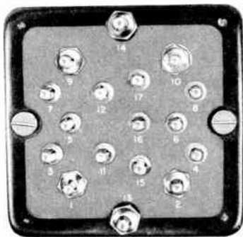
Figure 1. Bottom View of Vibrator VB-16. Showing Pin Arrangement
