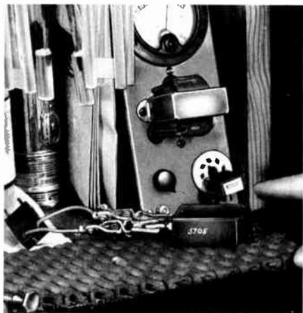
**Figure 2. Test Oscillator Used To Determine Crystal Frequency**
