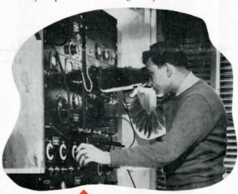
Bernie Liebermann, Eng., aligns test apparatus used in checking the operation of military electronic and radio devices for combat aircraft.
