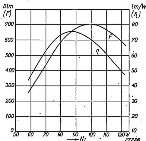
Fig. 10. Light flux  $F$  (in decalumsens) and efficiency  $\eta$  (in lm/W) for a sodium lamp SO 650 as a function of the power on the lamp  $N_l$ .
