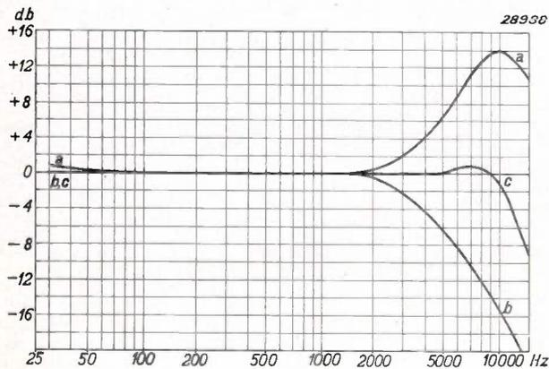
Fig. 9. Frequency characteristic of amplifier *B* combined with the frequency characteristic of the ribbon microphone.
