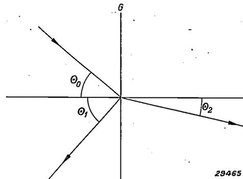
Fig. 2. Reflection and refraction at a boundary surface.  $\theta_0$  angle of incidence,  $\theta_1$  angle of reflection and  $\theta_2$  angle of refraction. The relation between the angles  $\theta$  is given by Snellius' law:
