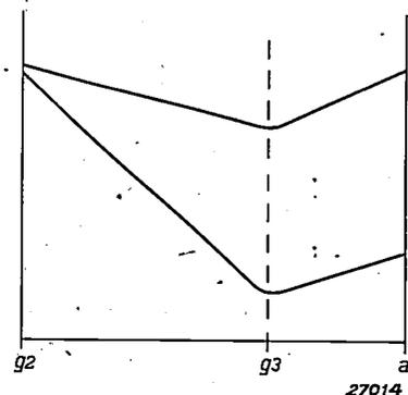
*Fig. 3.* Variation of the potential between screen grid and anode in a pentode without space charge (plane parallel electrodes).
