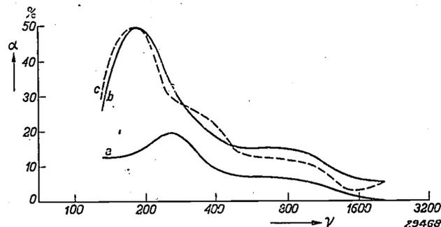
Fig. 5. Absorption coefficient  $\alpha$  per  $m^2$  expressed in per cent as a function of the frequency in c/s for 5 mm thick triplex panels of 1.5 m by 1 m, placed 5 cm in front of the wall.
