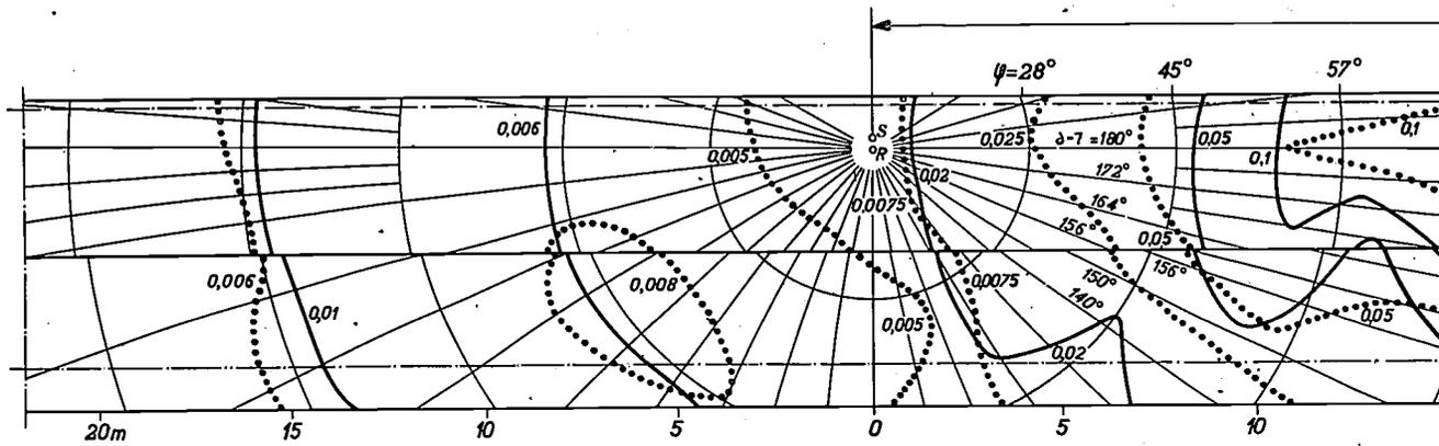
Fig. 7. Curves of equal brightness coefficient (iso- $q$  curves) for a roof-shaped road (slope 1 : 50) 8 metres wide. Height of the light source 8 metres above the curb. The eye of the observer is at a distance of 100 metres from the lightsource and
