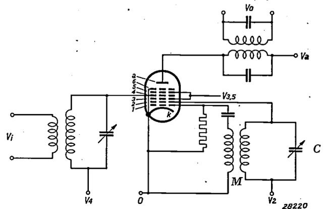
Fig. 1. Diagram of the principle of a frequency-changing stage when an octode is used. The cathode *k* with the grids *1* and *2* forms an oscillator triode; grids *4*, *5* and *6* form, with anode *a*, an amplifier and frequency-changing pentode. The screen grid *3* is the shield between these two parts of the octode;  $V_1$  is the input voltage and  $V_0$  the output voltage.
