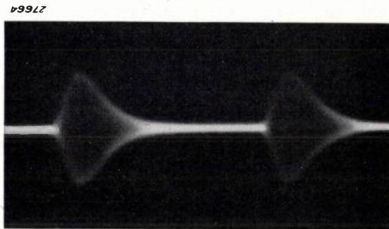
Fig. 8. “Blocking” of an oscillating circuit. If the amplitude of the oscillations exceeds a certain critical value, the valve suddenly ceases to oscillate. The oscillations then start decaying exponentially. Only when the oscillations have nearly become zero does the valve start oscillating again.
