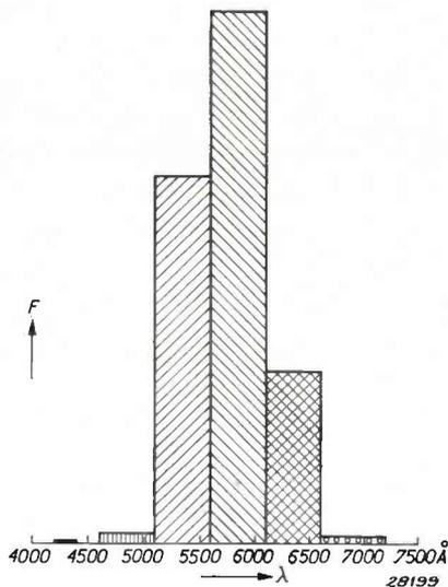
Fig. 8. Block diagram of the light of a mercury tube made of copper-uranium glass and containing zinc beryllium silicate.
