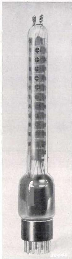
Fig. 7. Electron multiplier type 4698, constructed according to the scheme of fig. 6 with eleven stages.
