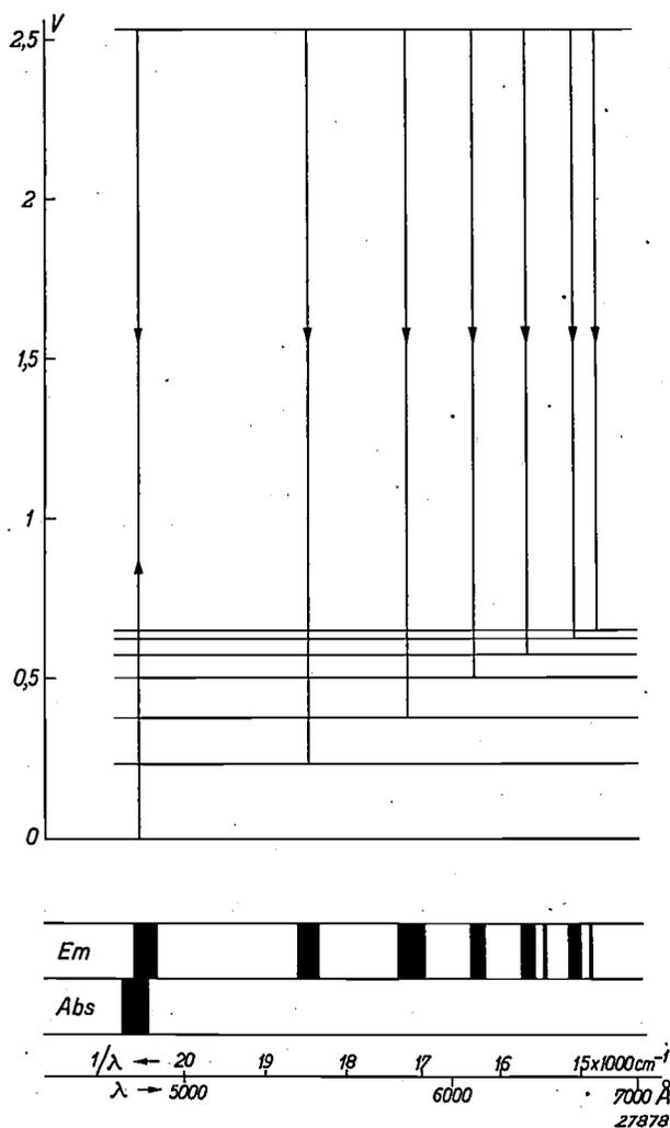
Fig. 1. Energy scheme of the ion  $\text{Tb}^{+++}$  and absorption and emission spectra of  $\text{Tb}_2(\text{SO}_4)_3 \cdot 8 \text{H}_2\text{O}$  according to Gobrecht (1937). Each of the transitions shown corresponds to a group of fine lines, each group being shown in the figure enclosed by a black rectangle. Particularly at low temperatures are these lines distinctly separated.
