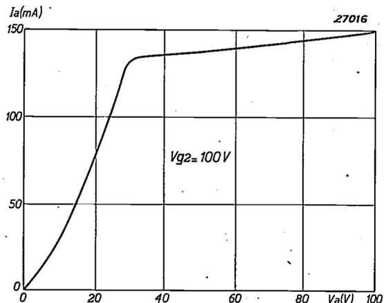
Fig. 6.  $I_a - V_a$  characteristic of a tetrode with auxiliary electrode as in *fig. 5*.
