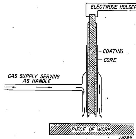
Fig. 2. Apparatus for welding in different atmospheres.
