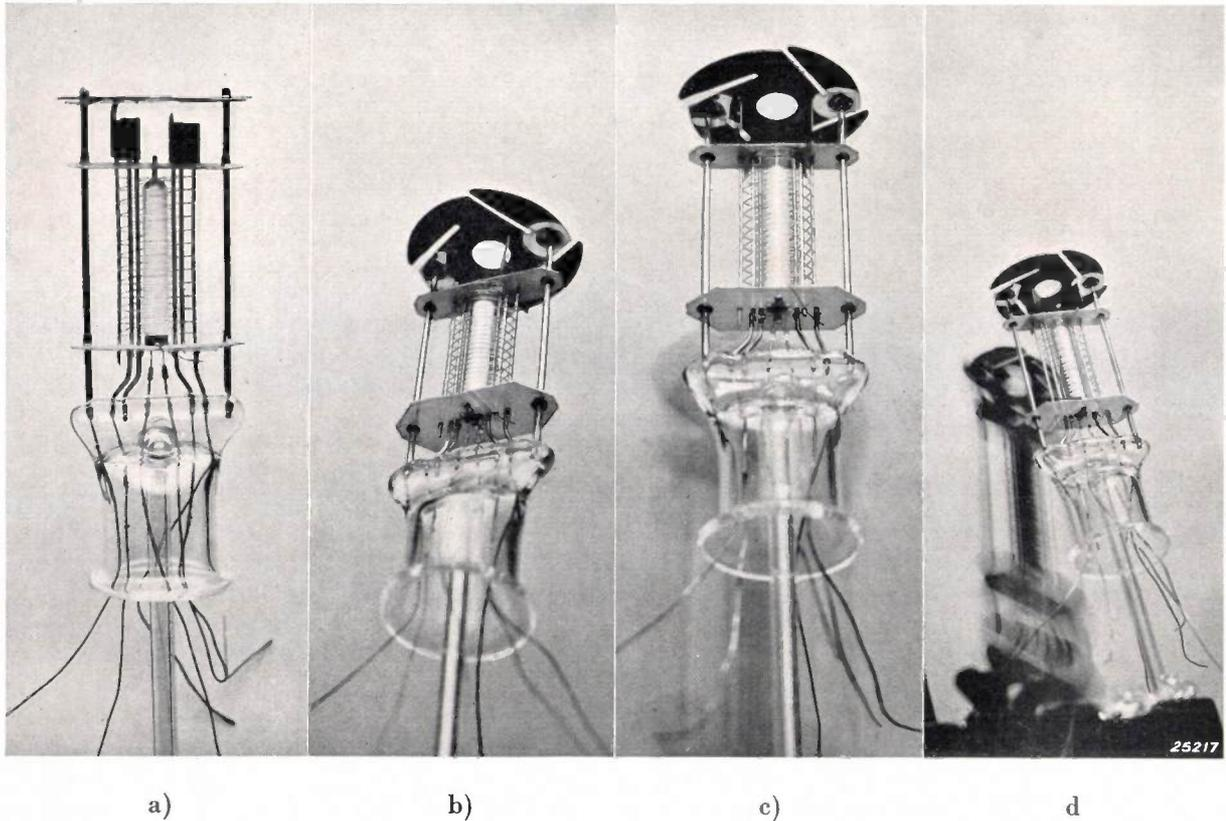
Fig. 3. The inside of a pentode, photographed under various systems of local illumination.
