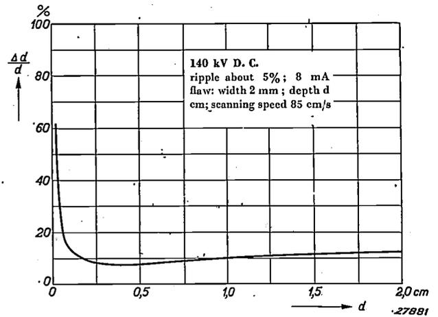
Fig. 4. The relative flaw  $\Delta d/d$  detectible as a function of the wall thickness  $d$  at a constant tube voltage (140 kilovolts constant direct voltage; 8 milliamperes), constant width of flaw (0.2 cm) and constant scanning speed (85 cm per sec.).
