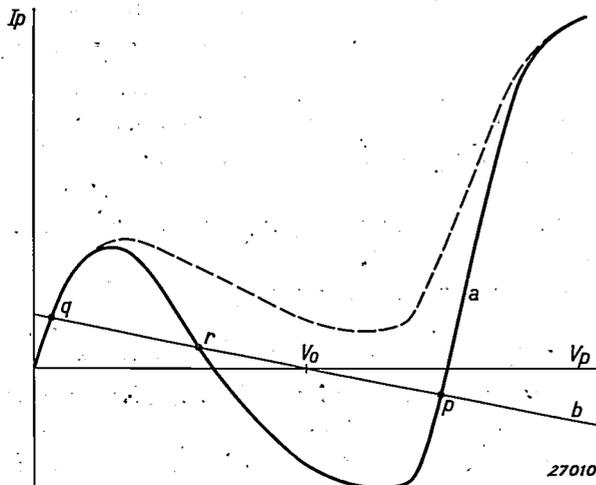
Fig. 8. Curve *a*: current  $I_p$  of a plate with a high secondary emission which is bombarded with electrons as a function of the plate voltage. With a lower secondary emission the current will vary according to the dotted-line curve.
