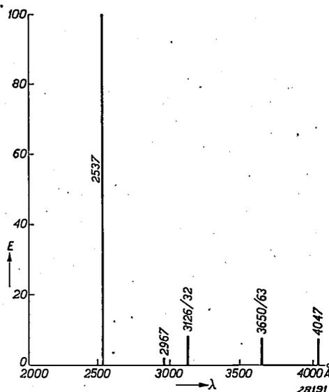
Fig. 3. Relative energy distribution of a typical low-pressure mercury discharge; intensity of the line 2537 Å set equal to 100.
