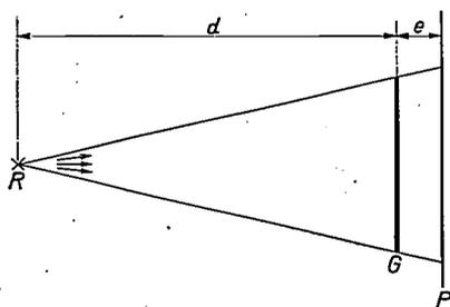
Fig. 1. Arrangement in taking an X-ray photograph. The object  $G$  is at a distance  $d$  from the square focus  $R$ . The distance between object and film  $P$  is  $e$ . With an area  $F$  of the focus every point of the object is projected as a shadow spot of width  $e \sqrt{F}/d$  (geometrical lack of sharpness  $O_g$ ).
