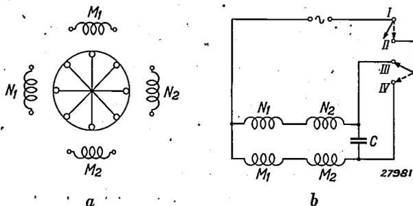
Fig. 6*a*. Diagram of the motor. A drum armature rotates in the field of four coils  $M_1, M_2, N_1$  and  $N_2$ . Fig. 6*b*. Circuit of the motor. *C* is a condenser which provides for the necessary phase shift in the currents in the pairs of coils  $M_1 - M_2$  and  $N_1 - N_2$ .
