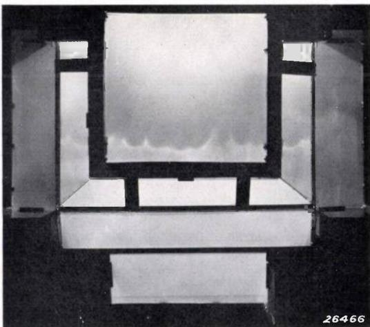
Fig. 8a). Distribution of light on the floor and rows of seats around the floor.
