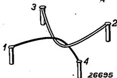
*Fig. 1.* Klemenčič's thermocouple. The wire of one metal is fastened to terminals 1 and 4, that of the other metal to terminals 2 and 3. The wires are joined in the middle electrically in some way. The current to be measured passes through along the terminals 1 and 2, the galvanometer is connected between 3 and 4.
