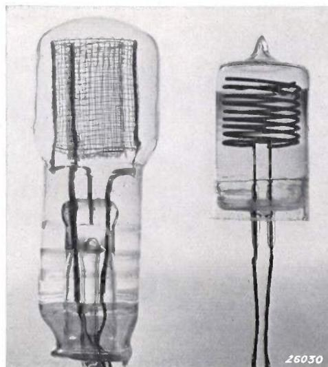
Fig. 1. Sealing of tungsten into silica bulbs with the aid of:
