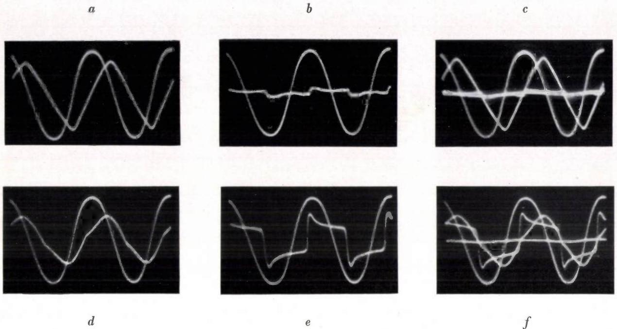
Fig. 9. Various combined oscillograms. Upper row: cold mercury lamp; lower row mercury lamp in working condition. The sine curve in each case represents the mains voltage.
