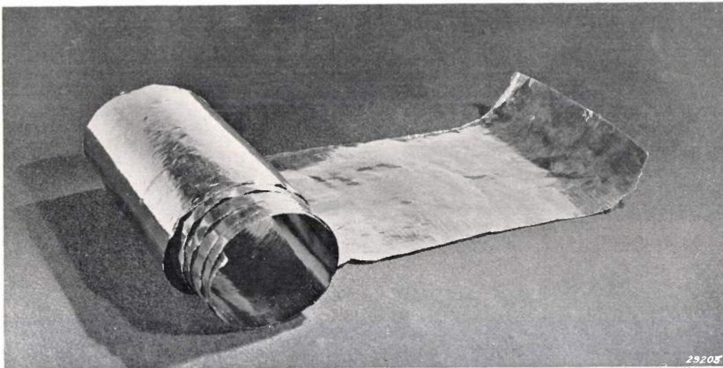
*Fig. 3.* Zirconium sheet 20 microns thick, obtained by cold rolling of the material from the thickness of 0.6 mm.
