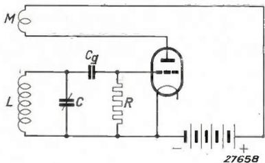
Fig. 7. Principle of an oscillating circuit.
