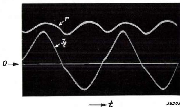
Fig. 11. Variation with time of the discharge current  $I_l$  and light flux  $F$  (sum of mercury light and luminescence light) for a low-pressure mercury discharge with phosphorescent zinc beryllium silicate (50 c/s).
