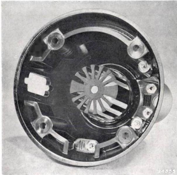
Fig. 3. Cover containing terminals of a vacuum cleaner.
