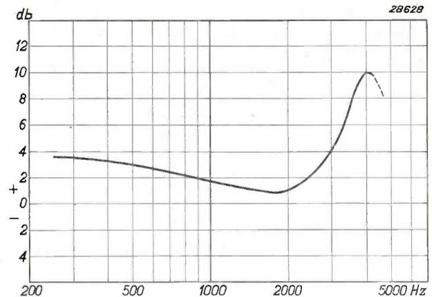
Fig. 8. The frequency characteristic calculated from the spectra of figs. 4 and 7. The ratio between the intensities of corresponding orders of figs. 4 and 7 is a measure for the corresponding ordinate of the frequency characteristic of the system for the frequency in question. By the measurement of intensities in the spectrum the whole frequency characteristic can be determined in this way.
