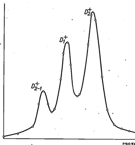
Fig. 3. Part of the magnetic "spectrum" of the ions in the ion beam. The deflection in the magnetic field is plotted horizontally, the ion intensity vertically. The ions  $D_1^+$  (deutons *d*) of the middle maximum are chiefly effective in the production of neutrons, since they possess the greatest velocity.
