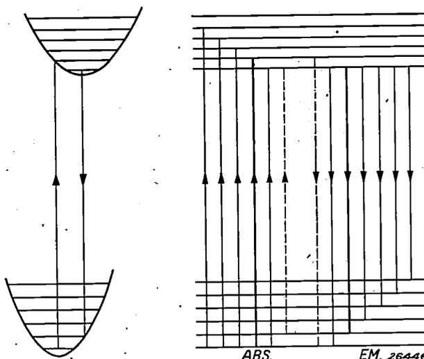
Fig. 13. Left: potential curves of the  $\text{UO}_2$  radical with the strongest transitions in emission and absorption. Right: energy levels with transitions in the same order as the lines in fig. 12. The levels indicated by dotted lines do not occur at  $-180^{\circ}\text{C}$ , while they do occur at room temperature.
