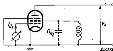
Fig. 8. The appearance of resonances in the valve at high frequencies. The self inductance  $L_{g_2}$  of the screen grid lead is tuned with the capacity  $C_{g_2}$  of the screen grid to the frequency of  $v_a$ . This is expressed in a strong current  $i_{g_1}$ , i.e., in a high conductivity from anode to the first grid.
