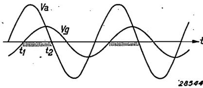
Fig. 11. The relay valve  $G$  (fig. 10) ignites as soon as the grid voltage  $V_g$  becomes positive (time  $t_2$ ). The valve works only during the time intervals indicated by cross hatching. If a direct voltage is superposed on  $V_g$ , i.e. if the curve  $V_g$  is raised somewhat in height the moments  $t_1$  occur somewhat sooner, the average anode current of the relay valve becomes greater.
