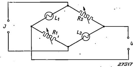
Fig. 6. Bridge circuit for obtaining the regulation voltage of an expander. The resistances  $R_1$  and  $R_2$  are so adjusted that the bridge is in equilibrium at room temperature of the filaments  $L_1$  and  $L_2$ . When an alternating voltage is applied the temperature of the filaments increases. The bridge is then no longer in equilibrium and a voltage acts across the output terminals which increases more rapidly than the alternating voltage.
