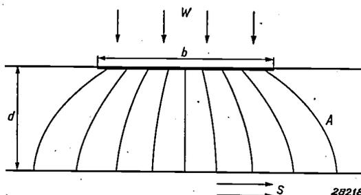
Fig. 6. The problem of heat conduction at the anode. At the focus  $f$  (whose longest side must be imagined perpendicular to the plane of the drawing) the heat flux  $W$  is developed. The heat is conducted through the body of the anode  $A$  to the rear wall where cooling takes place by means of running water  $s$ . As is indicated a divergence in the lines of heat flux occurs which is more pronounced the greater the thickness of the anode  $d$ .
