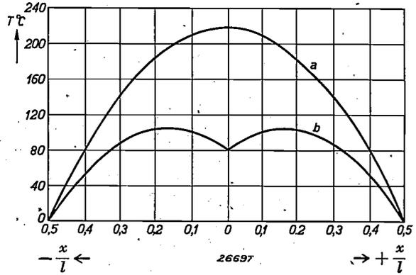
Fig. 3) a) Temperature of a stretched wire through which current is flowing.
