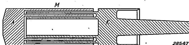
Fig. 6. The cooling of the anode *A*-rotating in a vacuum, which is necessary for continuous use of the tube, takes place by radiation of the blackened cylindrical shells *M* upon similar shells of the stationary support *K*.
