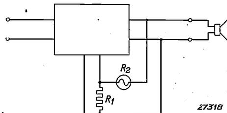
Fig. 7. A very simple expansion circuit, which uses a varying inverse feedback. With an increasing output-voltage the resistance  $R_2$  of the lamp becomes greater. In this way the strength of inverse feedback is reduced and the amplification factor increases.
