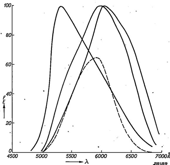
Fig. 1. Emission curves: energy as a function of wave length (full lines; maximum put equal to 100), for several zinc beryllium silicates activated with manganese in a low-pressure mercury discharge. The dotted line gives the light intensity as a function of wave length for the phosphorescent substance with its energy maximum at 6050 Å. At the wave length of maximum eye sensitivity the light intensity is put equal to the energy.
