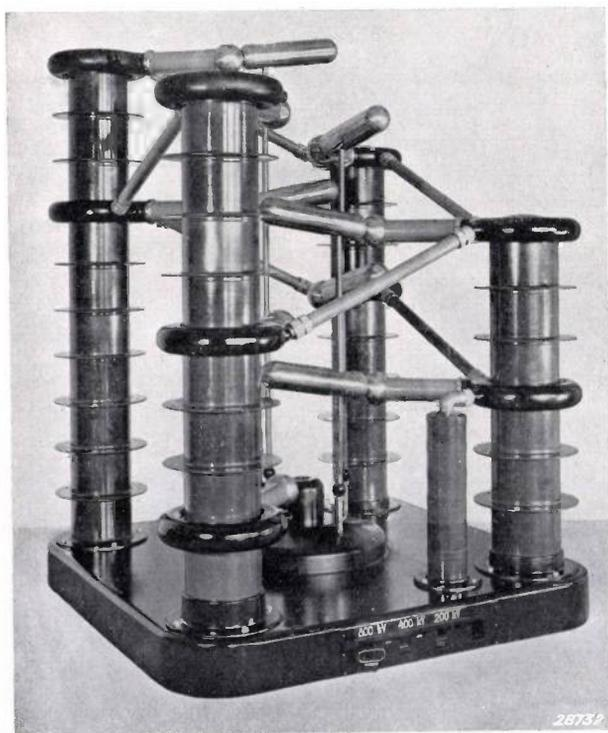
Fig. 5. Impulse generator with an impulse energy of 16 kW sec, commutable for 800, 400 and 200 kV (with 0.05, 0.2 and 0.8  $\mu$ F respectively) in the present form with large "Philite" cylinders. Height 2.6 m.
