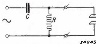
Fig. 3. A simple filter is connected between the mains and the deflection plates of the cathode ray tube in order to decrease the intensity of the fundamental frequency of the alternating voltage between the plates.
