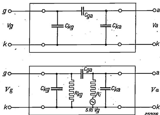
Fig. 1. a) Substitution diagram of a cold amplifier valve. The input admittance is determined by  $C_{kg}$ , the output admittance by  $C_{ka}$ , slope and reaction are given by the capacity  $C_{ga}$ .
