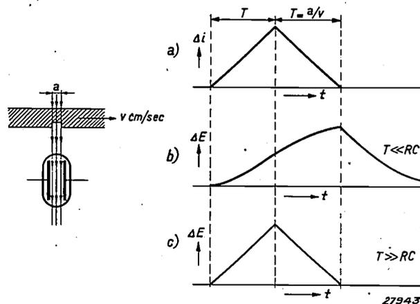
Fig. 6. Variation of current  $\Delta i$  (a) through the grid resistance and the voltage  $\Delta E$  (b and c) at the grid when a flaw of size  $a$  travels past one of the ionisation chambers with a velocity  $v$ .
