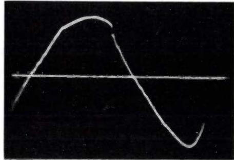
Fig. 4. Variation of the voltage in the secondary of the transformer of fig. 3. The moment at which the current through the rectifier valve is interrupted is distinguished by a voltage jump.
