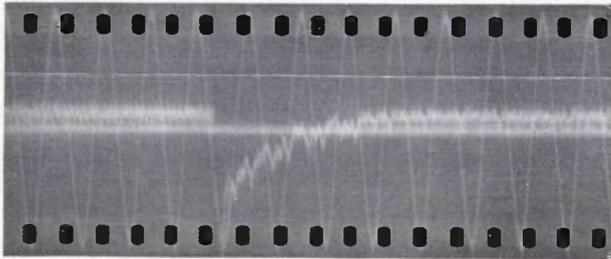
Fig. 2. Variation of the terminals voltage upon sudden application of the load.
