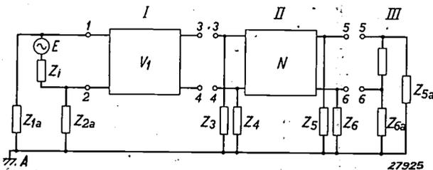
Fig. 1. Equivalent circuit of an interference source. The interfering voltage  $E$  with the internal impedance  $Z_i$  is located between terminals 1 and 2. Terminals 5 and 6 are the inputs of the receiver;  $A$  is earth.  $V_1$  and  $N$  are generalised quadripoles; the first connects the interfering voltage to the mains terminals of the interference producer, and the second represents the network between the interference source and the terminals of the receiver.
