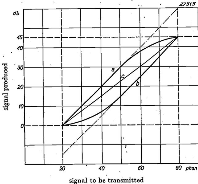
Fig. 2. Different compression characteristics which reduce variations in intensities from 60 db to 45 db.
