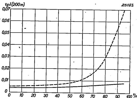
Fig. 2. Dielectric losses ( $\tan \delta$ ) measured at 200 m wave length between two insulated wires with 0.5 mm core diameter, which were twisted together with a pitch of 2.6 cm, as a function of the relative humidity of the surrounding atmosphere. The wires were kept in this atmosphere until the losses had become constant and they were not removed from it for taking the measurements.
