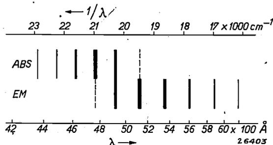
Fig. 12. Emission and absorption spectra of potassium uranyl sulphate ( $25^{\circ}\text{C}$ ). The lines represent diagrammatically the position and intensity of the bands. The bands indicated by broken lines disappear at very low temperatures  $1000\text{ cm}^{-1} = 0.1239$  electron volts).
