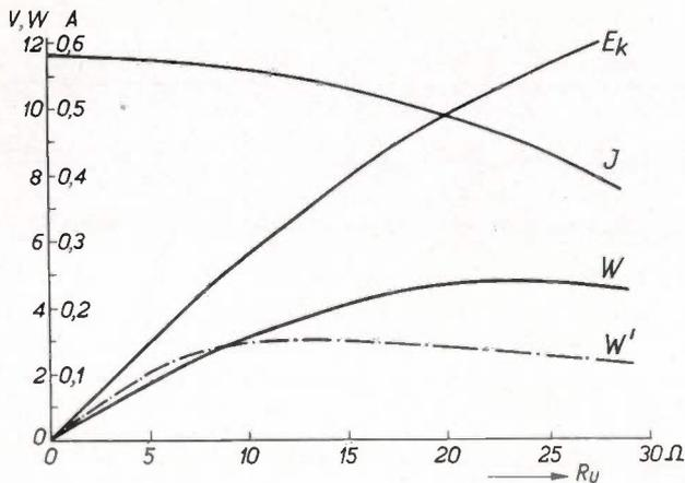
Fig. 5. Terminal voltage  $E_k$ , current  $I$  and power delivered  $W$  as dependent on the external resistance  $R_u$ ; the so-called external characteristic of the dynamo. The power delivered  $W'$  is indicated by a dot-dash line for a dynamo provided with a winding of 140 turns, in contrast to the final construction with 200 turns.
