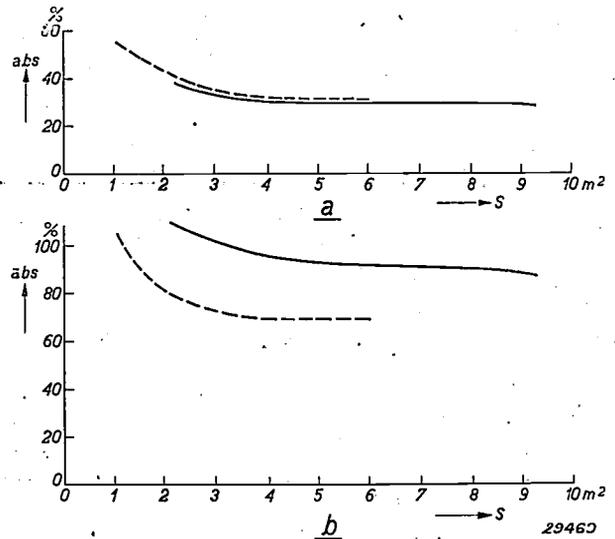
Fig. 6. Absorption coefficient as a function of the surface area of the absorbent material at 256 cycles/sec (a) and at 512 c/s (b), measured in two different American laboratories. Curves of same laboratory continuous and broken lines respectively.
