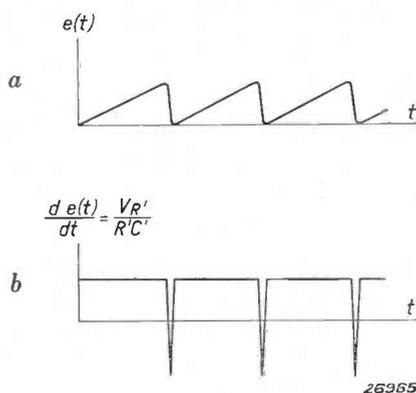
Fig. 4. Form of the sawtooth voltage  $e(t)$  and of its derivation  $d e(t) / dt$  as a function of the time.
