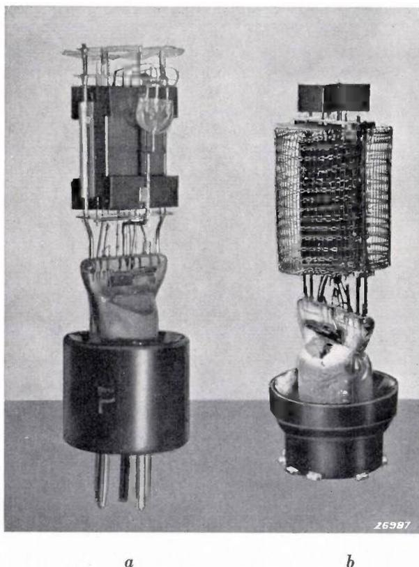
Fig. 12  $a$ ) Power amplifier valve in which the mica supporting plates and the glass wall are shielded against bombardment with electrons by enclosing caps at the ends of the system.  $b$ ) In an amplifier valve with a gauze anode the glass wall is exposed to a strong bombardment by electrons. In order to avoid this the anode is surrounded by a gauze cage which is connected to the cathode.
