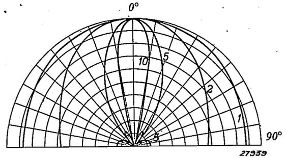
*Fig. 6.* Directional distribution of the sound intensity with a circular vibrating plate in an infinitely large baffle. The figures against the curves give the values of the parameter  $ka$  which determines the distribution.
