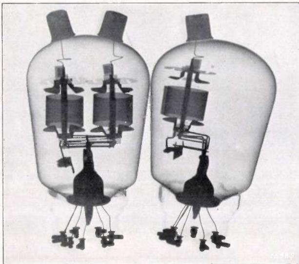
Fig. 5. X-ray photograph of a single and a double pentode (type EF5) for separating the two causes of the input damping on short waves.
