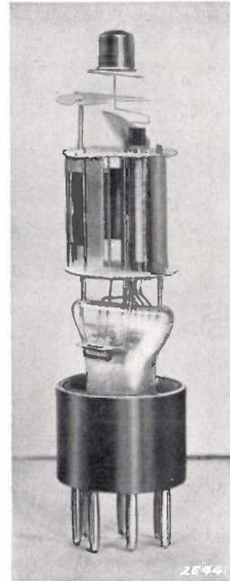
Fig. 10. Photograph of the interior of valve type 4696.
