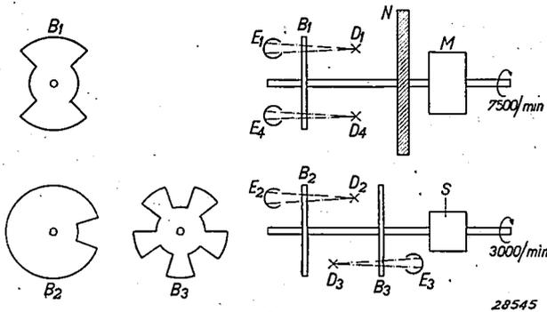
Fig. 7. Arrangement for obtaining picture synchronization signals.  $M$  = collector motor which drives the Nipkow disc,  $S$  = synchronous motor connected to the mains.  $B_1$ ,  $B_2$  = sector discs,  $D_1$ ,  $D_2$  = lamps,  $E_1$ ,  $E_2$  = photocells. The sector disc  $B_3$  and the photocells  $E_3$ ,  $E_4$  with their lamps serve for synchronization of the Nipkow disc with the mains, as described on page 294.
