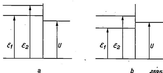
Fig. 6. a) The work function  $u$  of compounds of strongly electro-positive metals is lower than the minimum amount of energy  $\epsilon_1$ , which can be passed on to the electrons in the solid substance.
