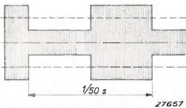
Fig. 5. Oscillogram of a carrier wave of  $10^7$  c/s with rectangular modulation of 50 c/s. This modulation is particularly suitable for investigating whether the carrier frequency depends on the modulation voltage (see fig. 6).
