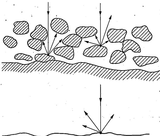
Fig. 8. Rough and smooth surfaces. In the case of the rough surface a portion of the secondary electrons are captured by the material itself, with the smooth surface they can escape unhindered.
