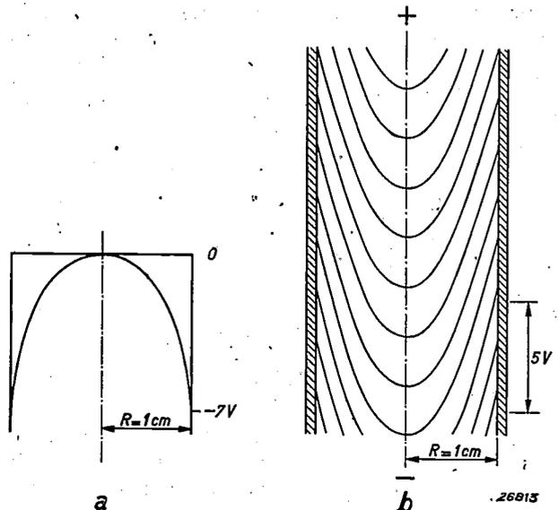
Fig. 5. a Potential variation along the radius, b Curvature of the equipotential planes.
