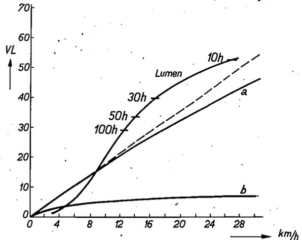
Fig. 4. Voltage in volts and light flux in lumens as functions of the riding speed. Curve a gives the variation of the no-load voltage and b the terminals voltage with the load of a lamp for 6 volts and 0.5 A. In the light flux curve the length of life of the lamp corresponding to the light flux also is indicated.
