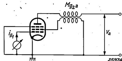
Fig. 7. Compensation of the reaction on ultrashort waves by means of a mutual induction  $M_{g_2a}$  between anode lead and screen grid lead.  $M_{g_2a}$  is chosen so that the  $\omega^2$  term in formula (8) is entirely compensated.
