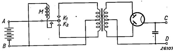
*Fig. 1.* Diagram of the supply of a motorcar radio set by means of a vibrator converter. The 6 or 12 volts accumulator is connected between the terminals *A* and *B*, while the anode voltage of about 250 volts is taken off between *C* and *D*. *M* is the electromagnet which keeps the vibrator moving; the contacts *K*<sub>1</sub> and *K*<sub>2</sub> are alternately made and broken.
