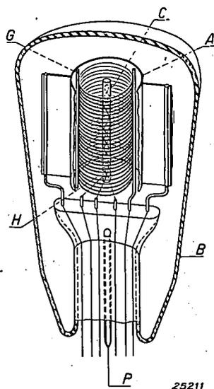
Fig. 2. Triode for measuring secondary emission.
