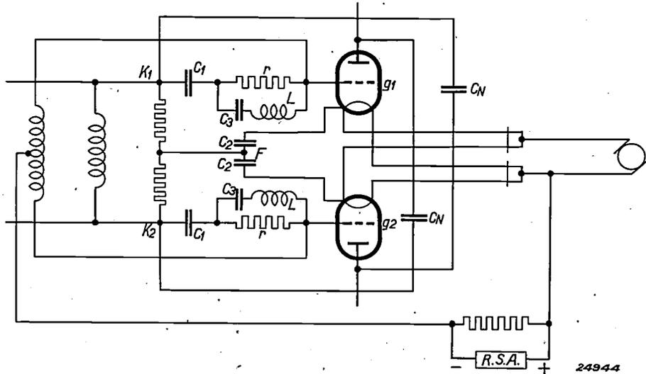
Fig. 11. Circuit diagram of the transmitting valves, in which self-inductances ( $L$ ) and capacities ( $C_3$ ), tuned to the working frequency, are introduced between grid ( $g_1$  and  $g_2$  respectively) and grid terminal ( $K_1$  and  $K_2$  respectively).
