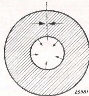
Fig. 4. Stresses occurring in glass part of lead-in, when  $\alpha_g < \alpha_m$ .
