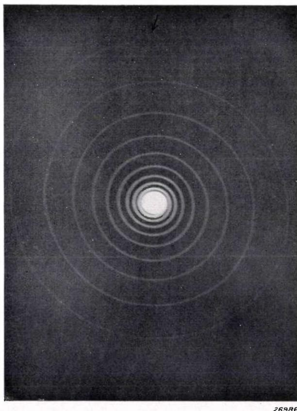
Fig. 5. Photograph for the determination of the scanning speed of a cathode ray tube DG 16. Electron current  $50 \mu\text{A}$ , anode voltage 2000 volts, ratio of size of photograph to object 1 : 1, aperture of lens 1 : 6.3, Agfa Isochrom plate.  $\omega = 2 \pi f = 2 \pi 1000$ . The spiral is still just visible for  $\varrho = 3.5 \text{ cm}$ . Maximum scanning speed 220 m/s. The enlargement of the reproduction is 1 : 3.
