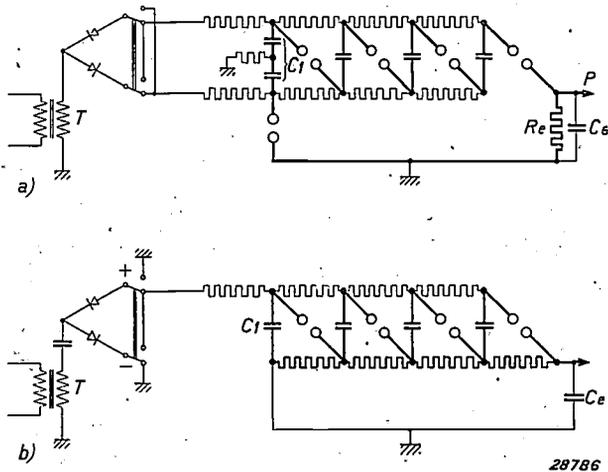
Fig. 1. Fundamental scheme of a uni-polar impulse voltage installation (four stages) a) with symmetrical charging generator, b) with uni-polar charging generator.  $T$  = high tension transformer,  $C_1$  = first impulse condenser,  $C_n$  = end condenser,  $R_n$  = discharging resistance. The test object is connected at  $P$ .
