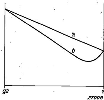
Fig. 4. Variation of potential between screen grid and anode in a tetrode; *a* without, and *b* with space charge. The space charge prevents the passage of secondary electrons from anode to screen grid.
