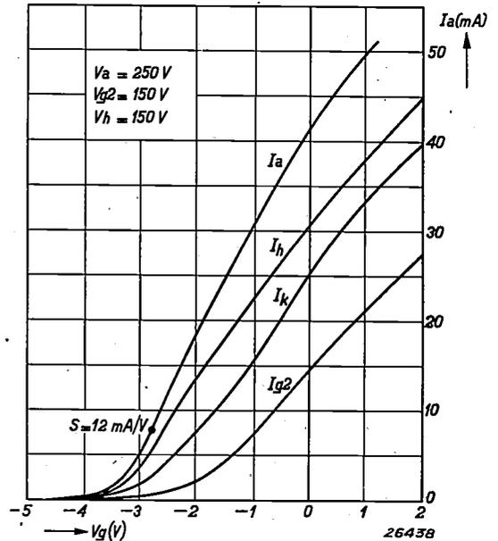
Fig. 13. Currents to the various electrodes of valve type 4696 as functions of the grid voltage  $V_g$ .  $I_a$  is the anode current,  $I_k$  is the cathode current,  $I_h$  is the current to the auxiliary cathode,  $I_{g_2}$  is the current to the screen grid.
