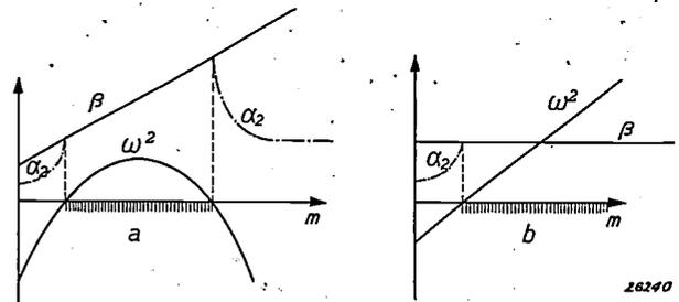
Fig. 3. Variation of  $\alpha_2$ ,  $\beta$  and  $\omega^2$  as functions of the amplification  $m$ . In the cross hatched area of the abscissa an oscillating adjustment must be made; outside of the area the adjustment is exponential.
