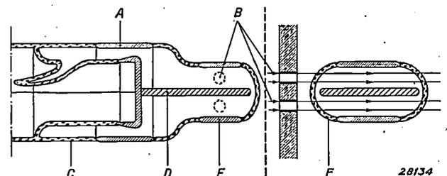
Fig. 5. Twin ionisation chambers for the automatic examinations of materials. A - earthed ring; B - beam of X-rays; the wall C is of a type of glass with very high insulating properties; D - exceptionally well insulated central electrode; E - electrodes connected directly to batteries. The wall F is made of a thin, very permeable type of glass.
