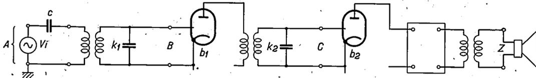
Fig. 1. Position of the sources of noise in a receiving set. The principal sources of noise are: first circuit  $k_1$  and first amplifier valve  $b_1$ , second circuit  $k_2$  and second amplifier valve  $b_2$ . The EMF induced in the receiver  $V_i$  acts in A. C represents the capacity of the aerial. The box represents the part of the apparatus not drawn.  $V_i$  causes the voltages  $V_i \gamma^{AB}$ ,  $V_i \gamma^{AC}$  and  $V_i \gamma^{AZ}$  in B, C and Z respectively.
