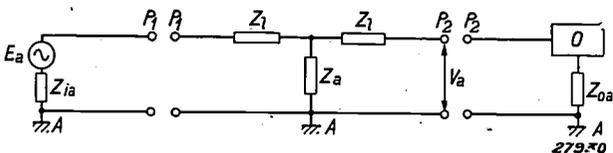
Fig. 7. Layout of the asymmetrical interference component. The interfering voltage  $V_a$  may be much greater than  $V_s$  (fig. 6), particularly when the earthing resistance  $Z_a$  of the mains is not too small.
