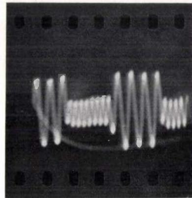
Fig. 6. Oscillogram of the voltage obtained by applying the heterodyne principle to the carrier in fig. 5 and an auxiliary voltage of  $10^7 +$  approximately 500 c/s. The differential frequency increases slightly with diminishing modulation voltage.
