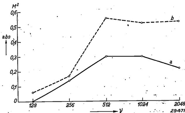
Fig. 7. The variation of the absorption per person in a hall as a function of the frequency  $\nu$ .
