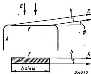
Fig. 5. Shape of the focus on the anode  $A$ . The electrons fall perpendicularly upon the anode ( $E$ ), the X-rays are observed at the angle  $\varphi$  ( $R$ ). The width of the focus is  $b$ , the length  $b/\sin \varphi$ , so that the focus is observed as a square in the direction  $\varphi$ .
