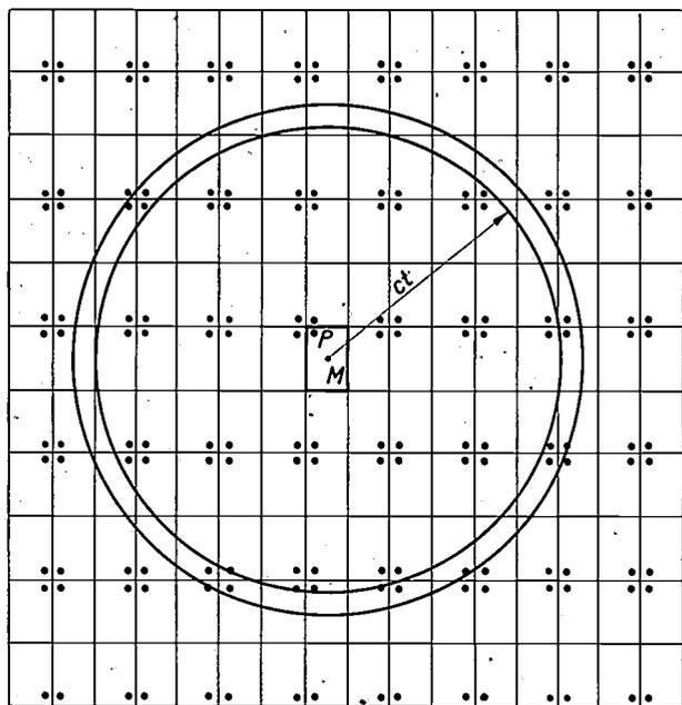
Fig. 4. Reflections of a sound impulse starting from *P* in a room with totally reflecting walls. Between  $t$  and  $t + \Delta t$  at *M* the sound from all the virtual sound curves lying between the two circles is heard. In this way the sound is always evenly distributed.
