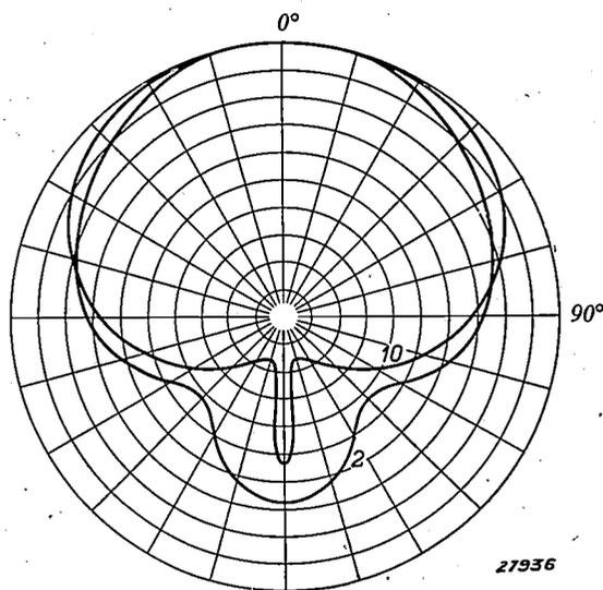
Fig. 3. Zone of silence behind an obstruction. Distribution of the sound pressure produced by a plane sound wave of wavelength  $\lambda$  at the surface of a sphere. The figures against the different curves are the values of the product  $ka$ , where  $k = 2\pi/\lambda$  and  $a$  is the radius of the sphere.
