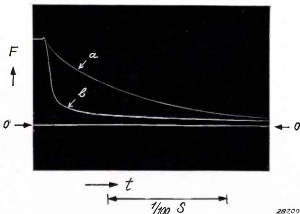
Fig. 9. Variation of the light intensity after interruption of the irradiation with ultraviolet light: a) for a phosphorescent silicate, b) for a phosphorescent sulphide.
