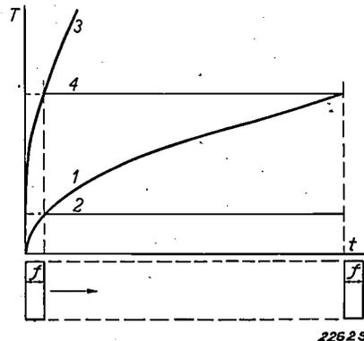
Fig. 2. Variation of the temperature  $T$  at the focus during loading. The initial temperature  $T_0$  is set equal to zero for the sake of simplicity. Curves 1 and 3 with stationary anode, curves 2 and 4 with rotating anode. The specific loading in curves 3 and 4 is four times as great as in curves 1 and 2.
