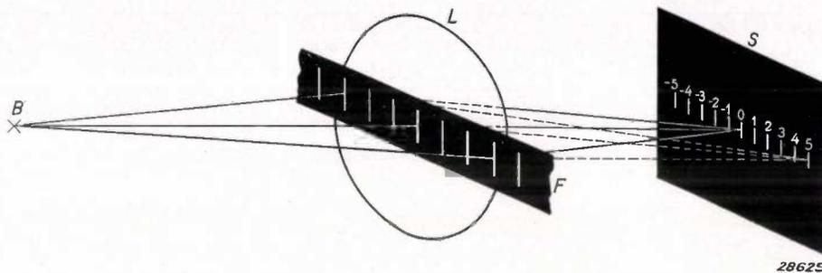
Fig. 1. Experimental arrangement for obtaining diffraction spectra. A point source of light  $B$  illuminates the strip of film  $F$  with practically parallel monochromatic light. On the screen  $S$  at the focus of lens  $L$  the diffraction spectrum may be seen. The strip of film  $F$  has a number of very narrow equidistant light transmitting slits. The spectrum now consists of a number of equidistant vertical lines.
