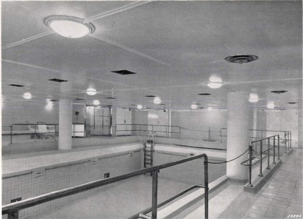
Fig. 9. The swimming pool of the "Nieuw Amsterdam" also has the low ceiling typical of ships. The plafonniers described in the text were used for the built-in illumination from above. By making the bowls of "Philippan" glass (see Philips techn. Rev. 3, 47, 1938) all the colours are deepened and the skin takes on a warm colour against the beautiful green of the pool.
