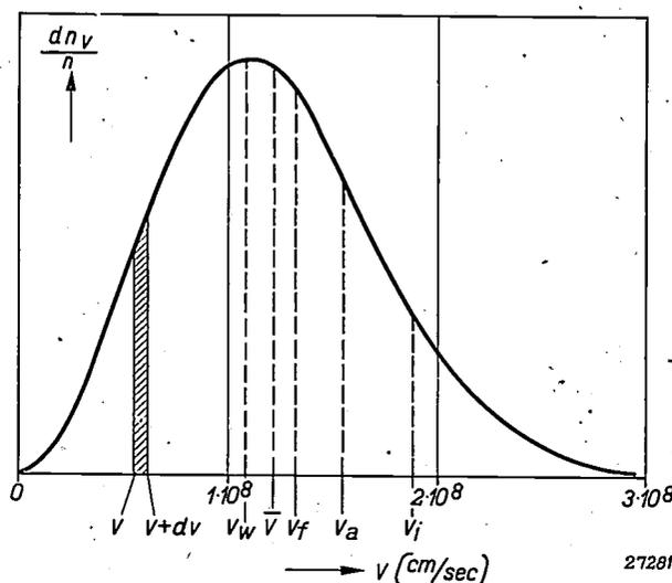
Fig. 4. Maxwellian distribution of the velocities of the electrons. The ordinates give the fraction  $dn_v/n$  of the electrons with a velocity between  $v$  and  $v + dv$ .  $v_w$ , velocity most commonly occurring,  $\bar{v}$ , average velocity, and  $v_f$ , quadratic average velocity. (The average energy in this example corresponds to a voltage of 5 volts,  $\frac{1}{2} m_e v_f^2 = e\bar{V}_e$ , where  $\bar{V}_e = 5$  volts).
