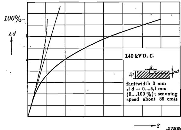
Fig. 3. Relationship between the depth  $\Delta d$  of the flaw expressed as a percentage of the wall thickness tested, and the signal strength  $S$ , in arbitrary units, with a flaw of constant width and a constant scanning speed.
