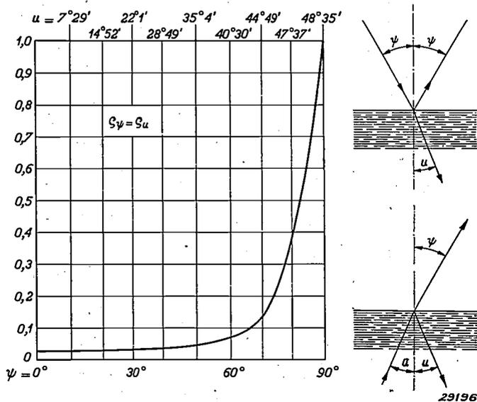
*Fig. 1.* Reflection coefficient  $\rho_{\Psi}$  for light falling on a water surface at an angle  $\Psi$  as a function of  $\Psi$ . The same curve gives the reflection coefficient of a ray which strikes the water surface from below at an angle  $u$ , as a function of  $u$  provided the angles  $\Psi$  and  $u$  are corresponding angles (see sketch above the diagram). This is expressed by noting the angle  $u$  as abscissa at the top of the diagram.
