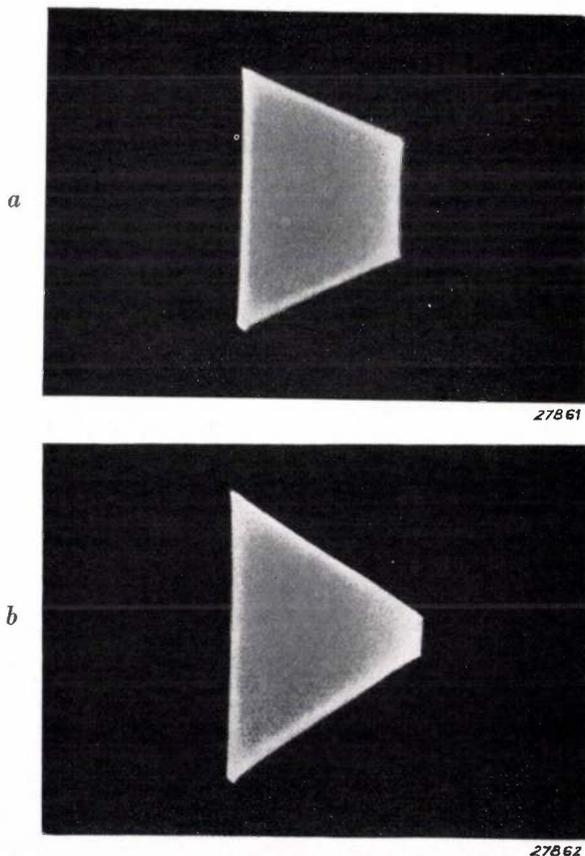
Fig. 3. Oscillogram of the same modulated high-frequency signal as in figs. 1 and 2, but plotted as a function of the instantaneous value of the modulation voltage instead of time. *a*) 35 per cent modulation, as in fig. 1; *b*) 75 per cent modulation, as in fig. 2.
