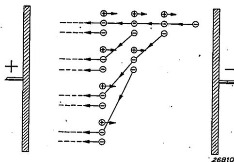
*Fig. 2.* Diagrammatic representation of an electron avalanche.
