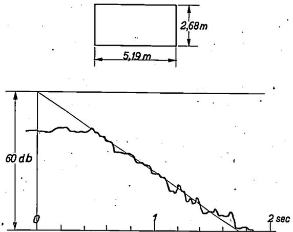
Fig. 1. Recording of the sound intensity in a room as a function of the time. The reverberation time is 1.75 sec. Above, a vertical cross section of the room.
