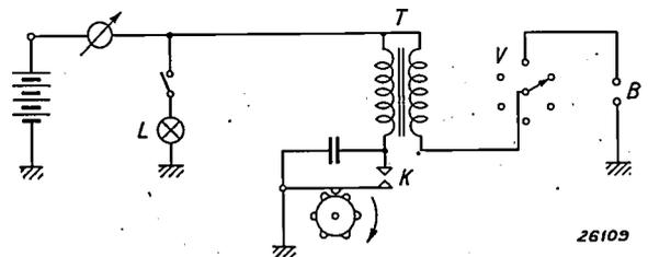
*Fig. 3.* Diagram of the ignition system. *K* is the "make and break" contact. The transformer *T* is the ignition coil, and *V* is the distributor through which the current is led to one of the sparking plugs *B*. *L* is the lighting circuit of the car which also is connected to the accumulator.
