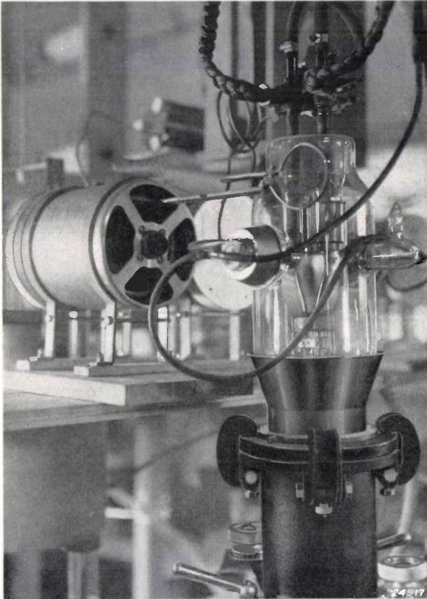
Fig. 1. The water-cooled output valve TA 20/250.
