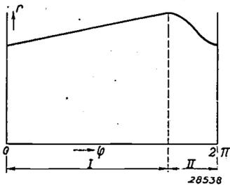
Fig. 4. Fundamental form of the development of the cam disc *K* (radius *r* as a function of the angle  $\varphi$ ). The curve also gives the variation of the displacement of the light spot on the film with the time. In part *I* scanning takes place, in part *II* the back flash.
