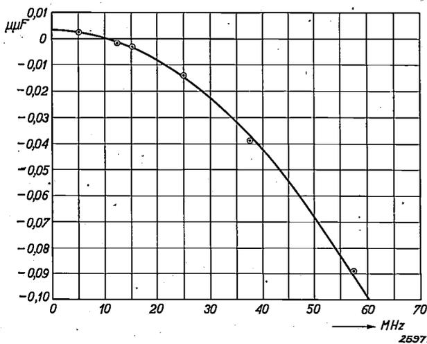
Fig. 6. The capacity  $C_{ga}$  of an AF3 valve plotted as a function of the frequency. Points measured. Curve drawn is given by the formula:  $C_{ga}' = (0.0030 - 0.285 \times 10^{-4}v^2) \mu\mu F$ , where  $v$  is in megacycles per sec. It may be seen that the measured points fall satisfactorily on the second order curve in agreement with formula (8).
