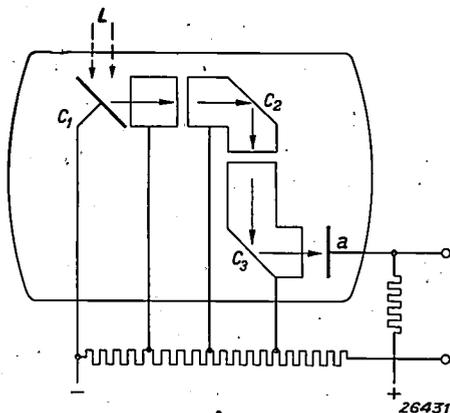
Fig. 3. L-electron multiplier,  $c_1$  photo-cathode,  $c_2, c_3$  secondary cathodes and  $a$  final anode. The cylindrical tubes serve as focussing electron lenses, the arrows indicate approximately the path of the electrons.
