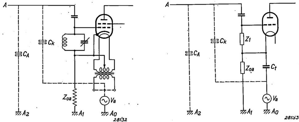
Fig. 8. Circuit of the input component of a receiver, with associated equivalent circuit. It is shown here how the asymmetrical interfering voltage  $V_a$  produces an alteration in voltage at the control grid of the high-frequency amplifying valve. This alteration in voltage is produced by currents which flow either through the capacity  $C_k$  between the aerial and the mains conductors or through the capacity  $C_t$  between the primary and secondary windings of the mains transformer.
