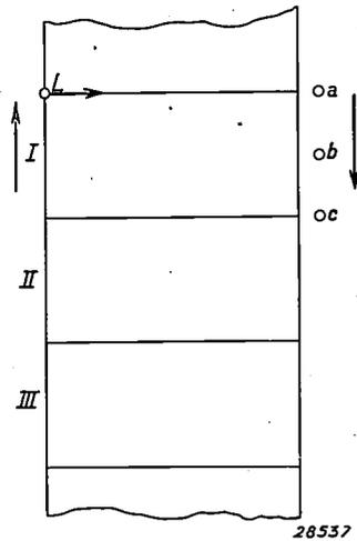
*Fig. 2.* Interlaced scanning of the film. The section of film moves in the direction of the left-hand arrow. The light spot *L* is projected through the holes in the Nipkow disc which move across the film picture. The light spot must be given a vertical motion equal and opposite to the motion of the film (arrow, right), and it must jump from the height *c* to *a* periodically.
