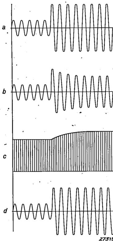
not only must we choose the characteristic of the expander correctly, but we must in addition make the process of regulation in the expander such that the effect of regulation in the compressor is completely cancelled. This is actually possible, and consists of making the time lags of compressor and expander the same.
