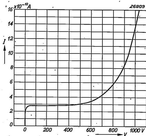
*Fig. 1.* Variation of the current as a function of the voltage between two large parallel plates (diameter 80 mm, separation 24 mm) with auxiliary ionization in the gas by X-rays. (Argon at a pressure of 27.6 mm).
