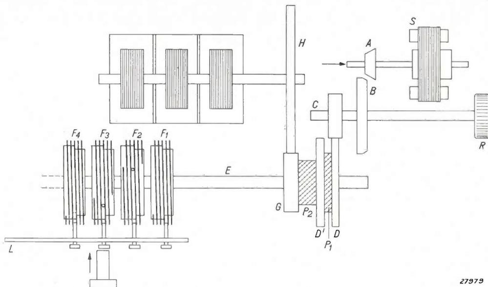
Fig. 1. Diagram of the mechanism of motor-driven push-button tuning. *S* = motor, *A-B* = friction drive, *C-D* and *G-H* = toothwheel transmissions, *F<sub>1</sub>, F<sub>2</sub> ...* = tuning cylinders *P<sub>1</sub>* and *P<sub>2</sub>* = friction couplings; *R* = knob for hand tuning, *L* = contact bridge.
