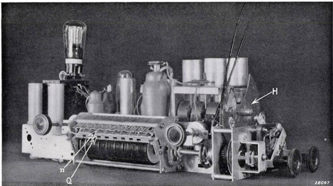
Fig. 4. Photograph of the push-button tuning arrangements mounted in the receiver. In the middle is the keyboard, to the right the motor and transmission. The locking arrangement *Q* holds down the key pressed: the end of the key *n* falls into the corresponding opening of the beam *Q*. When another key is pressed the beam *Q* is first pushed away against the action of a spring (visible in fig. 3 to the left), and the key previously held is thereby released.
