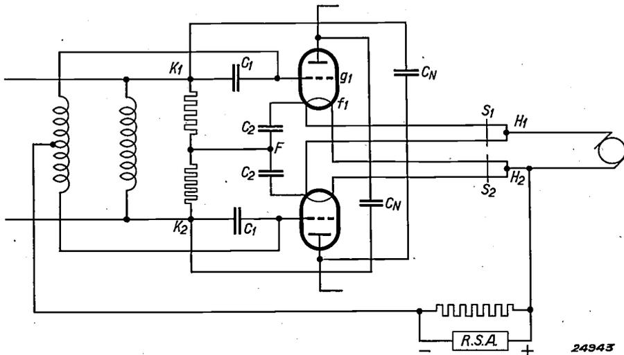
Fig. 9. Circuit diagram of two transmitting valves in parallel.  $H_1$  and  $H_2$  feeder terminals for the filaments  $f_1$  and  $f_2$ .  $S_1$  and  $S_2$  adjustable bridges for tuning the Lecher systems. R.S.A. is the grid bias voltage apparatus.
