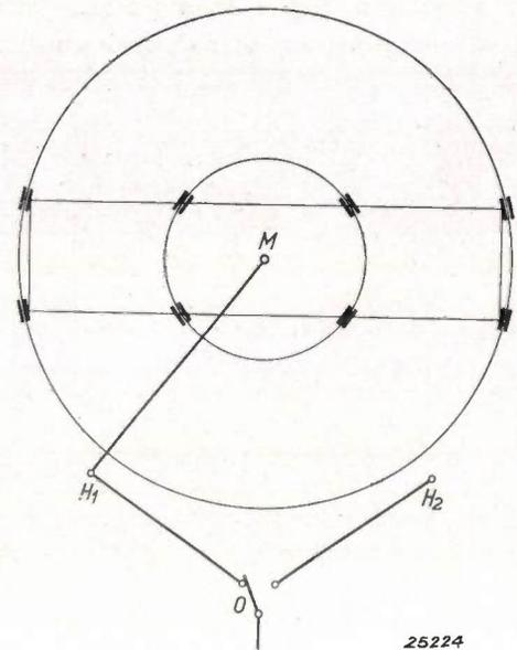
Fig. 8. Diagram of the supply of the aerial. The aerial can be fed from  $O$  via  $H_1$  or  $H_2$  to  $M$ .
