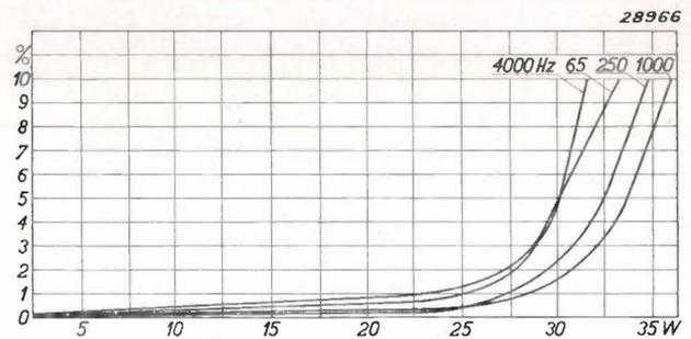
Fig. 10. Distortion characteristic of amplifier *C*<sub>2</sub> at different frequencies.
