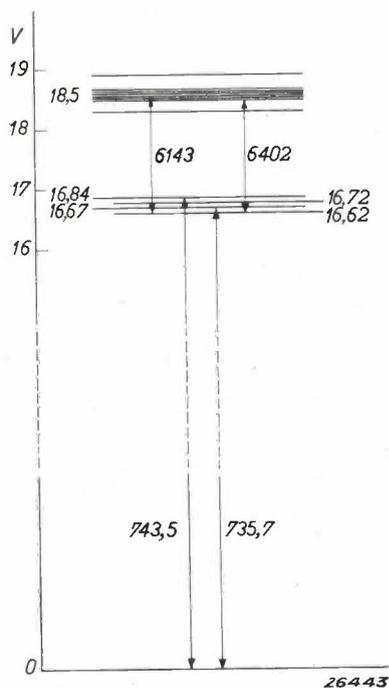
Fig. 7. Energy level diagram of a neon atom.
