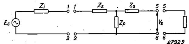
Fig. 6. A detailed scheme of the symmetrical interference component. The interfering voltage  $V_s$  is generally small compared with  $E_s$ , because the parallel impedance  $Z_p$  between the mains conductors is usually very small owing to their mutual capacity.
