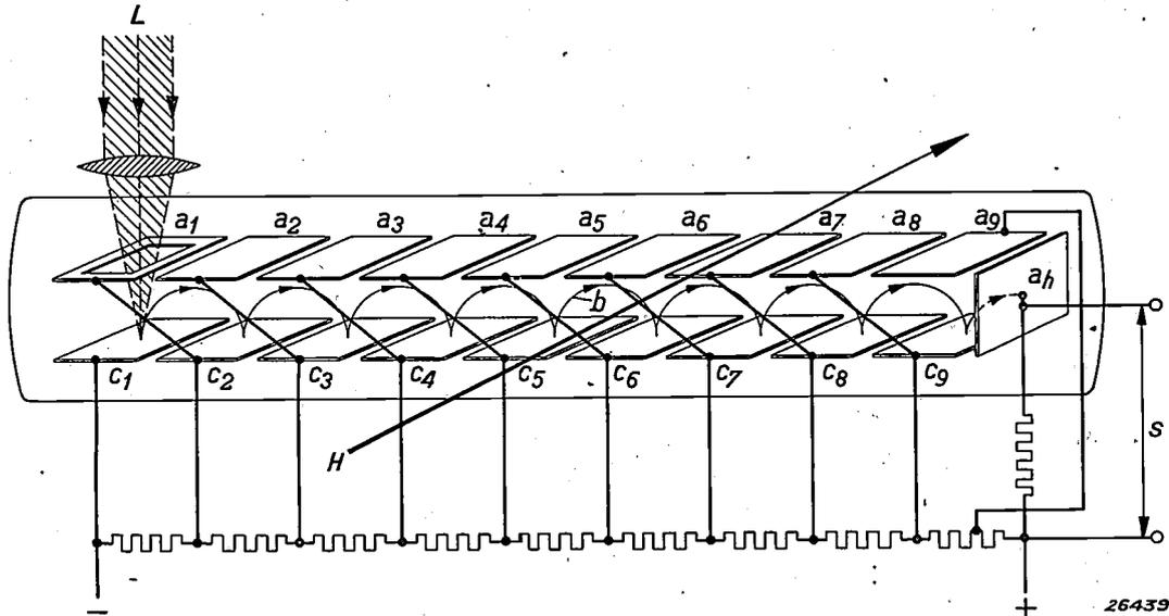
Fig. 6. Electron multiplier with magnetic focussing.
