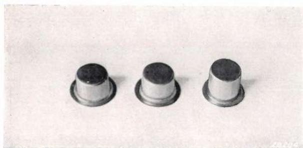
*Fig. 4.* Shell bodies made of zirconium sheet by application of a deep drawing process.
