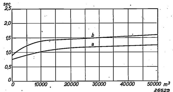
*Fig. 12.* Reverberation time for the spoken word as a function of the volume of the room, according to Knudsen. Upper curve: recommended values for ordinary theatre auditoria, lower curve: reverberation times at which intelligibility is at a maximum.
