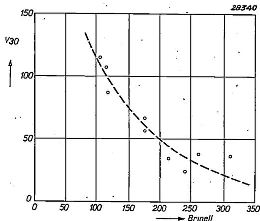
Fig. 2. The cutting speed in m/min. for a cutting edge life of 30 min ( $v_{30}$ ) as a function of the hardness in Brinell units with a ball diameter of 10 mm, a load of 3000 kg and a loading time of 30 sec.
