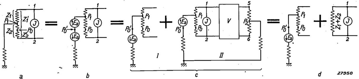
Fig. 4. Four similar equivalent circuits of the input in fig. 3. By introducing an asymmetrical e.m.f.  $E_a$  in such a way that the potential of  $P_0'$  is made equal to that of  $P_0$ , the source of interference can be subdivided into two components *I* and *II* (fig. c) of which the symmetrical component *II* produces no flow of current to earth.
