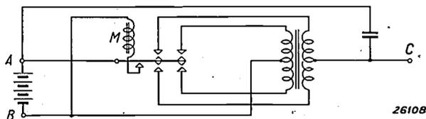
*Fig. 2.* Construction of the vibrator converter with a second set of contacts, whereby the current direction is reversed simultaneously in the primary and in the secondary winding of the transformer. This makes the use of a rectifier unnecessary. The anode voltage is taken off between the terminals *A* and *C*.
