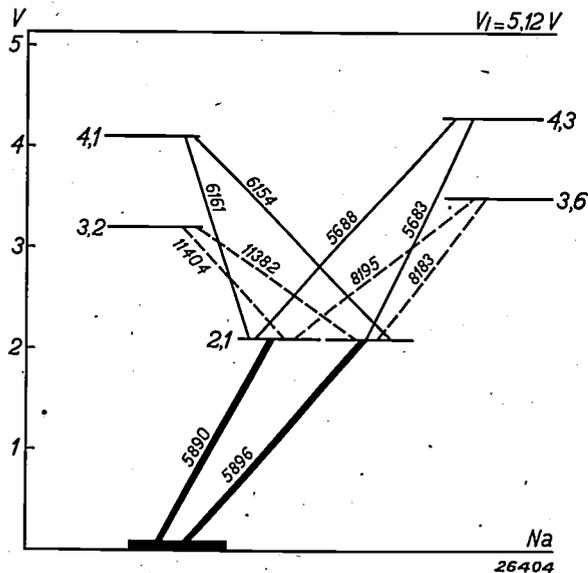
Fig. 1. Energy level diagram of a sodium atom. The lines indicate possible transitions (broken lines lie outside the visible part of the spectrum). The numbers indicate the wave length in Å of the spectrum line corresponding to the transition.
