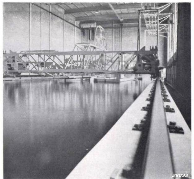
Fig. 10. Truck for towing models of ships at the testing station in Wageningen. The truck runs on two rails over a tank 10.5 m wide, 5.5 m deep and 160 m long. It is driven by four motors each of 20 H.P. fed with a voltage kept constant by means of a voltage regulator.
