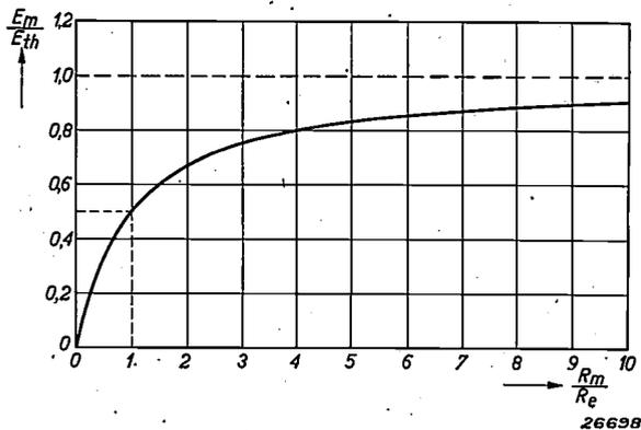
Fig. 4. Drop in terminal voltage of the thermocouple, when current is taken off by the meter.  $E_m/E_{th}$  is plotted as a function of  $R_m/R_e$ . When  $R_m = R_e$ , the most favourable energy transfer takes place.
