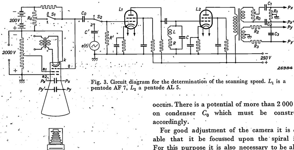
Fig. 3. Circuit diagram for the determination of the scanning speed.  $L_1$  is a pentode AF 7,  $L_2$  a pentode AL 5.
