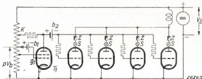
Fig. 5. Diagram of a voltage regulator with triodes.
