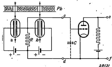
Fig. 1. Arrangement of two ionisation chambers *a* and *b* in a compensation circuit, enabling measurements to be made independent of simultaneous and equal fluctuations in the intensity of the two X-ray beams (fluctuations in mains voltage). A lead screen with two apertures for the passage of the beams is placed in front of the chambers.
