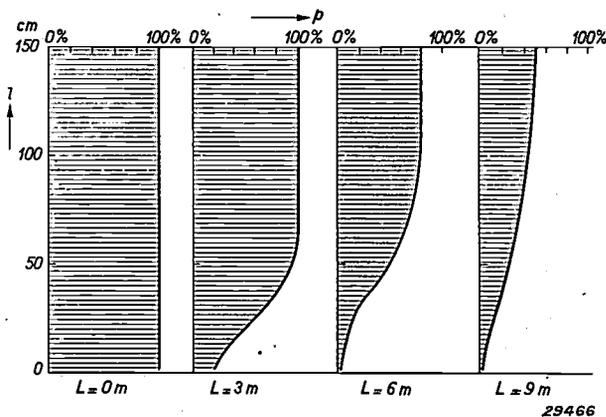
Fig. 3. A plane sound wave which proceeds parallel to a wall of absorbing material, is reduced in intensity close to the wall. The longer the distance along the wall covered by the wave, the greater the distance from the wall at which this weakening may be observed. The sound pressure  $p$  in per cent of the original value is plotted as a function of the distance  $l$  to the wall for several values of the distance  $L$  covered by the sound wave along the wall.
