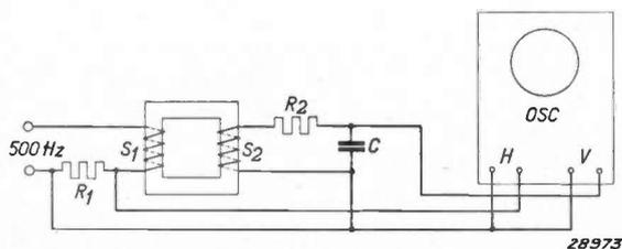
Fig. 4. Circuit for recording hysteresis loops. The voltage at the coil  $S_2$  is proportional to  $dB/dt$ . If the impedance of  $C$  is small with respect to  $R_2$  the voltage at  $C$  is proportional to the momentary value of  $B$ .
