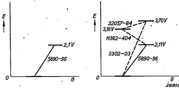
Fig. 9. Simplified diagram of the sodium spectrum. If only the 2.1 volt level is excited only the yellow lines with  $\lambda = 5890$  and  $5896 \text{ \AA}$  are emitted. When the 3.7 volt level is excited lines outside the visible spectrum are emitted also  $G = \text{ground, or zero state.}$
