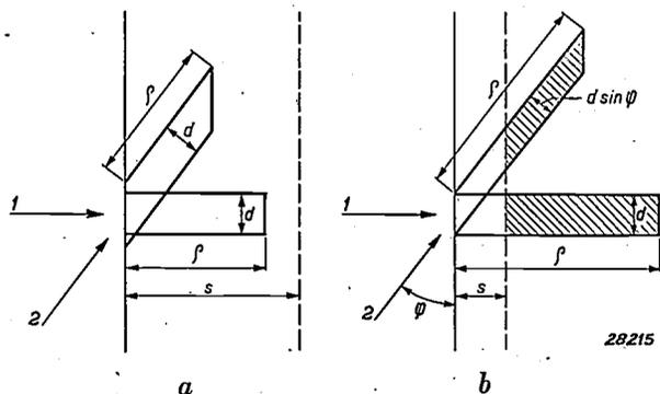
Fig. 3a) Body radiation. The depth  $s$  of the emitting layer is greater than the depth  $\lambda$  of the layer which contributes to the light emitted. Upon normal (1) and oblique (2) direction of observation the same light intensity is obtained from the same apparent surface ( $d$ ). The brightness is therefore the same in all directions (Lambert's law).
