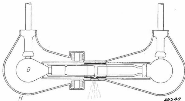
Fig. 7. For the cooling of the support  $K$  in fig. 6 a cooling bulb  $B$  is mounted on it, which gives off its heat by convection to the surrounding air and by radiation to the earthed container  $H$  of the tube.
