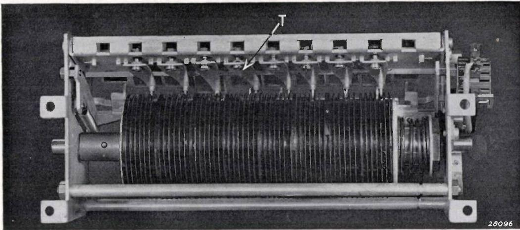
Fig. 3. Photograph of the keyboard, taken from the rear. The long strips carrying the pegs may be seen. To the right are the contacts which serve for starting and reversing the motor. The third from the left is pushed down.
