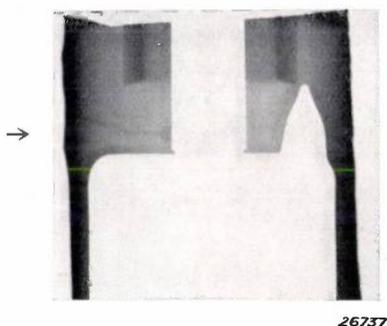
Fig. 3. Breakdown in a terminal for the connection of a high tension cable with an X-ray tube. The cause (a gas bubble in the cement) and the track of the breakdown may be clearly seen (at →).
