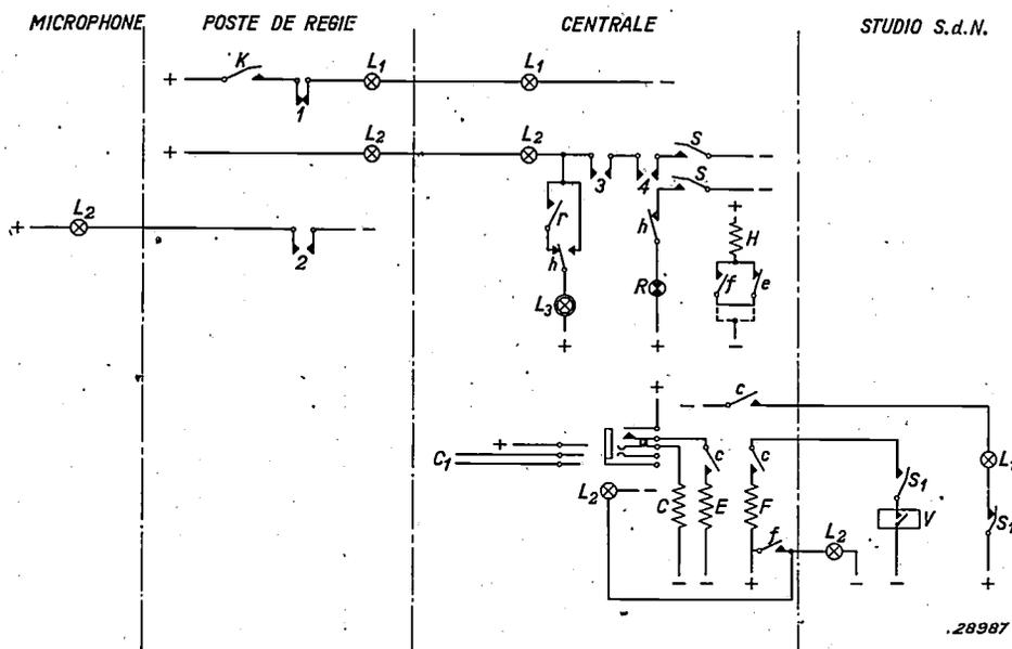
Fig. 12. Simplified diagram of the signaling system in which all relay contacts are shown in the currentless state.
