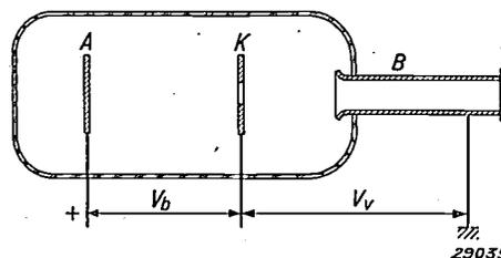
Fig. 1. Diagram of a canal ray tube. By a discharge between  $K$  and  $A$  ions are produced which pass through a canal in the cathode  $K$  and are accelerated by a voltage  $V_v$  between  $K$  and  $B$ . The ions may be allowed to strike a target at  $T$ .
