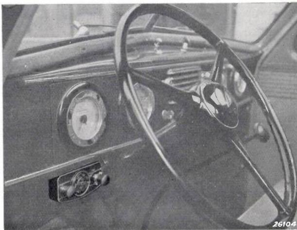
Fig. 8. Operation box under the dashboard.
