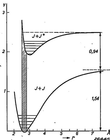
Fig. 10. Potential curves of an iodine molecule. The potential energy  $V$  in electron volts counted from the level corresponding to the lowest state as a function of the mutual separation  $r$  of the nuclei in Å. The vibration levels 0, 5, 10, 15, 20 and 25 are drawn.
