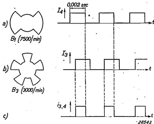
Fig. 9. a) Variation with time of the light flux  $I_4$ , falling on the photocell  $E_4$  and periodically interrupted by the disc  $B_1$ .
