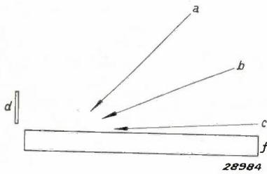
Fig. 3. Comparison of the reflective power of a wet slab upon observation from the directions a ( $60^\circ$ ), b ( $75^\circ$ ) and c ( $89^\circ$ ). The word STOP is written on the slab. On the board d there is an inscription in mirror script. Fig. 4 shows how the board is reflected better and better with increasing angle of incidence, while the inscription on the slab itself becomes vaguer and vaguer.
