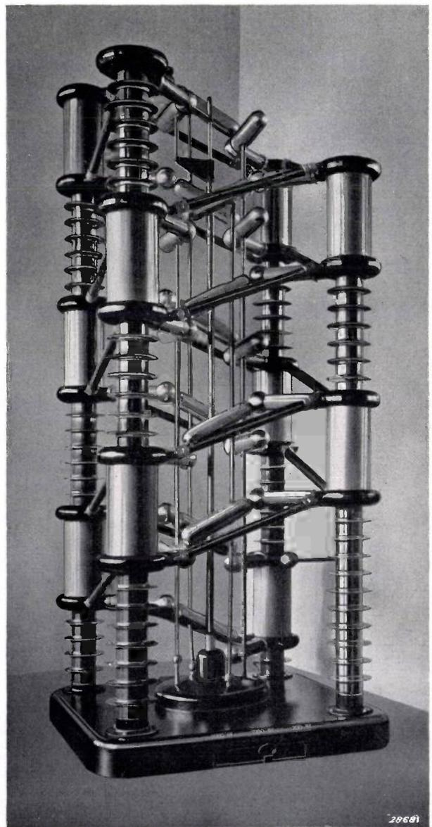
Fig. 3. Impulse generator with a impulse energy of 25 kW sec, commutable for 2000, 1000 and 200 kV (with 0.0125, 0.05 and 1.25  $\mu$ F respectively). Height 4.5 m, base 2x2 m. In this type the large "Philit" cylinders are not yet used, so that the condensers may easily be distinguished from the insulators.
