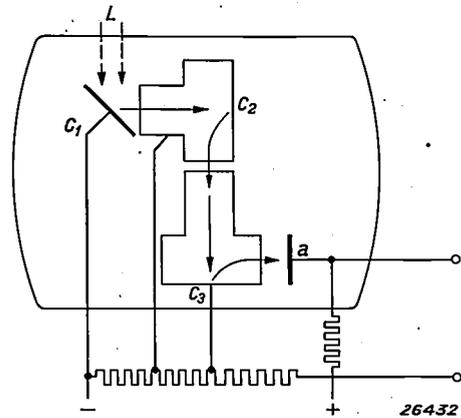
Fig. 4. T-electron multiplier. Explanation as in fig. 3.
