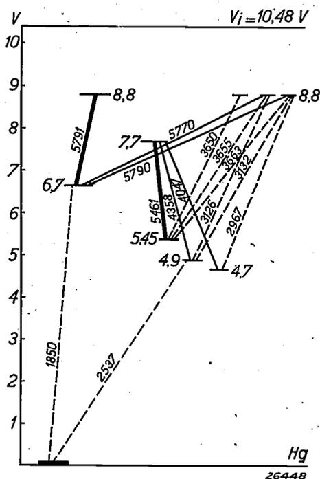
Fig. 3. Energy level diagram of a mercury atom.
