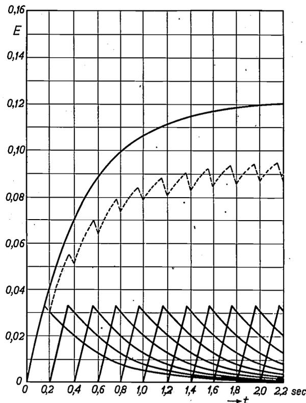
Fig. 7. Growth and fading of the sound in a space with a reverberation time of 6 sec. The sound consists of syllables which have a constant intensity for 0.15 sec and which are separated by intervals of silence of 0.05 sec. The intensity of the syllables projects only slightly above the average sound. The intelligibility is therefore poor.
