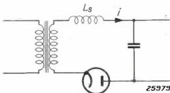
Fig. 3. Circuit diagram of a rectifier valve.
