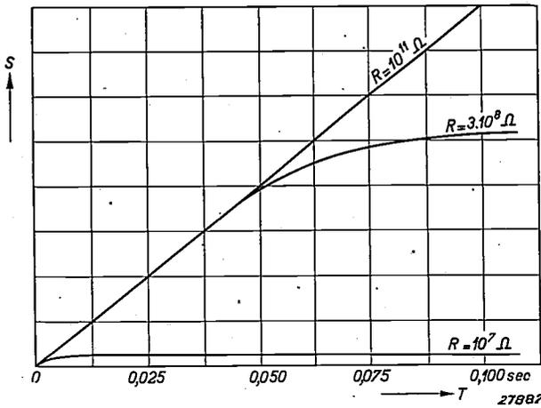
Fig. 7. Variation of the maximum signal strength  $S$  in arbitrary units with variable scanning speed  $v$ . The time  $T$  which the flaw takes to pass the chamber is plotted along the abscissa (see fig. 6);  $T$  is the quotient of the diameter of the flaw  $a$  and the scanning speed  $v$ .
