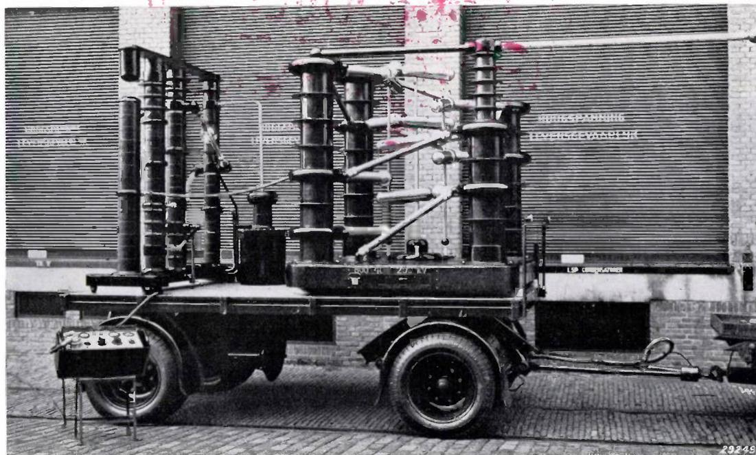
Fig. 7. Transportable impulse voltage installation with an impulse energy of 10 kWsec for 800 kV commutable for 400 and 200 kV. Surface of the trailer 2.20·4 m<sup>2</sup>, total height from the earth 3.30 m.
