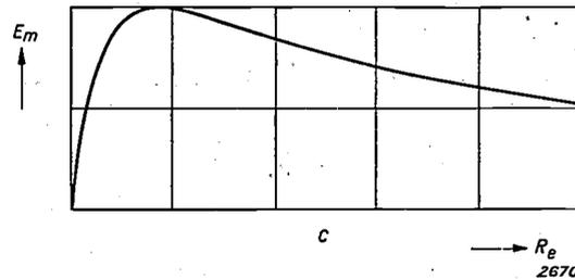
Fig. 5. c) Voltage on the meter as a function of the resistance of the thermocouple at a constant current through the filament.
