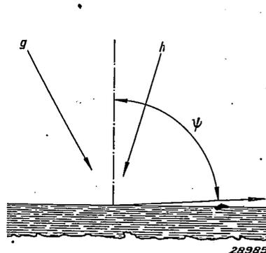
*Fig. 2.* In the direction of observation  $\Psi = 89^\circ$  only that light is observed which has been reflected at the water surface, and thus satisfies the conditions of specular reflection. Light which has penetrated into the water is practically unable to emerge at an angle of  $90^\circ$  (see under *fig. 1*).
