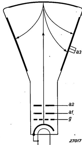
Fig. 9. Construction of a cathode ray tube. The collecting electrode  $a_3$  has the function of providing that the fluorescent screen shall assume a positive potential upon being bombarded with electrons, and in addition of capturing the secondary electrons.
