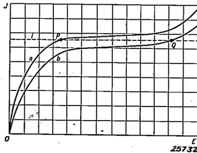
Fig. 9. Two barretter lamps of the same type, with slightly differing characteristics may have quite different working points *P* and *Q* at the same current. Because of this regulator lamps may not be connected in series.
