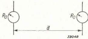
Fig. 6. Lecher system of round wires with a radius  $R_0$  and a distance  $d$  between them.
