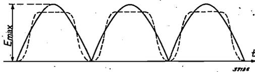
Fig. 4. Variation of the tube voltage with the time. The broken line gives the variation of the current which is in phase with the voltage. In each half period the current reaches a saturation value at a certain voltage. This current is given by the cathode emission.
