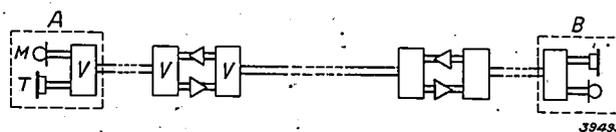
Fig. 3. If the distance between two subscribers *A* and *B* is great, repeaters are inserted in the line at regular intervals. Since repeaters give transmission in only one direction there are always two side by side, one for each direction, with a fork at each side in the case of a two-wire connection.
