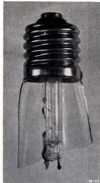
Fig. 3. Photograph of a series lamp which has been destroyed by an arc discharge.
