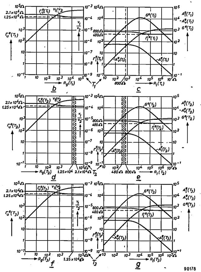
Fig. 10. Some important quantities plotted for the Philips OC 71 transistor in the common-emitter configuration (hence the e indices to the upper-right of symbols). All axes are on logarithmic scales. D.C. biasing (operating point):  $I_C = -3$  mA,  $V_{ce} = -2$  V.
