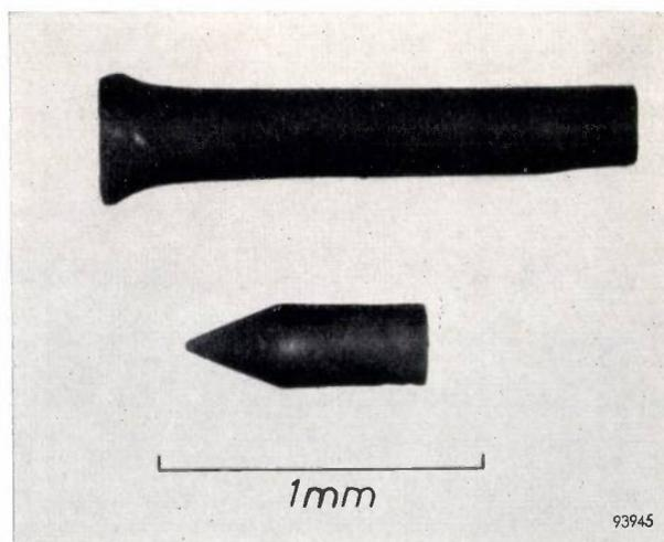
Fig. 4. Above, shadow photograph of diamond cylinder as bored from diamond platelet; below, shadow photograph of a finished stylus, 0.3 mm diam., 0.6 mm long.
