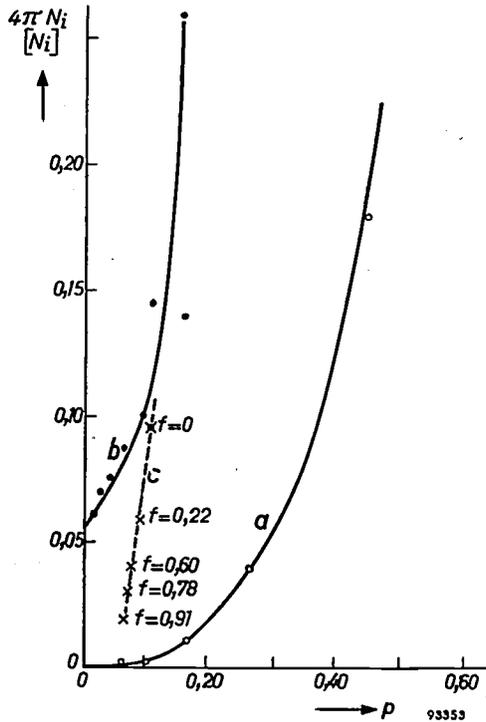
Fig. 11. The internal demagnetization factor  $N_i$  as a function of porosity  $p$ : a) for ferrocube; b) for unaligned ferroplana; c) for aligned  $\text{Co}_2\text{Z}$  with various degrees of alignment  $f$ .
