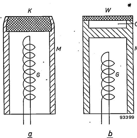
Fig. 1. a) A simple way of fitting a flat impregnated cathode (K) in a molybdenum holder. The latter consists of a cylinder (M) with a supporting ridge, in which the cathode disc, i.e. the porous aluminate-impregnated tungsten body, is fixed by bending over the lip of the cylinder. The heater filament (G) is pushed into the cylinder.
