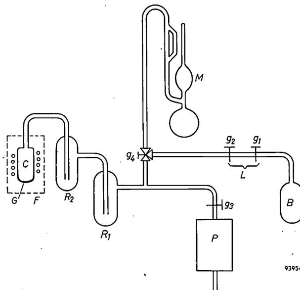
Fig. 13. Set-up used for measuring the absorption capacity for carbon monoxide. The letters have the same meaning as in fig. 6. The amount of gas admitted to *C* can be accurately controlled by the three-way cock  $g_4$  and the MacLeod gauge *M*. The extra liquid-air trap  $R_2$  was found necessary in those experiments in which the bulb wall was at a temperature lower than room temperature. *F* represents the heating or cooling device, as the case may be.
