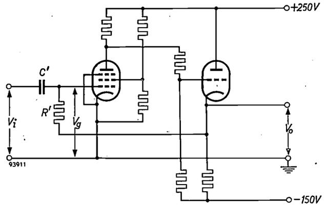
Fig. 5. Differentiator ( $C'$  and  $R'$ ) with amplifier.  $R'$  is connected to the output (triode cathode follower).
