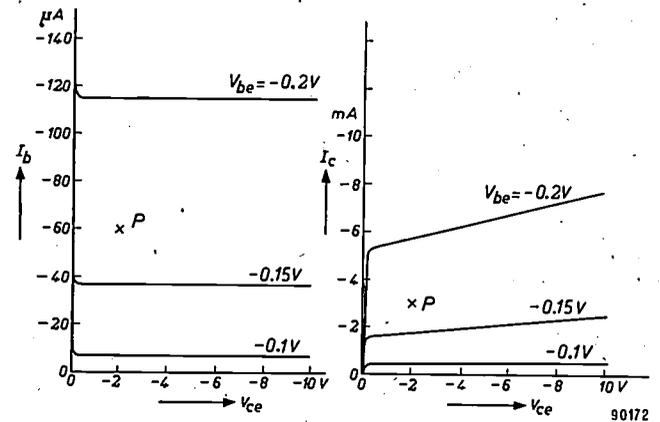
Fig. 2. Example of a pair of families of curves completely describing the properties of a transistor — here the Philips OC 71 — at low frequencies. The OC 71 being a transistor of the P-N-P type, all the quantities in the above graphs turn out to be negative. The biasing of the transistor might give an operating point at  $P$ , for example.
