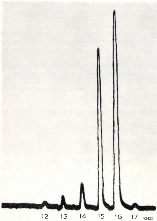
Fig. 4. A typical spectrogram. The peaks occur at frequencies which correspond, according to (1), to  $M = 12, 13, 14, 15, 16$  and  $17$  (the ions carrying a single elementary charge  $e$ ); these peaks are almost entirely attributable to  $C^+$ ,  $CH^+$ ,  $CH_2^+$ ,  $CH_3^+$ ,  $CH_4^+$  and  $C^{13}H_4^+$ , respectively.
