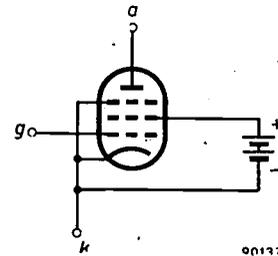
Fig. 3. A pentode has more than three terminals, but if screen and suppressor grids are given fixed potentials with respect to the cathode only three terminals are left, as is the case with a triode or transistor. Through the terminal marked *k* flows the sum of the cathode, screen-grid and suppressor-grid currents.
