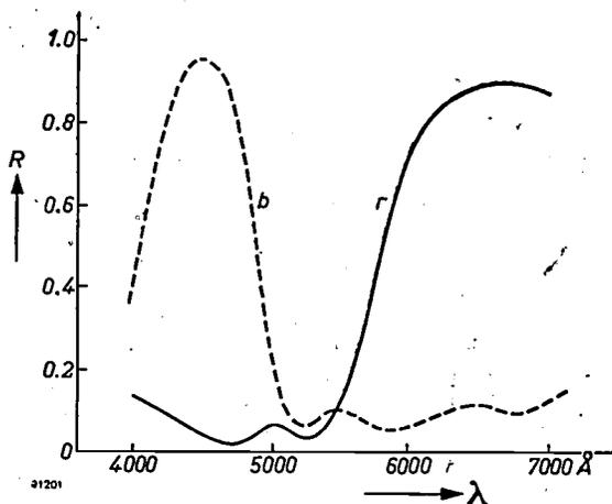
Fig. 6. Measured reflection coefficient  $R$  of two dichroic mirrors as function of the wavelength;  $r$  for a red,  $b$  for a blue reflecting mirror.
