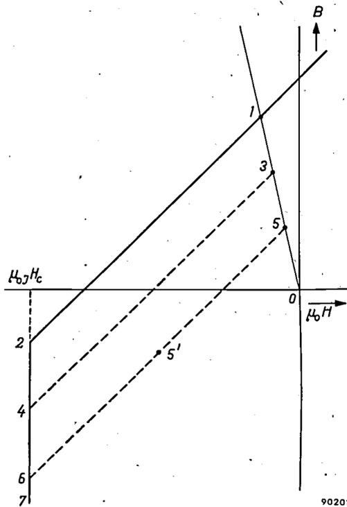
Fig. 9. 1-2-7 is part of the  $B-\mu_0 H$  curve of strongly magnetized ferroxdure, 3-4-7 the same for a more weakly magnetized ferroxdure, and 5-6-7 for a still more weakly magnetized ferroxdure. 0-1 working line of a ferroxdure magnet incorporated in a magnetic circuit. Working point 1 is impracticable (safety factor less than 1), 3 represents the critical case (safety factor = 1), and 5 permits a safety factor = 2.
