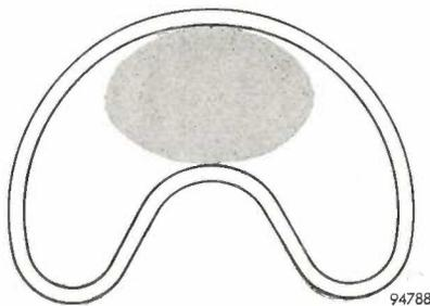
Fig. 4. Cross-section of the "Power-Groove" lamp (General Electric<sup>3)</sup>). The discharge is more or less concentrated in the shaded part; in the lower points of the cross-section the wall remains at a lower temperature.
