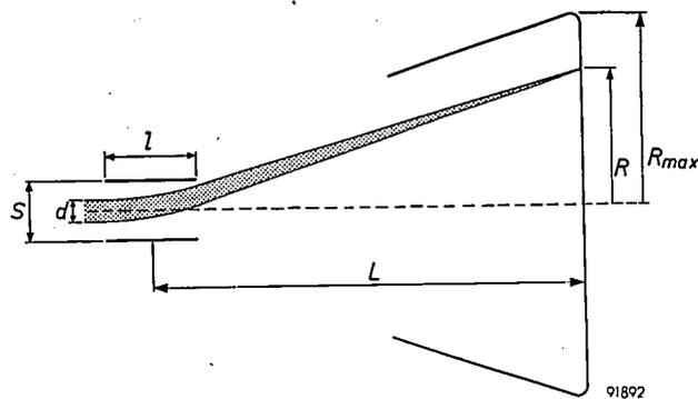
Fig. 5. The deflection of an electron beam by flat parallel plates.
