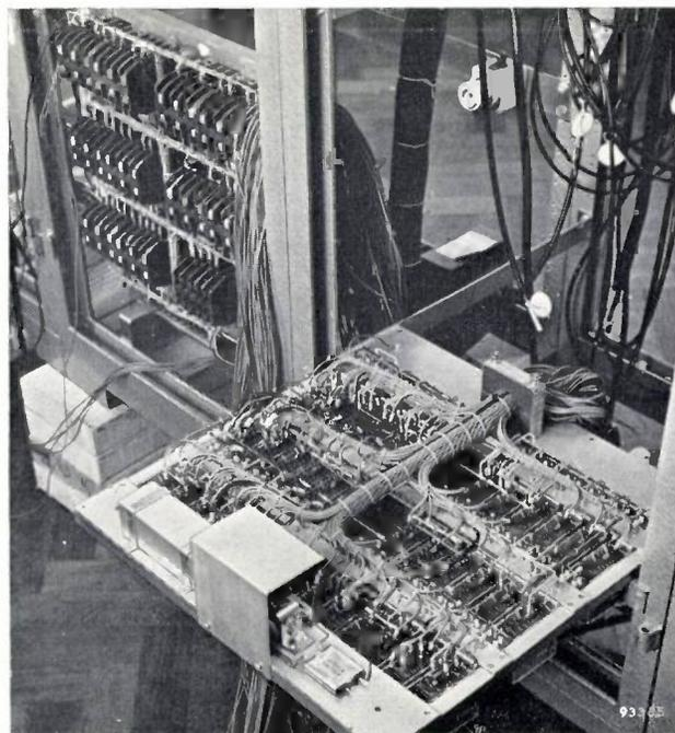
Fig. 5. Relay banks for servomotors and safety channels, one of the relay panels having been lowered for inspection.
