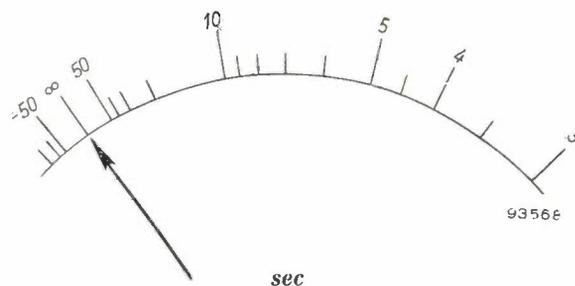
Fig. 10. Scale of period meter for high neutron flux. When the reactor is operating in the stationary state, the meter needle shows infinity. A positive deflection indicates increasing power, a negative deflection decreasing power. Audible and visible alarm signals are given if  $T$  drops below 10 sec; "fast scram" results automatically if  $T$  drops below 3 sec.
