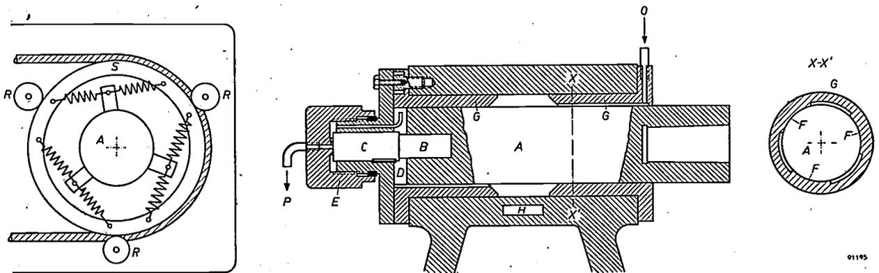
Fig. 1. Construction of the precision headstock. A steel shaft running in bronze bearing block *G* (which has three bearing surfaces *F*, see section *XX'* on right). *B* improved-wood end-piece; *C* metal thrust bearing block, which may be moved axially by means of the micrometer screw *E*. In the space *D* a constant pressure, beneath atmospheric, is maintained. *H* heating element. *O* oil inlet, *P* oil outlet.
