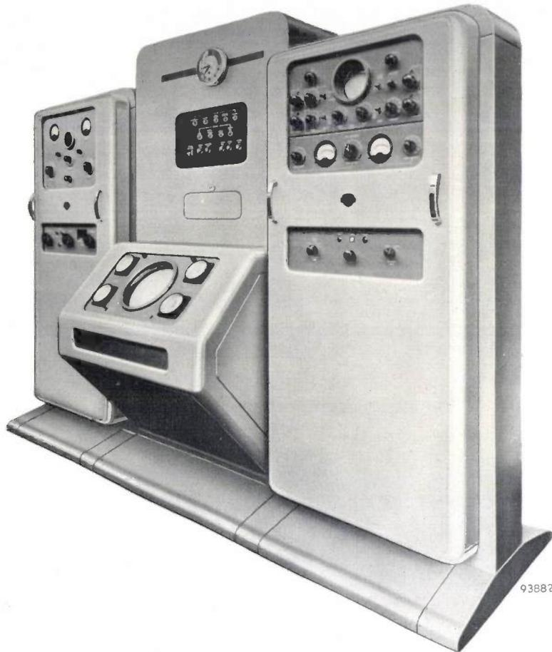
Fig. 4. The radar console. The left-hand unit contains the 50 kW transmitter, the right-hand unit the 10 cm wave receiver and the automatic ranging and aerial-alignment equipment. The centre unit is the display and control system.
