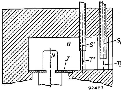
Fig. 9. Cross-section of the output guide, in which the iris is denoted by  $S_i$ ,  $T_i$ , and the reactive element with which the coupling is adjusted is denoted by  $S'$ ,  $T'$ . For the meaning of letters  $B$ ,  $N$  and  $J$  see *fig. 1*.
