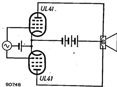
Fig. 1. Output stage with two pentodes UL 41 and a split-coil loudspeaker (type 9754) without output transformer. The resistance of the speech coil is 2 × 2000 ohms.
