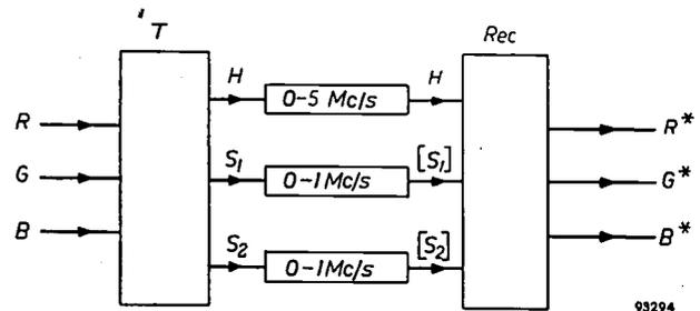
Fig. 11. Colour television system in which the transmitted signals consist of a luminance signal  $H$  and two colour signals,  $S_1$  and  $S_2$ , which are linear combinations of the signals  $R$ ,  $G$  and  $B$ . The signal  $H$  is radiated from the transmitter  $T$  to the receiver  $Rec$  with a bandwidth of 5 Mc/s, the signals  $S_1$  and  $S_2$  with a reduced bandwidth, e.g. of the order of 1 Mc/s.
