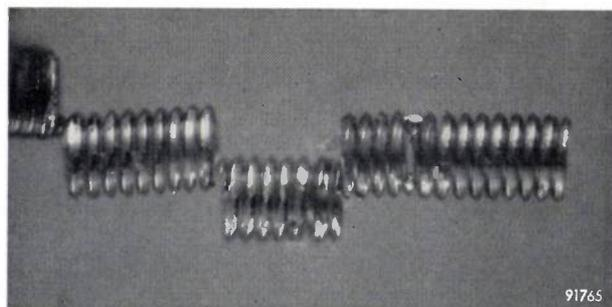
*Fig. 1. Above: Schematic diagram showing "offsetting" in a tungsten filament along crystal boundary planes which are roughly at right-angles to the wire axis. Below: Photograph of a coiled tungsten filament in which offsetting has occurred at various points.*
