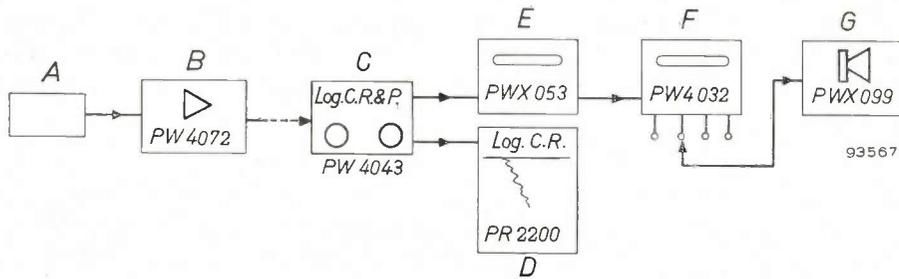
Fig. 6. Block diagram of measuring channel for low neutron flux. *A* fission chamber, *B* pulse amplifier, *C* logarithmic count-rate and period meter, *D* automatic recording potentiometer, *E* pre-set time unit, *F* pulse counter, *G* loudspeaker unit.
