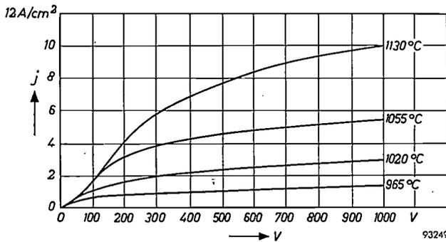
Fig. 4. Current density  $j$  of a pressed cathode (with CaO), measured in a diode and plotted as a function of the applied anode voltage  $V$  at various cathode temperatures.
