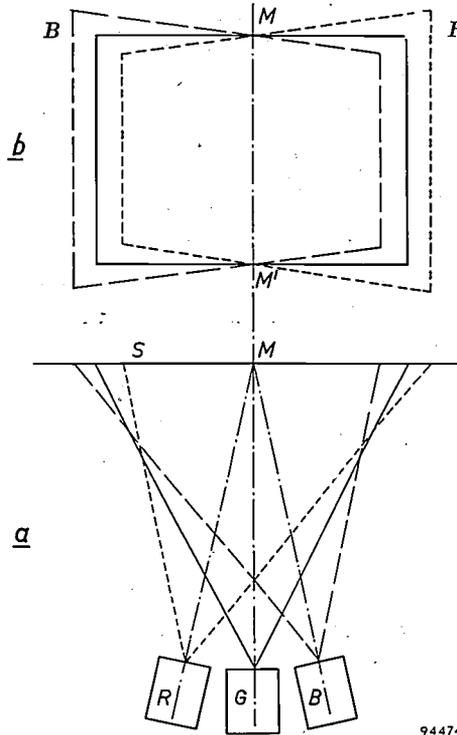
Fig. 5. a) Arrangement whereby the three primary-colour projectors R, G and B are placed side by side, with the two outer ones inclined inwards at an angle such that the vertical lines through the centres of the three images ( $MM'$  in diagram b) coincide. b) In consequence, the red and blue images suffer from trapezium distortion.
