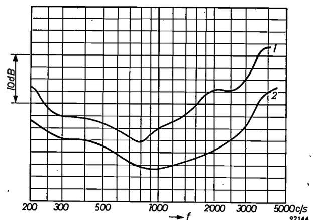
Fig. 10. Case-noise interference as a function of frequency, 1 with microphone opening partly covered, 2 with opening uncovered.
