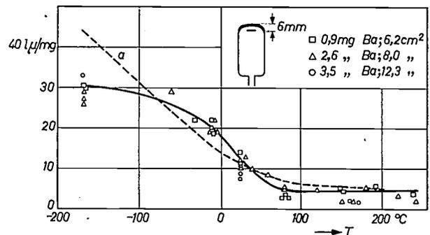
Fig. 14. Absorption capacity per mg of thick barium films as a function of the wall temperature during formation of the film. As in fig. 11, the plotted points refer to films containing 3.5 mg, 2.6 mg and 0.9 mg barium. The full curve is drawn to fit the points for the 0.9 mg films, but also applies fairly well to the others. Curve *a* from fig. 11 (dashed) is included for comparison.
