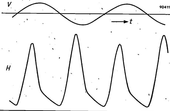
Fig. 2. Sinusoidal alternating voltage  $V$  and the electroluminescent effect (emittance  $H$ ) it produces, as functions of time. A flash is produced every half-period. The frequency of the voltage depicted here was 65 c/s.
