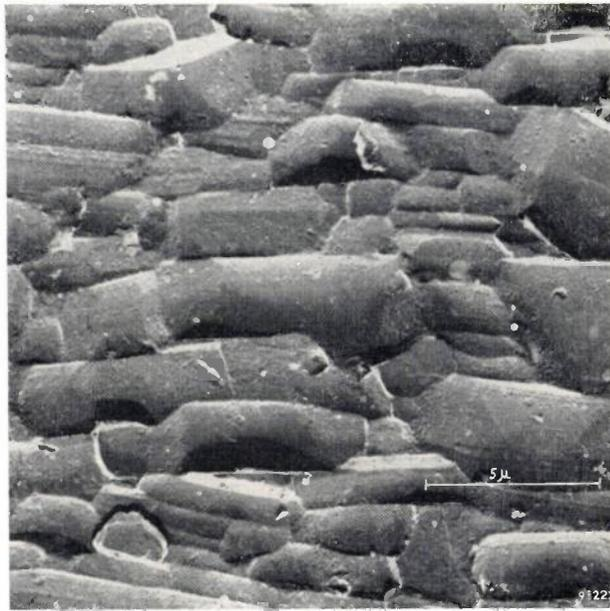
*a* Fig. 6. Electron-microphotographs of aligned ferroplana with foliate texture. In (a) the preferred planes are parallel to the plane of the paper, in (b) they are perpendicular thereto.
