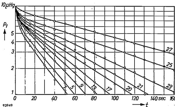
Fig. 7. Gettering rate for hydrogen measured on a single barium film, the logarithm of the pressure p<sub>1</sub> being plotted against the time t which has elapsed since the admission of a given quantity of gas. After a short time the relationship is linear. As more gas is absorbed the gettering rate decreases and the curve becomes less steep. The curves represent the pressure gradient after the first, fifth, ninth, etc. admissions of gas.
