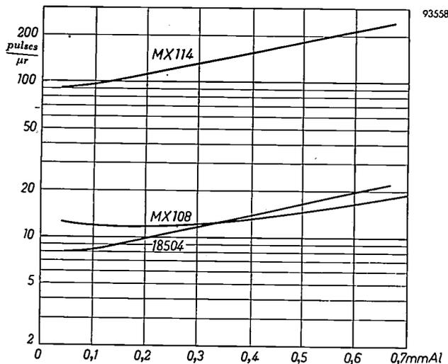
Fig. 4. Calibration curves of three different Geiger-Müller counter tubes, for X-radiation generated at voltages between 10 and 25 kV.
