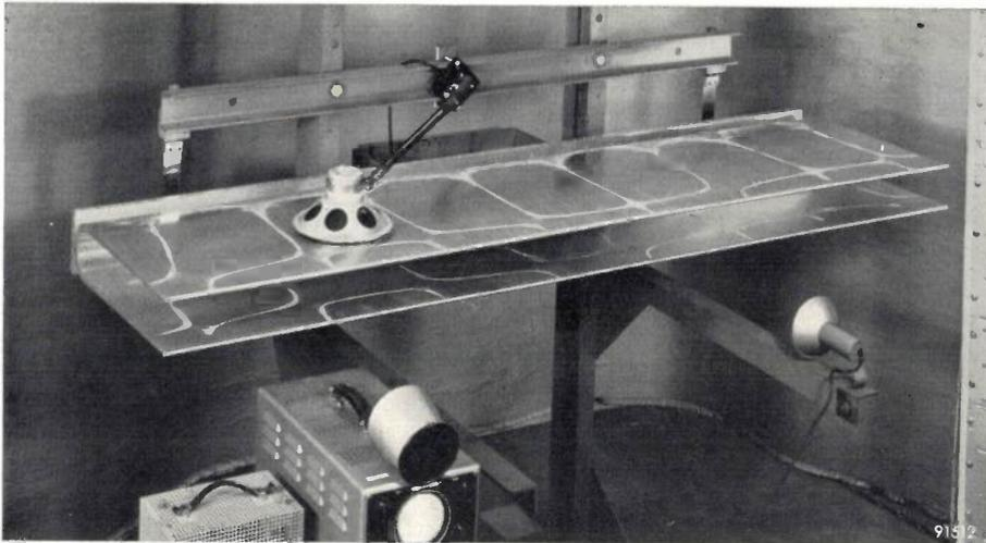
Fig. 2. Vibration pattern at 540 c/s.
