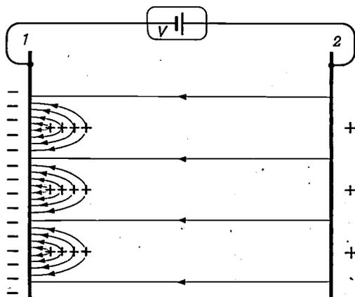
Fig. 5. In a zinc sulphide crystal provided with electrodes 1 and 2 connected to a voltage source  $V$ , a layer of positive space charge of certain thickness is set up on the cathode side of the crystal. The field strength in this layer, as indicated by the lines of force in the diagram, is much greater than the average field strength in the crystal.
