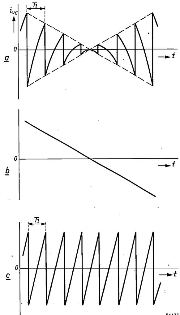
Fig. 8. Trapezium correction. a) Waveform of correction current  $i_{vc}$  that has to be added to the frame scanning current of the right-hand projector (B in *fig. 5a*); the left-hand projector requires correction with a current of the same magnitude but of opposite sense.  $T_l$  is the line period. The function drawn in diagram (a) is the product of the sawtooth (b) of frame frequency, and the sawtooth (c) of line frequency.
