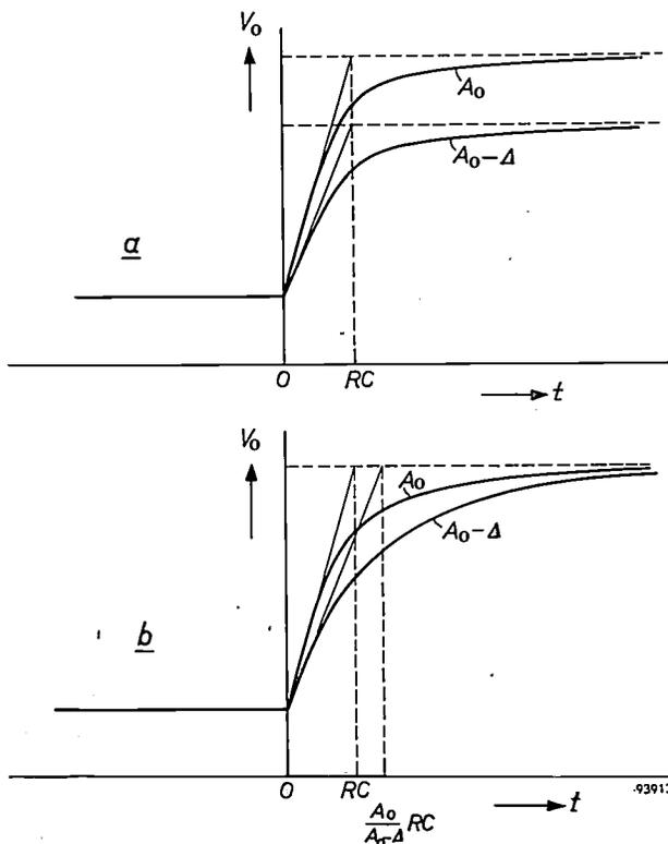
Fig. 7. a) Step-function response of the circuit in fig. 6a, for two values of the amplification,  $A_0$  and  $A_0 - \Delta$ . The end values differ, the time constant in both cases is  $RC$ . b) The same for the circuit in fig. 6b, with  $R'C' = A_0RC$  and  $A \gg 1$ . Now the time constants differ, but the end values are equal.
