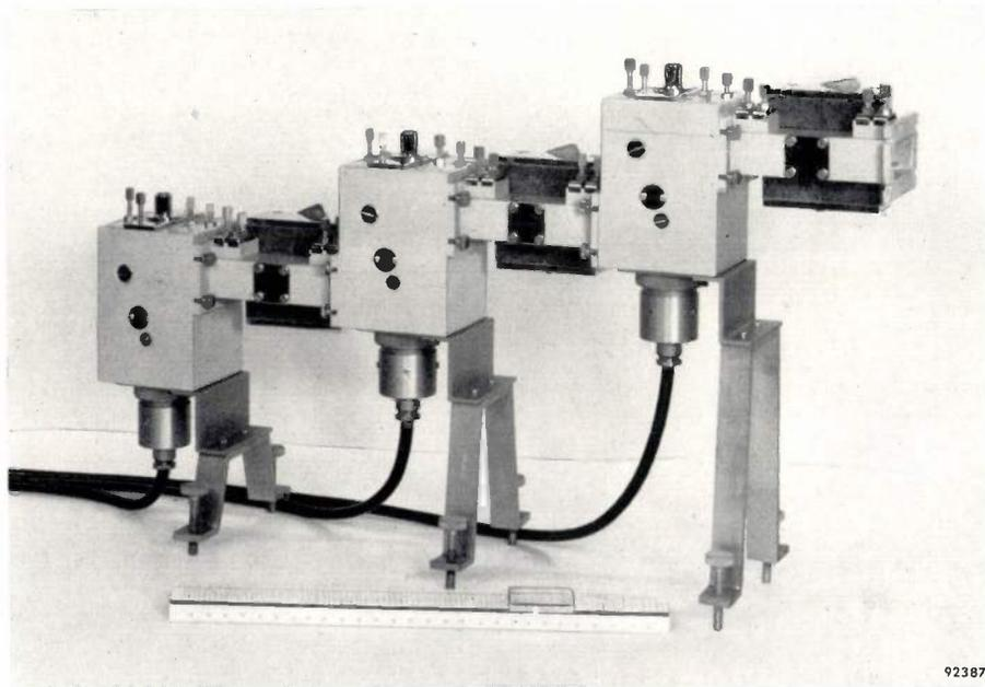
Fig. 16. Amplifier, consisting of three high-frequency stages coupled via ferrite isolators.
