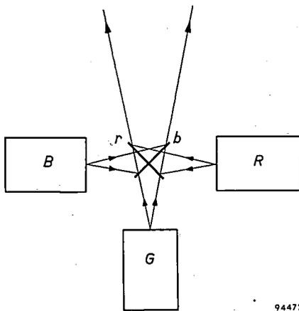
Fig. 2. Superposition of three primary-colour images by means of crossed dichroic mirrors (*r* and *b*). Mirror *r* reflects the red light from *R* and passes the green from projector *G* and the blue from projector *B*. Mirror *b* reflects blue light and passes red and green.
