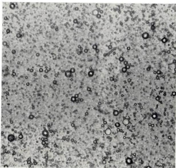
Fig. 1. Photo-micrographs of the acaricide "Tedion V18", formulated as emulsifiable concentrate. Magnification 500 $\times$ . *Above*: Emulsion of the emulsifiable concentrate in water. *Centre*: The emulsion is breaking down. Water droplets are emulsified in the oil droplets (still surrounded by water), which are by now fairly large. *Below*: After the emulsion has broken down and the solvent evaporated, the residue is left in the form of fine crystals.
