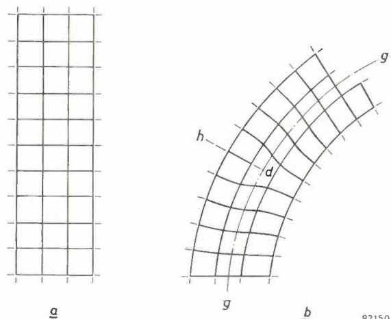
Fig. 8. Schematic diagram of part of a crystal lattice in which shearing has occurred as a result of bending, so that an edge dislocation has formed. *a*) The lattice prior to bending. *b*) The same section of the lattice after bending. Shearing has occurred along the glide plane *g*; this is equivalent to the insertion of an extra half-plane of atoms at *h*. The edge of this plane, i.e. the line at right-angles to the plane of the drawing through the point *d*, is the dislocation axis.
