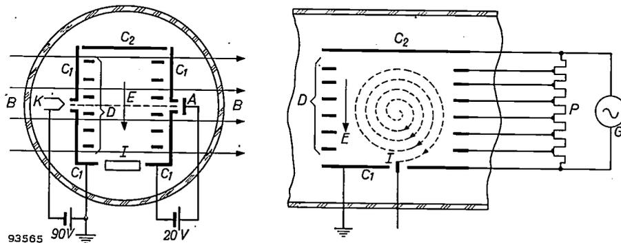
Fig. 1. Schematic diagram of an omegatron. *K* cathode (directly heated tungsten filament). *A* electron collector. *C*<sub>1</sub>, *C*<sub>2</sub> plates to which the radio-frequency voltage from the generator *G* is applied. Flat metal rings *D*, connected to tapplings of the voltage divider *P*, ensure homogeneity of the alternating electric field *E* in the discharge space. *B* constant magnetic induction. *I* ion collector.
