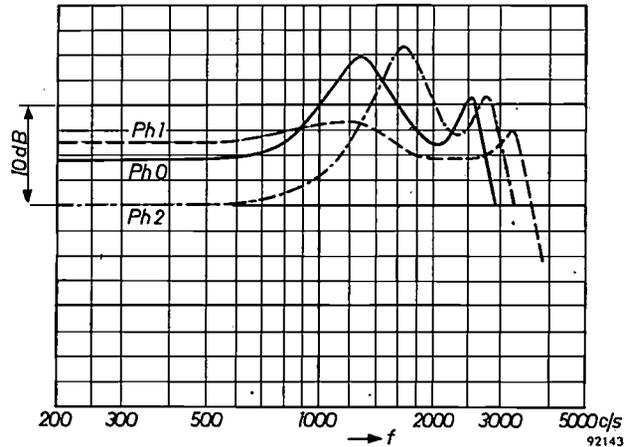
Fig. 8. Frequency characteristics of the three earphones (Ph 0, Ph 1, Ph 2) from which patients may choose. As a function of the frequency  $f$  of the constant current through the earphone, the sound pressure is plotted as measured in an artificial ear of 2 cm<sup>3</sup> volume in which the earphone was fixed.
