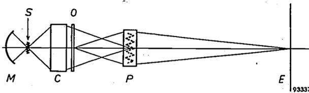
*Fig. 3.* Path of rays in a lantern-slide projector. The image of light-source *S* is formed in the projection lens *P*. The lantern slide *O* is immediately behind the condenser *C* and is thus uniformly illuminated. The auxiliary mirror *M* causes a somewhat larger fraction of the luminous flux emitted by the lamp to be usefully employed, but plays no part in the image formation. The projection lens projects the image of *O* on to the screen *E*.
