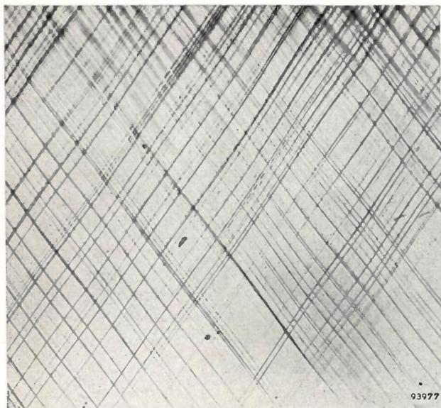
Fig. 4. Slip lines on a (110) plane of a plastically bent germanium crystal ( $75\times$ ). The lines run parallel to (111) planes.
