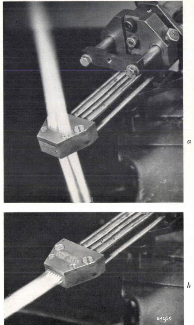
Fig. 5. The burner head, (a) with the jets for head-on heating in operation and (b) with the jets for after-heating in operation.
