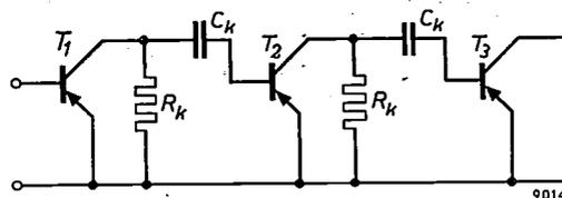
Fig. 12. Three transistors coupled by the resistors  $R_k$  and the capacitors  $C_k$ .
