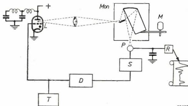
Fig. 2. Set-up for time-resolved spectroscopy using a stroboscopically operated photomultiplier tube. *T* trigger circuit, *L* pulsed light source to be analyzed (in this case a hydrogen thyratron), *Mon* grating monochromator with motor drive *M*, *S* circuit providing the pulse voltages for the photomultiplier tube *P*, *D* variable delay circuit, *R* recording D.C. microammeter.
