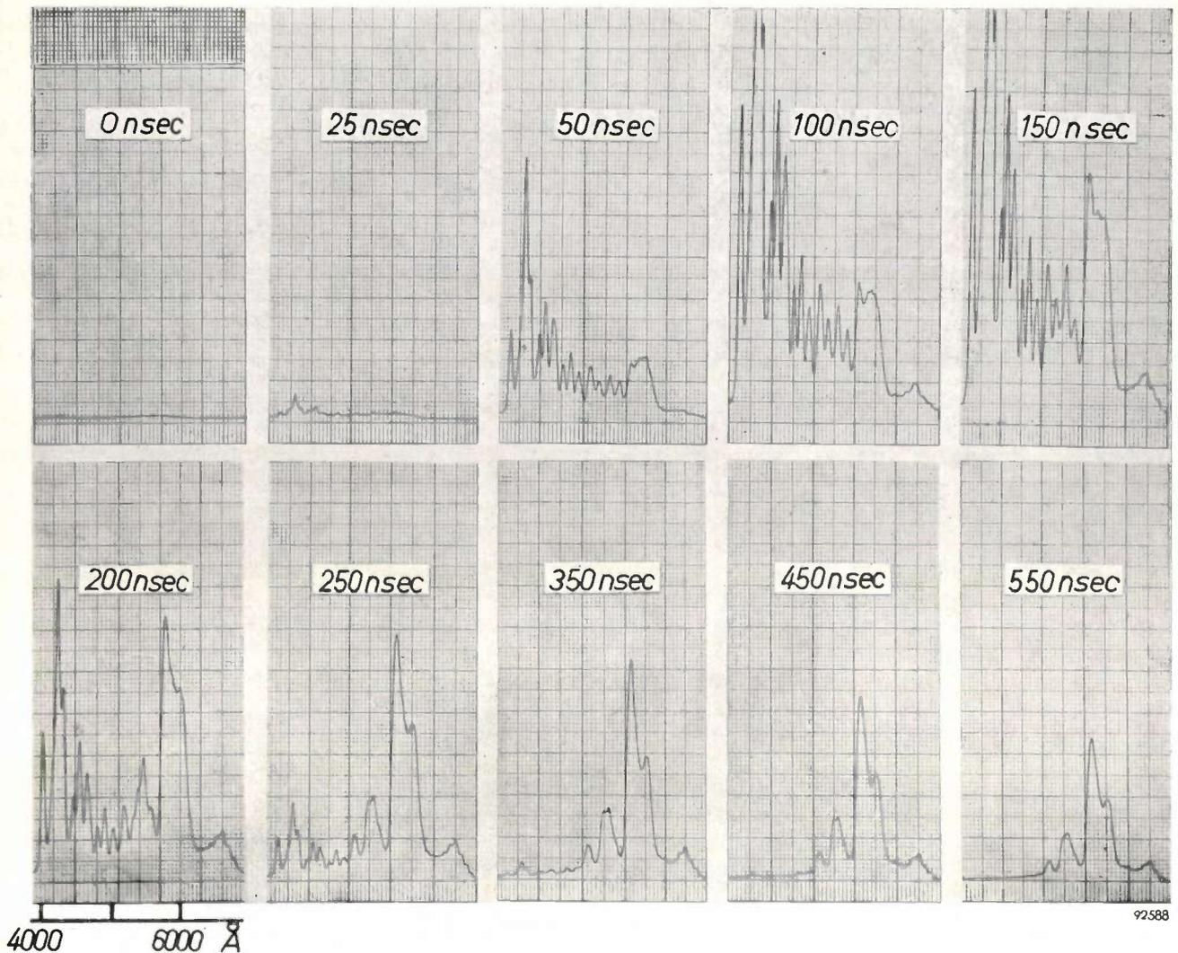
Fig. 6. Time-resolved spectroscopy: a series of spectra obtained from a pulsed nitrogen discharge at successive instants during the pulse, from 0 up to 550 nanoseconds ( $1 \text{ nsec} = 10^{-9} \text{ sec}$ ) after the initiation of the discharge.
