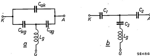
Fig. 15. a) Equivalent circuit for a tube with only its heater voltage applied. A anode, K cathode, G grid,  $L_g$  equivalent inductance of the grid wires. b) Diagram obtained by applying a delta-star transformation to the three capacitors.
