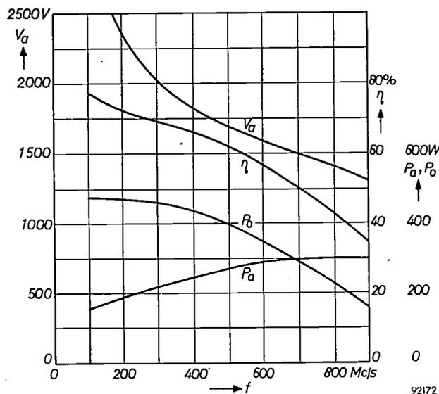
Fig. 14. Maximum permissible H.T. voltage  $V_a$ , maximum permissible dissipation  $P_a$ , power output  $P_o$ , and efficiency  $\eta$  of an oscillating TBL 2/300 tube, as a function of frequency  $f$ .
