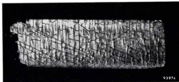
Fig. 2. Surface of a germanium rod quenched from 500 °C in a water bath. The crystal becomes covered with a large number of surface cracks (actual size).
