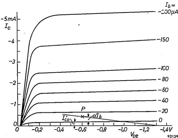
Fig. 4. Collector current  $I_c$  as a function of the voltage  $V_{ce}$  between collector and emitter, with the base current  $I_b$  as the running parameter, plotted for transistor OC 70, as used in the first three amplifier stages. The direct-current operating point is chosen at point P.
