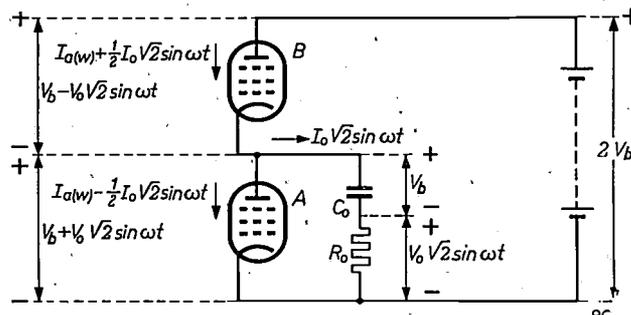
Fig. 4. Circuit of fig. 3 showing currents and voltages. A load resistance *R*<sub>0</sub> represents the loudspeaker.
