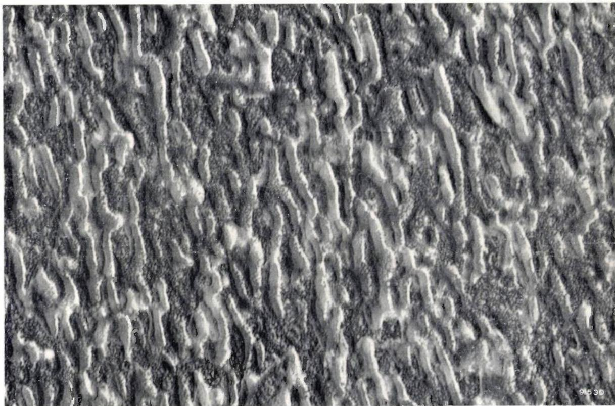
Fig. 2. Electron-microscope photograph of the structure of a (100)-plane *parallel* to the external magnetic field applied during cooling. Direct carbon replica of a platinum-shadowed, electrolytically polished surface, etched with a dilute solution of nitric acid in alcohol. Magnification 160 000 $\times$ . This photograph was made with the Philips electron microscope EM 100 b.
