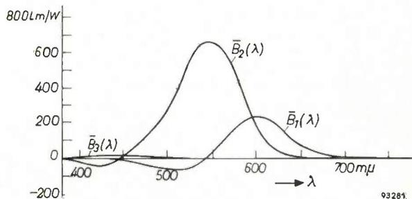
Fig. 4. The quantities  $\bar{B}_1(\lambda), \bar{B}_2(\lambda)$  and  $\bar{B}_3(\lambda)$  from (2) as a function of  $\lambda$ . This figure differs from fig. 3 in that it is based not on the luminous flux but on the energy flux  $E$ . Fig. 4 can be derived from fig. 3 by multiplication by the visual-sensitivity curve.
