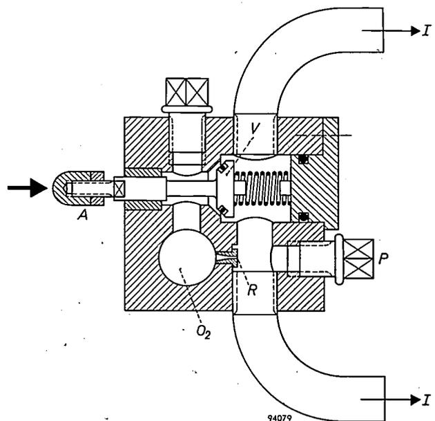
Fig. 7. Regulator for periodically varying the pressure under which the oxygen is fed to the ejector  $I$  of a burner. (This regulator serves two ejectors.)  $O_2$  oxygen feed to regulator;  $V$  valve, which is opened by the action of a cam on the stem (adjustable with nut  $A$ ) against spring pressure;  $R$  constriction, the only route which the oxygen can take when  $V$  is closed, resulting in a reduced pressure in the pipe to the ejector(s).
