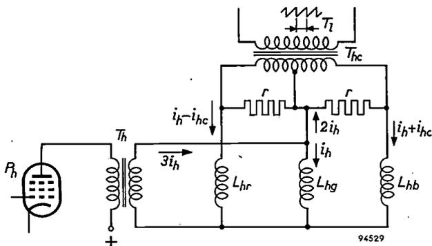
Fig. 16. Circuit for adding correction current  $i_{hc}$  to the line scanning current  $i_h$  in the inductances  $L_{hr}$  and  $L_{hb}$ . Transformer  $T_h$ , supplied from the output tube  $P_h$ , delivers an uncorrected sawtooth current  $3i_h$ . The centre-tapped transformer  $T_{hc}$  supplies resistors  $r$  with a sawtooth voltage, which causes  $i_{hc}$ , a correction current of parabolic shape, to flow through inductances  $L_{hr}$  and  $L_{hb}$ .
