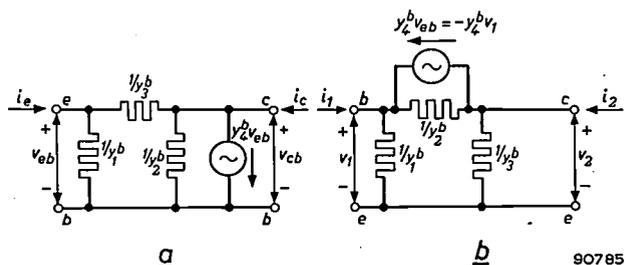
Fig. 3. a) The 'II' network of fig. 2b taken as the equivalent circuit for a transistor, the base terminal b being the common terminal. e: emitter terminal. c: collector terminal. b) The same network with the emitter terminal as the common terminal.
