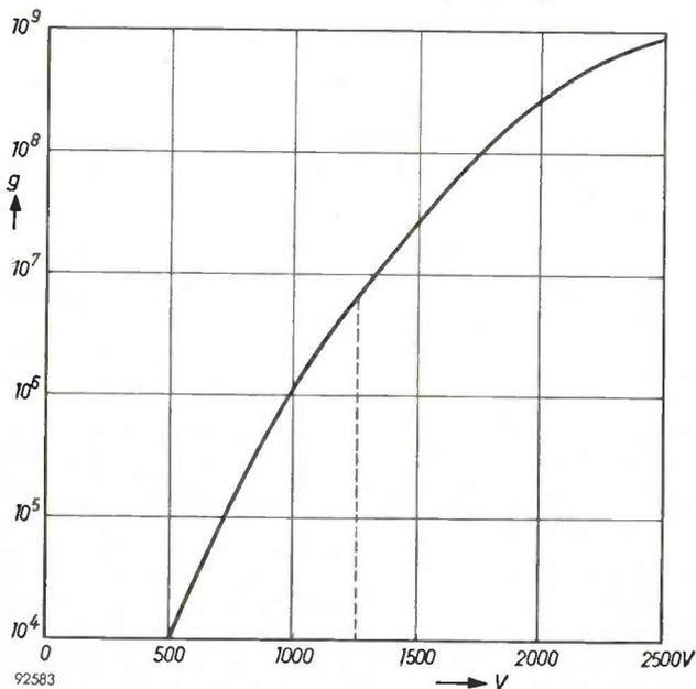
Fig. 7. Gains obtained when actuating a 1P21 photomultiplier tube with a  $10^{-7}$  sec pulse, plotted against the peak voltage applied between cathode and collector.
