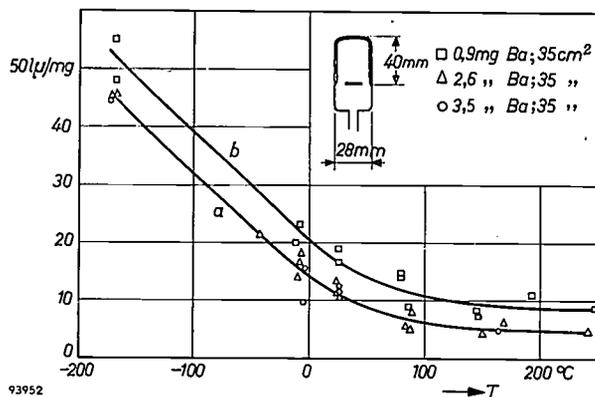
Fig. 11. Measurements of absorption capacity for carbon monoxide. The absorption capacity per mg barium, measured at room temperature, is plotted against the temperature of the bulb during the formation of the barium film. In all cases the getter holder was 40 mm away from the end of the tube. The values found for films containing 3.5 and 2.6 mg barium show no significant difference (curve a). Curve b applies to films containing only 0.9 mg barium.
