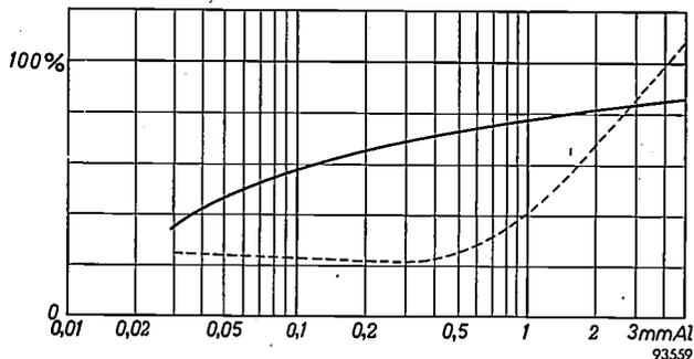
Fig. 5. Sensitivity of an ionization chamber (full curve, approaching 100% for very hard radiation) and of a Geiger-Müller counter type MX 108 (broken curve) as a function of the hardness of the X-radiation.
