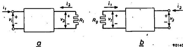
Fig. 9. a) Circuit for calculating the input resistance  $r_i$  of a fourpole having a resistance  $R_l$  as load. b) Circuit for calculating the output resistance  $r_u$  of the same fourpole when the generator has an internal resistance of  $R_g$ .
