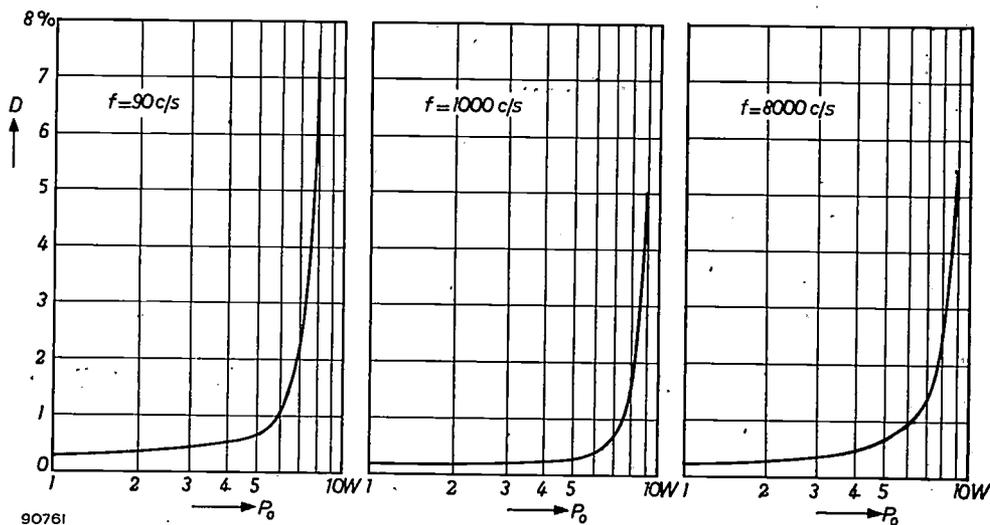
Fig. 9. Distortion  $D$ , measured on an amplifier of the type shown in fig. 8, plotted against the output power  $P_o$ , at the frequencies 90, 1000 and 8000 c/s. Both tone controls set to maximum.
