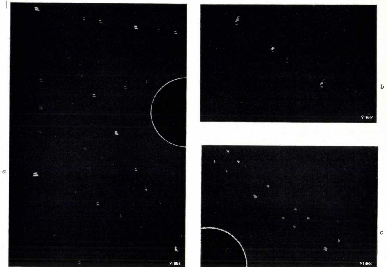
Fig. 7. Laue photographs of recrystallized tungsten wires. A splitting of the spots is observed, this being due to small differences in the orientation of the crystallites: *a*) two-fold splitting (three times actual size); *b*) five-fold splitting (four and a half times actual size); *c*) the spots in this photograph originate from two crystals which are at an angle of  $2^\circ$  and are each separately re-split (three times actual size).
