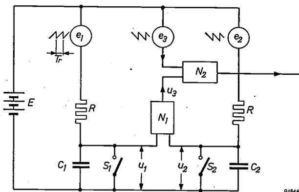
Fig. 14. Schematic diagram of the circuit for generating  $i_{vc}$ , the current for correcting trapezium distortion. Switches  $S_1$  and  $S_2$  (in reality they are valves) are closed only during the flyback of the line sawtooth.  $e_1$ ,  $e_2$  and  $e_3$  are sawtooth voltages having the frame frequency. The subtraction  $u_1 - u_2 = u_3$  takes place in network  $N_1$ , the addition  $u_3 + e_3$  in network  $N_2$ .
