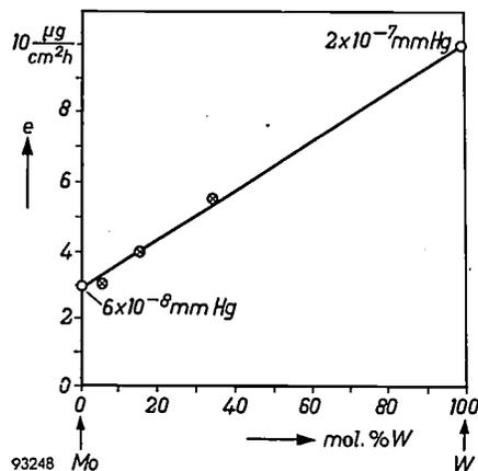
Fig. 2. The evaporation rate  $e$  of barium and barium oxide from pressed cathodes using a tungsten-molybdenum alloy, as a function of the tungsten content of the alloy.
