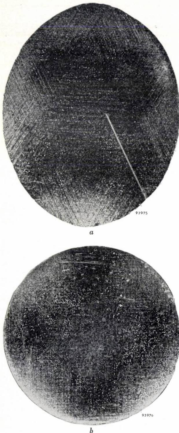
Fig. 3. *a*) Etch-pit pattern produced after etching on an oblique (111) cross-section of a cylindrical crystal with its axis in a [110] direction, which was cooled in a stream of gas. The etch pits lie in rows parallel to the intersections of the surface with the three other (111) planes. Note the minimum in the etch-pit density about midway along the radius of the cross-section. *b*) Etch-pit pattern for a perpendicular (100) cross-section of a [100] crystal, cooled as (*a*).
