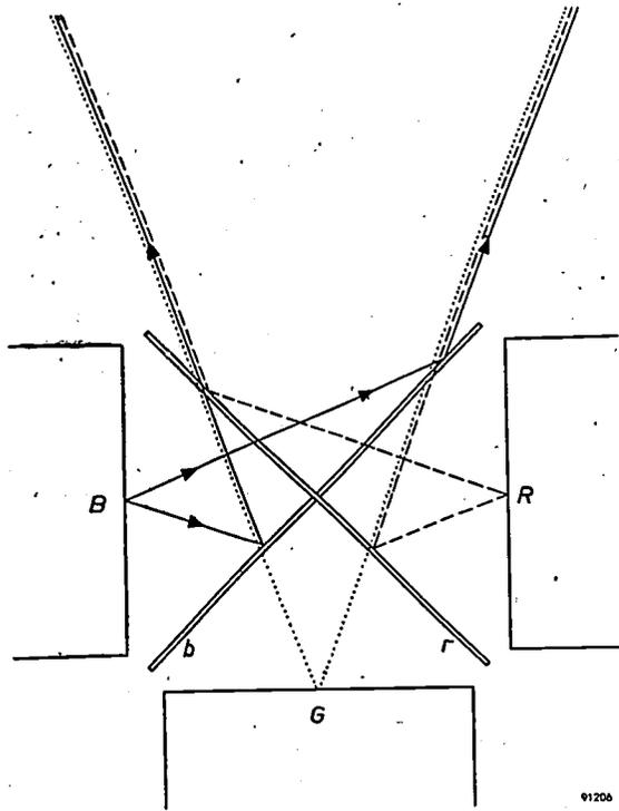
Fig. 12. As fig. 11, but with the arrangement modified so that the red reflecting mirror  $r$  need be no larger than the blue reflecting mirror  $b$ .
