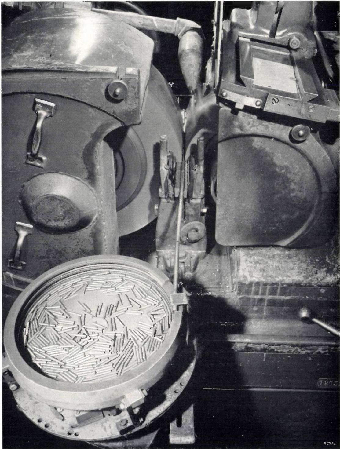
Ceramic sleeves of various types and sizes are used on a large scale in the electronics industry. The photograph shows such sleeves undergoing centreless grinding down to a certain external diameter. A circular vibratory hopper (foreground) feeds the sleeves via a metal tube to the grinding wheel and pressure roller.
