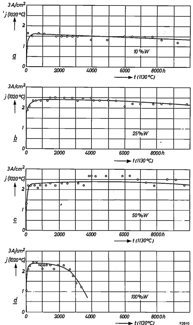
Fig. 5. Current densities  $j$  of various pressed cathodes at an anode potential of 1000 V, as a function of the operation time  $t$ .
