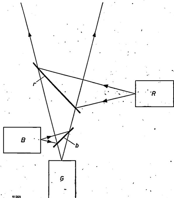
Fig. 11. With the use of semi-reflecting, dichroic mirrors, the beams from the three projectors (*R* red, *G* green, *B* blue) can be made to coincide, with little loss of light. *r* is a red, *b* a blue reflecting mirror.
