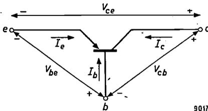
Fig. 1. The three voltages and three currents occurring as variables in transistors.  $e$  is the emitter,  $c$  the collector and  $b$  the base terminal. In accordance with the usual convention, the emitter terminal has an arrowhead to distinguish it from the collector terminal. The direction of the arrow shows whether the transistor is a P-N-P or N-P-N type; in the former case it points towards the base, in the latter case away from it.
