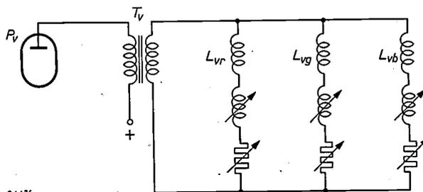
Fig. 11. Adjustment of the amplitude of the frame scanning currents.  $L_{vr}$ ,  $L_{vg}$  and  $L_{vb}$  are the frame scanning coils of the red, green and blue tubes respectively.  $P_v$  is the output tube of the common sawtooth generator. In series with each of the coils are a variable resistor and a variable inductance, the purpose of the latter being to keep the ratio between total resistance and inductance constant.
