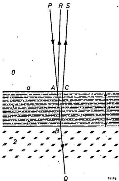
Fig. 1. Reflection, for almost normal incidence, of ray *PA* (in air, medium 0) at a film of water (medium 1) on glass (medium 2). *PABQ* and *BCS* are assumed to be straight lines.
