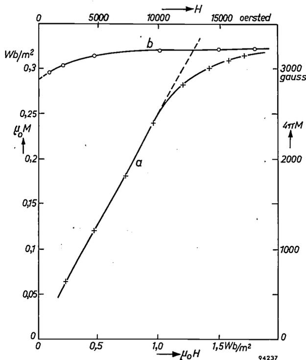
Fig. 2. The magnetization  $M$  of a  $\text{Co}_2\text{Z}$  single crystal as a function of the applied magnetic field  $H$ ; a) preferred plane at right angles to  $H$ ; b) preferred plane parallel to  $H$ .
