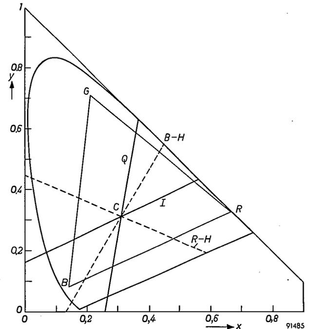
Fig. 15. Variation of signal  $I$  (eq. 19) causes a change of colour along line  $I$  in the colour triangle; variation of signal  $Q$  (eq. 20) causes a change along line  $Q$ . The colour points of the primary colours are  $R$ ,  $G$  and  $B$ . The signals  $S_1$  and  $S_2$  correspond to the lines  $R-H$  and  $B-H$ .
