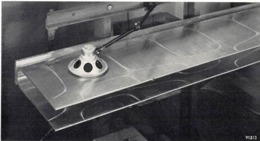
Fig. 3. Vibration pattern at 380 c/s.
