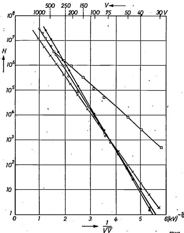
Fig. 4. The logarithm of the emittance  $H$  is a linear function of  $1/\sqrt{V}$ . The above curves were obtained experimentally, with various zinc sulphide powders, the  $H$  scale being in arbitrary units.
