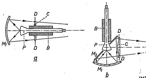
Fig. 1. Schmidt optical systems for the projection of television images; a) "in-line" Schmidt system, b) "folded" Schmidt system.  $P$  projection tube with focussing coil and scanning coils  $B$ .  $M_1$  spherical concave mirror.  $C$  corrector plate mounted in diaphragm  $D$ . The centre of curvature of  $M_1$  lies in the plane of  $D$  in the case of (a) and in the image of  $D$  given by plane mirror  $M_2$  in the case of (b).
