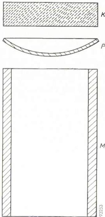
Fig. 2. The construction of a flat impregnated cathode in which the heater filament and the emitting surface are completely separated from each other. The cathode disc *K*, the molybdenum cylinder *M* and the molybdenum separating plate *P* are resistance-welded together in one operation.
