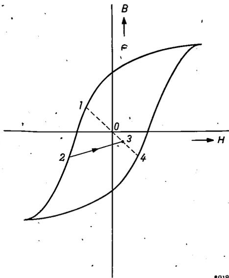
Fig. 6.  $B-H$  curve of a magnet steel. 1-0-4 working line of a magnet made of this steel, pre-magnetizing a pulse transformer. 1 initial working point. During a pulse the flux is reversed and point 2 is reached. At the end of the pulse, point 3 becomes the new working point. The pre-magnetization has thus taken on the wrong polarity.
