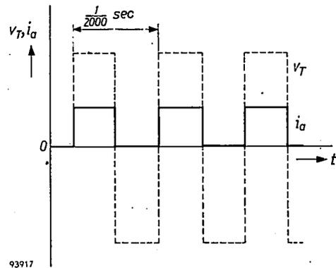
Fig. 12. Supply voltage *v<sub>T</sub>* and anode current *i<sub>a</sub>* of the thyatron in fig. 11, as a function of time *t*.
