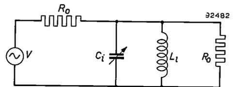
Fig. 8. Equivalent circuit for the iris, placed in a waveguide with matched termination; the waveguide is connected to an energy source which is also matched.
