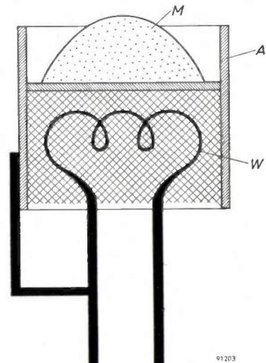
Fig. 9. Section of evaporation element.  $A$  molybdenum cup,  $W$  tungsten heater coil (insulated with aluminium oxide).  $M$  is the substance to be evaporated.
