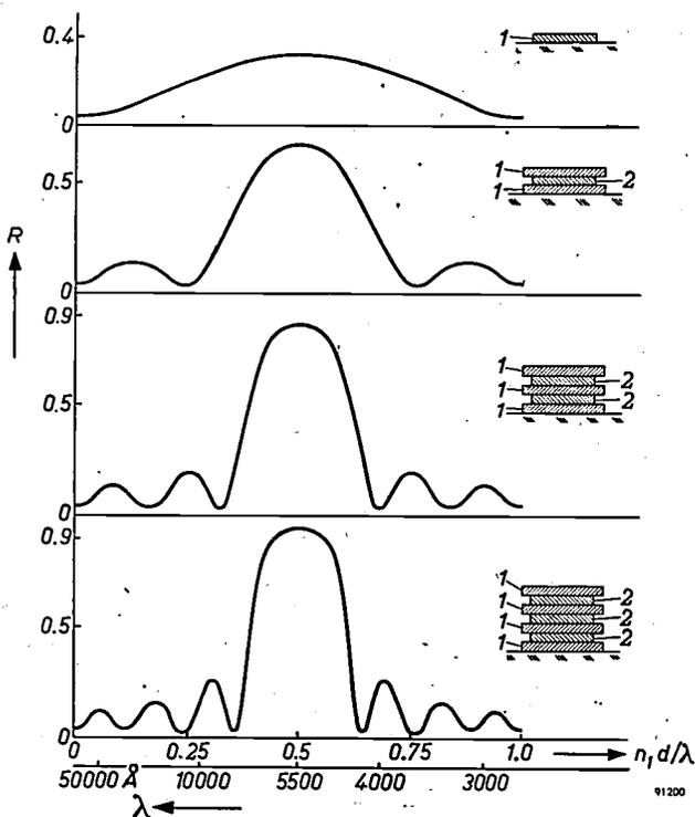
Fig. 5. Reflection coefficient  $R$  (calculated) for a single layer of zinc sulphide and for three-, five- and seven-fold layers on glass. The multiple layers consist of alternate layers of zinc sulphide 1 (thickness  $d$ , refractive index 2.4) and cryolite 2 (refractive index 1.3); the carrier substance is glass (refractive index 1.5).
