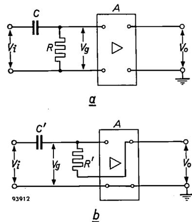
Fig. 6. a) Differentiator ( $C$  and  $R$ ) followed by an amplifier with amplification  $A$ . The output voltage is proportional to  $A$ . b) Differentiator ( $C'$  and  $R'$ ) and amplifier, with  $R'$  connected to the amplifier output. Under certain conditions the output voltage is practically independent of  $A$ .
