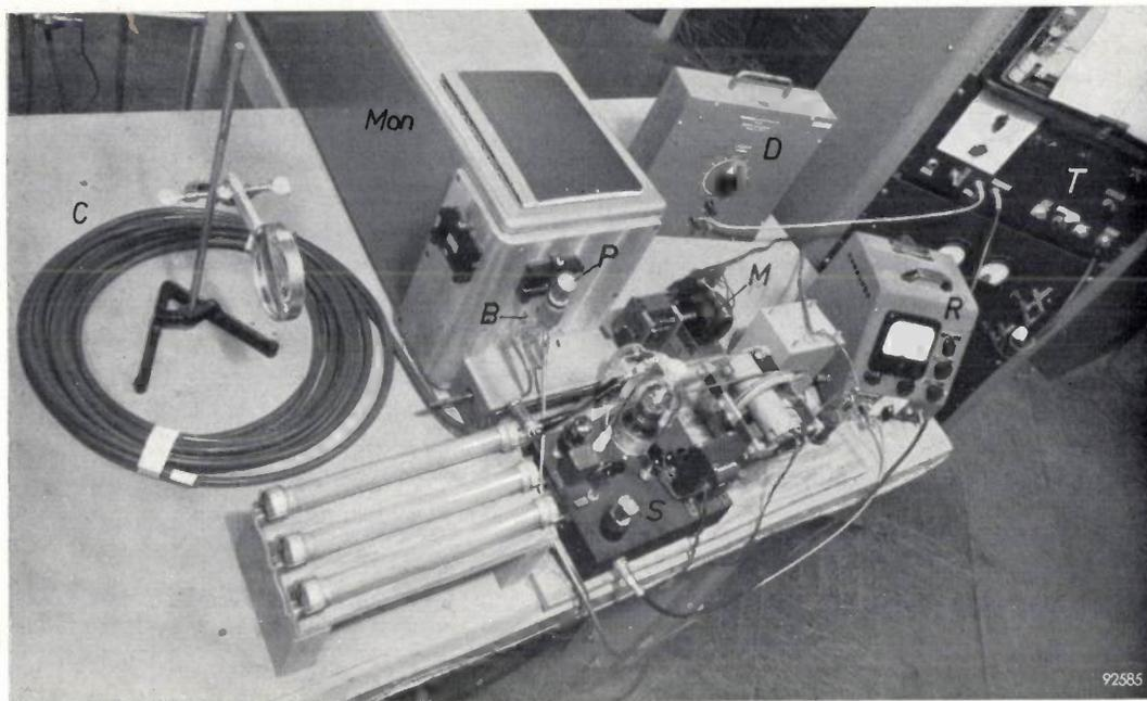
Fig. 3. Photograph of equipment outlined in fig. 2. Same lettering as in fig. 2. The light source is to the left (not visible). To the right, a rack containing the trigger circuit *T* and the recording part of the current meter *R* is seen. *C* is a length of coaxial cable acting as a pulse forming network in the circuit *S*. *B* are the voltage-divider resistors for the photomultiplier-tube dynodes (see fig. 10).
