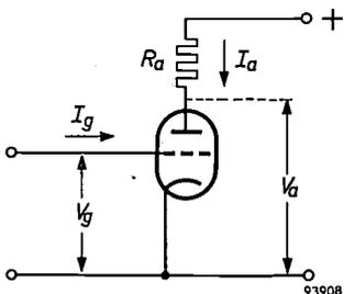
Fig. 2. A logarithmic relation exists between the anode voltage  $V_a$  and the grid current  $I_g$  of a triode operating in the lower region of its characteristic, at constant anode current  $I_a$ . The anode current is here kept approximately constant by the high resistance  $R_a$  in the anode circuit.
