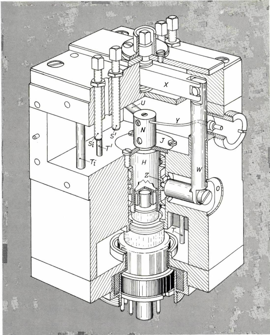
Fig. 13. The complete amplifier block, cut away to show the most important components. *W* denotes the driving rods for plunger *Z*. These rods are fixed at pivots to cross-beam *X*. Underneath they carry pins which engage with the plunger. The other letters have the same meaning as in earlier figures.
