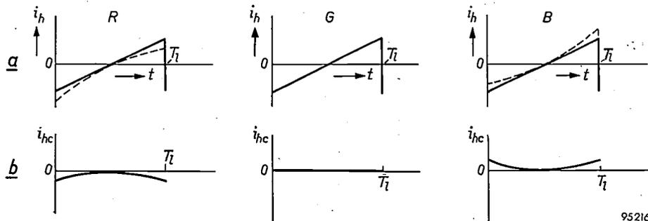
Fig. 6. a) Waveform required (dashed curves) for the line scanning current ( $i_h$ ) in primary-colour tubes R, G and B (mounted as in fig. 5a) in order that linearity be restored to the movement of the three spots across the projection screen.  $T_l$  is the line period. b) To obtain the above waveforms, the linear sawtooth currents in R and B (full lines in a) must have correction currents  $i_{hc}$  added to them; the two correction currents are equal and opposite.
