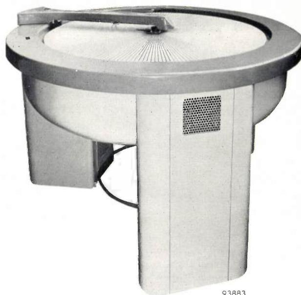
*Fig. 5.* The wind computer. A magslip turns the rotatable 4 ft diameter table so that at every instant it has a position corresponding to the computed wind direction. A recording pen moving at constant speed along the fixed radial arm traces out a graph of wind direction as a function of time (cf. *fig. 7*).
