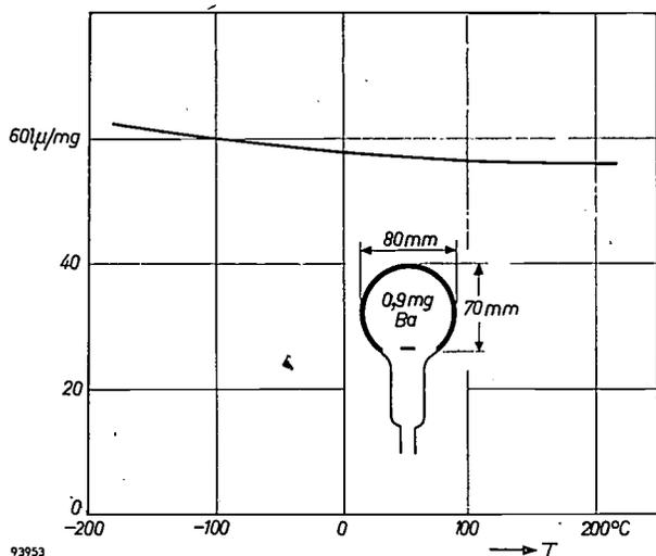
Fig. 12. Absorption capacity per mg of barium films whose grains are not in contact with each other. It can be seen that in this case the temperature of the bulb wall during the formation of the film has only a negligible effect on the absorption capacity.
