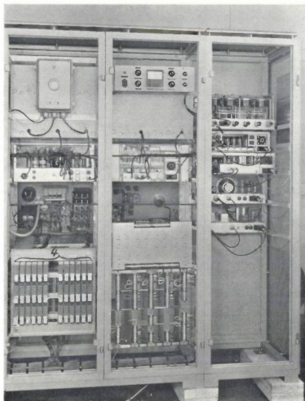
Fig. 4. Rear view of console. 1 three stabilized D.C. power supplies. 2 A.C. voltage stabilizer. 3 and 4 relay banks for servomotors and safety channels (see fig. 5).
