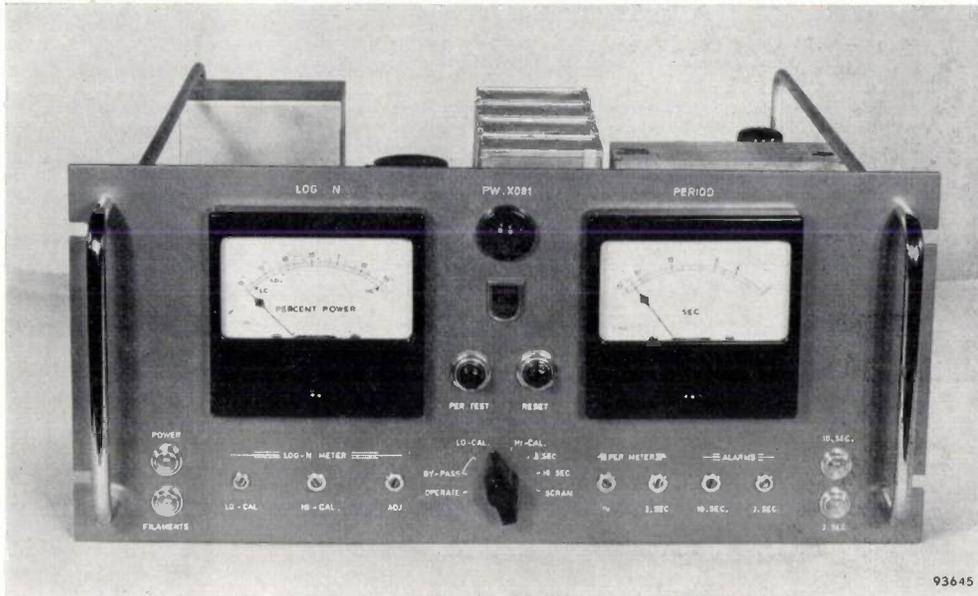
Fig. 1. Unit PW X081 of the logarithmic measuring channel for high neutron flux. Left, the neutron-flux meter with logarithmic scale from  $10^{-4}\%$  to  $300\%$ ; right, the period meter with scale from  $-30$  via  $\infty$  to  $3$  seconds. Below the meters, the correction resistors, adjustable with a screwdriver; between them a switch with eight positions (one operating position and seven calibration and test positions).
