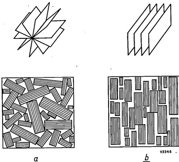
Fig. 3. Anisotropic ferroxplana. Above: basal planes in perspective; below: orientation of crystals in a section perpendicular to the basal planes. a) Fan texture; b) foliate texture.
