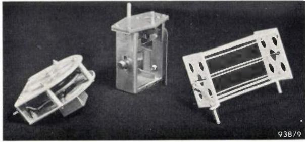
Fig. 2. *Left:* the aneroid barometer; *right:* the fine-wire resistance thermometer; *centre:* the skin hygrometer. The aneroid and hygrometer are conventional elements, but the thermometer is a considerable improvement over earlier types. It is constructed with fine, coiled-coil, tungsten wire, has a very short time constant and a very small radiation error at high altitude.
