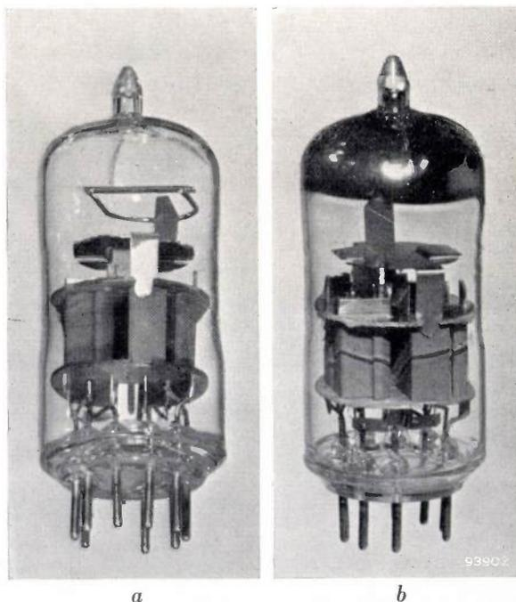
*Fig. 3.* Radio valve containing a getter holder of the type shown in *fig. 1, a)* before, and *b)* after vaporization of the barium.
