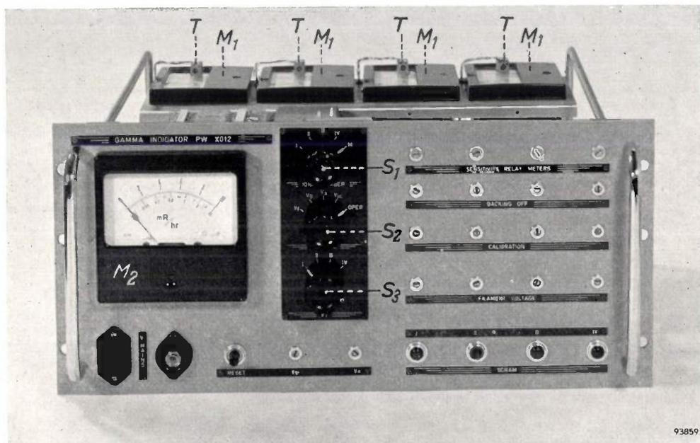
Fig. 9. Gamma-indicator unit PW X012. Above: the four light-relay meters  $M_1$  on which are mounted transistors  $T$ . On the front panel: meter  $M_2$  indicates the dose rate, or functions as a test voltmeter, depending on the position of switches  $S_1$ ,  $S_2$  and  $S_3$ .
