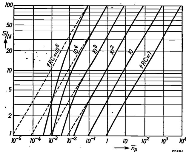
Fig. 11. Signal-to-noise ratio  $S/N$  of the photomultiplier-tube collector current, plotted against the average number  $\bar{n}_p$  of primary photoelectrons per photomultiplier pulse, for different pulse repetition rates  $f$  and integration time constants  $RC$  (see eq. 2). The dashed curves would be obtained if no thermal electrons were emitted by the photocathode.
