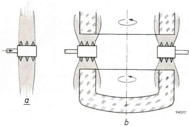
Fig. 2. By the method developed at Philips, thick-walled glass parts are sealed by means of burners (a) whose gas jets are directed head-on to the edges to be joined (b).
