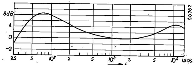
Fig. 10. Output voltage with constant input voltage versus frequency  $f$ , measured on an amplifier of the type shown in fig. 8, loaded with 800 ohms. Both tone controls set to maximum (i.e. minimum negative feedback). Boosting of the low and high notes as shown is desirable in the audio amplifier of a radio receiver.
