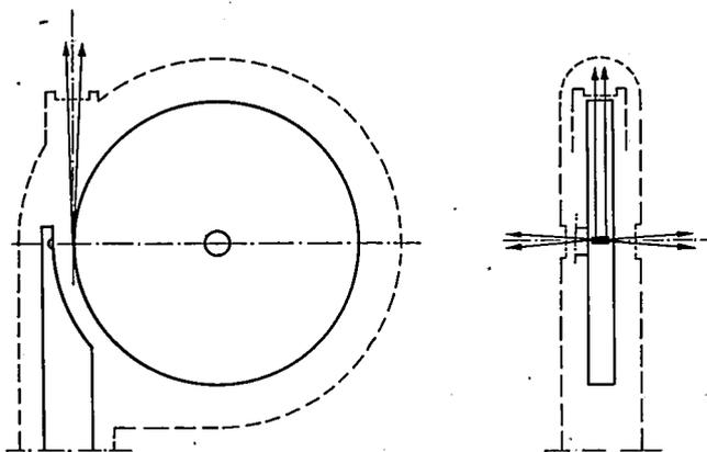
Fig. 2. Schematic diagram of the cathode, the anode disc and the housing with its three beryllium windows. The dimensions of the focus are approximately  $1 \text{ mm} \times 10 \text{ mm}$ . Looking through the horizontal windows, a point focus is seen of effective dimensions about  $1 \text{ mm} \times 1 \text{ mm}$ ; looking in the vertical direction, a line focus about  $0.1 \text{ mm} \times 10 \text{ mm}$  is seen.
