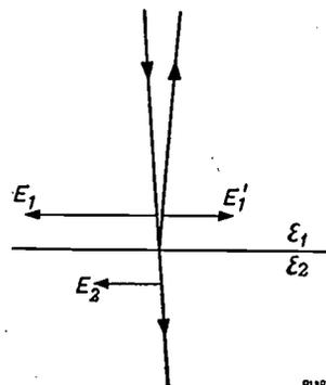
Fig. 3. The almost normally incident ray and the reflected and the refracted rays at the boundary of two media of dielectric constants  $\epsilon_1$  and  $\epsilon_2$ . The tangential components of the electric field are  $E_1$ ,  $E_1'$  and  $E_2$  respectively. The tangential components of the magnetic field are perpendicular to the plane of the drawing and all point in the same direction.
