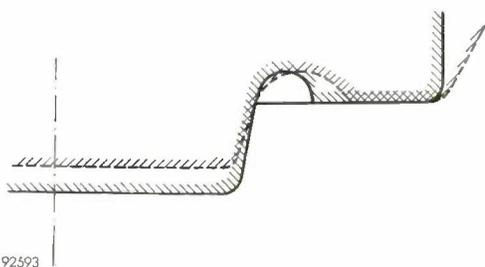
Fig. 4. Old profile (dashed) and new profile (full line) of cleating tool.
