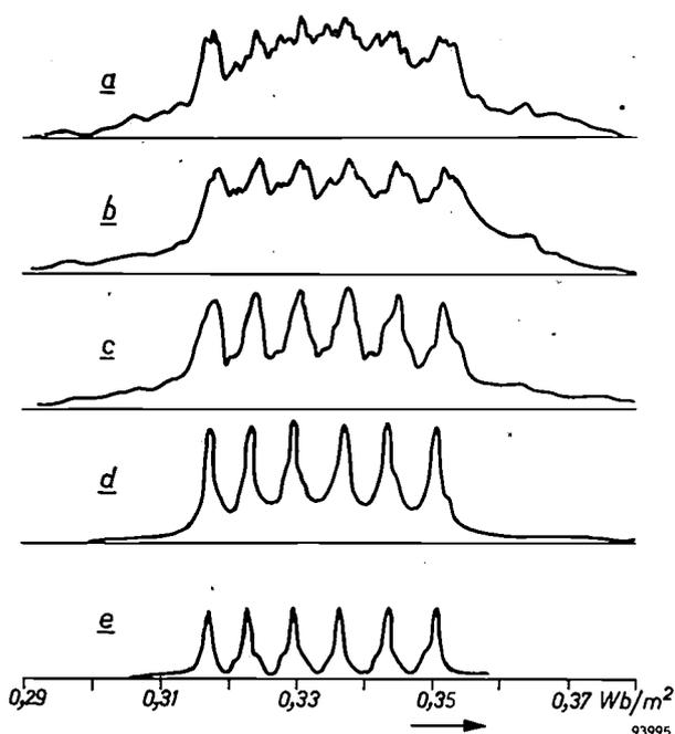
Fig. 9. Example of how the symmetry of the crystal lattice affects the resonance spectrum. In a) and e) are shown the resonance spectra of  $Mn^{2+}$  (0.05%) in wurtzite (hexagonal ZnS) and in sphalerite (cubic ZnS), respectively. The other spectra show how, under an applied pressure, the crystal structure changes from hexagonal to cubic. The relevant pressures were: b) 750 kg/cm<sup>2</sup>, c) 1500 kg/cm<sup>2</sup>, d) 3500 kg/cm<sup>2</sup>.
