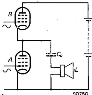
Fig. 3. Single-ended push-pull circuit with two pentodes A, B (EL 86) requiring no central tapping of the H.T. supply. A large capacitor *C*<sub>0</sub> is placed in series with the speech coil of loudspeaker *L*.
