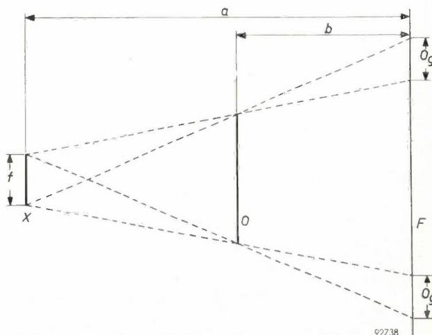
Fig. 3. The geometric unsharpness  $O_g$  of a microradiograph is determined by the dimensions of the focus ( $X$ ) and the distances from film ( $F$ ) to focus and from film to object ( $O$ ). If the latter distance is very small (contact method),  $O_g$  is also very small.
