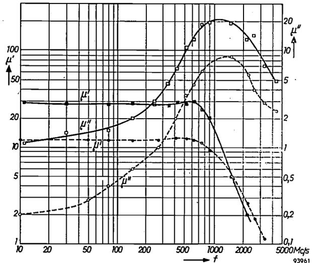
Fig. 12. The quantities  $\mu'$  and  $\mu''$  as a function of frequency  $f$ ; full curve for aligned  $\text{Co}_2\text{Z}$ , broken curve for unaligned  $\text{Co}_2\text{Z}$ .
