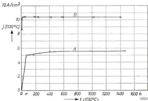
Fig. 6. Current densities of pressed cathodes at an anode voltage of 1000 V, as a function of the life. Temperature was the same during operation and measurement, namely 1130 °C. A barium aluminate; B barium-calcium aluminate.
