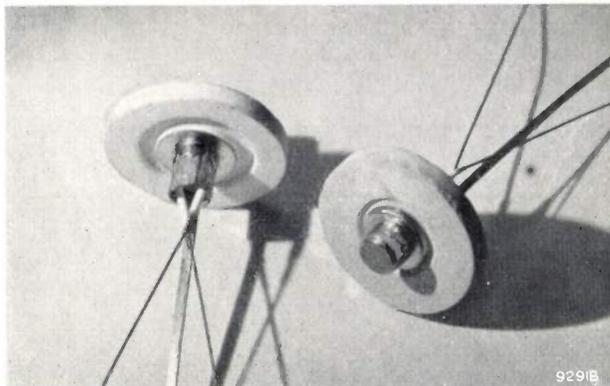
Fig. 3. Pressed cathodes with flat emitting surface (diameter 3 mm) contained in cylindrical molybdenum holders.
