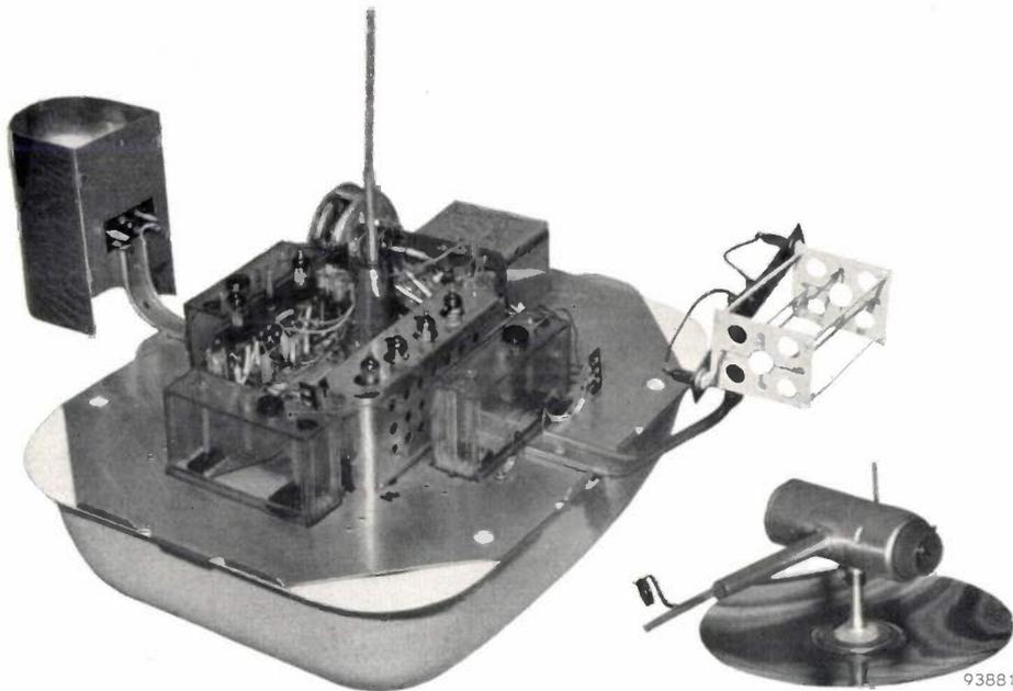
Fig. 1. Airborne unit of the radar sonde (cover removed). The humidity and temperature measuring elements are carried on external arms; the main part of the unit is enclosed in a thermally insulating case. The aerial, receiver, telemetering circuit, switch, barometer and batteries are seen mounted on the chassis plate. The 10 cm wave transmitter and aerial assembly, which are mounted underneath the chassis plate, are shown separately on the right-hand side of the photograph.
