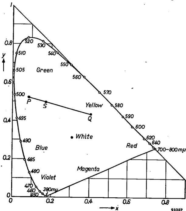
Fig. 6. The colour triangle<sup>5</sup>). The wavelengths of the spectral colours are given around the circumference.
