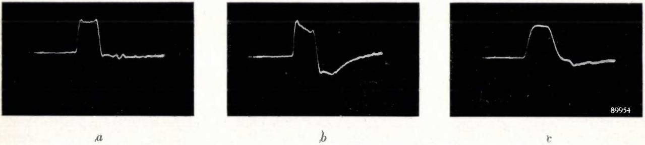
Fig. 4. Oscillograms of the secondary voltage of a pulse transformer whose primary voltage consists of a series of nearly rectangular pulses (duration 1  $\mu$ sec) and whose secondary winding is resistance-loaded.
