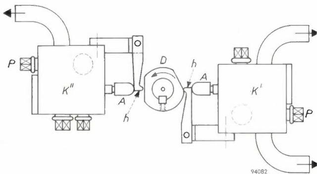
Fig. 8. The block containing eight adjacent regulators *K'* for head-on heating, and a similar block with regulators *K''* for after-heating, are both driven by a single camshaft with eight cams *D*. The end *A* of each valve stem is not directly in contact with its associated cam, but rests against a separate rocker arm *h*, so that the valve stem is subjected only to an axial load.
