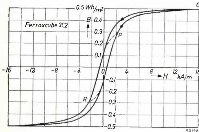
Fig. 5.  $B$ - $H$  curve of ferroxcube 3C2. The curve  $OP$  corresponds to a large  $\mu_r$  ( $= 300$ ), but  $\Delta B$  is only  $0.3 \text{ Wb/m}^2$ . If the curve  $OQ$  is chosen, then  $\Delta B = 0.5 \text{ Wb/m}^2$ , but  $\mu_r$  is reduced to 25. The condition with a pre-magnetization corresponding to  $-0.3 \text{ Wb/m}^2$  (point  $R$ ) is a great deal more favourable: for the curve  $RP$ ,  $\Delta B = 0.6 \text{ Wb/m}^2$  and  $\mu_r = 300$ .
