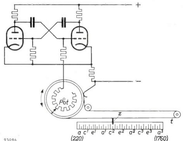
Fig. 5. Circuit diagram of a multivibrator with continuously variable pitch. The pitch is controlled by a potentiometer *Pot* whose sliding arm is fixed to a wheel; a cord and pulley system enables the musician to turn the wheel by moving a clip *z* along a scale calibrated in notes from *a* to *a*<sup>3</sup>. By moving *z* rapidly to and fro a natural vibrato can be produced.
