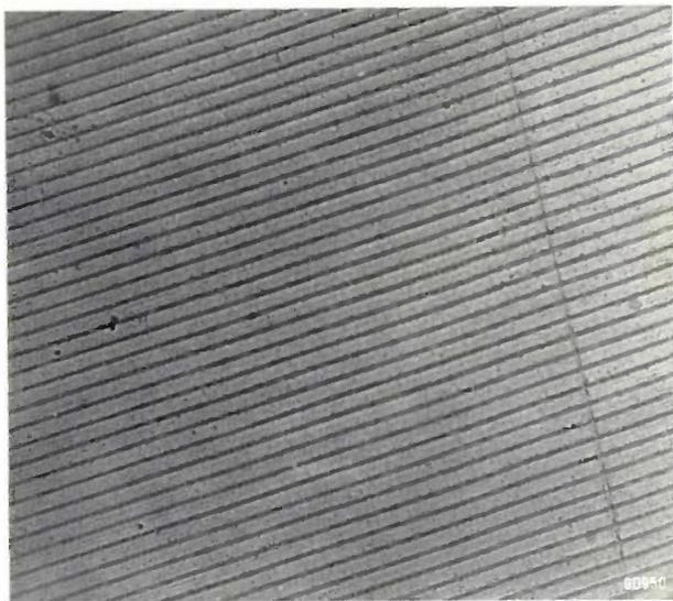
*Fig. 2.* Photomicrograph ( $\sim 250\times$ ) of the surface of a disc of plastic material machined flat with a diamond tool on a precision lathe provided with the headstock described here. From the uniformity of the groove width it can be deduced that movement in the axial direction during working was less than 1/200 micron.
