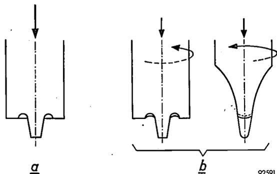
Fig. 2. a) Tool for direct pressure method (solid of revolution). b) Tool for spinning method (front and side views).
