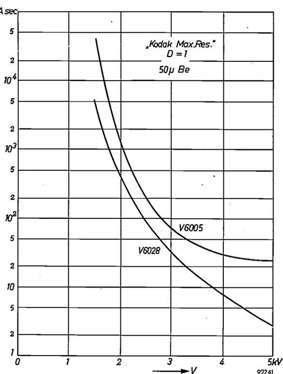
Fig. 9. The exposure, expressed in mA.sec, needed to produce a photographic density 1, as a function of anode voltage. The upper curve relates to standard Kodak "Maximum Resolution" film (emulsion V 6005) and the lower to an experimental Kodak emulsion V 6028. The curves show that the latter emulsion is at least 2 × as sensitive as the other, and at 5 kV even 10 × as sensitive.
