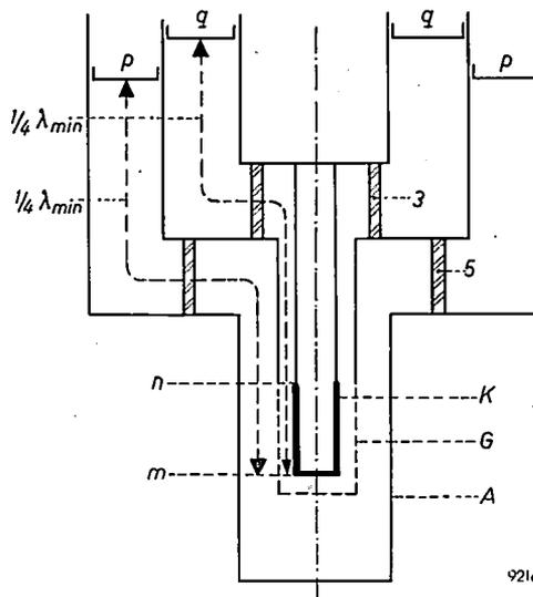
*Fig. 6.* Schematic cross-section of TBL 2/300 and coaxial resonant system. *K* cathode. *G* grid. *A* anode. 3, 5 glass rings. *p-p* annular shorting-piston for anode circuit. *q-q* annular shorting-piston for grid circuit. The triode proper lies between *m* and *n*. The distances *mp* and *mq* are  $\lambda/4$ .
