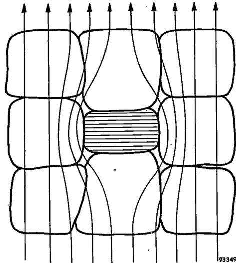
Fig. 4. Demagnetization due to a wrongly oriented crystal in ferroxplana. The preferred planes of the surrounding crystals lie in the plane of the drawing; that of the central crystal is perpendicular to the plane of the drawing and parallel to the hatching. The lines of force must bend round the "crosswise" crystal.
