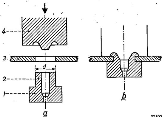
Fig. 1. a) 1 cleat, 2 "rim" of cleat, 3 plate with which joint is to be made, and 4 cleating tool for effecting the joint. b) Completed joint.
