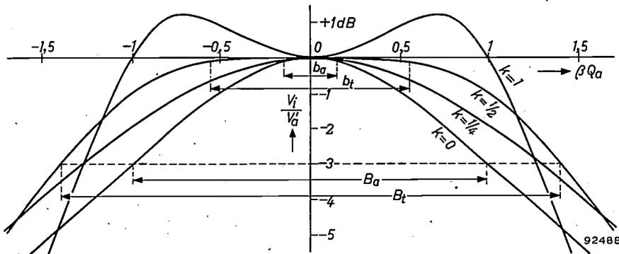
Fig. 7. The voltage ratio  $V_i/V_a'$  from fig. 6b, plotted in dB as a function of the product  $\beta Q_a$ . The curves hold for three different values of  $k$ . At  $k = \frac{1}{2}$ , transitional coupling is obtained.
