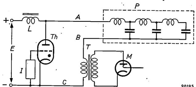
Fig. 1. Circuit for supplying the anode-voltage pulses for a radar transmitter. *E* direct-voltage source. *L* choke coil. *Th* thyatron. *I* ignition device for the thyatron. *P* pulse-shaping network (delay line). *T* pulse transformer. *M* magnetron.
