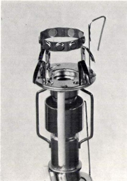
Fig. 4. Part of the electrode system of a television picture tube on which a ring-type holder (fig. 2) is mounted. To avoid any disturbing effect on the electron beam, the getter holder in television picture tubes is made of non-magnetic material.
