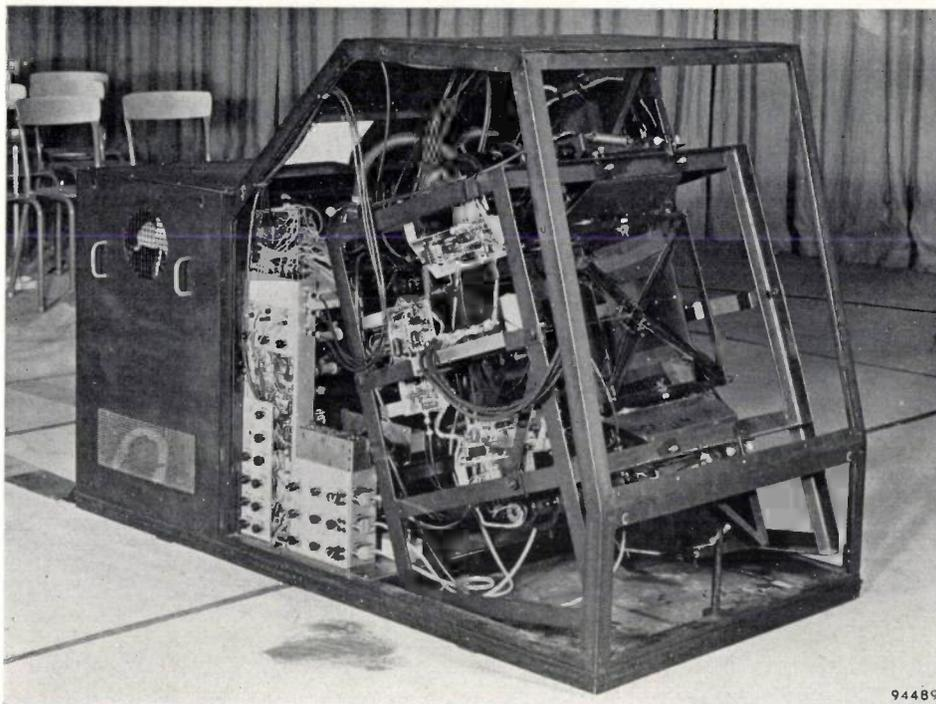
Fig. 4. Photograph of the colour-television projector sketched in fig. 3. The size of the projected picture is  $2.25 \text{ m} \times 3 \text{ m}$  ( $\approx 7\frac{1}{2}' \times 10'$ ) and its maximum luminance is about  $10 \text{ cd/m}^2$ . Electrical adjustments are carried out from a control desk (not shown in the photograph).
