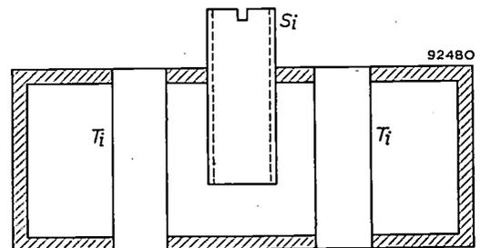
Fig. 5. The output waveguide contains a resonant iris, which consists of a screw  $S_i$  and two rods  $T_i$ .
