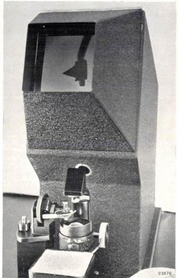
Fig. 7. Projection microscope (magnification  $50\times$ ) for the individual inspection of mounted sapphire and diamond styli. The three lines on the screen serve for the checking of dimensions and alignment.
