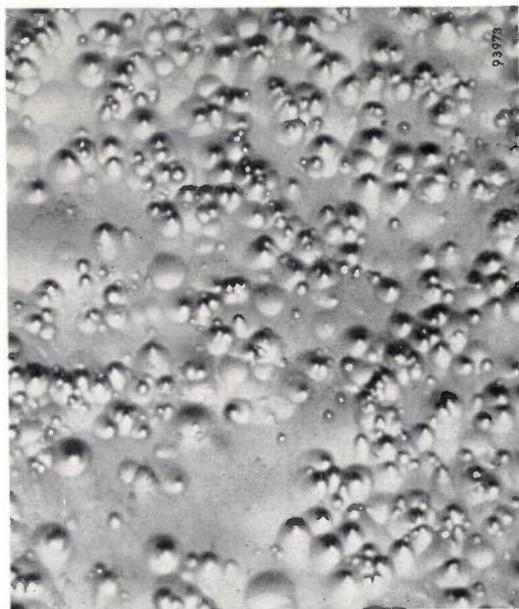
Fig. 1. Etch pits on the surface of a slightly deformed germanium crystal. The pits indicate the places where dislocation lines terminate at the surface (magnification 75 $\times$ ).
