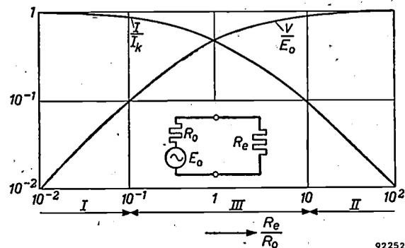
Fig. 8. Current and terminal voltage of a generator (e.m.f.  $E_0$ , internal resistance  $R_0$ ) connected to an external resistance  $R_e$ , as functions of the ratio  $R_e/R_0$ . The scales of both axes are logarithmic. In region I the current approaches the short-circuit value  $I_k$ . In region II the terminal voltage approaches  $E_0$ , the e.m.f. of the generator. In region III matters are more complicated.
