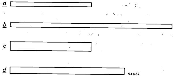
Fig. 2. Given a tubular fluorescent lamp of a certain power, a lamp with double the power may be realized in various ways: a) Original lamp. b) Lamp with the same diameter and double the length; the arc voltage is doubled. c) Lamp having the same length as (a) but with double the diameter; the arc voltage becomes very low. d) Lamp having the same arc voltage as (a); both length and diameter have been increased; the proportions of the lamp are similar to (a).
