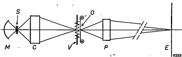
*Fig. 4.* Path of rays in a film projector. The image of the light-source *S* is formed near the film gate *V* by the condenser *C*. The auxiliary mirror *M* has the same function as in *fig. 3*. *P* projects the image of film *O* on to *E*.
