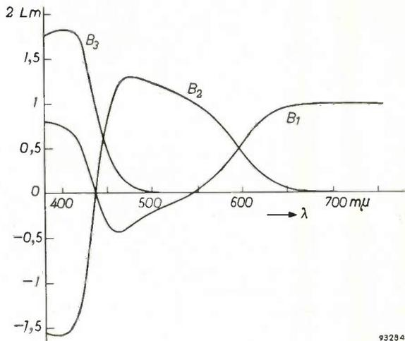
Fig. 3. The colour coordinates  $B_1, B_2$  and  $B_3$  of 1 lumen of the spectral colours with wavelength  $\lambda$ , in the system of primary colours given by (1). ( $1 \text{ m}\mu = 10^{-9} \text{ m}$ .)
