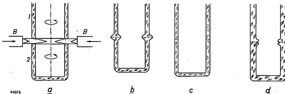
Fig. 1. *a*) For sealing two thin-walled sections 1 and 2 the sections are heated, while rotating, by burners *B*, the jets being directed radially on the glass parts to be joined. *b*) Joint obtained by pressing the hot ends together. *c*) Joint after stretching. *d*) The sealing of two thick-walled sections by the same method does not produce a good joint (notch on the inside).
