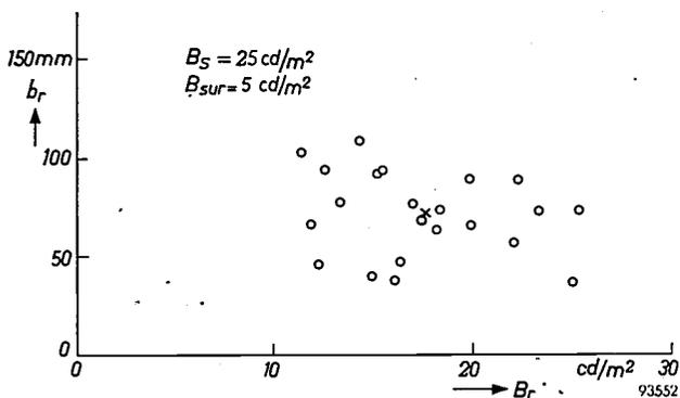
Fig. 3. Example of a cluster of points consisting of all points  $Q$  derived in the manner shown in fig. 2 (each observer supplying one point). This scatter diagram, which clearly illustrates individual differences, is, like fig. 2, only valid for a given set of luminance values of screen and surroundings. The cross shows the average preferred combination.
