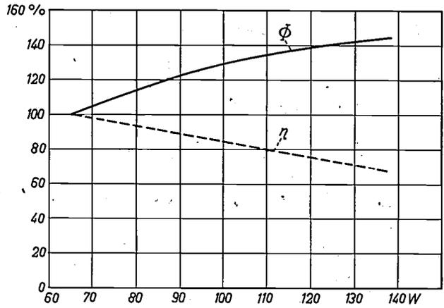
Fig. 3. Variation of the luminous flux and the luminous efficiency (both plotted as percentages of the rated values) of a given "TL" 65 W lamp for various values of the power developed in it. The lamp was not of course operated with its ordinary ballast: it was fed from a special supply. (The lamp differed from the ordinary "TL" 65 W lamps only in having somewhat heavier electrodes, fitted for the purpose of this experiment to withstand the larger current.)
