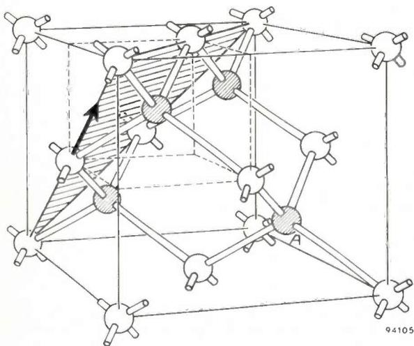
Fig. 5. Unit cell of the diamond structure, the crystalline structure of germanium. The hatching indicates one of the four (111) planes, and the arrow one of the six  $[110]$  directions.
