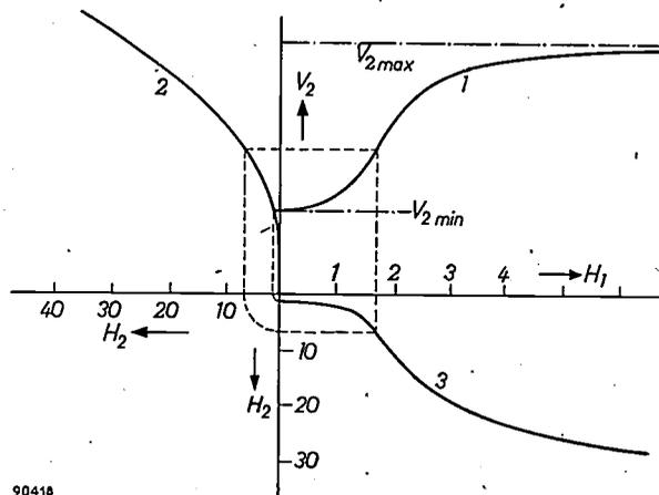
Fig. 9. Amplificon characteristic (3) constructed by combining the  $V_2$ - $H_1$  characteristic (1) and the  $H_2$ - $V_2$  or electroluminescence characteristic (2).  $V_{2max}$  = maximum voltage acting across layer *II* when the radiation falling on layer *I* is very intense (when  $H_1 \rightarrow \infty$ ).  $V_{2min}$  = minimum voltage acting across layer *II* in the absence of incident radiation (when  $H_1 = 0$ ).
