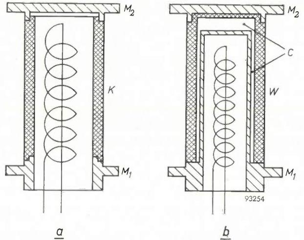
Fig. 4. *a*) Fixing a cylindrical impregnated cathode (*K*) into a molybdenum holder (*M*<sub>1</sub>, *M*<sub>2</sub>). *b*) The corresponding construction of the cylindrical L cathode, shown for comparison. The chamber *C* is charged with the barium compound.
