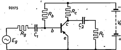
Fig. 7. A circuit with a transistor in the common-emitter configuration and with provision for the biasing.  $E_g$  is the e.m.f. and  $R_g$  the internal resistance of the signal source,  $R_L$  is the load,  $C_1$  and  $C_2$  are blocking capacitors, and  $R_b$  and  $R_c$  are resistors for setting the biasing.  $V_0$ : battery voltage.
