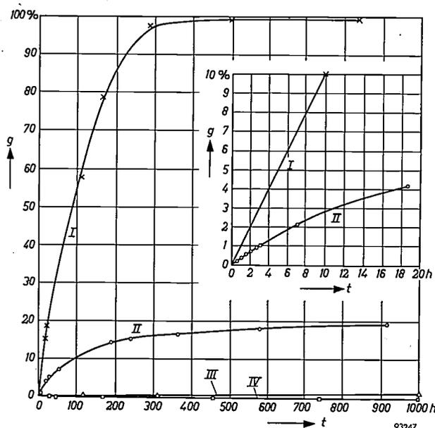
Fig. 1. The stability in air of the pressed cathode and of various emitting materials that may be used in this cathode. The percentage increase in weight *g* by uptake of water is plotted as a function of the time *t*. *I* powdered BaO, *II* powdered Ba-aluminate, *III* fused pellet of Ba-aluminate, *IV* pressed cathode.
