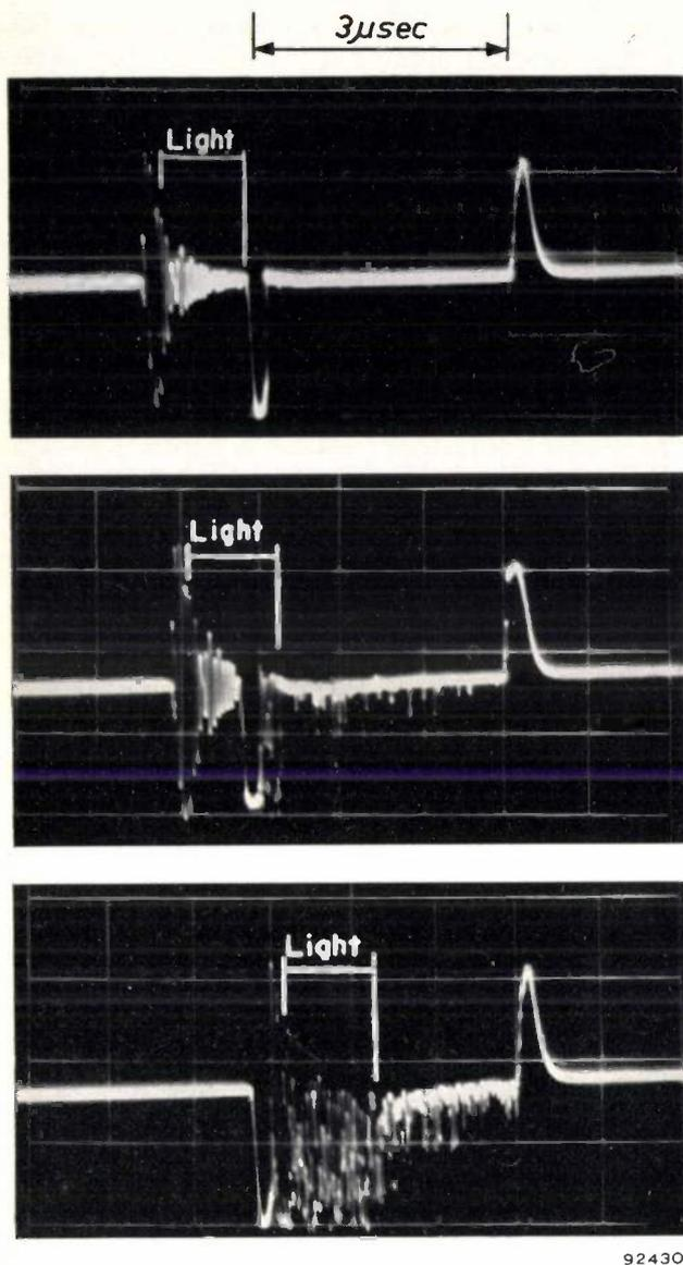
Fig. 9. Same as in fig. 8, at a pulse voltage of 2.0 kV, with a 1  $\mu$ sec light flash falling on the phototube just prior to or in the beginning of the pulse. No afterpulses whatever are recorded in the first case.
