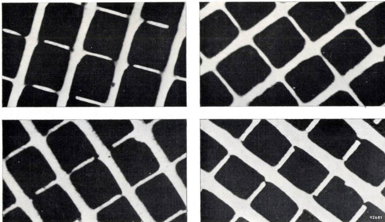
Fig. 11. Comparison of the resolution of emulsion V 6005 (above) and emulsion V 6028 (below). The two micrographs on the left were taken at an anode voltage of 3 kV, the two on the right at 1.5 kV. The object radiographed was a fine silver mesh, the thicker wires being 6 microns in diameter, the thinner 2 microns. It can be seen that the resolution of the experimental emulsion is roughly equal to that of the old; at 1.5 kV it is perhaps slightly better.
