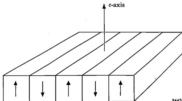
*Fig. 4.* Schematic diagram showing the configuration of Weiss domains in the single-crystal platelets of  $\text{BaFe}_{12}\text{O}_{19}$ . The domain walls are perpendicular to the flat surface of the platelets, parallel to the hexagonal *c*-axis. The arrows show the directions of the magnetization.
