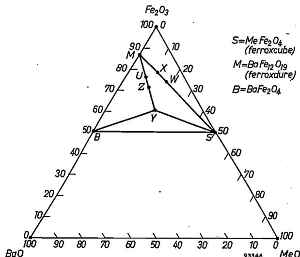
Fig. 1. The composition of the materials W, Y, Z, X and U can be represented by points in the triangle BaO-MeO- $\text{Fe}_2\text{O}_3$ . B, S and M represent the known materials  $\text{BaFe}_2\text{O}_4$ , ferroxcube and ferroxdure, respectively.
