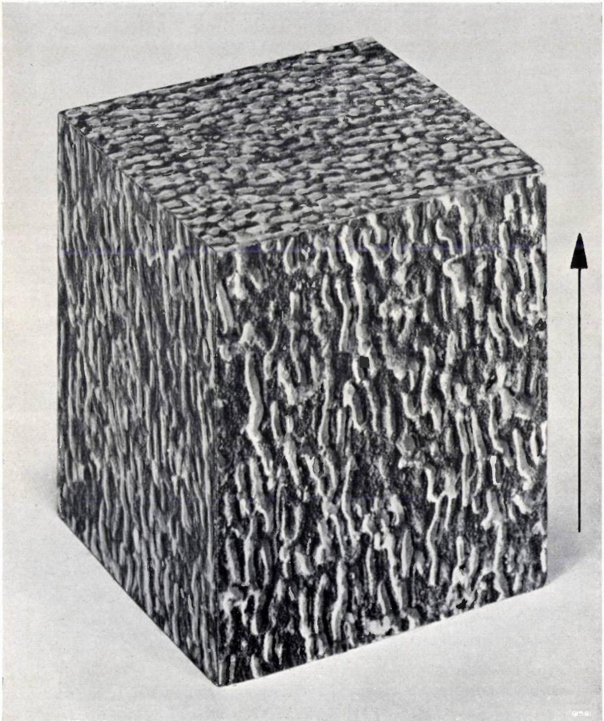
Fig. 1. Photo-montage giving a three-dimensional impression of the metallographic structure of a single crystal of "Ticonal" G. The arrow indicates the direction of the magnetic field applied during the cooling period. This picture was obtained by placing the structural photographs (magnification 160 000 diameters) shown in figs. 2 and 3 on the corresponding faces of a wooden cube.
