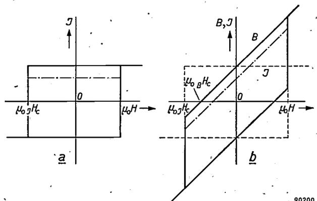
Fig. 7. a) Magnetization  $J$ , and (b) induction  $B$  of ferroxdure, as functions of  $\mu_0 H$  (idealized). The value of  $J$  is shown as the dotted line in (b). The chain-dotted lines in both figures apply to a less strongly magnetized ferroxdure.
