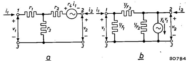
Fig. 2. Equivalent circuits for a linear active fourpole in the form of (a) a 'T' network and (b) a 'II' network.
