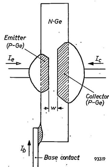
Fig. 6. Diagram showing schematically the construction of a *P-N-P* junction transistor of the alloy type. Most transistors, including all Philips transistors, are of this type.
