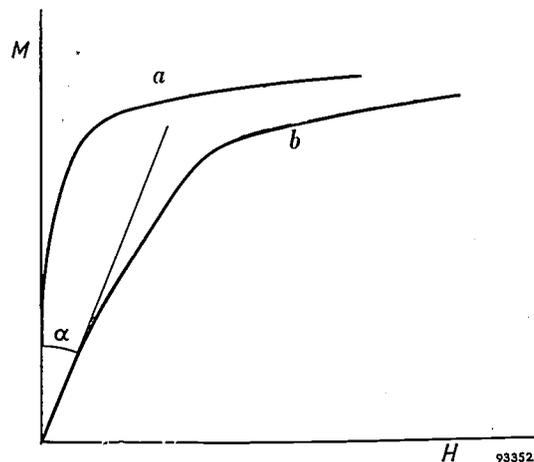
Fig. 10. The ideal magnetization curve. a) No internal demagnetization; b) internal demagnetization factor  $N_i = \tan \alpha$ .
