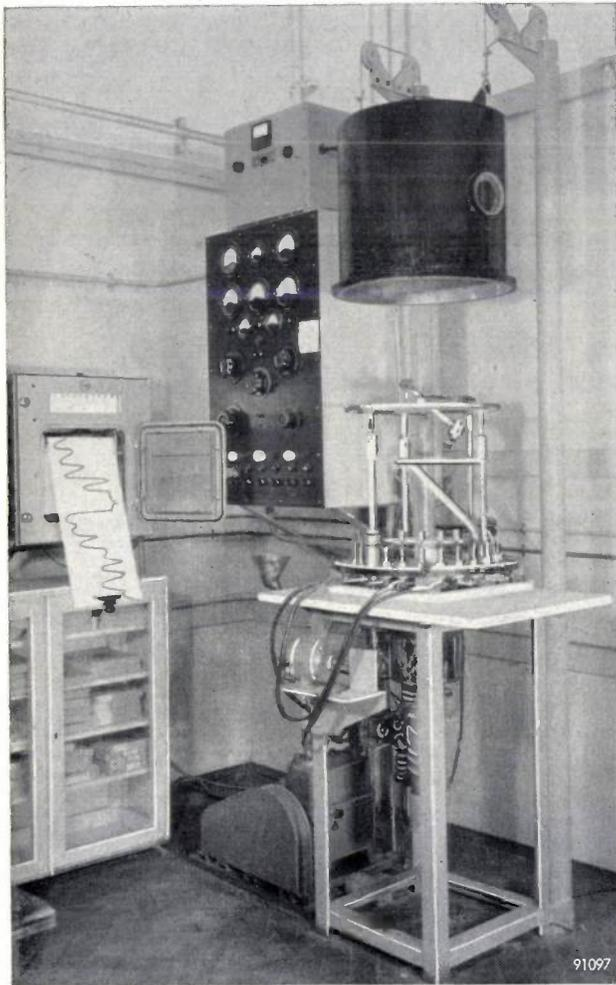
Fig. 7. Equipment for the sublimation of thin films in vacuum. The dome under which the sublimation is carried out (compare fig. 8) is shown raised; in the centre background is the switch-board for the control of the heating current to the evaporation elements. On the left can be seen a recording potentiometer which records the transmission of the glass plate under treatment as a function of the time.
