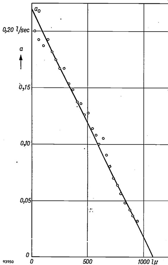
Fig. 9. The absorption of hydrogen by barium shows the appearance of a volume effect: the absorption rate (ordinate) depends linearly on the amount of gas already absorbed (abscissa). Extrapolation of the line drawn through the measured points gives the initial rate (point of intersection with vertical axis) and the total absorption capacity (point of intersection with horizontal axis).
