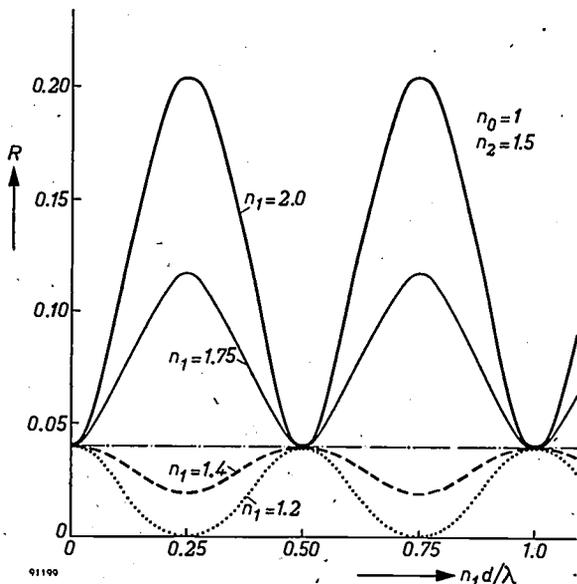
Fig. 4. Reflection coefficient *R* of a thin film (thickness *d*, refractive index  $n_1$ ) as function of  $n_1d/\lambda$ , for various values of  $n_1$ . The refractive indices  $n_0$  and  $n_2$  of the adjacent media are 1 and 1.5 respectively.
