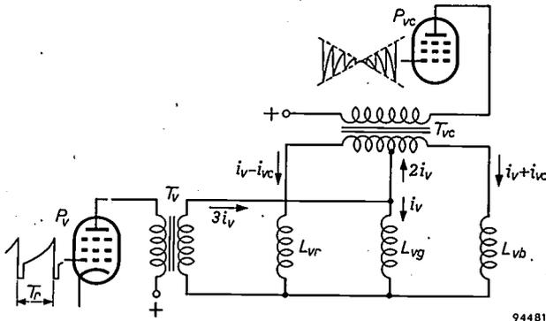
Fig. 13. Circuit for adding  $i_{vc}$ , the current for correcting trapezium distortion, to the frame scanning current  $i_v$  in the inductances  $L_{vr}$  and  $L_{vb}$ . The correction current is delivered by tube  $P_{vc}$ .  $T_{vc}$  is a centre-tapped transformer. The remaining letters have the same meaning as in fig. 11.
