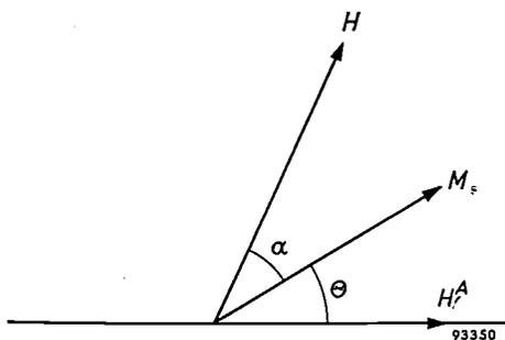
Fig. 5. Rotation of a ferroxplana crystal in an external field  $H$ . Owing to the couples  $\mu_0 H M_s \sin \alpha$  and  $\mu_0 H^A M_s \sin \theta \cos \theta$  acting on  $M_s$ , the preferred plane tends to take up a position parallel to  $H$ .
