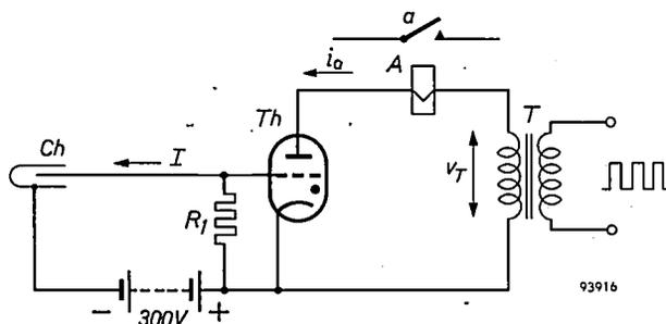
Fig. 11. Simplified circuit of safety amplifier. The current  $I$  from the ionization chamber  $Ch$  produces across resistor  $R_1$  a voltage which, when greater than a critical value, prevents the thyratron  $Th$  from igniting. The relay  $A$  is then de-energized and contact  $a$  opens, the result of which is to stop the reactor. The anode circuit is supplied with a square-wave voltage via transformer  $T$ .
