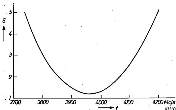
Fig. 2. Standing-wave ratio  $S$  in the input waveguide as a function of the frequency  $f$ .
