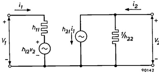
Fig. 1. An equivalent circuit for any linear fourpole can be drawn, given a set of fourpole equations for that fourpole. The above equivalent circuit is that corresponding to the equations involving the  $h$  parameters (equations (1)). The input loop contains a voltage generator of magnitude  $h_{12}v_2$ , the output loop a current generator of magnitude  $h_{21}i_1$ .
