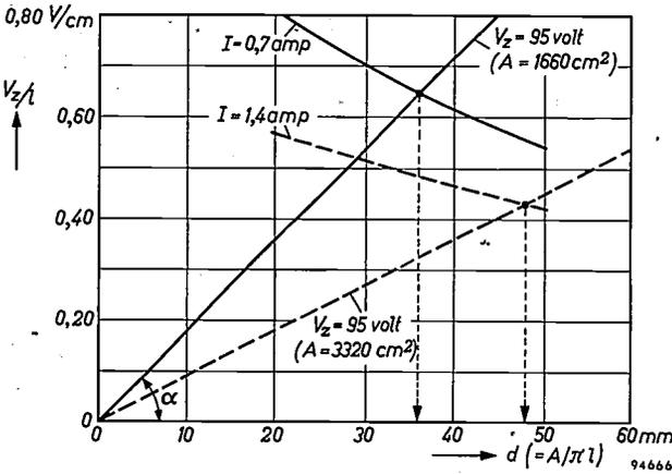
Fig. 1. The curved lines show how the gradient  $V_z/l$  in the column of a low-pressure mercury discharge varies as a function of the internal diameter  $d$ , for various discharge currents  $I$  (for an argon pressure of 1.5 mm Hg).
