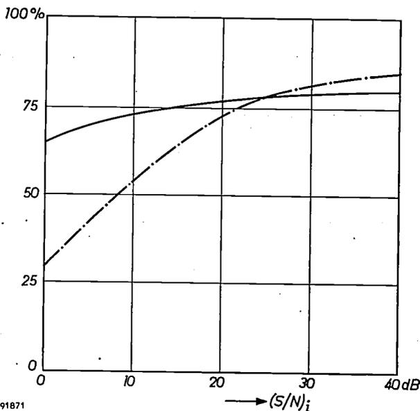
Fig. 5. Intelligibility of speech transmitted by the Frena system (i.e. percentage of sounds, embodied in logatoms, that were correctly recognized), when noise of variable strength was added to the frequency channel. There was still a reasonable degree of intelligibility even when noise and signal had the same power, i.e. when  $(S/N)_i = 0$  dB. The chain-dotted curve relates to normal single-sideband modulation.
