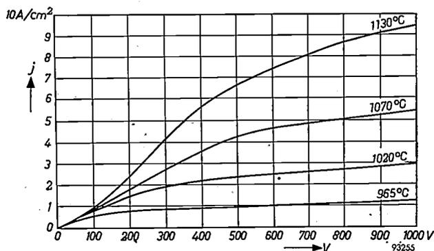
Fig. 5. Current density  $j$  of an impregnated cathode measured in a diode as a function of the anode voltage  $V$ , for various cathode temperatures.
