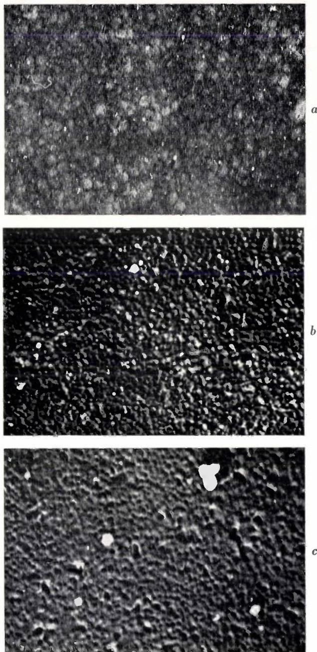
Fig. 8. Photomicrographs made with an electron microscope, of SiO replicas of the surface of barium films having a macroscopic area of 35 cm<sup>2</sup> and containing respectively 0.9, 2.6 and 3.5 mg barium. Magnification 80 000  $\times$ .
