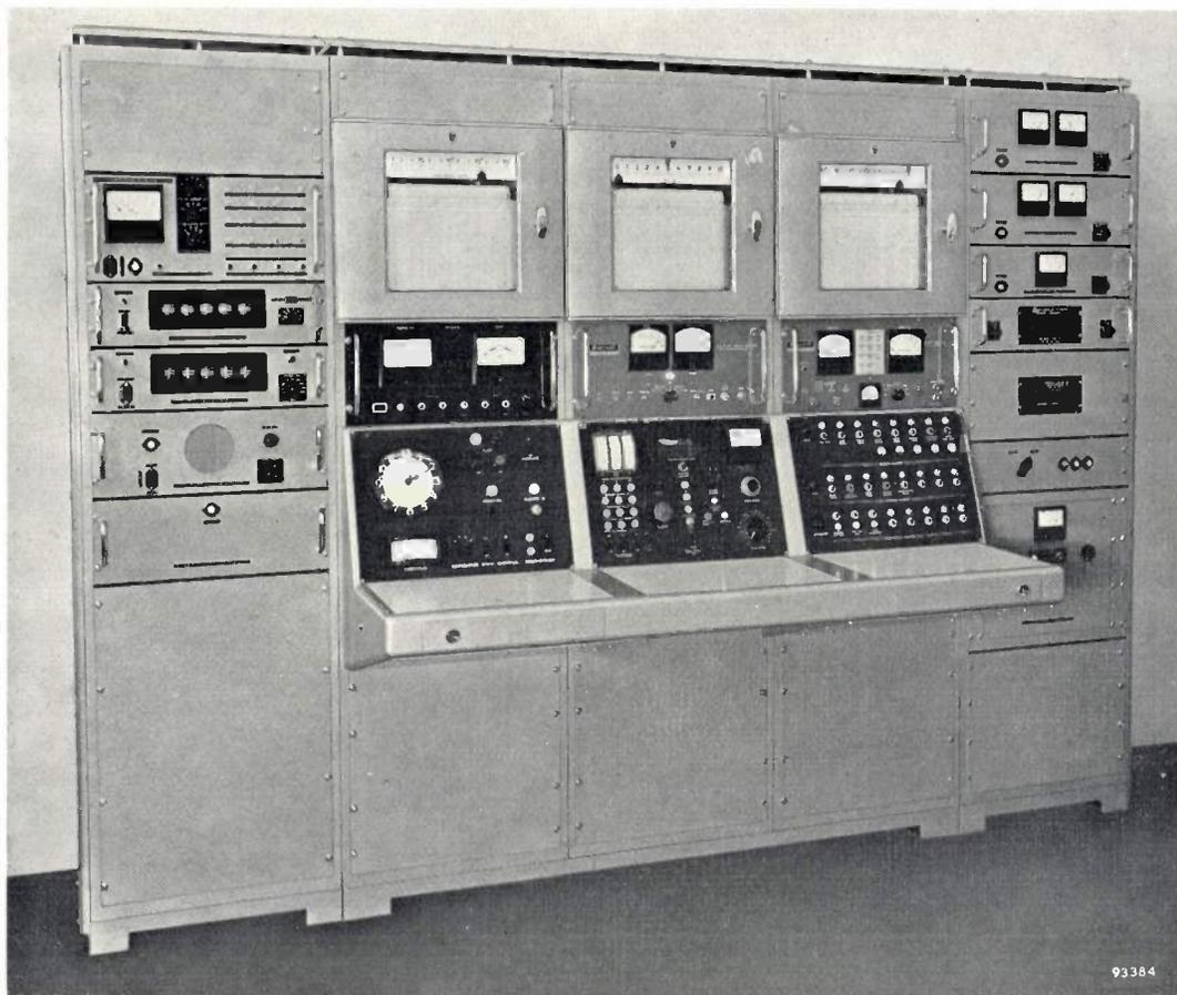
Fig. 3. Console carrying the monitoring control, and safety equipment. Left rack, from above: gamma indicator, pulse counter, pre-set time unit, loudspeaker unit, unit for temperature measurements. The rack on the right contains, among other things, the stabilized voltage sources. For the central section (three racks), see fig. 7.
