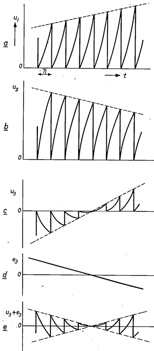
Fig. 15. Voltage waveforms  $u_1$  and  $u_2$ ,  $u_3 (= u_1 - u_2)$ ,  $e_3$  and  $u_3 + e_3$  occurring in the circuit of fig. 14.
