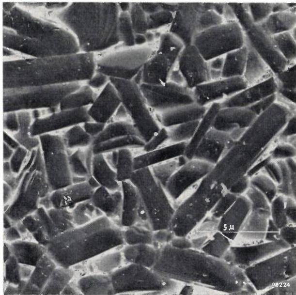
*a* Fig. 7. Photographs of a specimen with fan texture; the direction to which the preferred planes are parallel lies in (a) in the plane of the paper (roughly vertical) and in (b) perpendicular to the plane of the paper.
