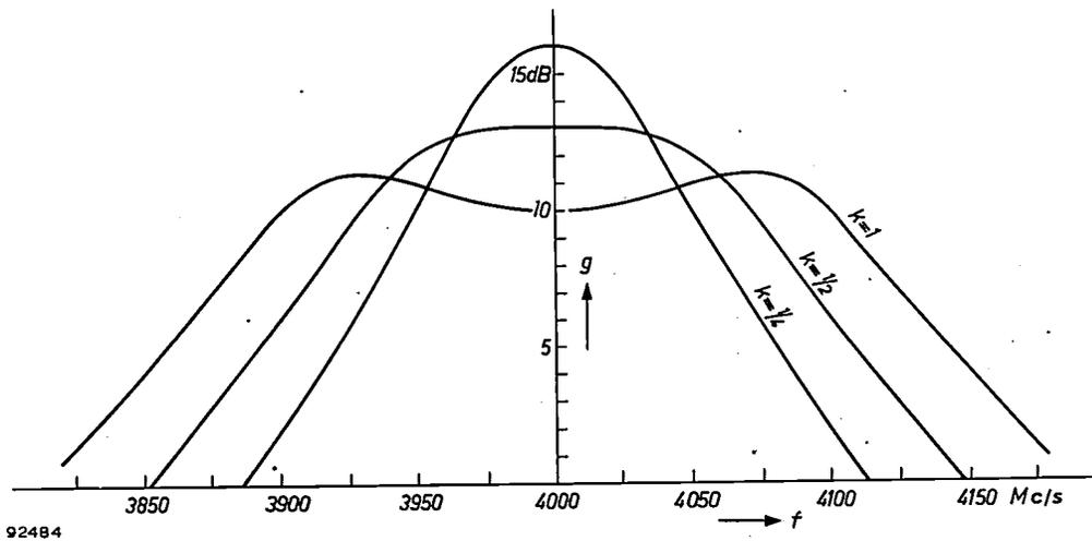
Fig. 10. The gain obtained with an tube EC 57, tuned to a central frequency of 4000 Mc/s, for various values of the coupling factor  $k$ , and an iris bandwidth  $B_i$  of 200 Mc/s.
