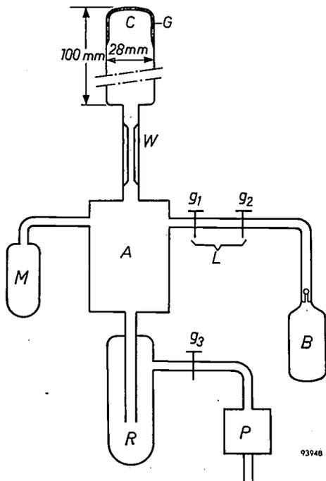
Fig. 6. Set-up used for measuring the "gettering rate" of a barium getter film. A constant quantity of the gas in B is admitted to A via the lock L, consisting of stopcocks g<sub>1</sub> and g<sub>2</sub>. Via the capillary W the gas flows into the bulb C containing the barium getter film G. The time-variation of the pressure in A, measured by a Pirani gauge M, is governed by the permeability of the capillary W and the gettering rate to be measured.
