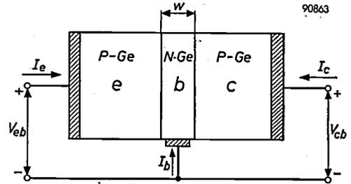
Fig. 4. Schematic diagram of a  $P-N-P$  junction transistor. Between the emitter  $e$  and the collector  $c$ , both of which are composed of  $P$ -germanium, is the thin base layer  $b$ , composed of  $N$ -germanium and having a thickness  $w$ . Each of the three regions has its own connecting wire.
