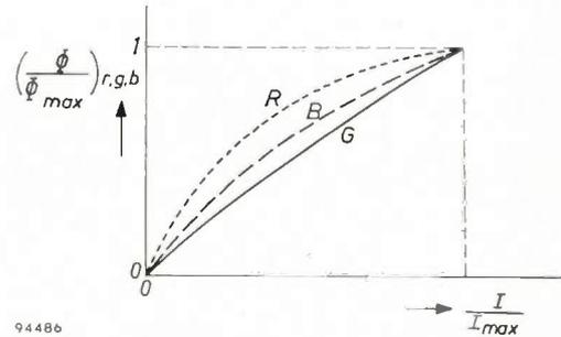
Fig. 18. Ratio of the luminous flux  $\Phi$  to  $\Phi_{max}$  as a function of the ratio of anode current  $I$  to  $I_{max}$ , for the red, green and blue projection tubes (R, G and B respectively). Saturation is heaviest in the red CRT and lightest in the green one.
