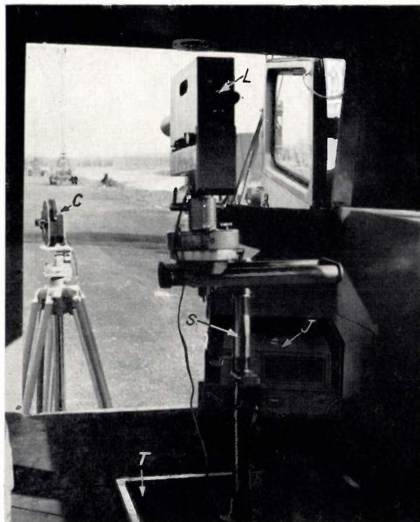
Fig. 5. Interior view (towards the rear) of the van (see also *fig. 2*) equipped with measuring instruments. The luminance meter *L* is mounted on a stand *S*, which is let down to the road through a hatch *T* in the floor of the van. *J* is a luxmeter, *C* a cine camera.
