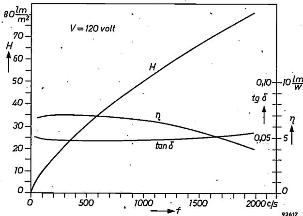
Fig. 7. The same quantities as in fig. 6 plotted as functions of  $f$ , the voltage being constant at  $V = 120$  volts.
