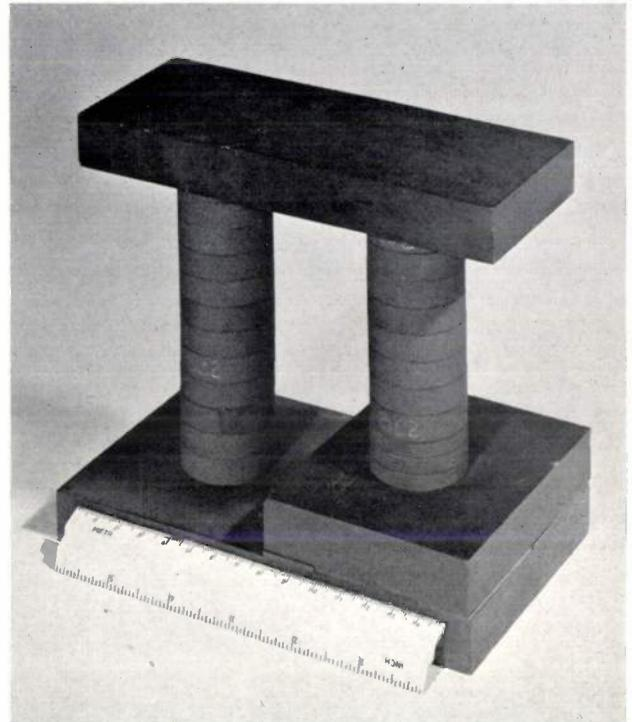
**Fig. 12.** Core of the pulse transformer of a testing installation for magnetrons. Principal dimensions: base 100 × 170 mm, height 162 mm. Further principle data:
