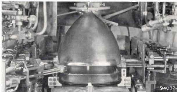
Fig. 9. a) View of the glass-sealing machine, showing the window and cone sections of a 17" picture-tube in position. The burners are withdrawn.
