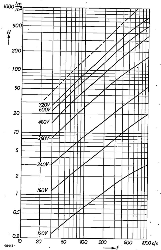
Fig. 3. If the r.m.s. value of voltage  $V$  applied to the cell be kept constant, emittance  $H$  increases near enough directly proportional to frequency  $f$ . (The curves are roughly parallel to the broken line at  $45^\circ$ .)
