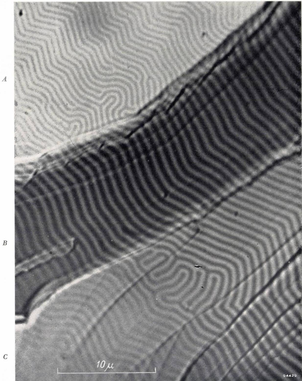
Fig. 3. Similar photo to that of fig. 2, showing another region of the same platelet. Terraced thickening of the specimen can be seen in this region by the dark broad bands across the pattern. The Weiss domains are seen to be wider within these dark bands. The "contraction" of the pattern on passing the boundary from a thick to a thinner place is at some points taken up by dislocation-like imperfections in the pattern.
