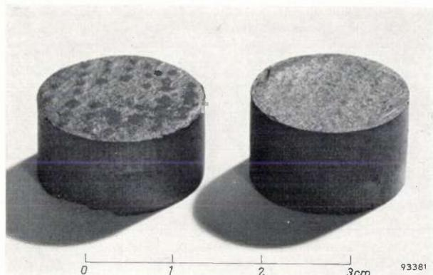
Fig. 8. Anisotropic shrinkage occurs during the sintering of an aligned pressed material. *Right*: an unaligned specimen; *left*: an aligned specimen with foliate texture. In the latter case there is considerable shrinkage in the direction of the  $c$ -axes of the crystals, but less at right angles to that direction. Before sintering, the dimensions of both specimens were identical.
