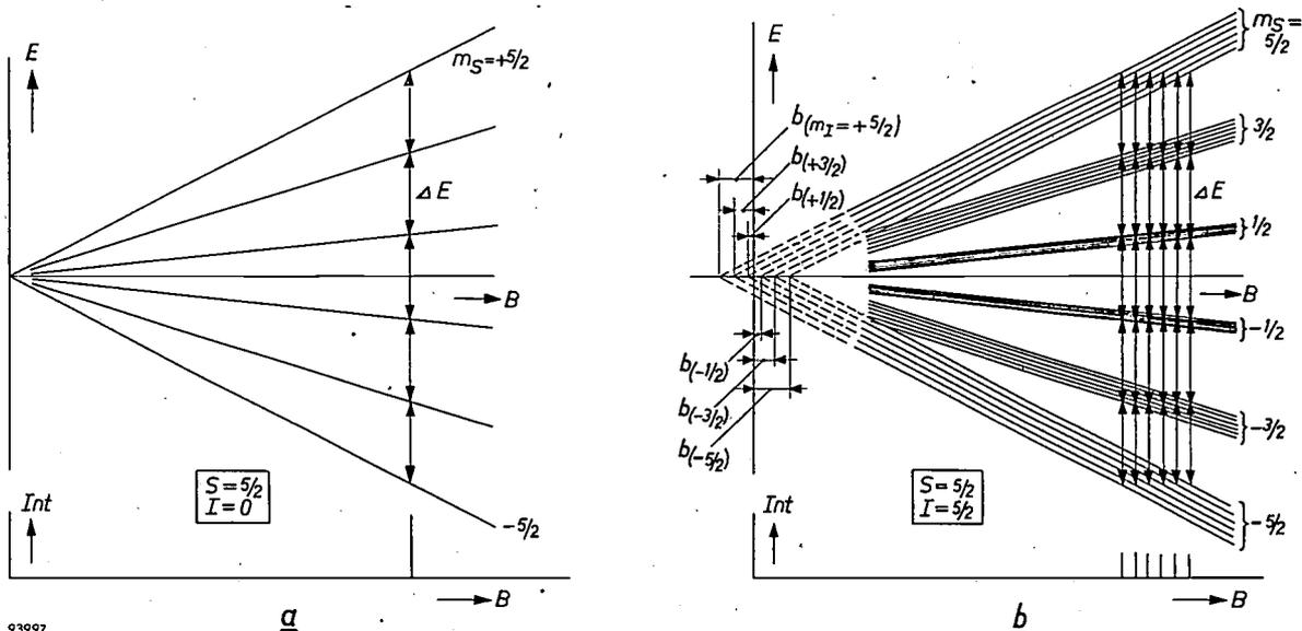
Fig. 5. a) Energy-level scheme of an ion with  $S = \frac{5}{2}$  in a magnetic field  $B$ ; below, the resulting resonance spectrum (intensity  $Int$  as a function of  $B$ ), which in this case consists of a single line.
