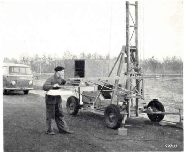
Fig. 2. Changing a fitting in one of the masts. The arm is brought down to its lowest position on the mast. The fitting is mounted on a frame which is slid on to the arm. The frames also fit in the slots at the sides of a compartment in the trolley; the compartment is made light-tight by a sliding panel (see also fig. 3). A van equipped with measuring instruments can be seen on the left (see also fig. 5).
