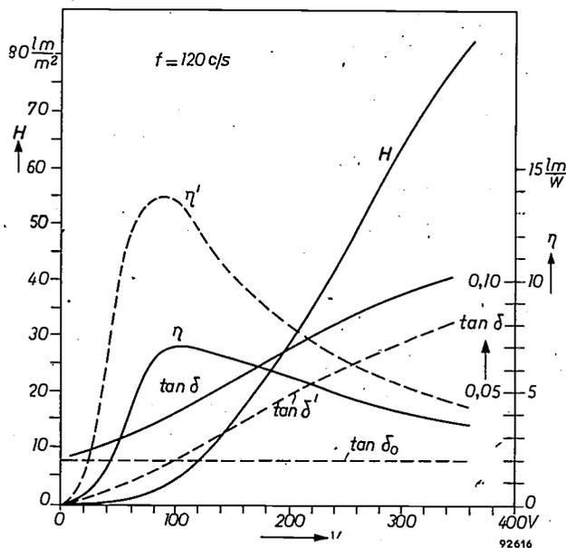
Fig. 6. Power factor tan δ, emittance *H* (in lumens/m<sup>2</sup>) and efficiency η (in lumens/watt) as functions of voltage *V*, the frequency being constant at *f* = 120 c/s, as obtained from measurements on a luminous panel giving green light. The dotted-line curves refer to the intrinsic efficiency η' (efficiency when the loss corresponding to tan δ<sub>0</sub> is neglected, see text).
