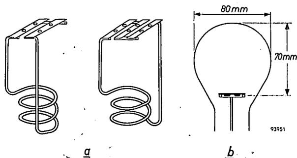
Fig. 10. a) Getter holders made by combining two and three strips, respectively, and provided with a coiled support for induction heating.
