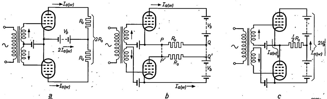
Fig. 2. a) Conventional push-pull circuit. b) Circuit which is electrically equivalent to (a). By interconnecting  $P$  and  $P'$  and  $Q$  and  $Q'$ , the single-ended push-pull circuit (c) is obtained, which matches to a 4 times lower load resistance ( $\frac{1}{2}R_0$  instead of  $2R_0$ ), whilst no D.C. flows through the load.
