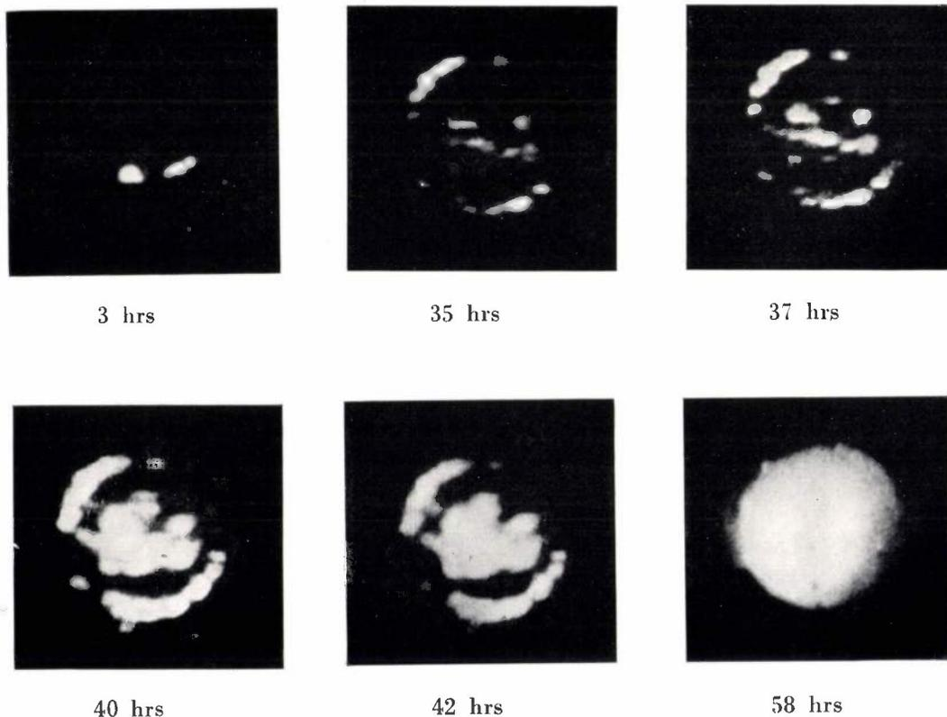
Fig. 7. Electron-optical images of the emitting cathode on a fluorescent screen, photographed at various phases in the activation process. (The latter was performed at 950 °C and was therefore much slower than normal.) The activation time is indicated under each photograph.
