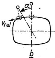
Fig. 6. a) Relative speed ( $v_{rel}$ ) of a burner with respect to the glass, as a function of the position (angle  $\alpha$ ) of the burner carriage with respect to the revolving glass parts. The broken curve is that which would be obtained if the burner, instead of swivelling, were always pointed radially inward. b) Sketch illustrating the definition of  $\alpha$ .
