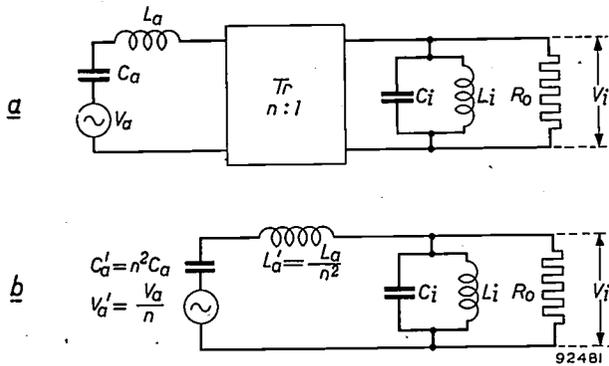
Fig. 6. a) Equivalent circuit in which the tube is represented by a voltage source  $V_a$ .  $L_a$  and  $C_a$  represent the anode resonant cavity, while  $L_i$  and  $C_i$  represent the iris. The iris is damped by the characteristic impedance  $R_0$  of the output waveguide. The transmission system between resonant cavity and iris is represented by a transformer  $Tr$  with a transformation ratio  $n$ .
