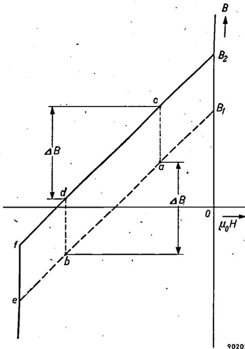
Fig. 10. *a-b* working line of a ferroxdure magnet completely filling the gap of the pulse transformer; remanence  $B_1$ . If the gap is partly filled with more strongly magnetized ferroxdure (remanence  $B_2$ ), the working line becomes *c-d*, situated vertically above *a-b* and along the characteristic  $B_2f$ , which runs parallel with  $B_1e$ . The change in induction  $\Delta B$  as well as the safety factor is the same in either case (at least in these idealized curves).
