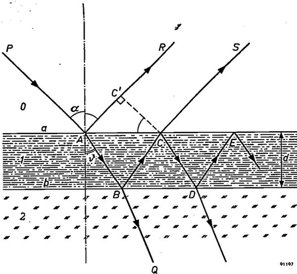
Fig. 2. As in fig. 1 but now for oblique incidence. Some of the multiple reflections are shown.
