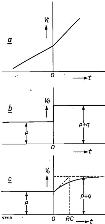
Fig. 4. a) Voltage  $V_i$  linear with time  $t$ , but with a discontinuity in the derivative at  $t = 0$ :
