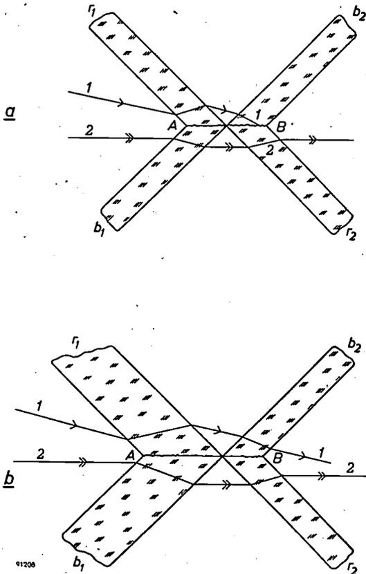
Fig. 14.  $r_1 r_2 - b_1 b_2$  are dichroic mirrors in an arrangement differing slightly from that in fig. 12. In (a) ray 2 which enters parallel to the boundary plane  $AB$ , can pass unhindered, but the obliquely incident ray 1 is lost in  $AB$ . In (b) the first mirrors ( $r_1$  and  $b_1$ ) are made so thick that ray 1 is laterally displaced far enough to avoid  $AB$ .
