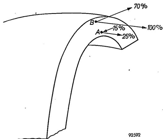
Fig. 3. Section of rim after cleating by old method; external diameter (before cleating) 4 mm. At *A* the radial and tangential deformations are about 15% and 25% respectively; at *B* about 70% and 100%.
