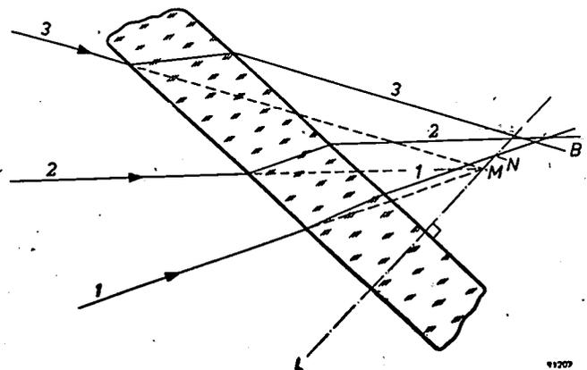
Fig. 13. The thickness of the glass of the semi-reflecting mirror produces aberrations in the transmitted beam: the rays 1, 2 and 3 converging towards  $M$  no longer intersect in one point after passing through the mirror.
