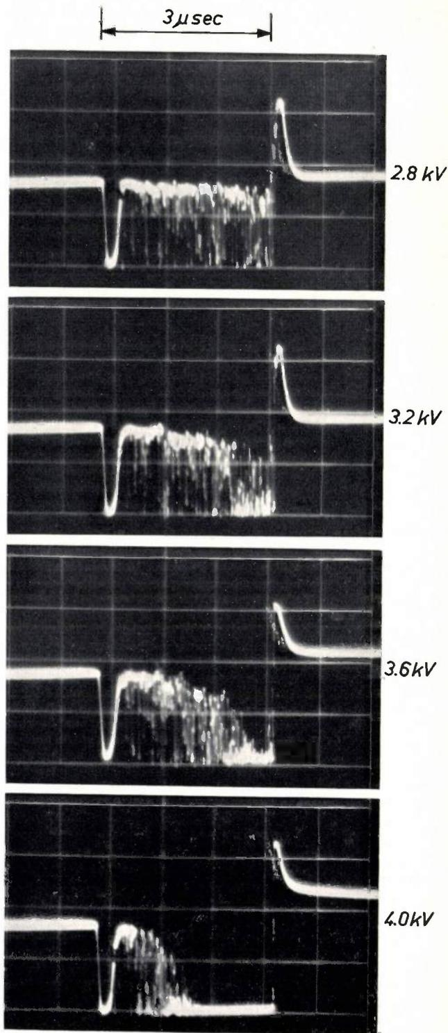
Fig. 8. Oscilloscope traces of the output of a photomultiplier tube during a single 3  $\mu$ sec pulse, with no illumination, at high pulse voltages (peak value indicated at the right). The numerous pips probably are due to positive ions from residual gas in the tube (gas noise). The density of pips at the highest voltages becomes so large towards the end of the pulse as to cause a continuous trace.
