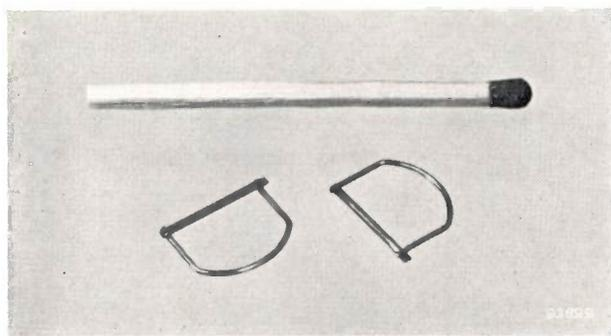
*Fig. 1. a)* Illustration of a getter holder having the form of a longitudinally ground-off tube. The "stirrup" welded to it makes it possible to heat the holder by induction.
