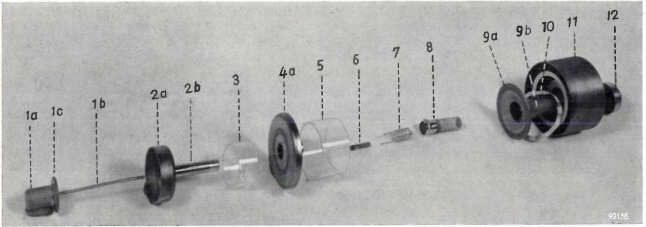
Fig. 3. Exploded view of the TBL 2/300 tube. Symbols as in fig. 2.
