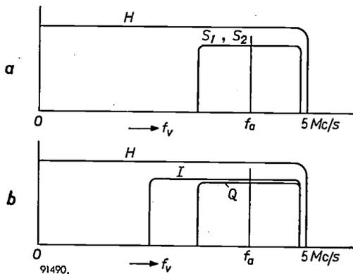
Fig. 14. a) Video-frequency spectrum in which the two colour signals,  $S_1$  and  $S_2$ , have equal bandwidths. Each is modulated with two sidebands of limited width on a subcarrier with video frequency  $f_a$ ; the two subcarriers are  $90^\circ$  out of phase with each other. b) Video-frequency spectrum in which the two colour signals,  $I$  and  $Q$ , have different bandwidths (see (19) and (20)). In this case,  $I$  can have a wider lower sideband. This system is employed in America.
