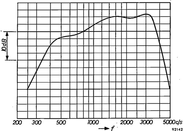
Fig. 7. Frequency characteristic of the microphone. The quantity actually plotted is the voltage across a resistor of 1000  $\Omega$  terminating the microphone, the latter being in a sound field of constant pressure.
