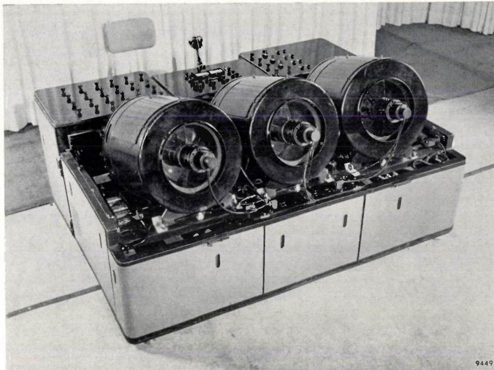
Fig. 20. Large-picture projection set with cover removed. The Schmidt optical systems, which are of the "in-line" type, are mounted side by side. See also figs. 21 and 22.
