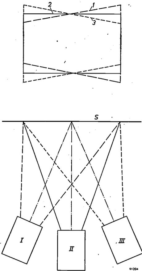
Fig. 10. The pictures from the three projectors *I*, *II* and *III* on the screen *S* do not properly coincide, since the projectors *I* and *III*, placed at an angle, give trapezium-shaped pictures (*1* and *3*), and the projector *II* a rectangular picture (*2*).
