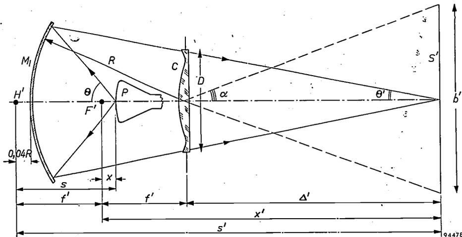
Fig. 9. Schmidt optical system of the "in-line" type. *P* projection tube. *M*<sub>1</sub> concave mirror of radius *R*. *C* corrector plate of diameter *D*. *S* projection screen, the image on which is of breadth *b'*. *F'* focus of mirror plus corrector plate. *H'* pole of mirror plus corrector plate.
