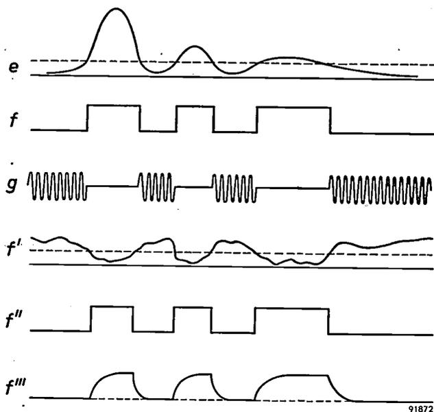
Fig. 6. In the Frenac system the amplitude component ( $e$ ) of the speech signal is reduced to a square waveform ( $f$ ) that is transmitted in the form of short wave-trains ( $g$ ). Detection at the receiving end yields a signal ( $f'$ ) that has been deformed by interference; but this can be used to reconstruct the square waveform ( $f''$ ) which, after rounding off ( $f'''$ ), serves to switch the frequency channel on and off at the appropriate instants.
