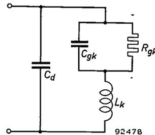
Fig. 3. Equivalent circuit of the amplifier input.  $R_{gk}$  is the input resistance between grid and cathode,  $C_{gk}$  the capacitance between these electrodes;  $L_k$  the inductance of cathode base and cathode disc, and  $C_d$  the capacitance between grid disc and cathode disc.
