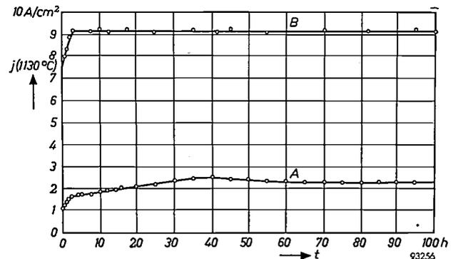
Fig. 6. The improvement in the emission of the impregnated cathode on replacing the barium aluminate (curve A) by barium-calcium aluminate (curve B). The graph shows the rise in current density during activation subsequent to seal-off.
