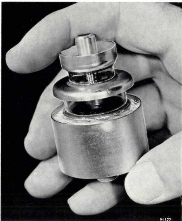
Fig. 1. The transmitting triode TBL 2/300.
