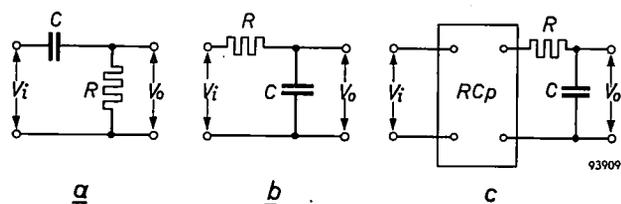
Fig. 3. a) Non-ideal differentiator. b) Non-ideal integrator. c) The non-ideal differentiator (a) is equivalent to the ideal differentiator  $RCp$  and the non-ideal integrator (b) in cascade.
