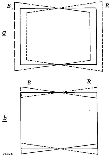
Fig. 7. a) Outlines of the three primary-colour images on the projection screen prior to correction (cf. *fig. 5b*). b) Application of the correction illustrated in *fig. 6* brings the vertical edges of the three images into coincidence. To get complete coincidence of the images, correction of the vertical (frame) scanning is further necessary — see *fig. 8*.
