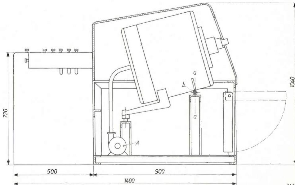
Fig. 21. Sketch showing the principal dimensions of the large-screen projector shown in figs. 20 and 22. Controls within the operator's reach allow him to turn the primary-colour projectors about a vertical axis *a-a* (in a ball and socket joint) and about a horizontal axis *b-b* (perpendicular to the plane of the drawing). *A* is the fan for cooling the projection tubes.
