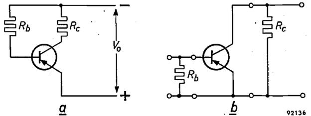
Fig. 5. a) The direct-current circuit of an amplifier stage, for the case that the resistors  $R_b$  of fig. 3a are connected directly to the battery; b) alternating-current circuit.
