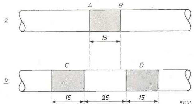
Fig. 9. Schematic diagram of the recrystallization experiments designed to obtain crystal boundaries with the certainty that the crystals involved had been nucleated far apart from each other. A sleeve ("shunt") was fixed around the wire. Within the shunt the wire is less strongly heated, so that recrystallization cannot occur there. The dimensions are given in mm. The "cold" sections are shaded in.
