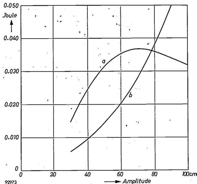
Fig. 7. The energy supplied per period to the pendulum (curve  $a$ ) and that lost by air resistance (curve  $b$ ) as a function of amplitude of swing. At an amplitude of approx. 80 cm the curves intersect. At smaller amplitudes the energy supplied is greater than that lost, i.e. the point of intersection represents a stable state of equilibrium.
