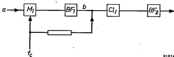
Fig. 8. Block diagram of a simplified circuit at the transmitting end of a Frenac system.
