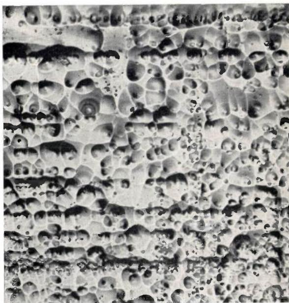
Fig. 6. Etch pits produced after etching a (100) plane, containing slip lines, of a plastically bent germanium crystal. The rows of pits lie along the intersections with (111) planes i.e. along  $[110]$  directions.
