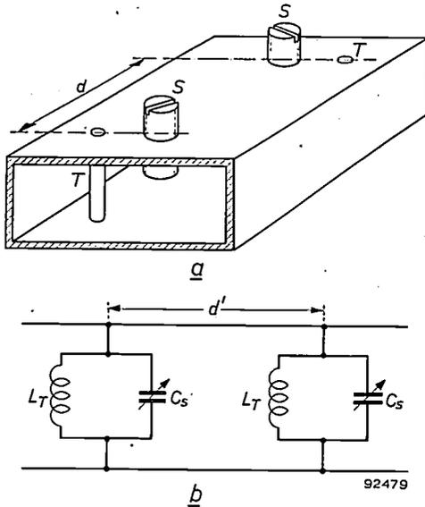
Fig. 4. a) The input waveguide contains two variable reactive elements, each of which consists of a screw  $S$  and a rod  $T$ . The distance  $d$  is approximately one-eighth wavelength. b) Equivalent circuit of the arrangement in fig. 4a.  $C_S$  and  $L_T$  are respectively the "capacitance" of the screw  $S$  and the "inductance" of the rods  $T$ . The distance  $d'$  is about one-eighth wavelength.
