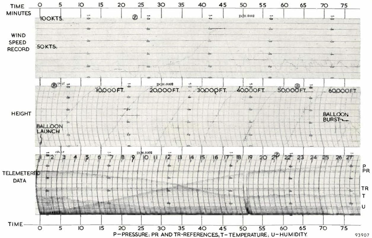
Fig. 9. Example of wind-speed, height and telemetering records obtained from the radar sonde system.
