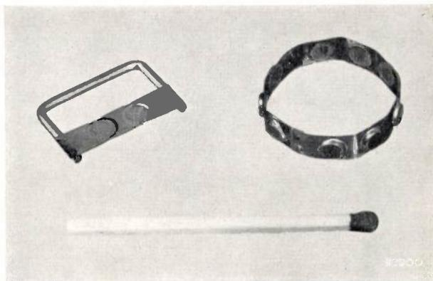
*Fig. 2.* Getter holders made from a metal strip with round equally spaced depressions containing barium "pills". For the purpose of induction heating a loop is welded to the getter shown on the left. The other consists of a longer strip bent to form a ring.
