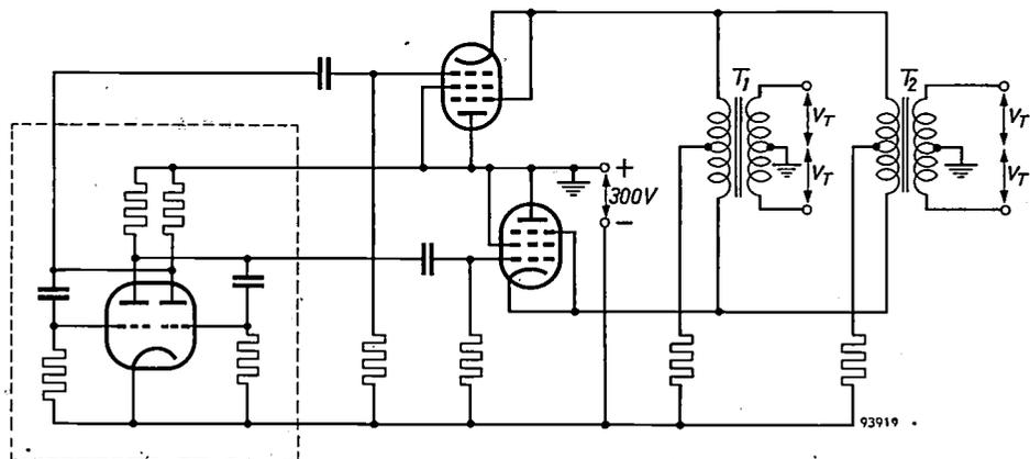
**Fig. 15.** Circuit diagram of 2000 c/s square-wave generator. Inside the broken lines is the multivibrator with double triode E 90 CC. Right, balanced push-pull output stage with two pentodes EL 34 giving cathode-follower output.  $T_1$  and  $T_2$  are the output transformers, each of which supplies two safety amplifiers.
