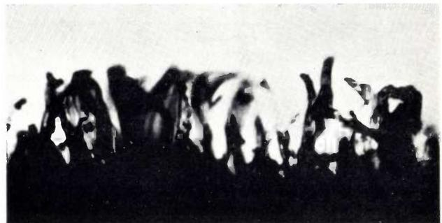
Fig. 6. Molybdenum-oxide crystals, which can form on the electrodes of the 155 UG if the peak current through the tube is too low. Magnification 30x.
