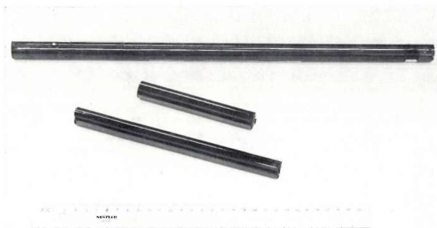
Fig. 5. Some ceramic rods made by continuous hot pressing.
