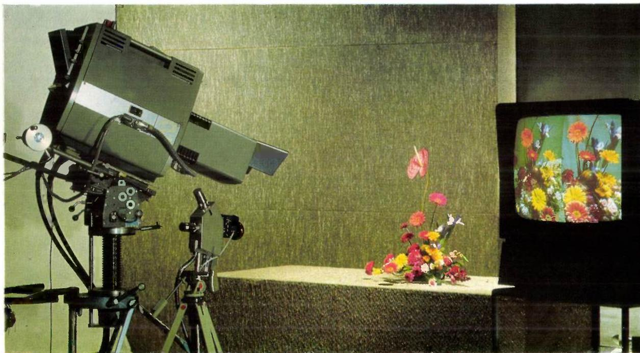
Fig. 13. The studio camera described in reference [4], and the miniature camera, both equipped with "Plumbicon" tubes. The "intermediate unit" (fig. 11) associated with the miniature camera is not shown. Both cameras are taking pictures of the same object to give a comparison of the picture quality: an electronic switching circuit permits the two pictures to appear side by side on the monitor screen at the right.
