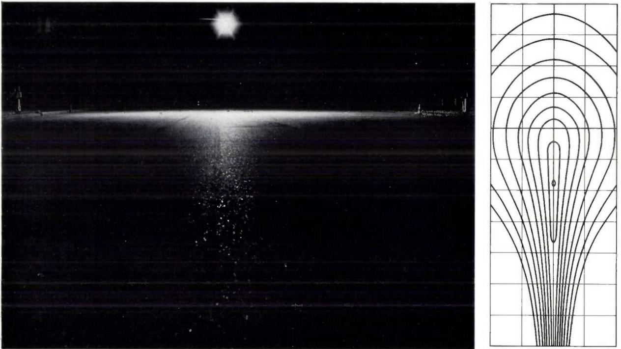
Fig. 3b. The road surface to which the luminance-factor diagram of fig. 3a applies, lighted by a lamp without a lantern ( $I = \text{constant}$ ). The luminance distribution thus obtained is proportional to the luminance factor distribution (shown again on the right); the photograph gives a kind of perspective picture of the distribution.
