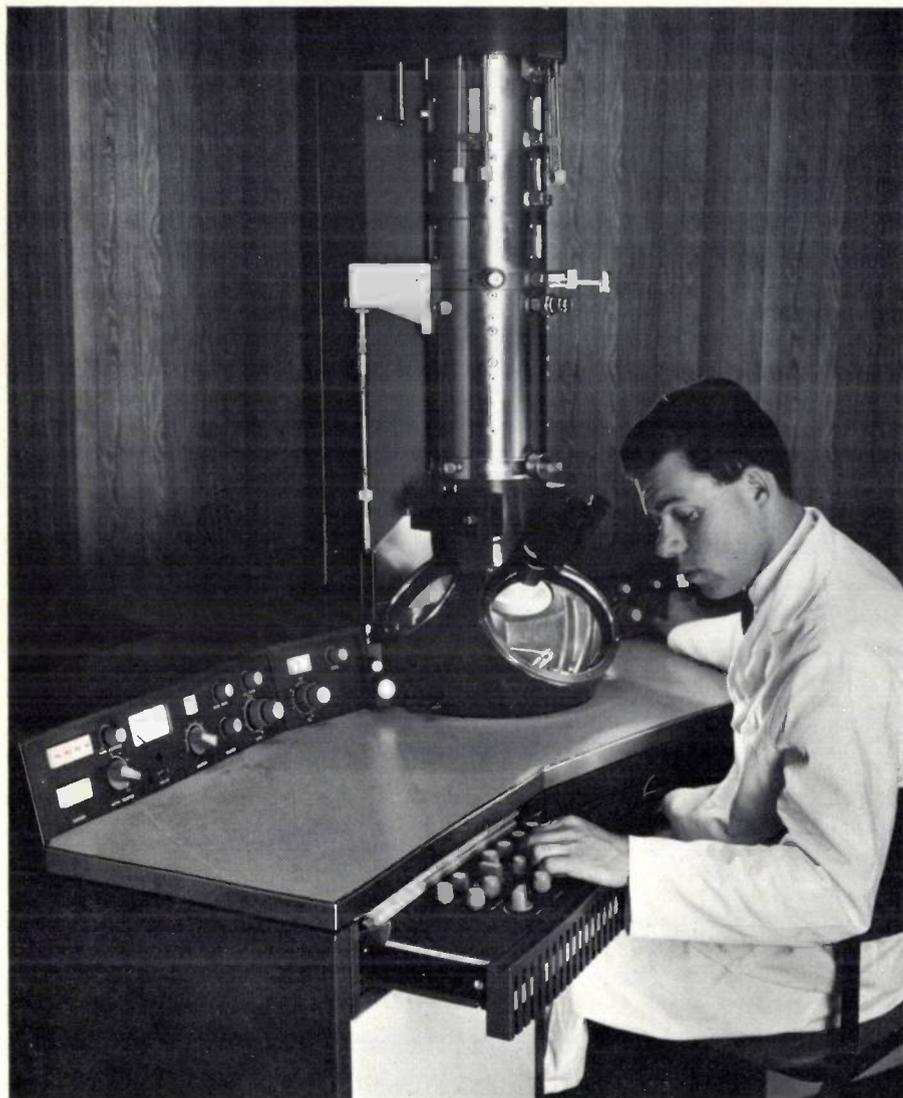
Fig. 2. The operating controls that are most frequently needed are within easy reach above the table-top; the others are on sliding panels immediately below it.
