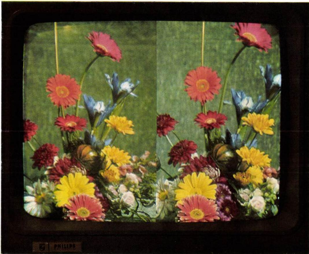
Fig. 14. The monitor screen in the experiment shown in fig. 13. The left-hand half shows the picture from the studio camera, which for this experiment was fitted with "Plumbicon" tubes of increased red sensitivity. The right-hand half of the screen shows the picture from the miniature camera.
