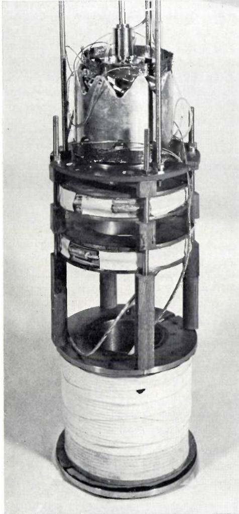
Fig. 13. A superconducting magnet coil (below) complete with superconducting dynamo (above).
