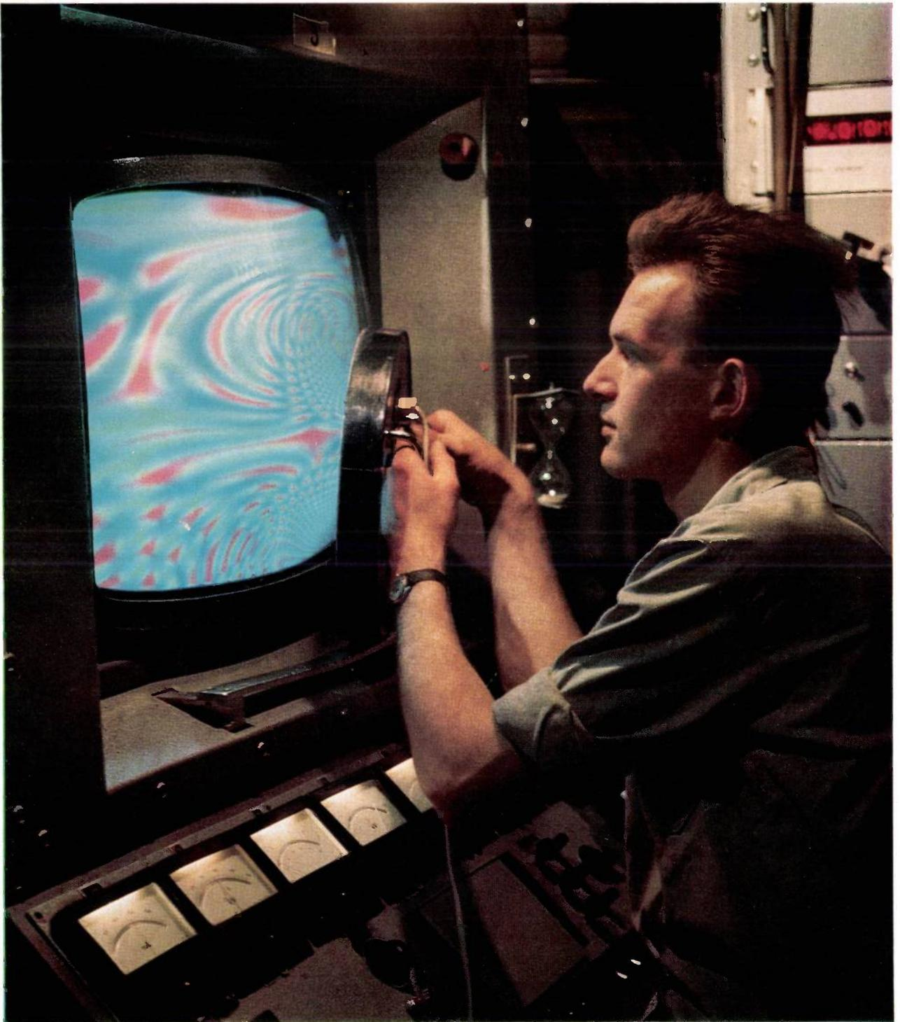
In colour-television tubes of the type now in use (shadow-mask tubes) the picture is traced out on the screen by three electron beams. The red, green and blue fluorescent phosphor dots are arranged on the screen in a repetitive pattern designed so that the transmission by the shadow mask of the three beams,
