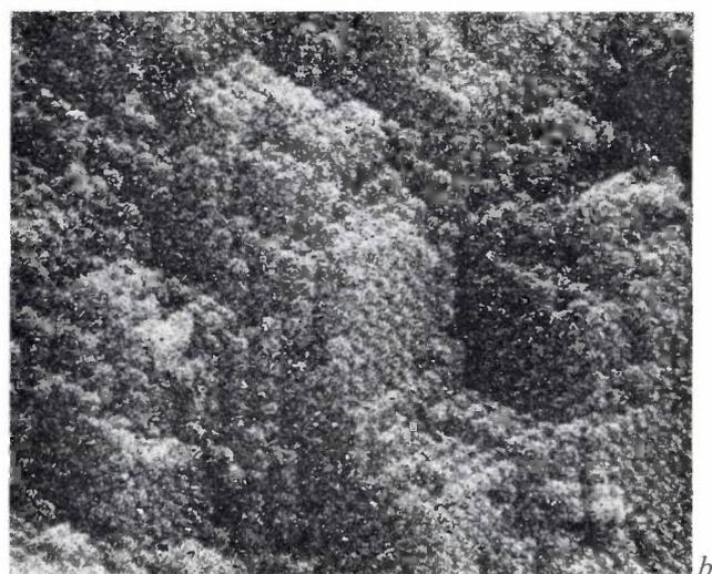
**Fig. 8.** Effect of the scanning rate on the image quality. *a)* Time for one line scan 125 ms. *b)* Time for one line scan 1 ms. The images were produced from a synthetic opal specimen, provided by Mr. B. Dawson, Monash University, Clayton, Melbourne, Victoria, Australia. Magnification 9000 $\times$ .
