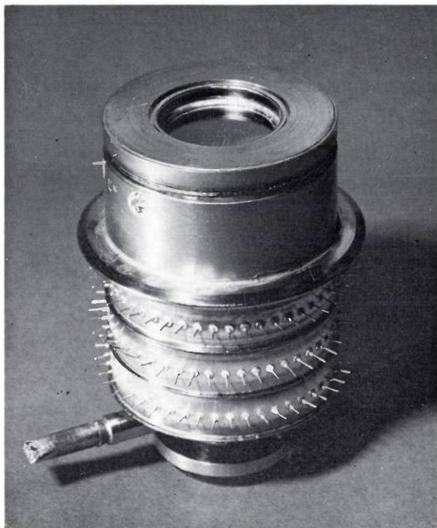
**Fig. 4.** Dewar vessel for cooling an infrared-detector array consisting of a large number of elements. The synthetic sapphire window has been brazed into the metal dewar wall at the top. A large number of ceramic-insulated connectors are brazed into the wall.
