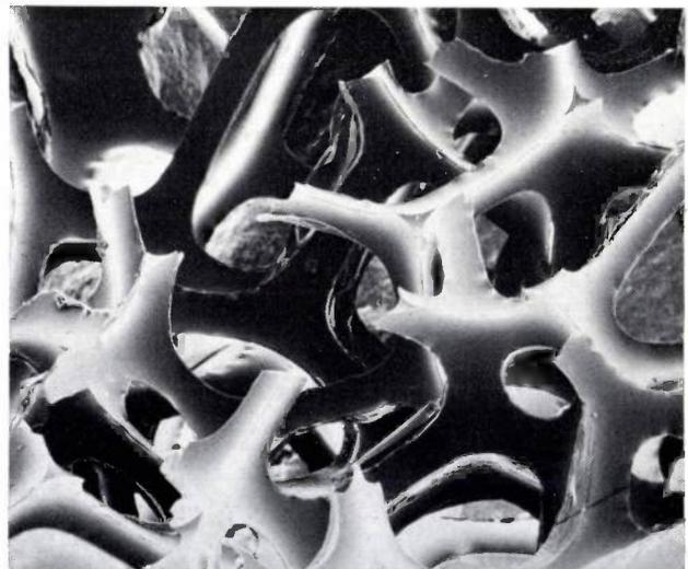
**Fig. 1.** Scanning-microscope picture of plastic foam, coated with an extremely thin gold film for this picture. The depth of field is clearly much greater than the resolving power. This is different from optical microscopy, where the two quantities are approximately equal. Magnification 75 $\times$ .
