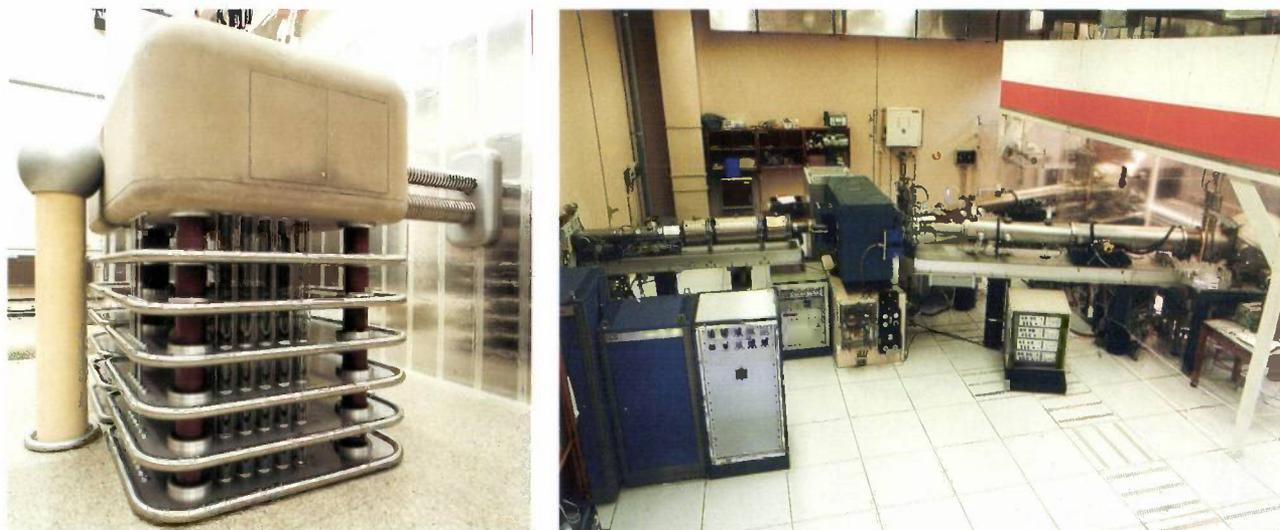
Fig. 3. Photograph of a) the high-voltage section and b) the low-voltage section of the 800-kV ion-implantation machine.
