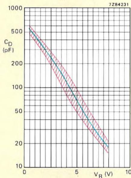
Fig.3 Typical voltage/capacitance characteristic for variable capacitance diode pair BB212. The shaded area indicates the characteristic spread for 98% of all components dispatched from the factory
