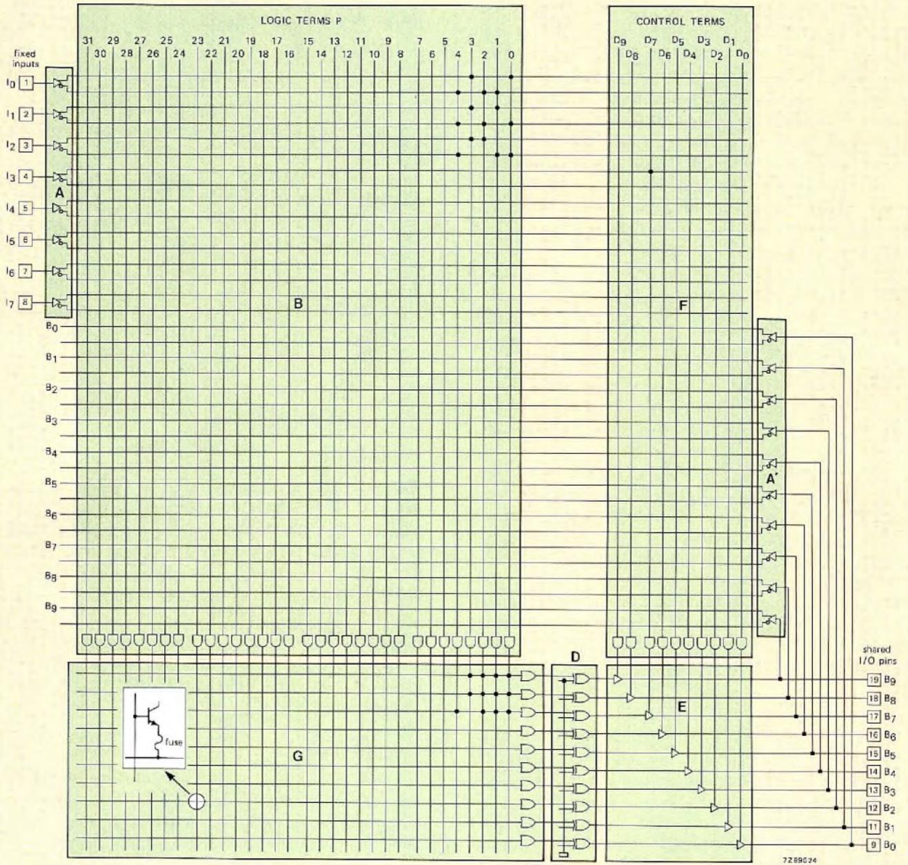
Fig.2 Field-programmable logic array 82S153. A to F, as in Fig.1. G, sum (OR) matrix. Connected as shown, the array is programmed as a single-bit full adder with Carry Enable
