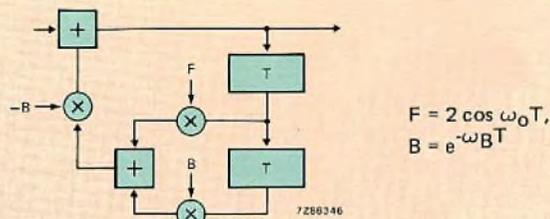
Fig.6 Three-multiplier resonator
