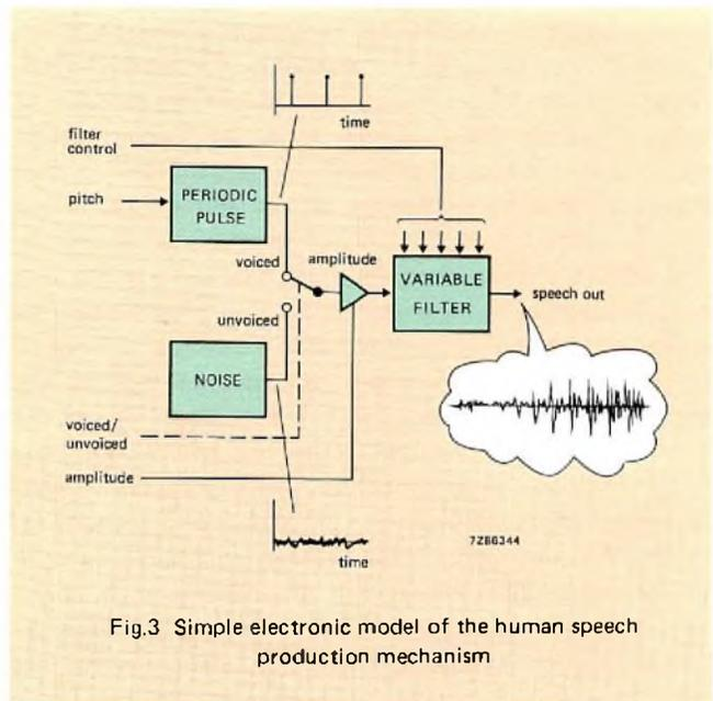
Fig.3 Simple electronic model of the human speech production mechanism
