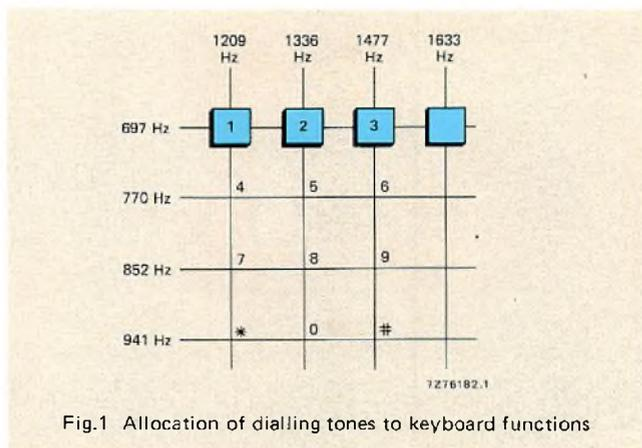
Fig.1 Allocation of dialling tones to keyboard functions
