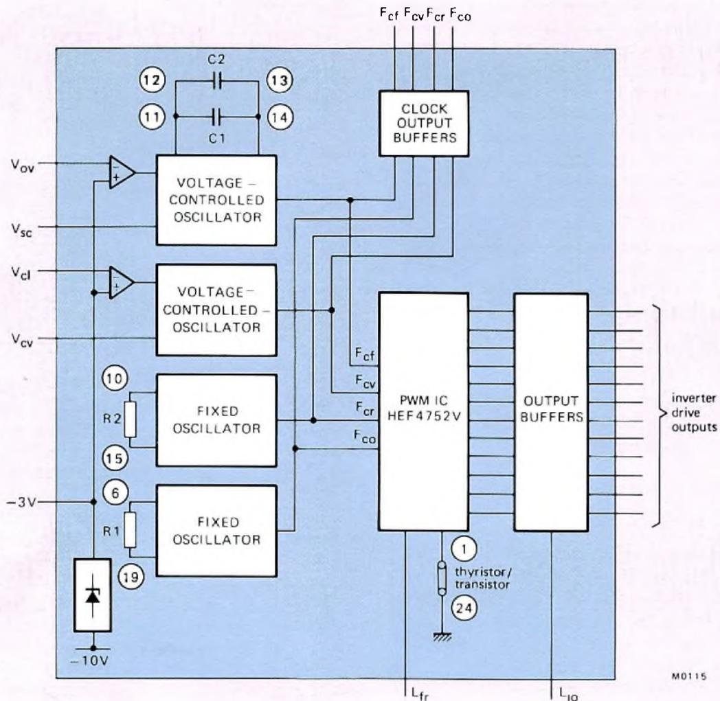
Fig.8 Block diagram of PWM waveform generation module
