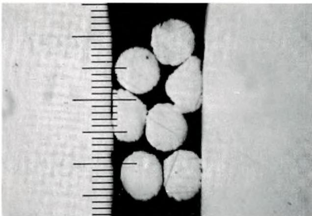
Fig.4 The strands in a stranded conductor are rearranged before deforming to form the actual joint. Microphotograph at 50 X magnification
