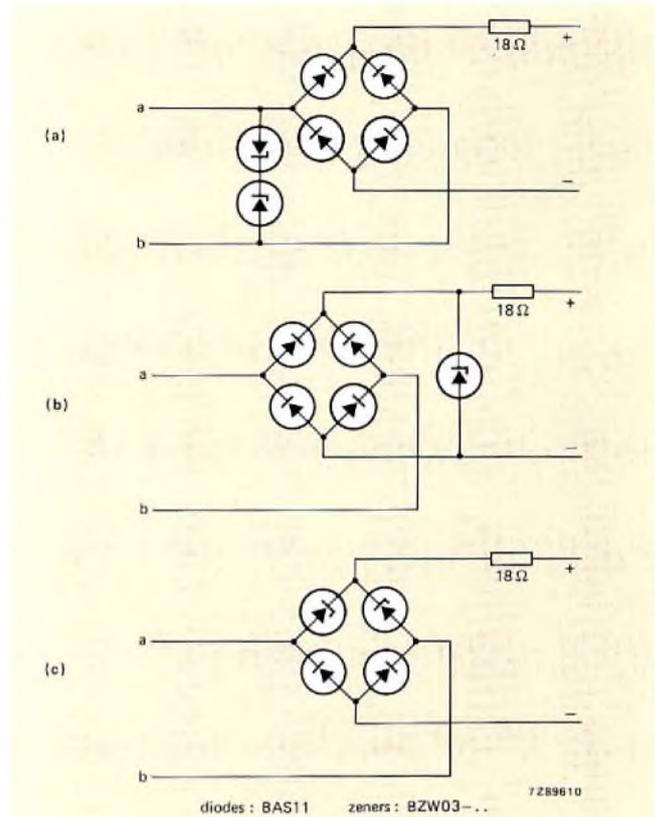
Fig.13 Polarity-guards and line-transient suppression circuits
