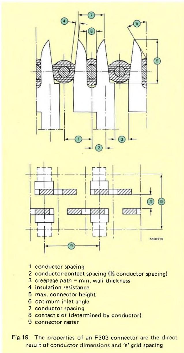
Fig.19 The properties of an F303 connector are the direct result of conductor dimensions and 'e' grid spacing
