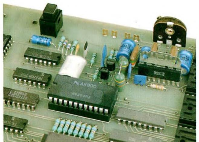
Part of a demonstration board incorporating the MEA8000 voice synthesiser and an integrated output stage TDA1011
