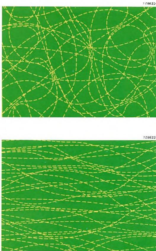
Fig.16 Arrangement of the molecular filaments in PVC, (a) unextruded; (b) extruded. Note the areas of crystallisation in both cases
