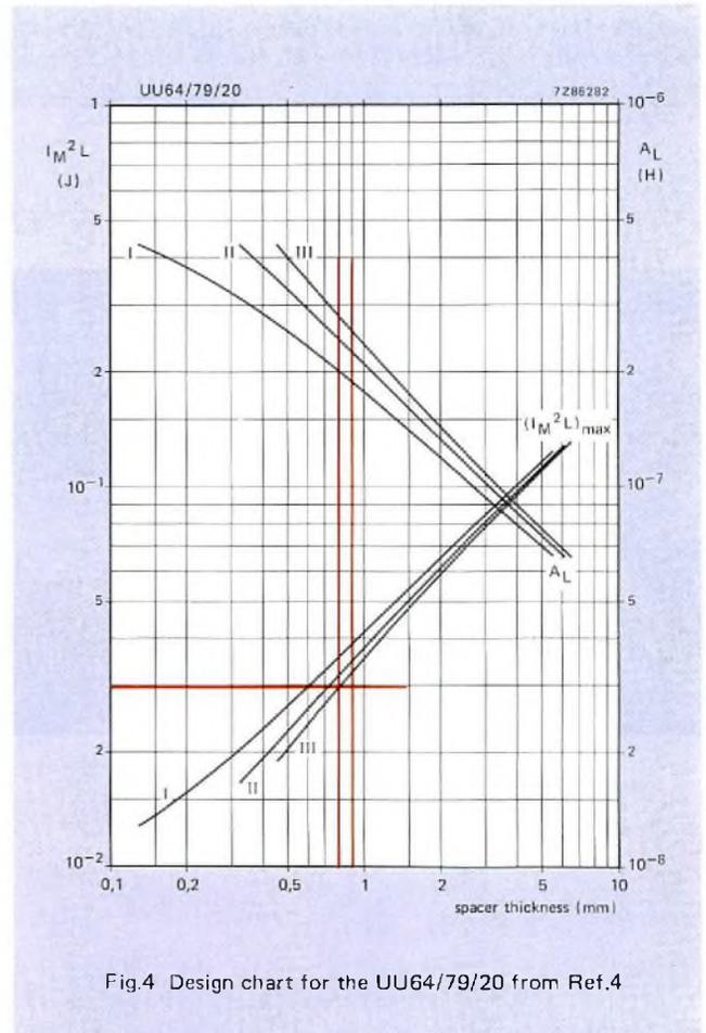
Fig.4 Design chart for the UU64/79/20 from Ref.4
