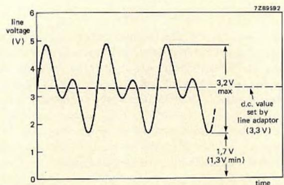
Fig.3 The output bias level is determined by the minimum voltage required by the integrated circuit and by the maximum amplitude of the dual-tone output
