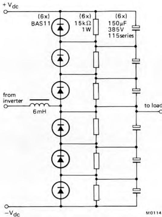
Fig.5 Single phase of L-section filter
