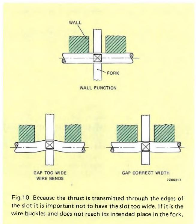
Fig.10 Because the thrust is transmitted through the edges of the slot it is important not to have the slot too wide. If it is the wire buckles and does not reach its intended place in the fork,
