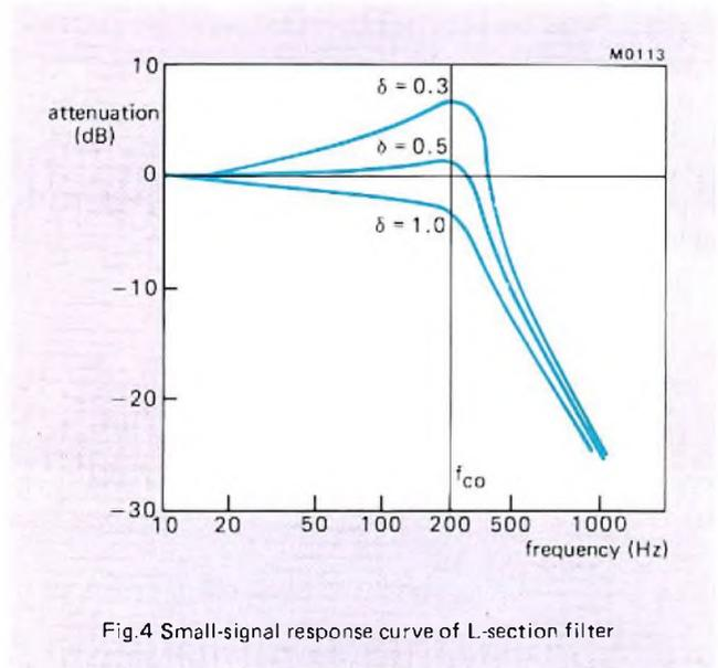
Fig.4 Small-signal response curve of L-section filter
