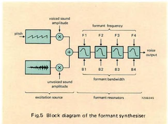
Fig.5 Block diagram of the formant synthesiser
