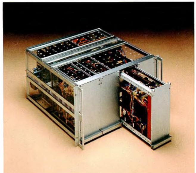
Fig.3a Laboratory prototype of PWM UPS, showing single phase of the three-phase inverter
