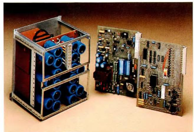
Fig.3b UPS lowpass filter (left), power supply module (centre), waveform generation module (right)
