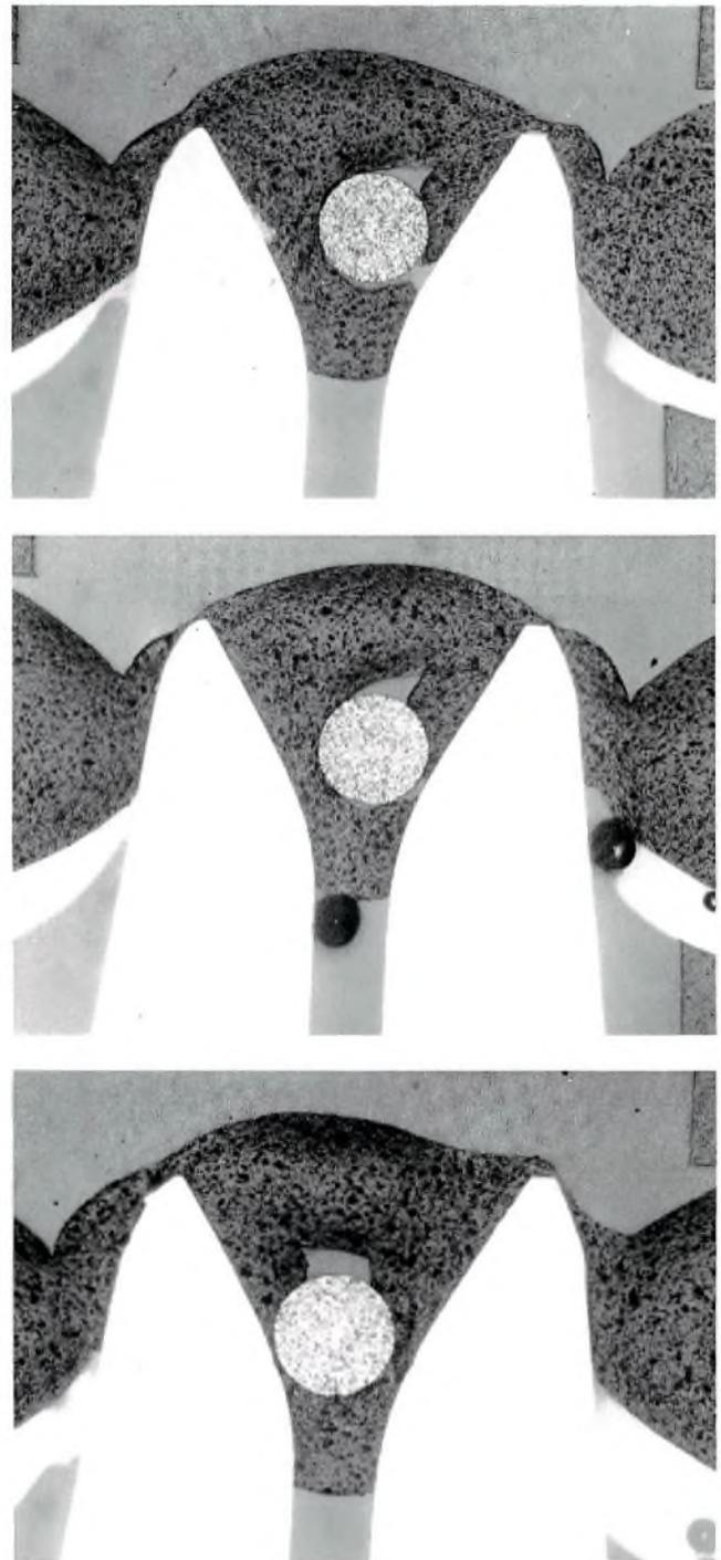
Fig.5 Micrograph showing how the inlet guides the wire into the contact fork. Magnification 50 X
