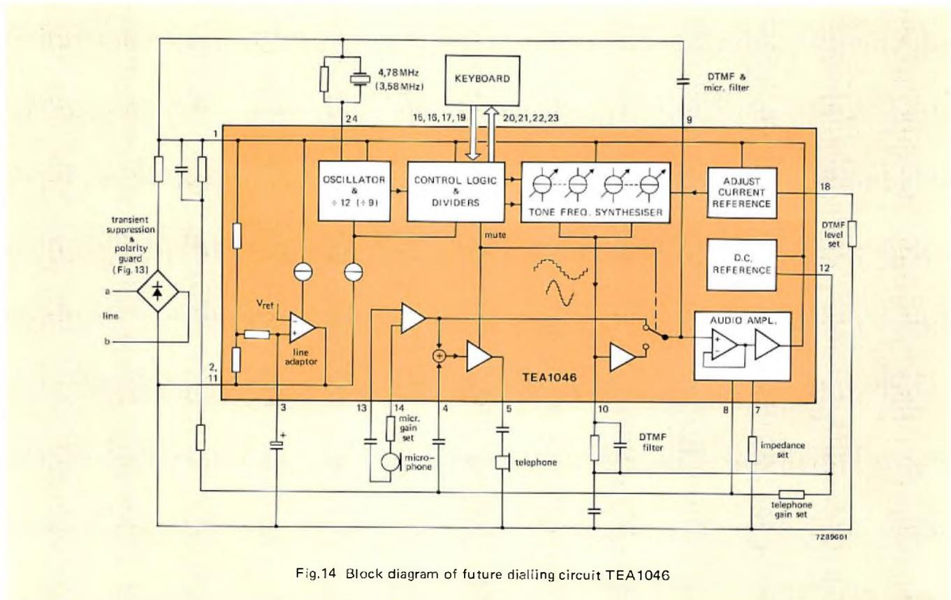
Fig.14 Block diagram of future dialling circuit TEA1046
