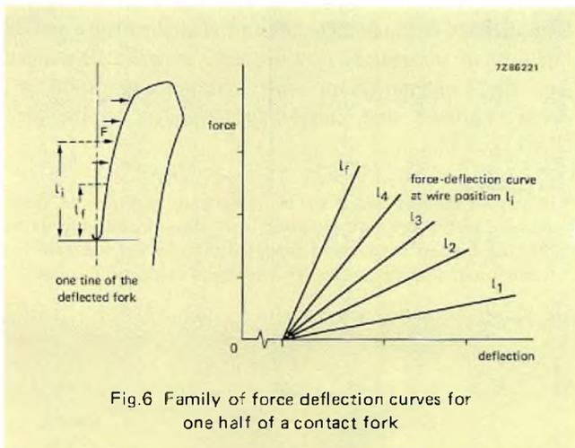
Fig.6 Family of force deflection curves for one half of a contact fork
