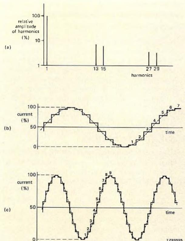
Fig.4 Form and frequency spectrum of the synthesised tones
