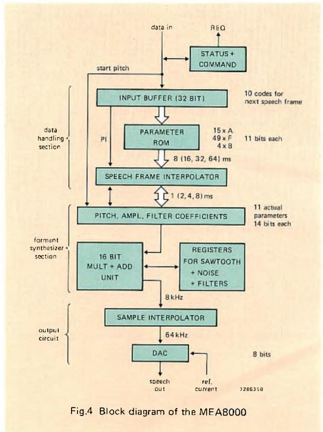
Fig.4 Block diagram of the MEA8000
