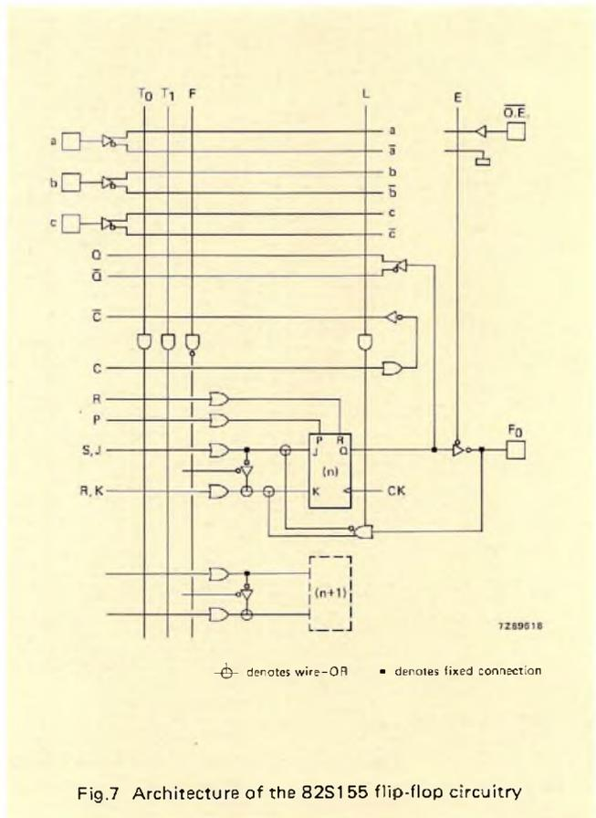
Fig.7 Architecture of the 82S155 flip-flop circuitry
