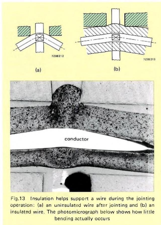
Fig.13 Insulation helps support a wire during the jointing operation: (a) an uninsulated wire after jointing and (b) an insulated wire. The photomicrograph below shows how little bending actually occurs
