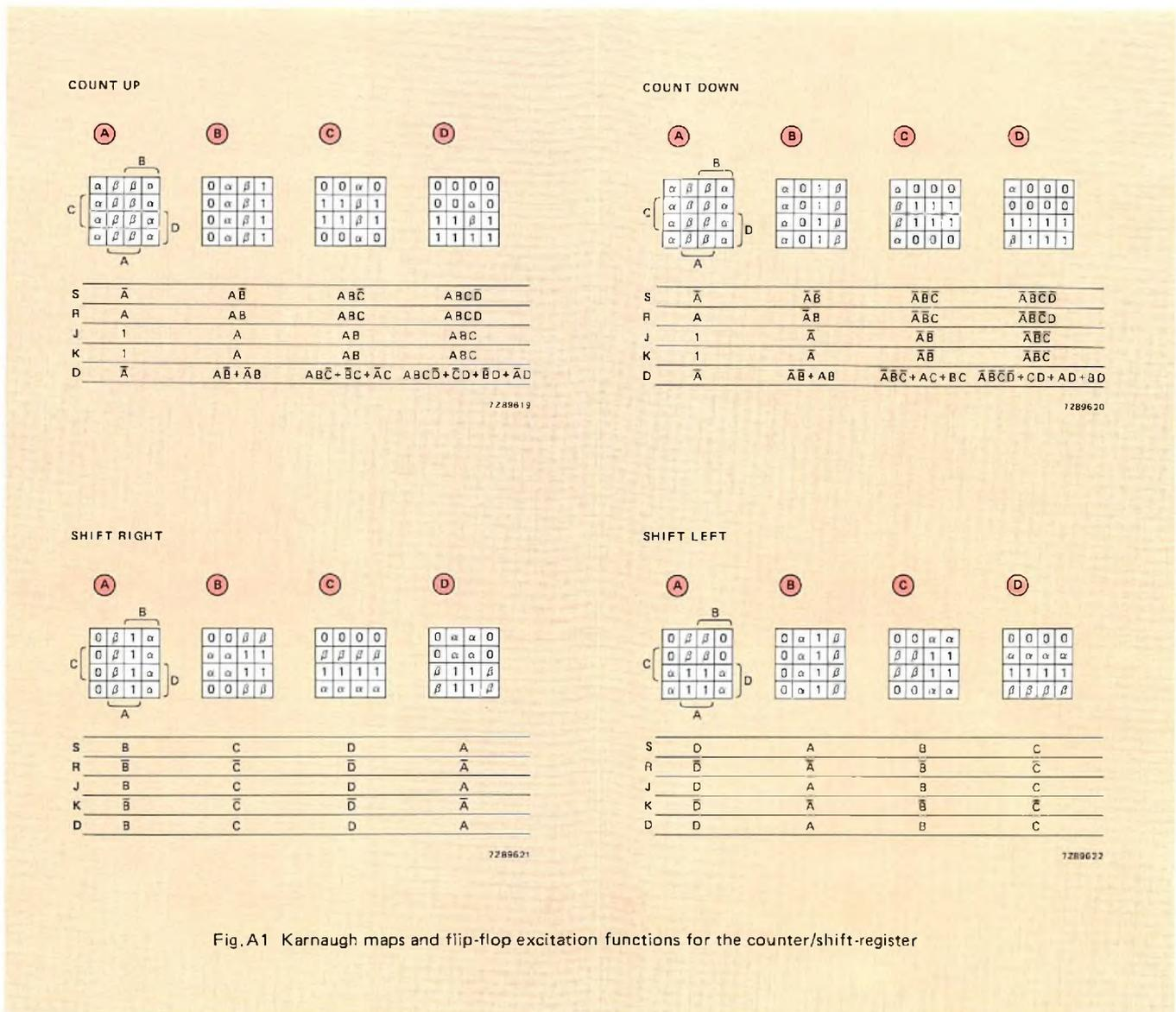
Fig. A1 Karnaugh maps and flip-flop excitation functions for the counter/shift-register
