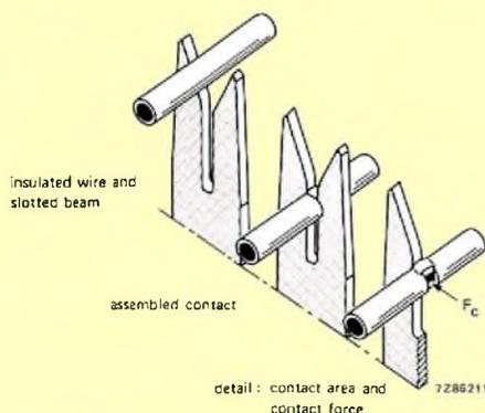
Fig.1 Principle of the ID connection. When a wire is forced between the tines of an ID fork the insulation is parted and the bare copper forces the tines apart
