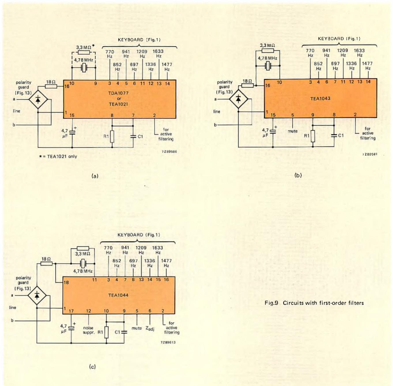
Fig.9 Circuits with first-order filters
