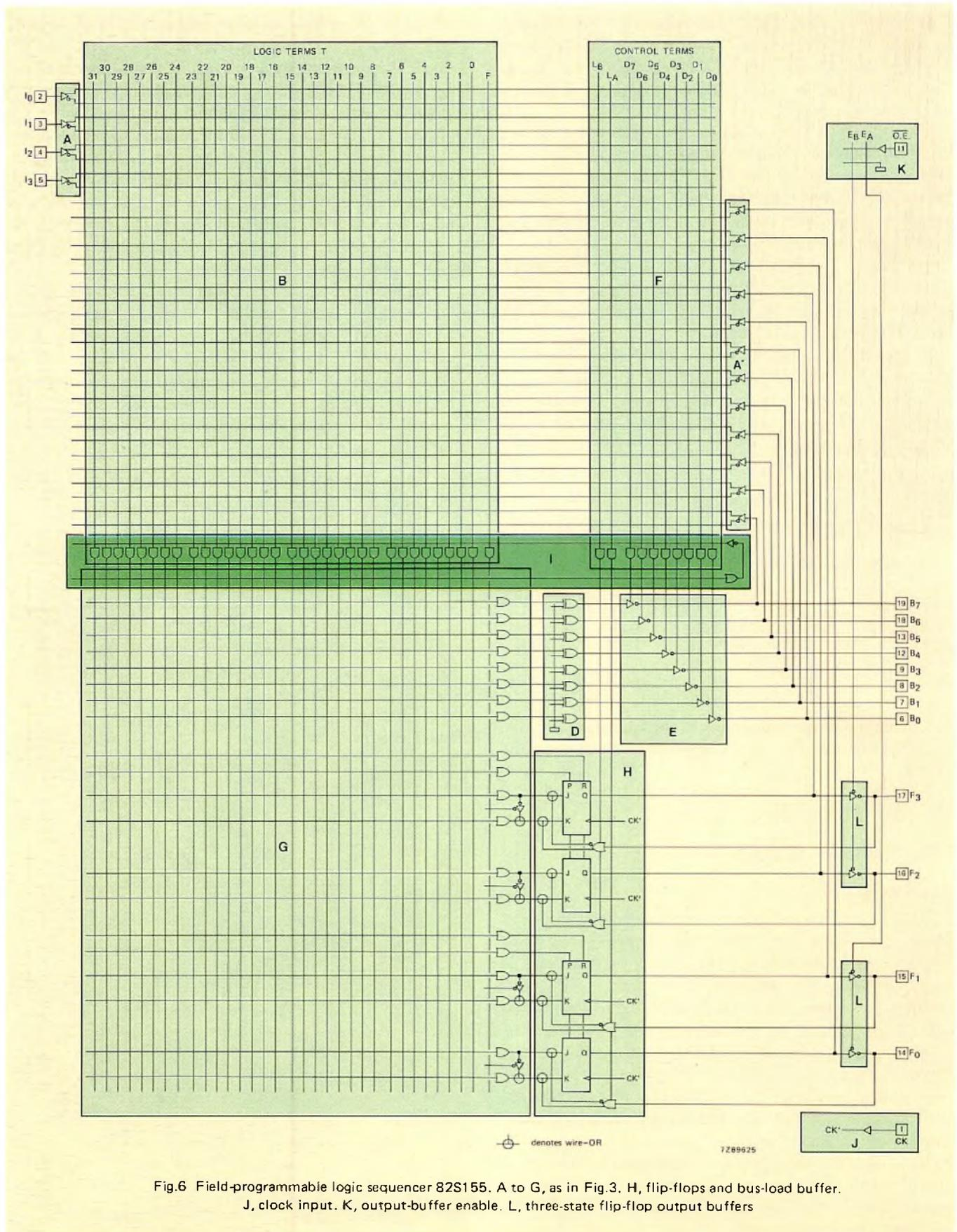
Fig.6 Field-programmable logic sequencer 82S155. A to G, as in Fig.3. H, flip-flops and bus-load buffer. J, clock input. K, output-buffer enable. L, three-state flip-flop output buffers
