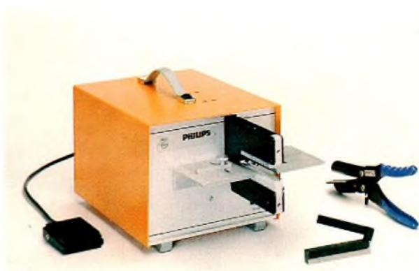
Fig.20 Manual and automatic tools used for making F303 ID connections
