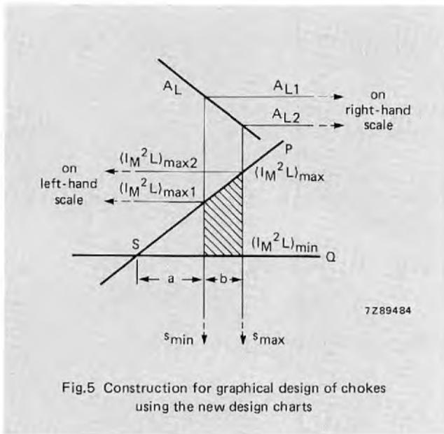
Fig.5 Construction for graphical design of chokes using the new design charts
