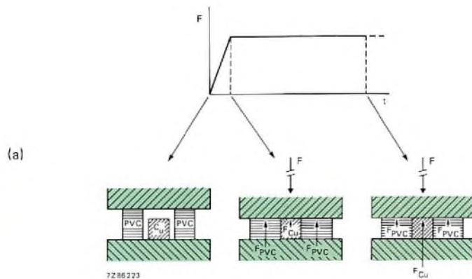
Fig.17 The stress strain relationship in PVC is dependent on temperature and time
