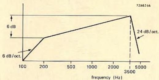
Fig.16 Output filter transfer characteristic for obtaining optimum voice quality
