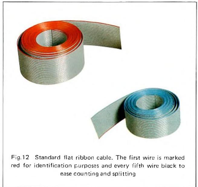
Fig.12 Standard flat ribbon cable. The first wire is marked red for identification purposes and every fifth wire black to ease counting and splitting
