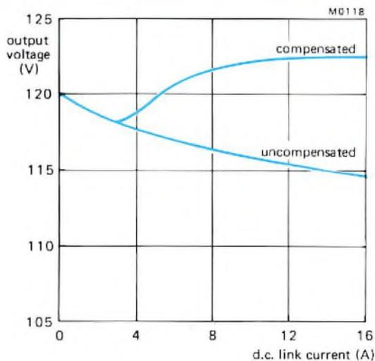
Fig.11 Output voltage versus d.c. link current
