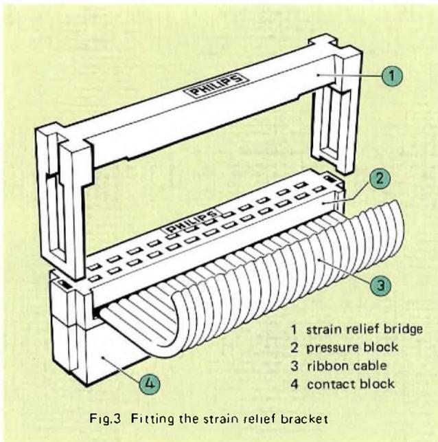
Fig.3 Fitting the strain relief bracket
