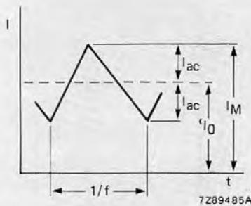
Fig.1 Symbols for choke current used in the text. (See also the Table)
