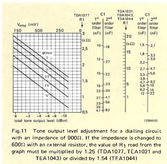
Fig.11 Tone output level adjustment for a dialling circuit with an impedance of 900Ω. If the impedance is changed to 600Ω with an external resistor, the value of R<sub>1</sub> read from the graph must be multiplied by 1.25 (TDA1077, TEA1021 and TEA1043) or divided by 1.54 (TEA1044)
