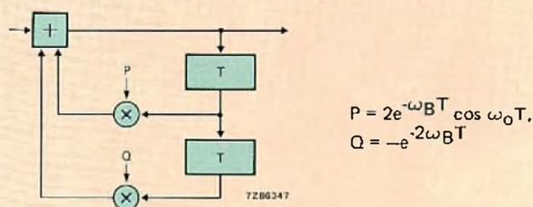
Fig.7 Two-multiplier resonator
