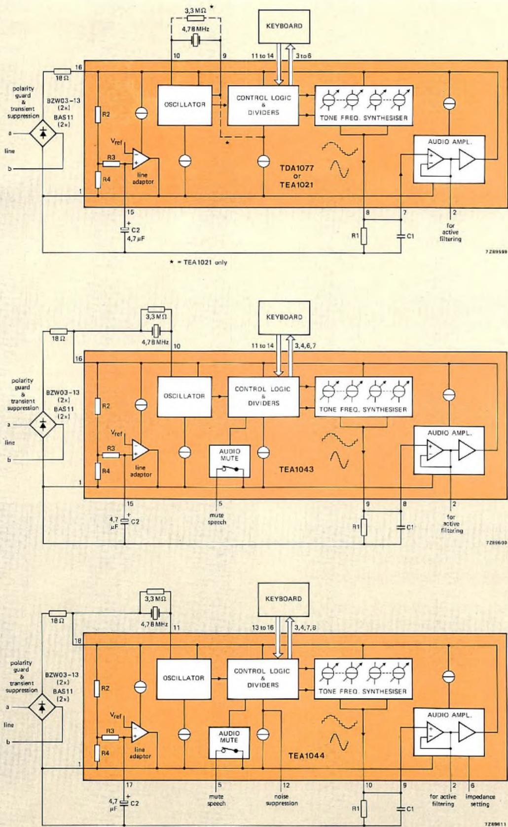
Fig.2 Block diagrams of the dialling circuits
