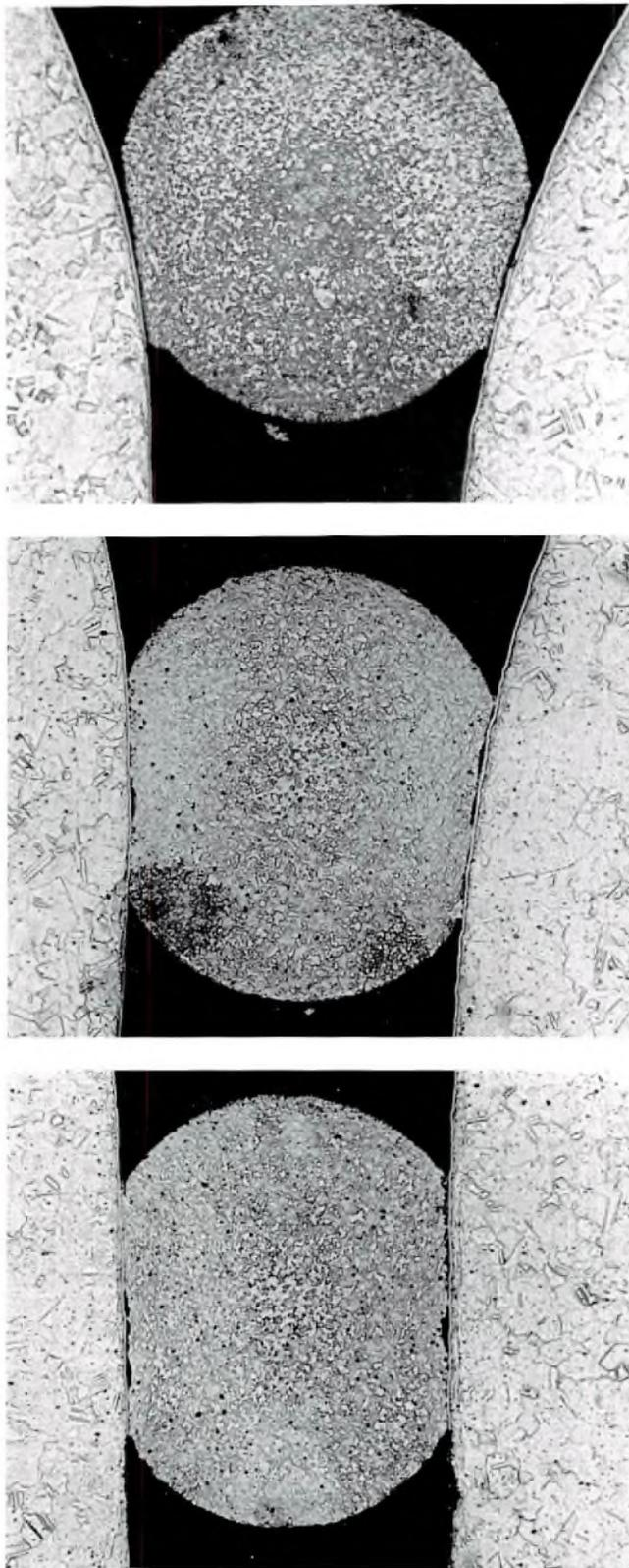
Fig.9 Three stages in forming the ID connection. At a magnification of 200 times one can see the importance of the shape of the inlet slot. In the lowest view the wire is fully deformed but has not yet reached its final position
