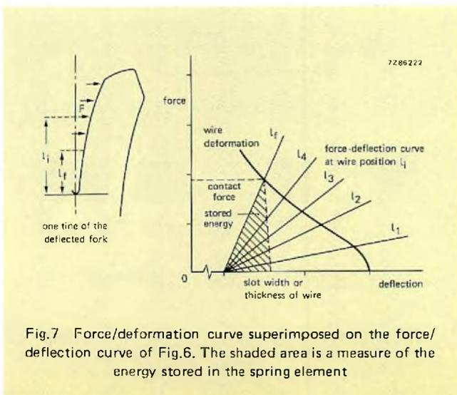
Fig.7 Force/deformation curve superimposed on the force/deflection curve of Fig.6. The shaded area is a measure of the energy stored in the spring element
