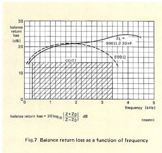
Fig.7 Balance return loss as a function of frequency
