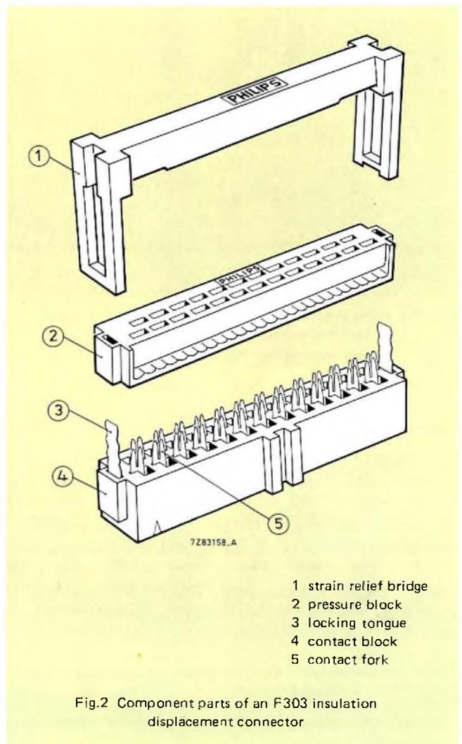
Fig.2 Component parts of an F303 insulation displacement connector
