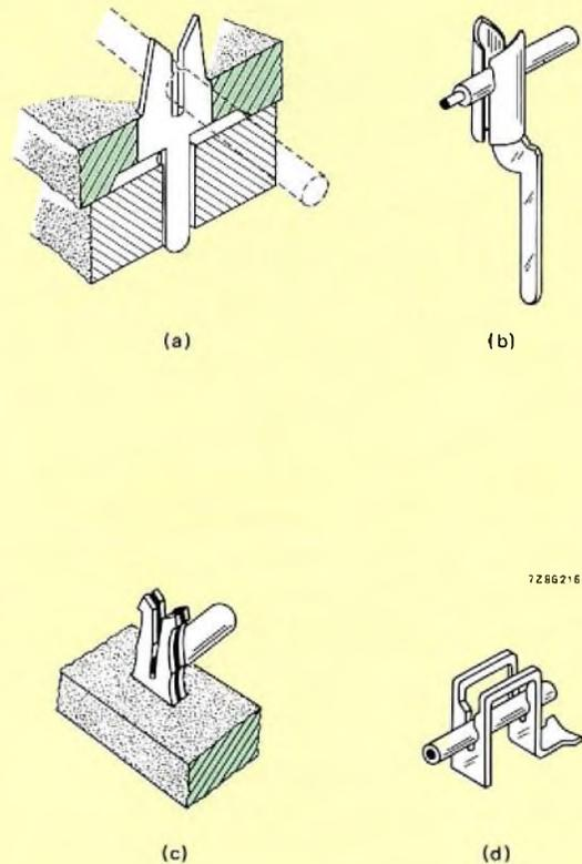
Fig.15 Four common types of contact fork. The double fork contacts shown in (b), (c) and (d) seem to offer greater security but this is far from being the case. When the mechanisms involved are fully analysed it is seen that a properly designed and manufactured single fork contact achieves minimum contact resistance, maintains it indefinitely and does not suffer the drawbacks associated with being mechanically coupled to another system
