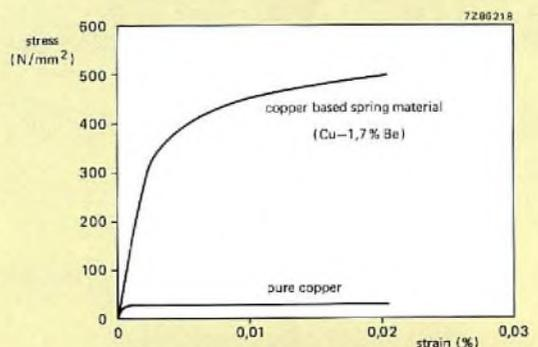
Fig.8 Stress/strain relationship for copper and beryllium copper. Just the addition of 1.7% beryllium transforms copper into an excellent spring material
