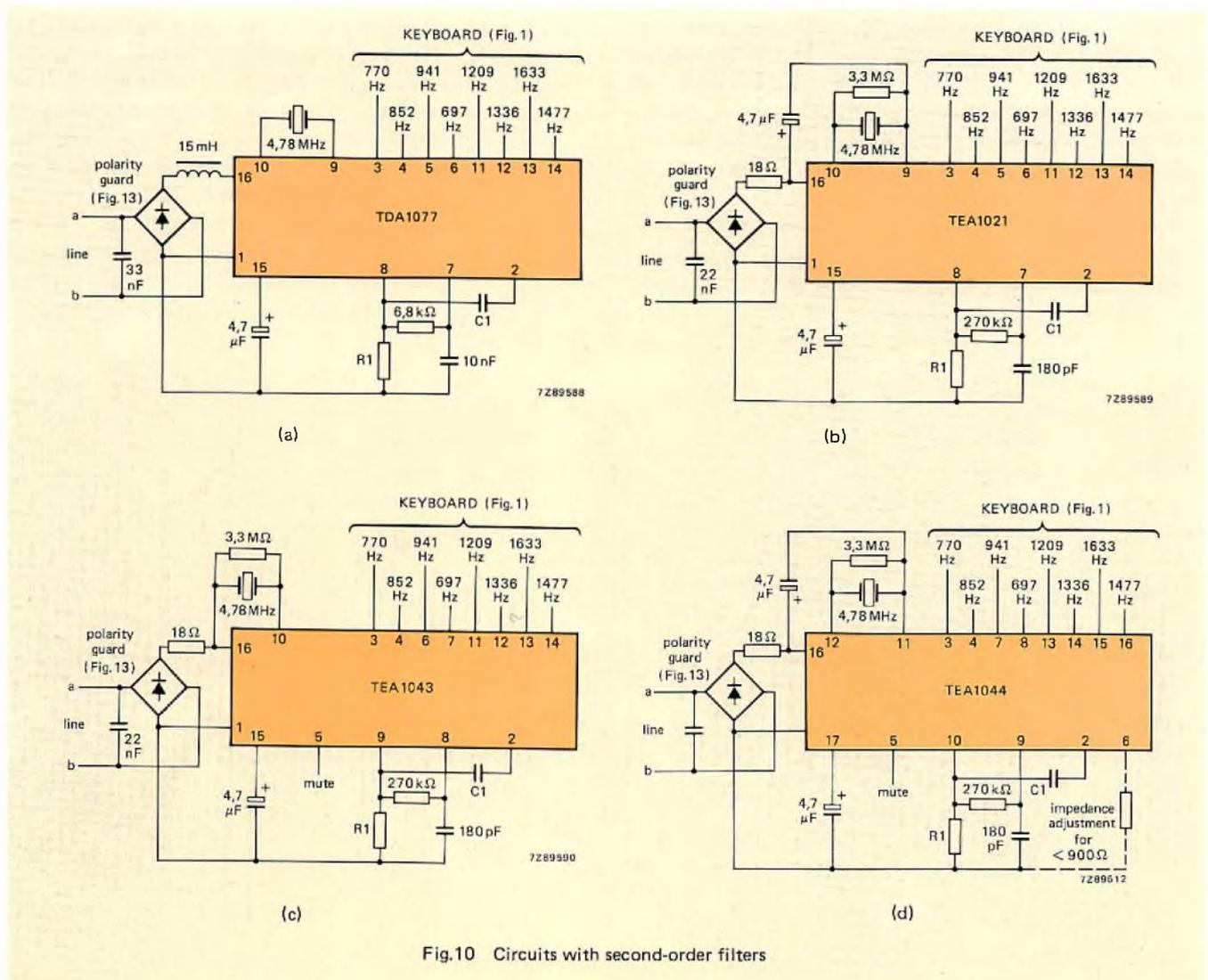
Fig.10 Circuits with second-order filters
