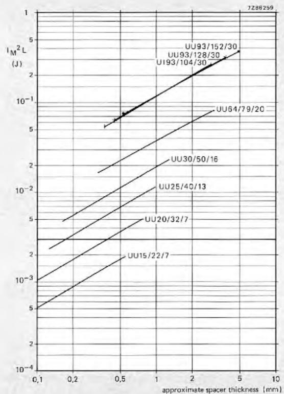
Fig.2 Selection chart for U cores as given in Ref.4
