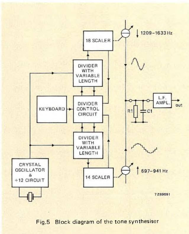
Fig.5 Block diagram of the tone synthesiser
