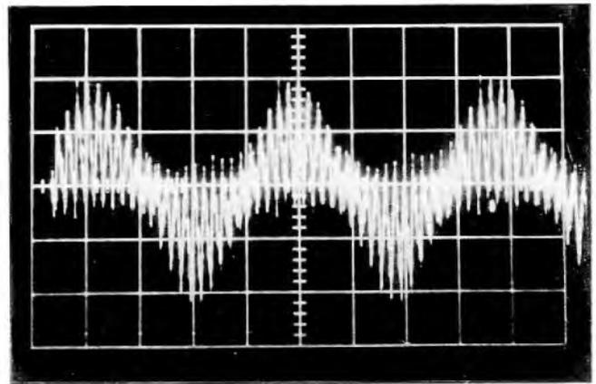
Fig.7 Lowpass filter capacitor ripple current waveform
