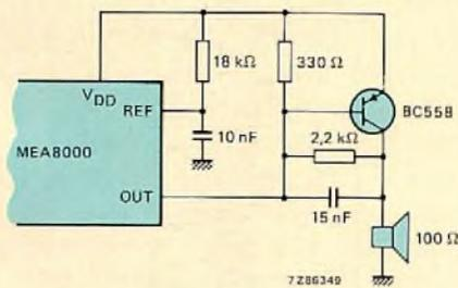
Fig.15 Simple audio output stage
