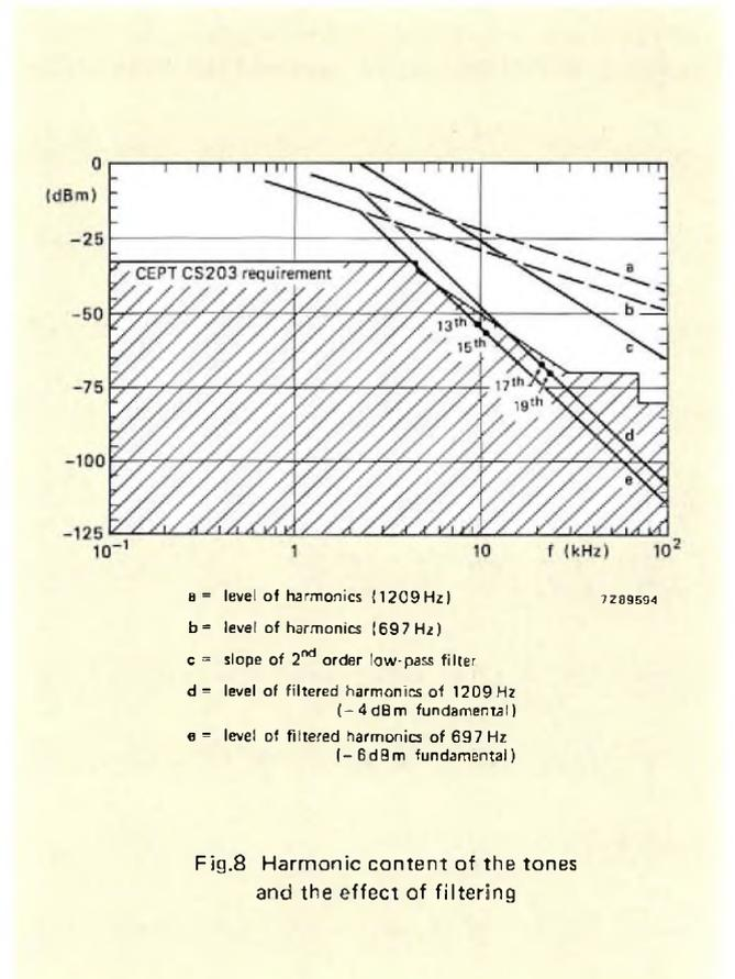
Fig.8 Harmonic content of the tones and the effect of filtering
