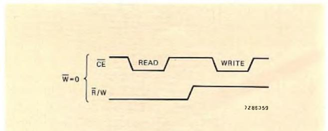
Fig.11 Chip enable (CE) used as a read or write strobe
