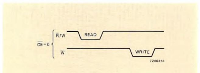
Fig.12 Separate read and write strobes
