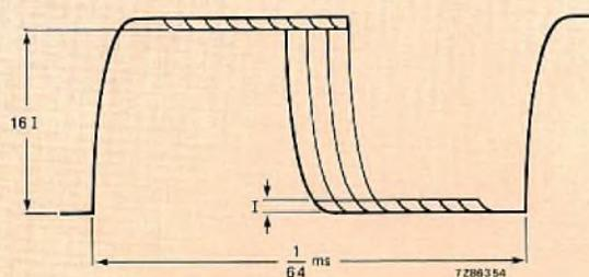
Fig.9 Superimposed output pulses from the DAC
