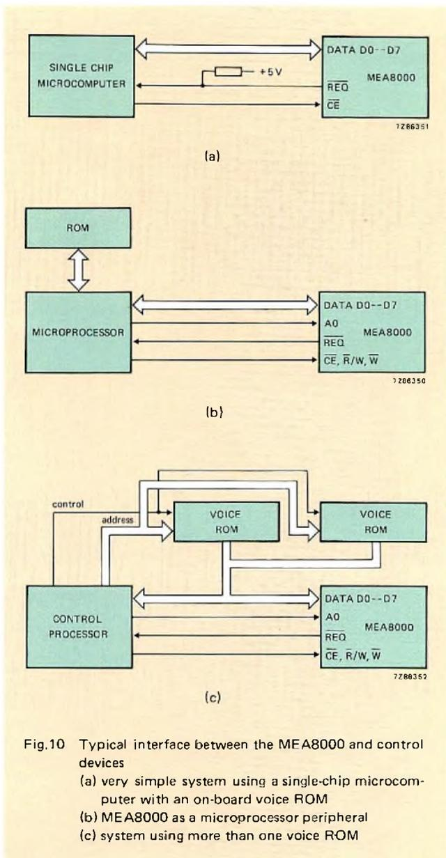
Fig.10 Typical interface between the MEA8000 and control devices
