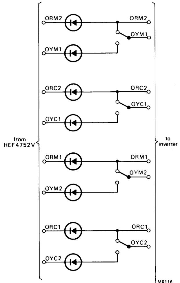
Fig.9 Three-phase to single-phase conversion; switch shown in single-phase position
