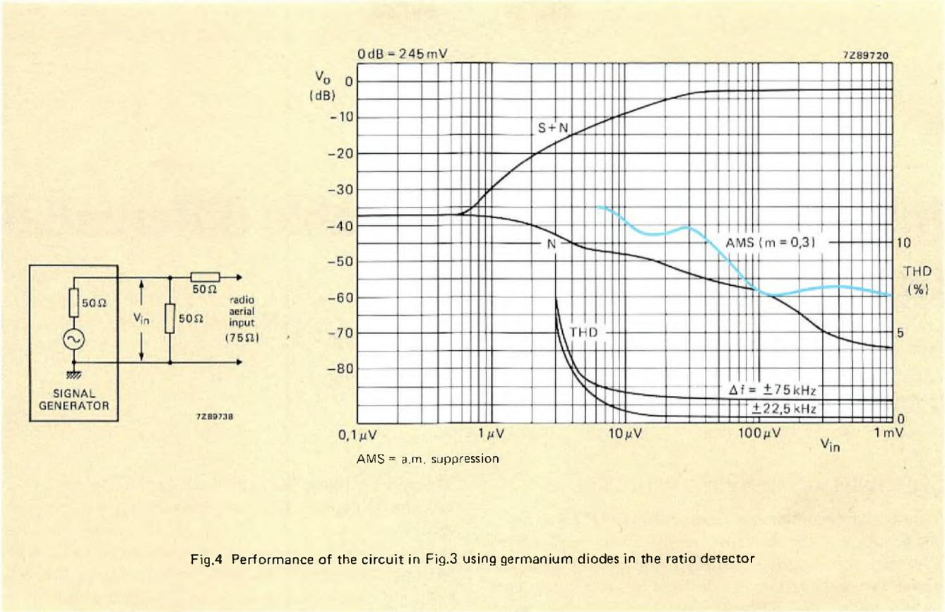
Fig.4 Performance of the circuit in Fig.3 using germanium diodes in the ratio detector
