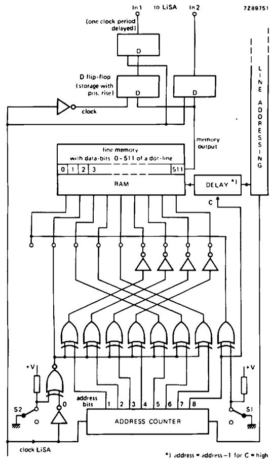
Fig.15 Practical data encoding circuit. For direct or reversed imaging of the LiSA dot pattern, S1 exchanges right and left shift registers, and S2 exchanges upper cell bank with lower
