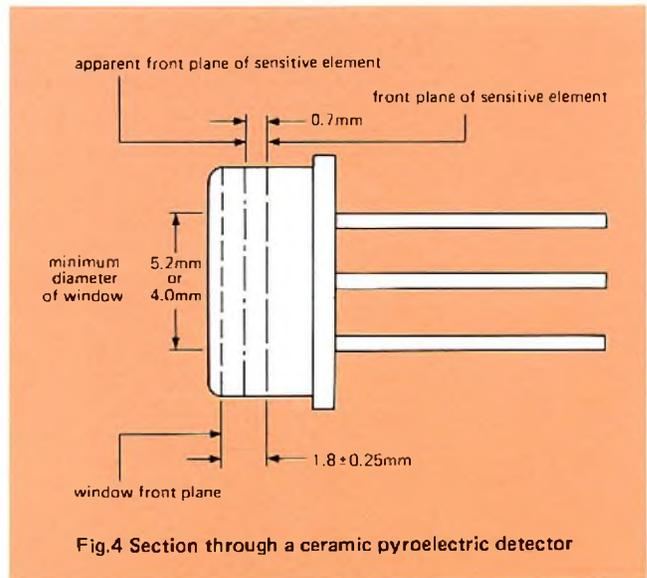
Fig.4 Section through a ceramic pyroelectric detector
