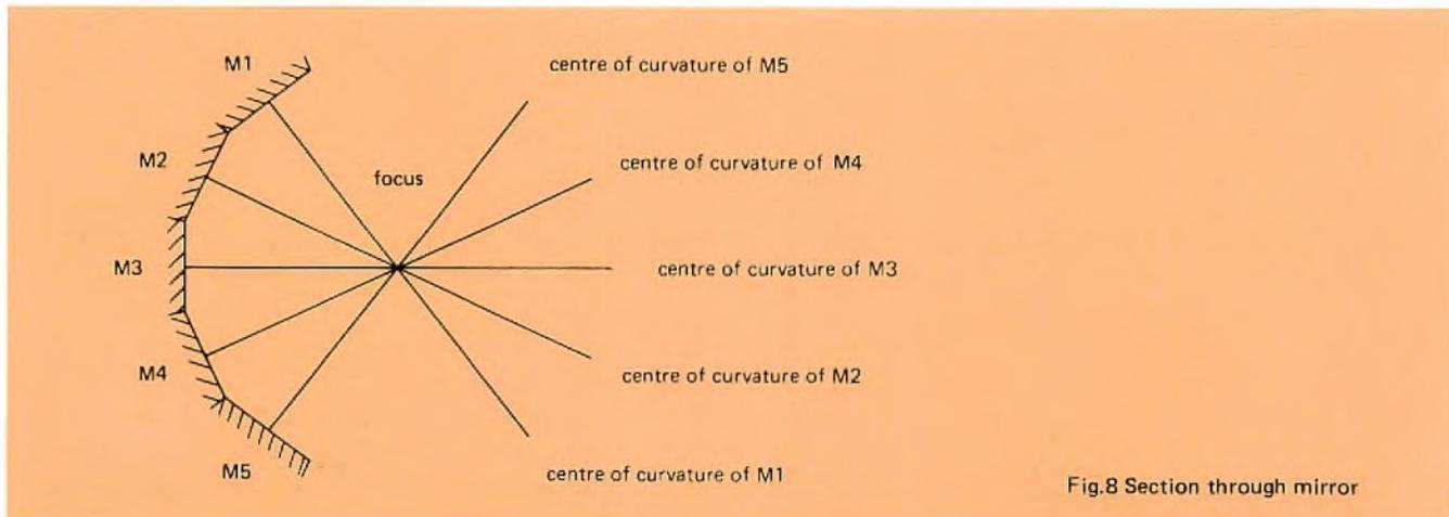
Fig.8 Section through mirror
