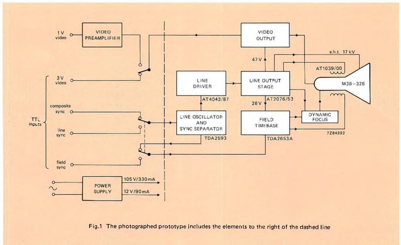
Fig.1 The photographed prototype includes the elements to the right of the dashed line
