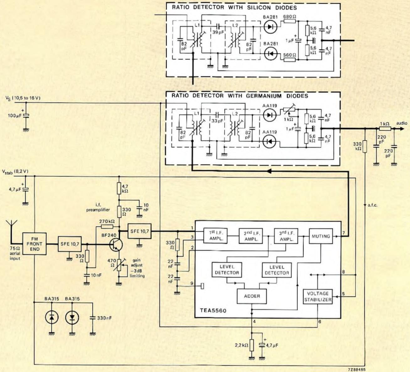
Fig.3 Small signal section of an f.m. radio using integrated f.m. i.f. system TEA5560 and a ratio detector with germanium or silicon diodes
