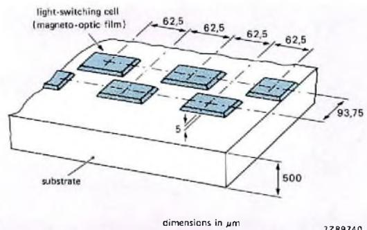
Fig.2 The LiSA chip consists of a bismuth iron garnet film, grown epitaxially on a substituted gadolinium gallium garnet substrate and etched into separate light switching cells. Each cell is 65 × 65 μm<sup>2</sup>, smaller than the smallest possible magnetic domain (about 100 to 200 μm diameter). An opaque metallic film covers the space between the cells
