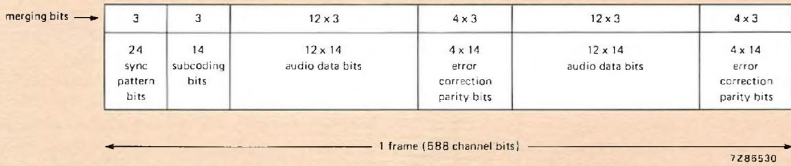
Fig.4 Data stream after Eight-to-Fourteen Modulation (EFM)
