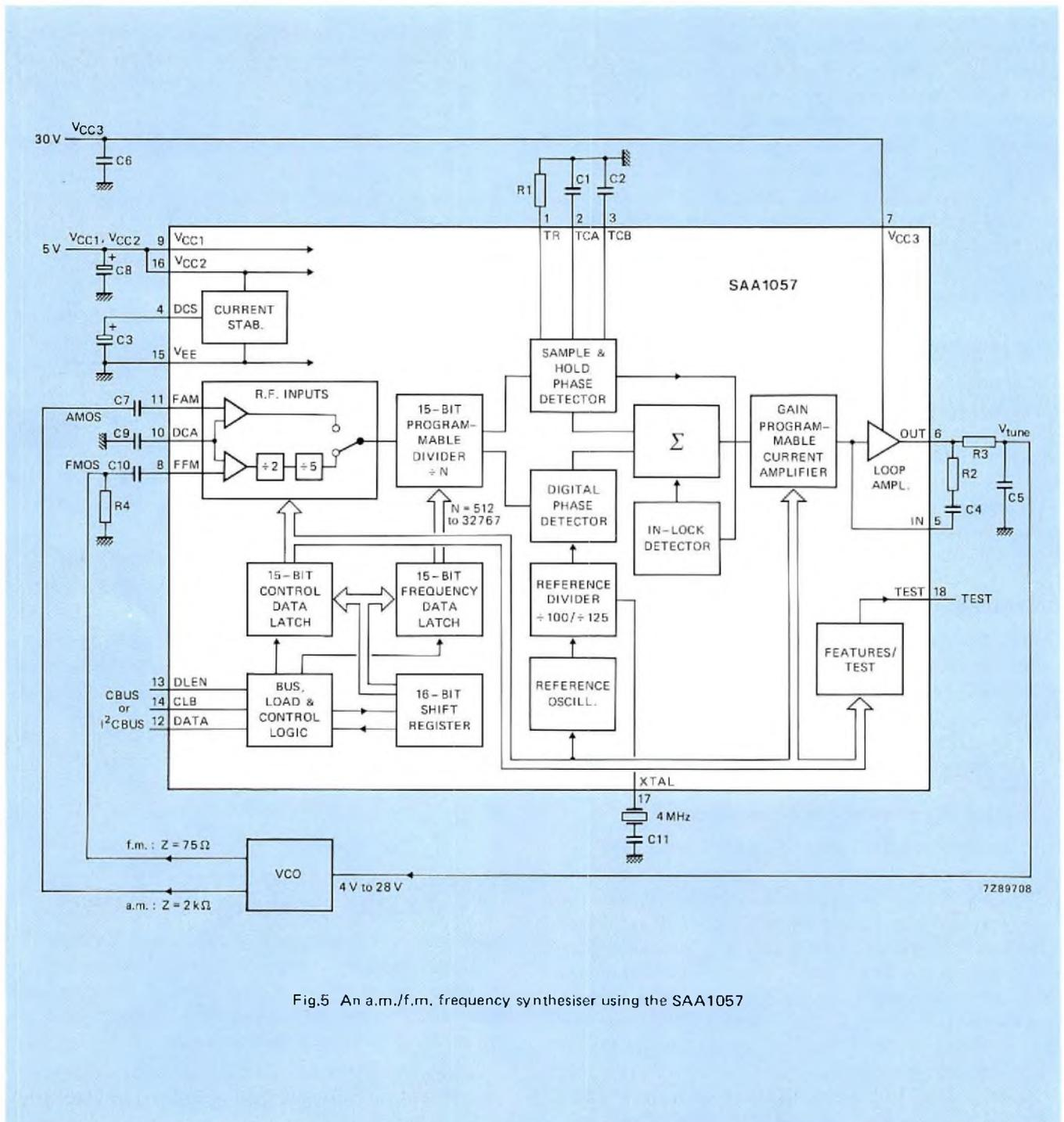
Fig.5 An a.m./f.m. frequency synthesiser using the SAA1057
