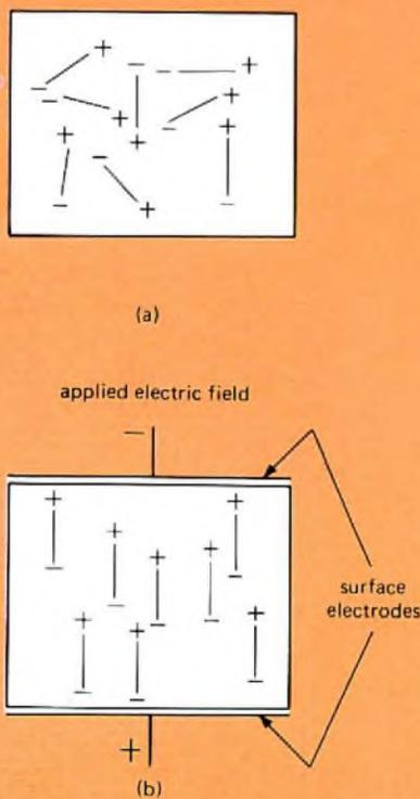
Fig.5 —Orientation of electric dipoles
