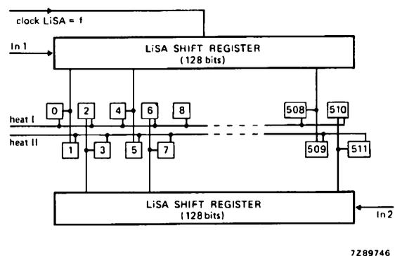
Fig.12 LiSA 512 switching cell layout and signal input
