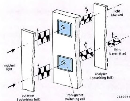
Fig.3 In combination with an optical polariser and analyser, the iron garnet cells act as light valves controlled by the direction of magnetisation
