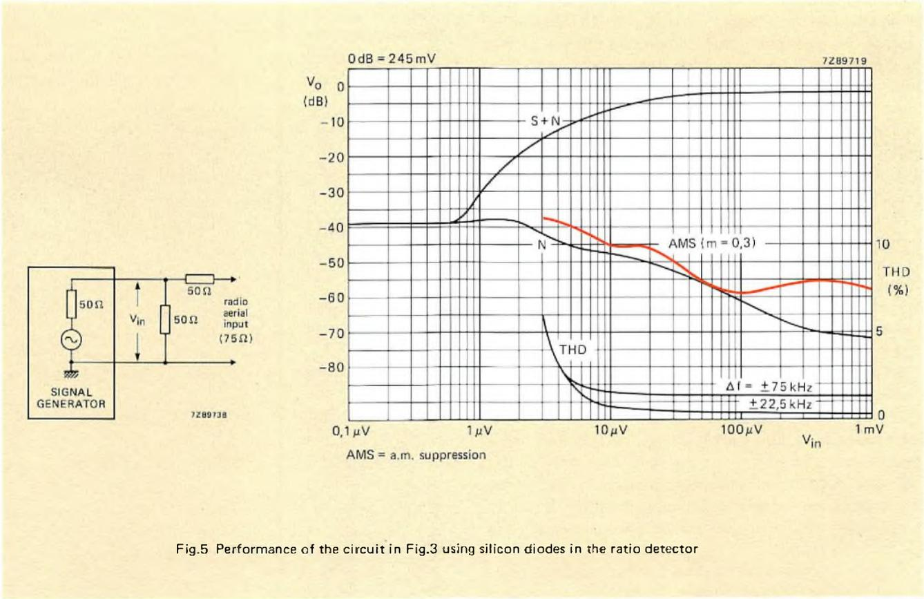
Fig.5 Performance of the circuit in Fig.3 using silicon diodes in the ratio detector
