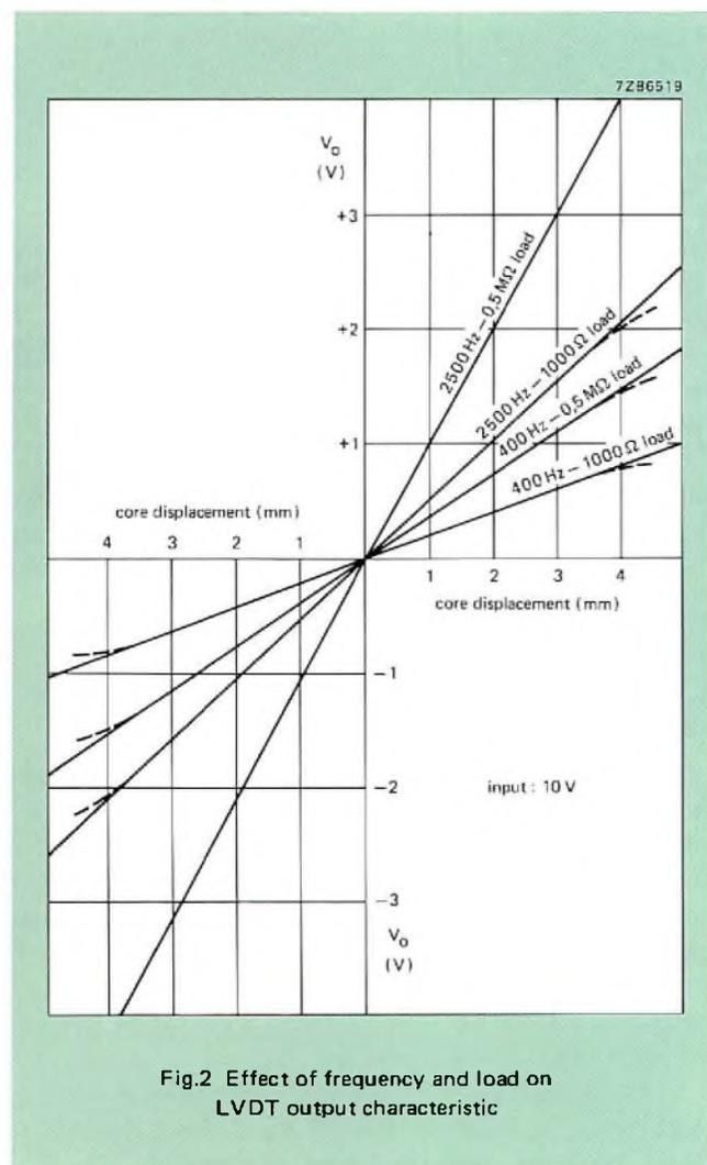
Fig.2 Effect of frequency and load on LVDT output characteristic
