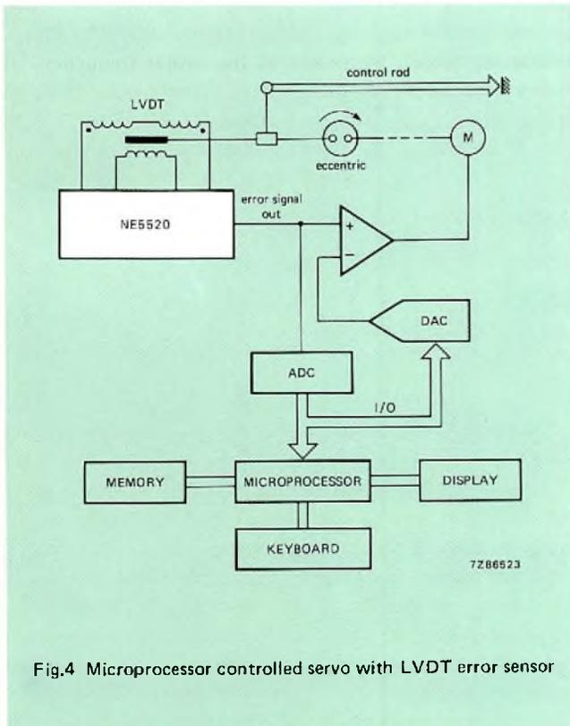
Fig.4 Microprocessor controlled servo with LVDT error sensor
