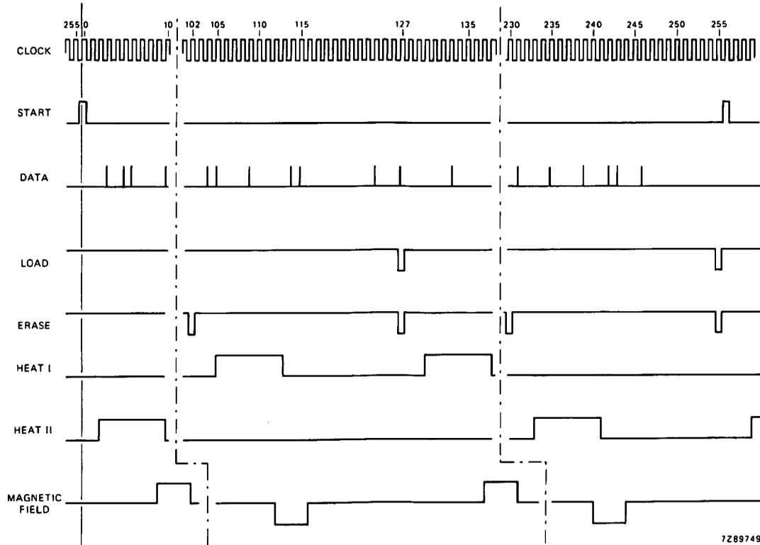
Fig.11 Pulse sequence for the LiSA 512 unit. Data input frequency 500 kbits/s
