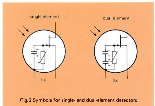
Fig.2 Symbols for single- and dual-element detectors
