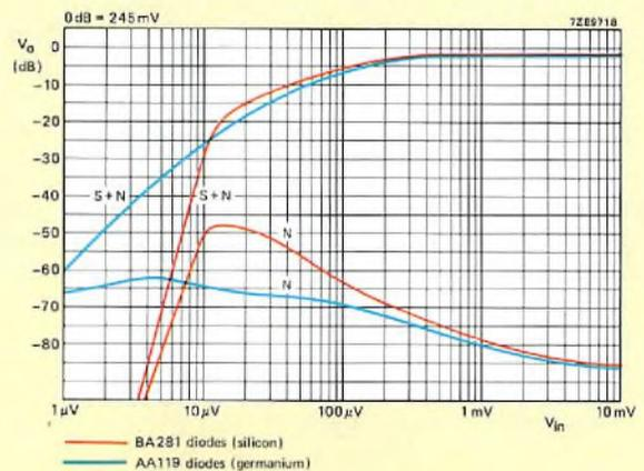
Fig.2 Signal-to-noise curves for the circuit of Fig.1 using germanium or silicon diodes in the ratio detector
