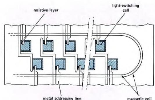
Fig.4 Basic setup for switching the cells. A thin film resistive layer on top of each cell supplies a heat pulse, heating the cell corner to about 100 °C. This sets up a region of magnetic instability, and the cell's magnetisation can then be reversed by an external magnetic field
