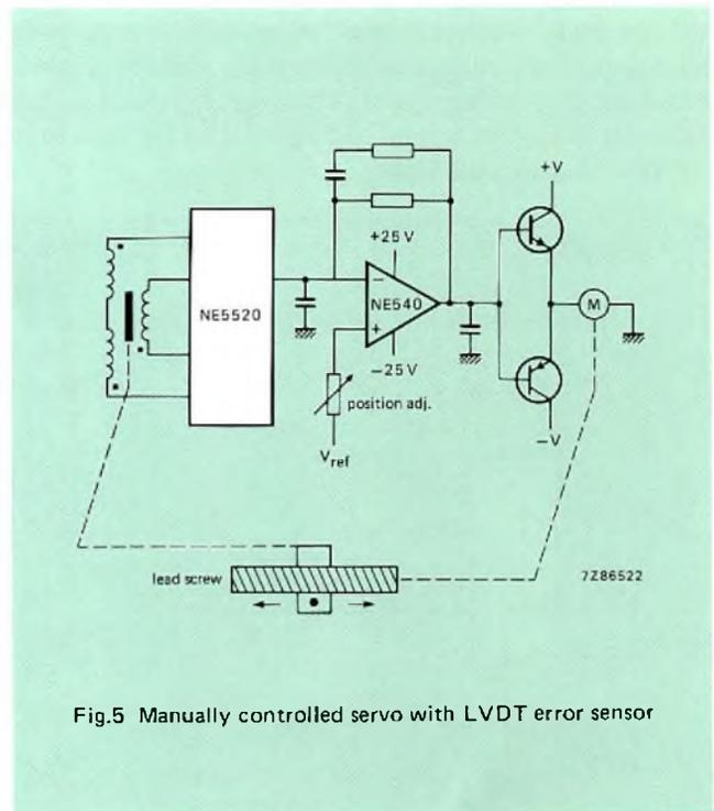
Fig.5 Manually controlled servo with LVDT error sensor
