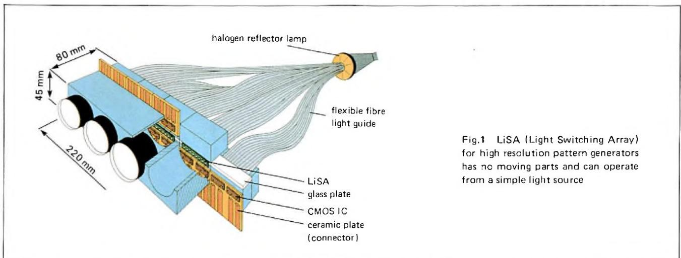
Fig.1 LiSA (Light Switching Array) for high resolution pattern generators has no moving parts and can operate from a simple light source
