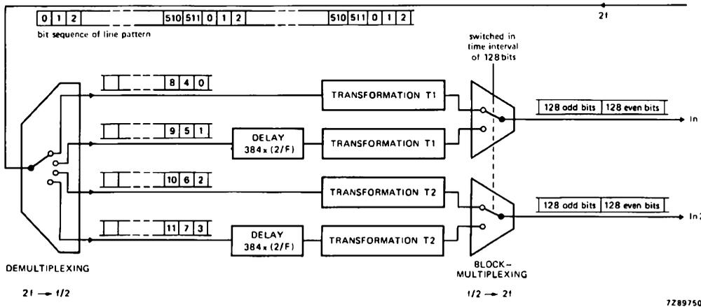
Fig.13 Encoding the serially arranged data for supply to the LiSA 512 unit
