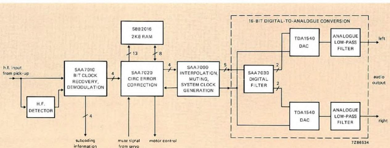
Fig.5 Block diagram of a Compact Disc decoder
