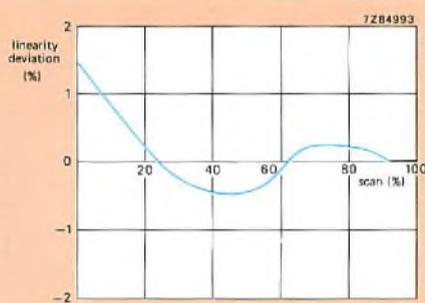
Fig.4 Line-scan linearity
