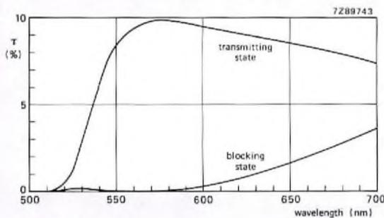
Fig.6 Transmission coefficient ( $\tau$ ) of a LiSA unit as a function of wavelength (with the polariser and analyser inclined at  $15^\circ$  to each other)
