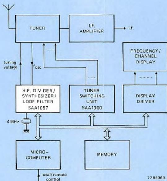
Fig. 2 Integrated circuits for tuning systems using SAA1057.
