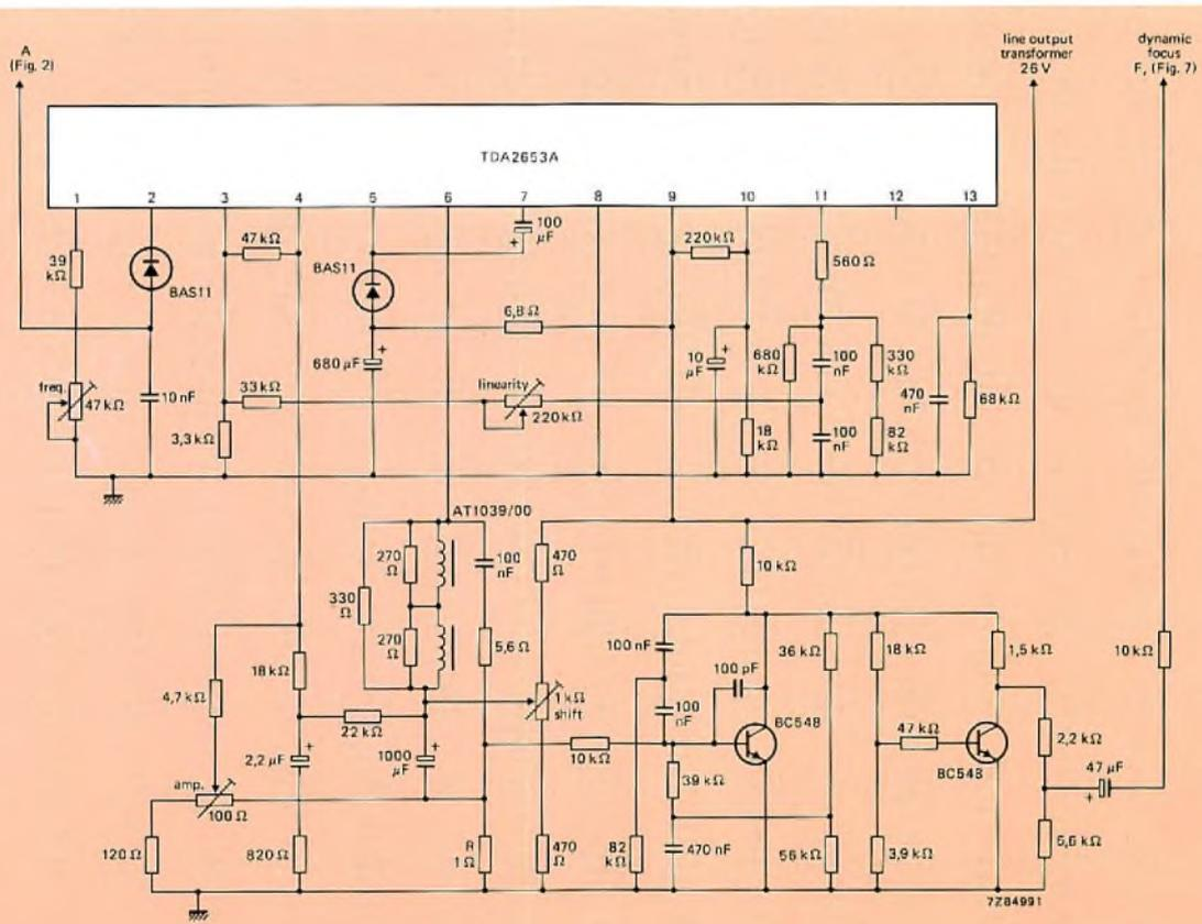
Fig.5 Field timebase and wave-shaping circuit
