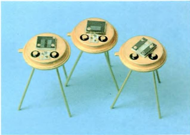
Fig.3 Detector interiors: top RPY86/87 single-element detector, bottom left RPY93 dual-element detector, bottom right RPY94/95 dual-element detector.
