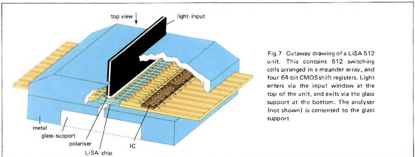
Fig.7 Cutaway drawing of a LiSA 512 unit. This contains 512 switching cells arranged in a meander array, and four 64-bit CMOS shift registers. Light enters via the input window at the top of the unit, and exits via the glass support at the bottom. The analyser (not shown) is cemented to the glass support
