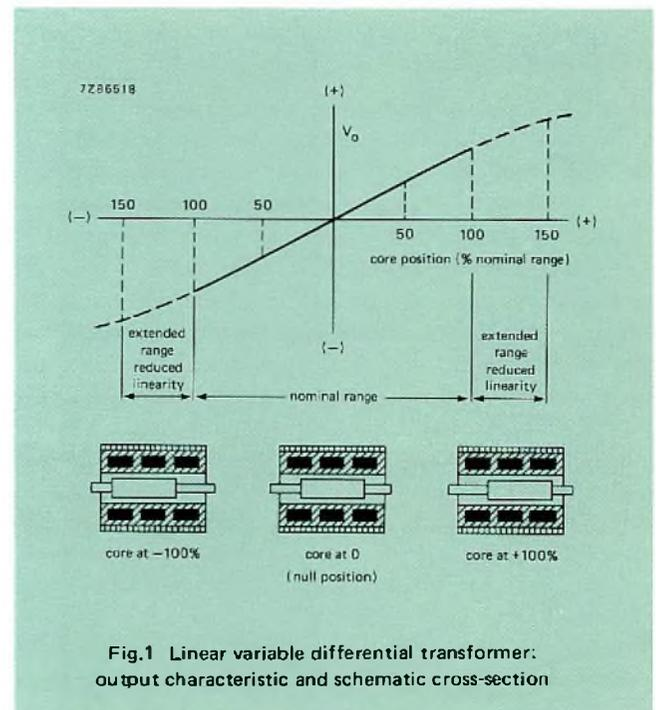
**Fig.1 Linear variable differential transformer: output characteristic and schematic cross-section**
