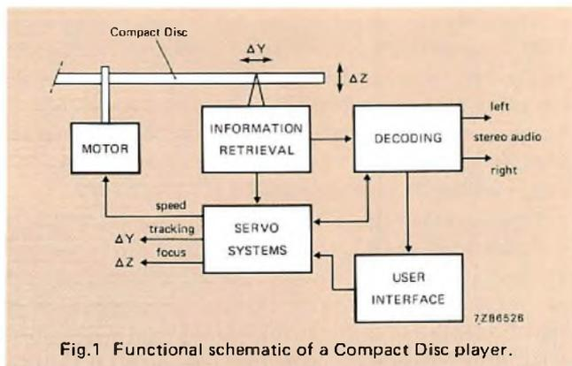
Fig.1 Functional schematic of a Compact Disc player.
