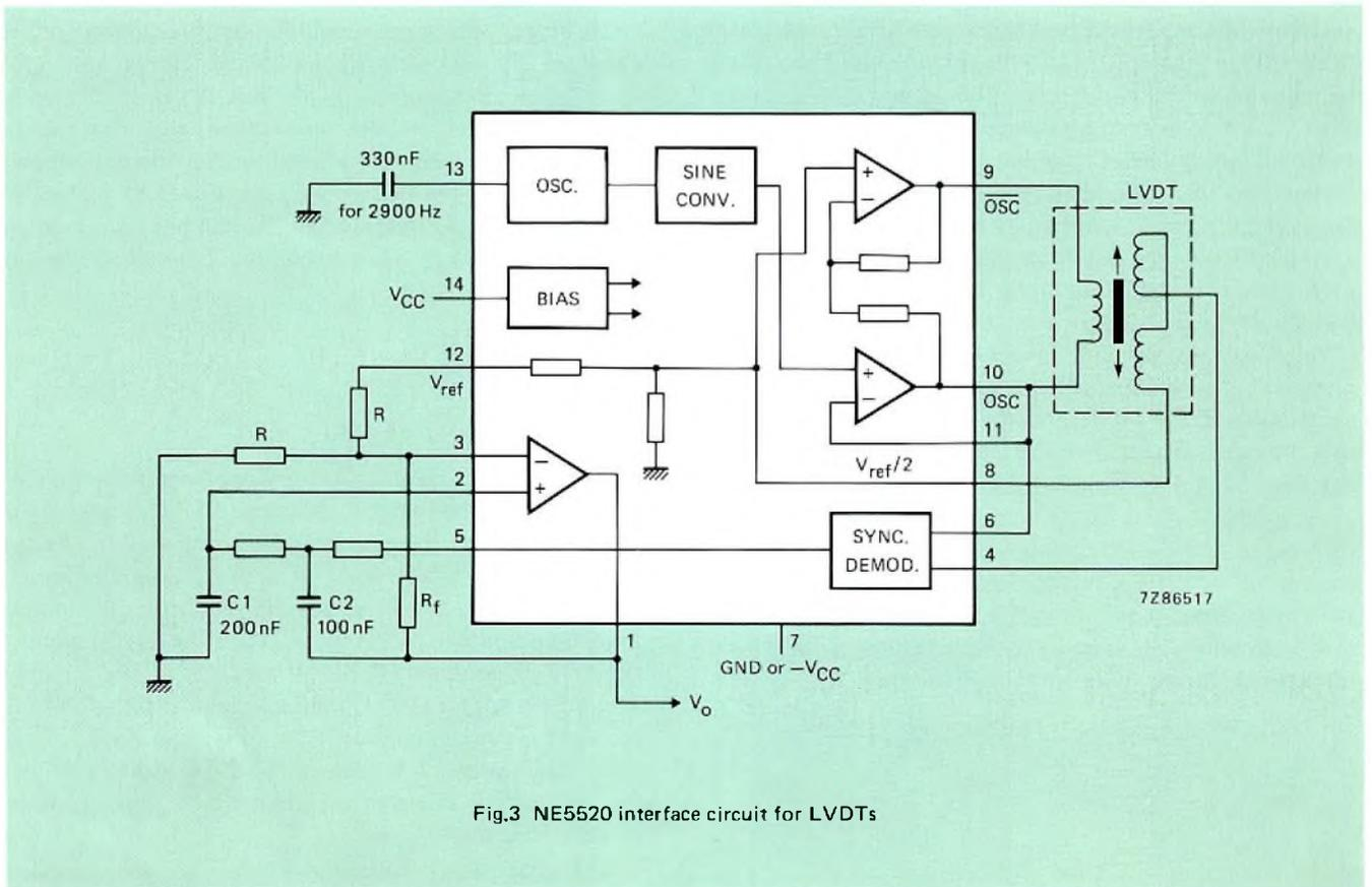
Fig.3 NE5520 interface circuit for LVDTs
