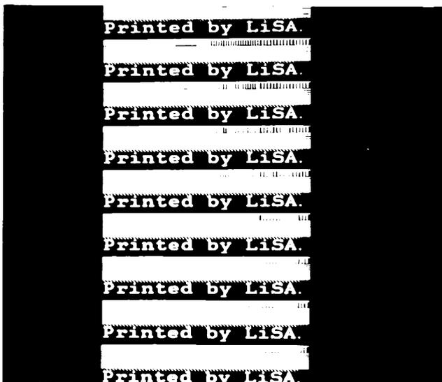
Fig.8 Pattern generated by a single (experimental) LiSA unit generating 12 dots/mm
