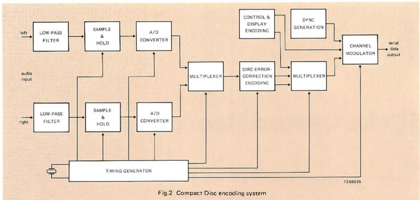
Fig.2 Compact Disc encoding system
