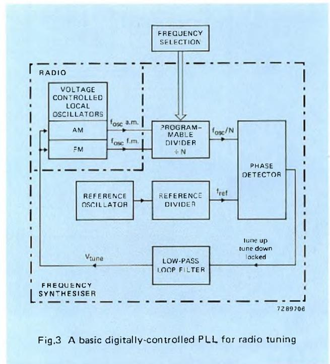
Fig.3 A basic digitally-controlled PLL for radio tuning
