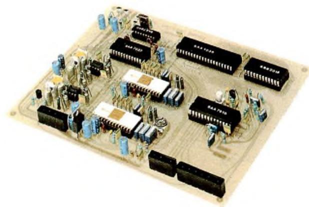
Development decoder board which performs more than 4 million decoding, control and error-correction operations every second of playback of a Compact Disc. The four new NMOS LSI circuits at the heart of this mammoth processing task enable a complete decoder controlled by one master clock to be assembled on one small single-sided board ( $\approx 220 \text{ cm}^2$ )
