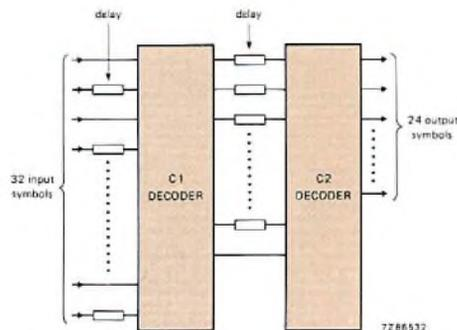
Fig.7 Principle of a CIRC decoder
