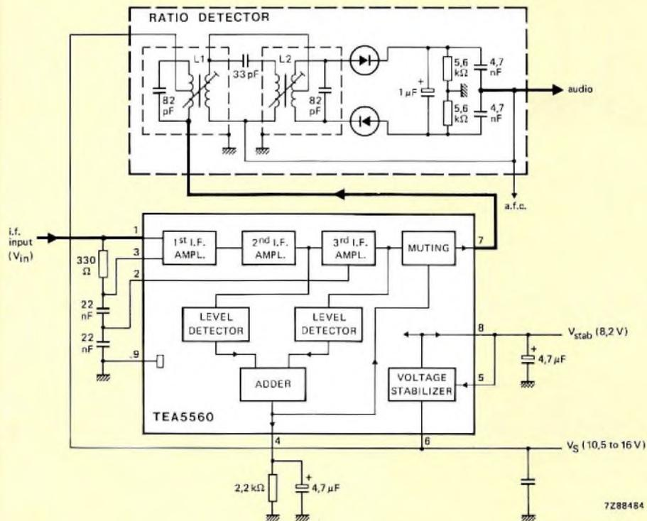
Fig.1 Ratio detector with integrated f.m. i.f. system TEA5560
