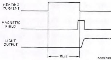
Fig.5 Pulse sequence for cell switching
