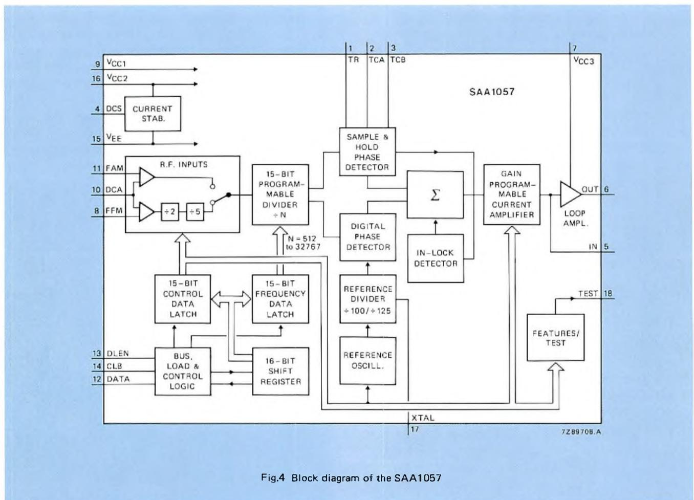
Fig.4 Block diagram of the SAA1057
