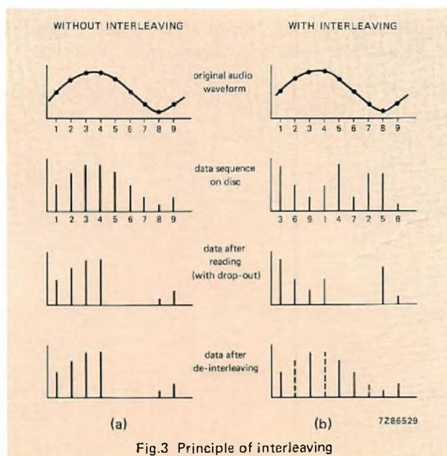
Fig.3 Principle of interleaving
