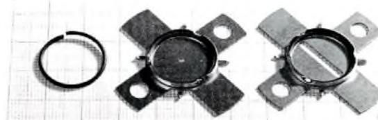
A magnetic ring of the kind used in the D14-360GY/93, and grids 4 and 5 with rings mounted. The elongated aperture in grid 5 is to accommodate beam displacement due to deflection
