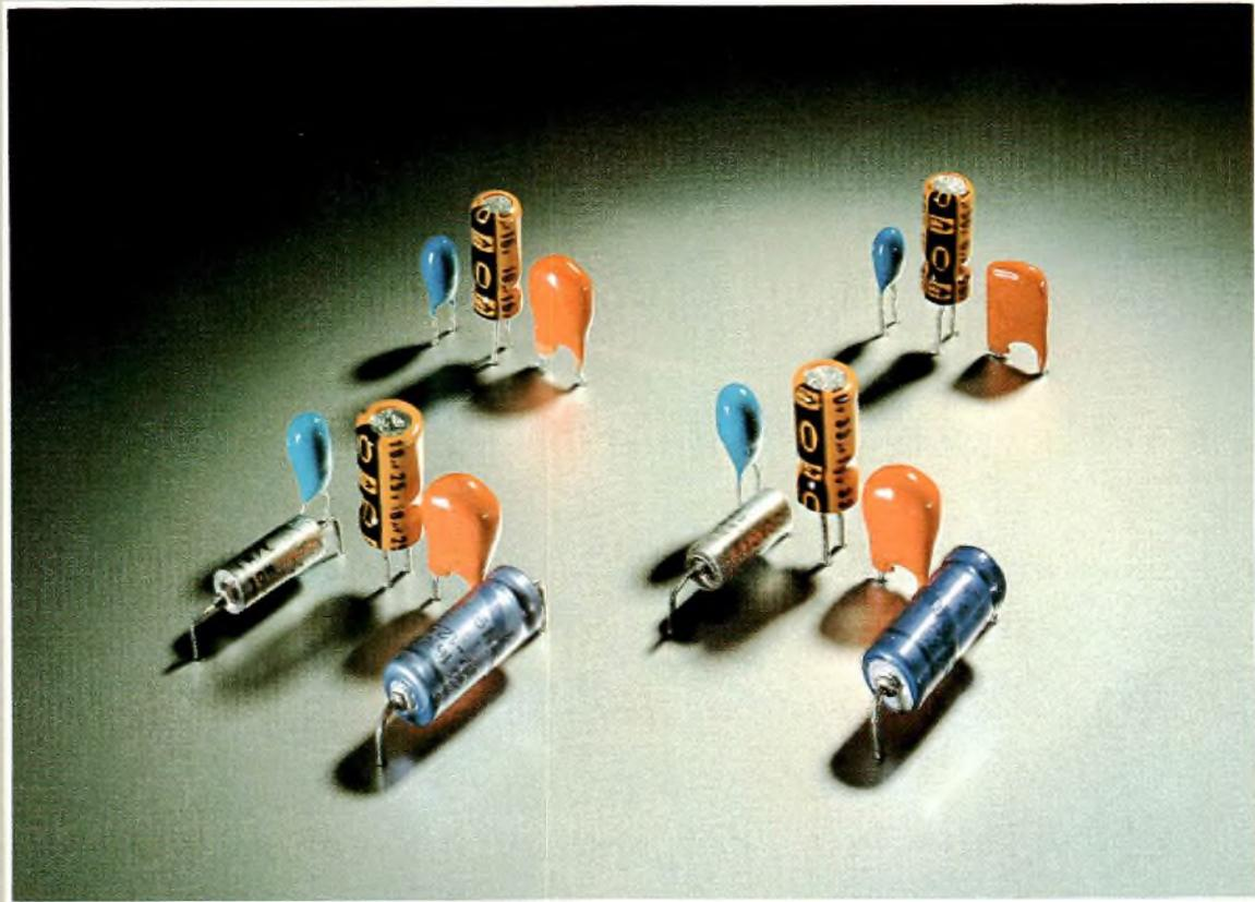
Fig.1 Comparison of small and miniature electrolytic capacitors. The two groups at the rear are, from left to right, solid tantalum, wet aluminium, solid aluminium with radial leads. The two groups in the foreground are, from left to right, solid tantalum with radial leads, solid tantalum with axial leads, wet aluminium, solid aluminium with radial leads, solid aluminium with axial leads. Each group shows capacitors of similar CV product.
