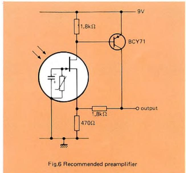
Fig.6 Recommended preamplifier
