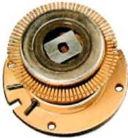
Fig.6 Thermoelectrically cooled vacuum encapsulation for  $3\ \mu\text{m}$  to  $5\ \mu\text{m}$  infrared detectors with up to 64 elements. The radial connectors around the window are for the detector elements, the two prongs near the base are for the cooler supply
