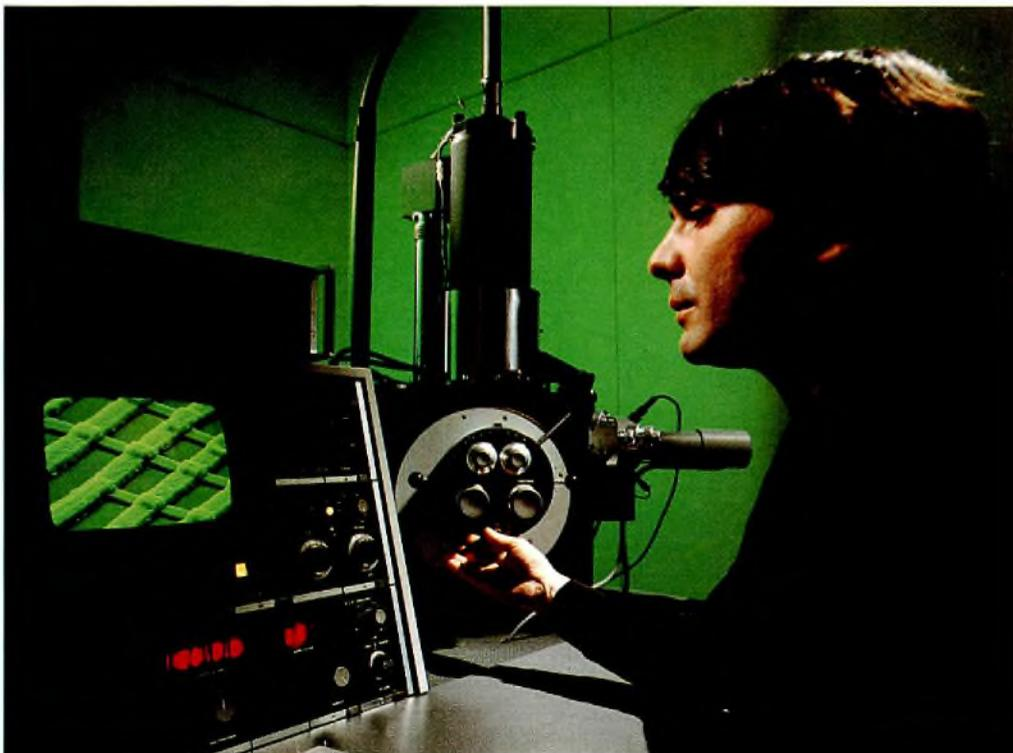
Fig.2 Quality in diffusion: Inspection of the step-coverage of the aluminium metallisation in a LOC MOS circuit, using a scanning electron microscope
