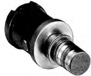
Fig.21 M3RPY dewar for arrays of up to 55 elements; engine cooled, with anti-reflection coated germanium window, for 8  $\mu\text{m}$  to 13  $\mu\text{m}$
