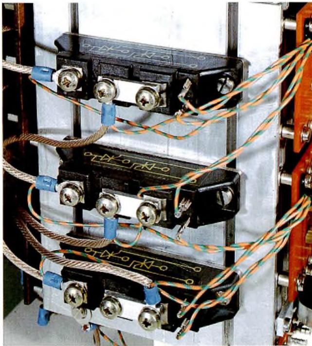
Fig.8 Thyristor stack comprising three BGX12 Isolated Power Modules. Each module contains two thyristors and has a totally isolated mounting base, thereby permitting the three modules to be mounted on a common heatsink.
