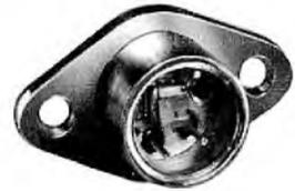
Fig.20 M2RPY dewar for arrays of up to 50 elements; Joule-Thomson cooled, with anti-reflection coated germanium window, for 8  $\mu\text{m}$  to 13  $\mu\text{m}$
