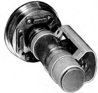
Fig.22 M5RPY dewar for linear arrays of up to 120 elements; engine cooled, with anti-reflection coated window, for 3  $\mu\text{m}$  to 5  $\mu\text{m}$  or 8  $\mu\text{m}$  to 13  $\mu\text{m}$
