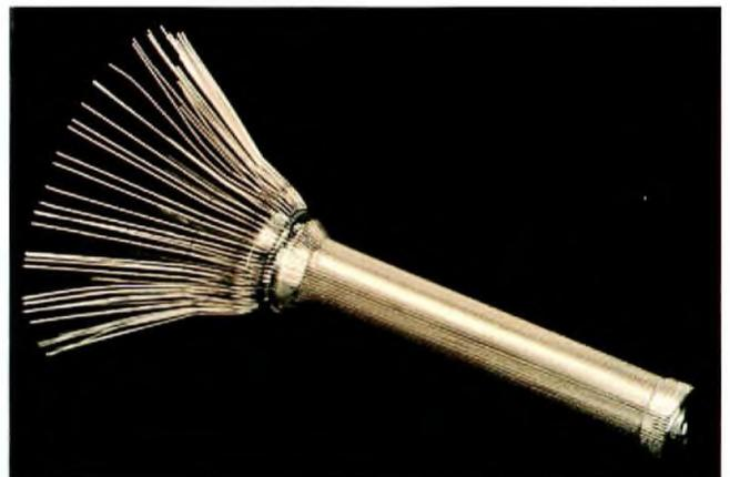
Fig.5 Precision-bore inner wall of a dewar before assembly, showing leads-in-glass construction
