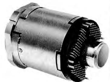
Fig.23 Dewar for linear arrays of up to 60 elements; engine cooled, anti-reflection coated germanium window, for 8  $\mu\text{m}$  to 13  $\mu\text{m}$ ; a larger version accommodates up to 120 elements
