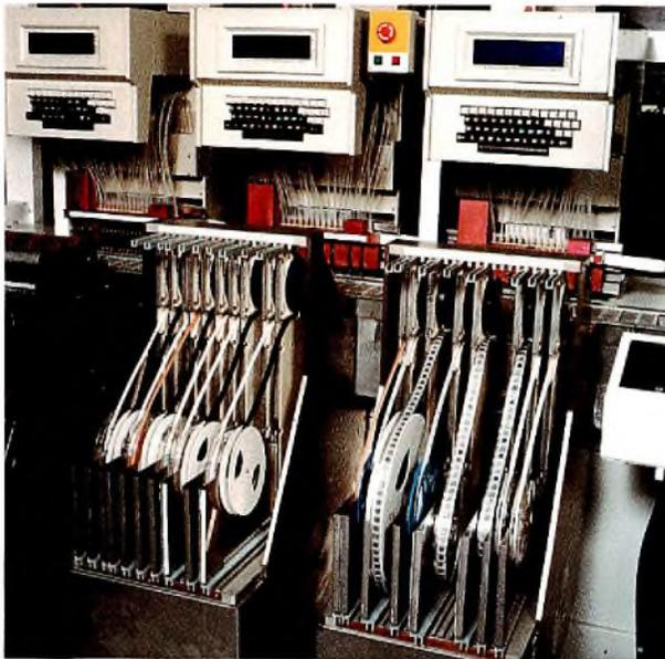
MCM IV placement heads can be fed by 8 mm tapes in 32-reel magazines or, as here, 12 mm, 16 mm or 24 mm tapes in cassettes holding up to 20 reels
