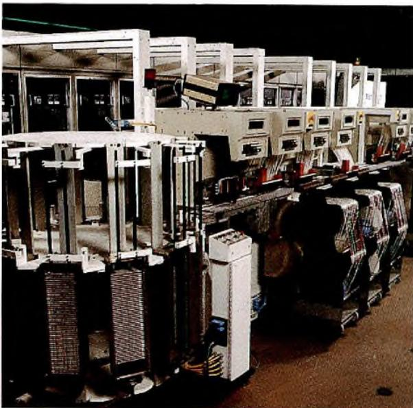
The multiple-station MCM IV includes a revolving stock turret to ensure an uninterrupted supply of substrates to the placement heads
