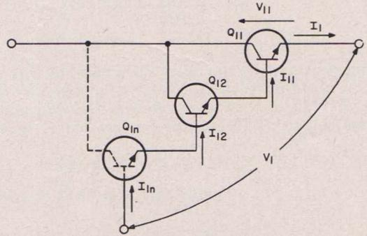
Fig.10 - Typical series regulator element.
