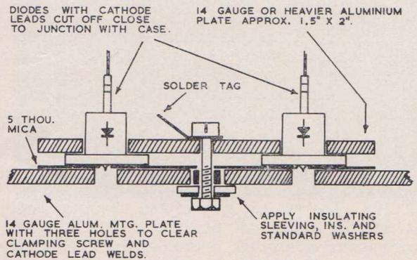
NOTE: FOR MAXIMUM EFFICIENCY OF COOLING, LIGHTLY SMEAR BOTH SIDES OF MICA PLATE WITH SILICONE GREASE BEFORE FINAL ASSEMBLY. FOR GROUND + SUPPLY, OMIT MICA INSULATOR.
