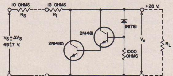
Fig.9 - Complete circuit for transistorized shunt voltage regulator.
