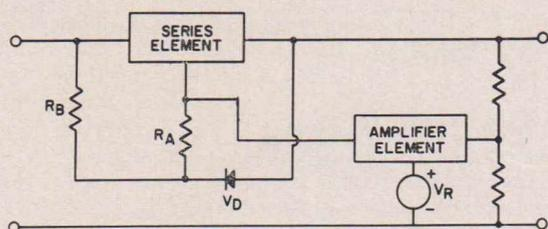
Fig. 4 - Circuit using current limiting to provide protection against overload.
