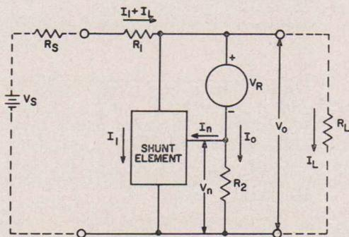
Fig.7 - Typical transistorized shunt voltage regulator.
