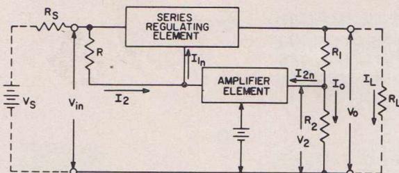
Fig. 1 - Typical transistorized series voltage regulator.
