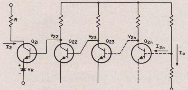
Fig. 11 - Typical cascaded dc amplifier element.
