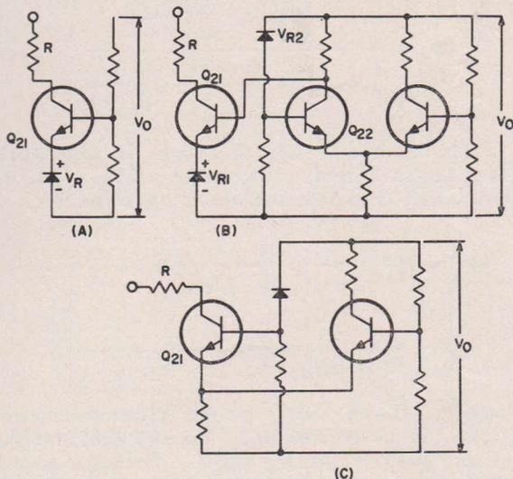
Fig. 3 - Three typical dc amplifier elements.
