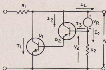
Fig.8 - Typical transistor shunt element.
