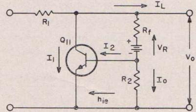
Fig. 13 - Typical single-stage shunt regulator.
