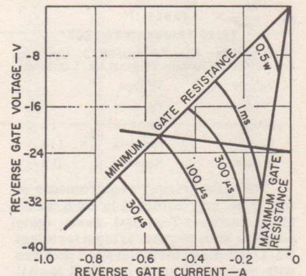
Figure 37: Reverse gate characteristics for typical RCA SCR showing load-line for a reverse gate-source voltage of 24 volts and an external circuit resistance of 5 ohms.
