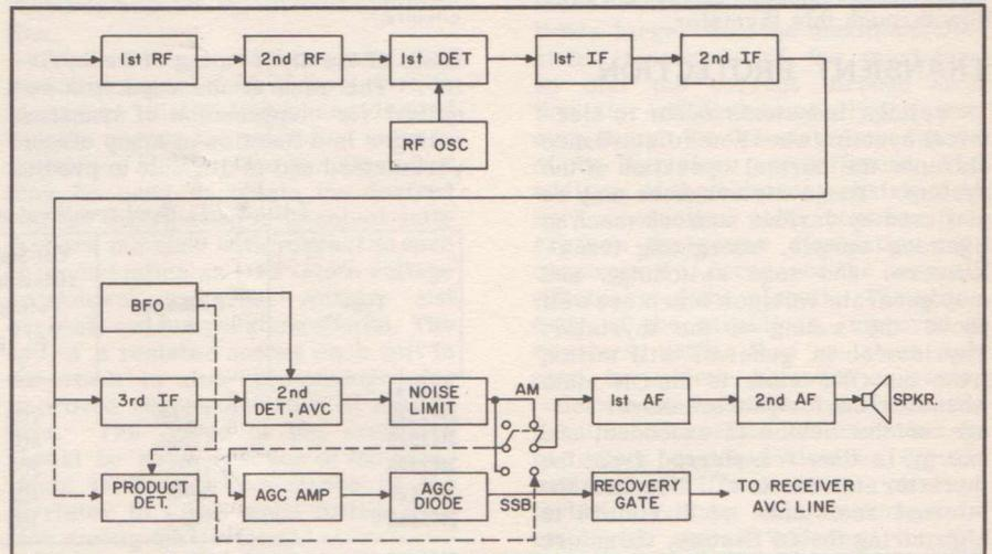
Figure 1: Block Diagram of a typical general-purpose communications receiver showing additions (dashed lines) of product detector and AGC system.
