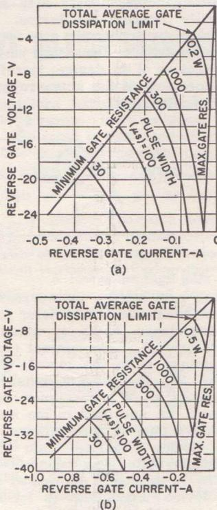
Figure 33: Reverse gate characteristics of RCA SCR: (a) low-current types, (b) high-current types.
