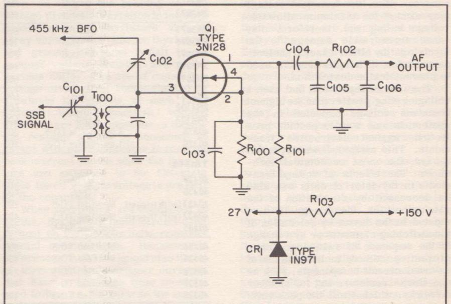
Figure 2: Schematic diagram of product detector.
