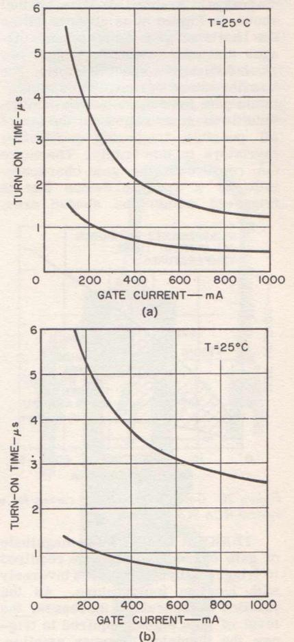
Figure 35: Turn-on time distribution among RCA SCR's: (a) low-current types, (b) high-current types.
