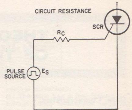
Figure 34: Equivalent diagram of the basic gate-trigger circuit for a thyristor.
