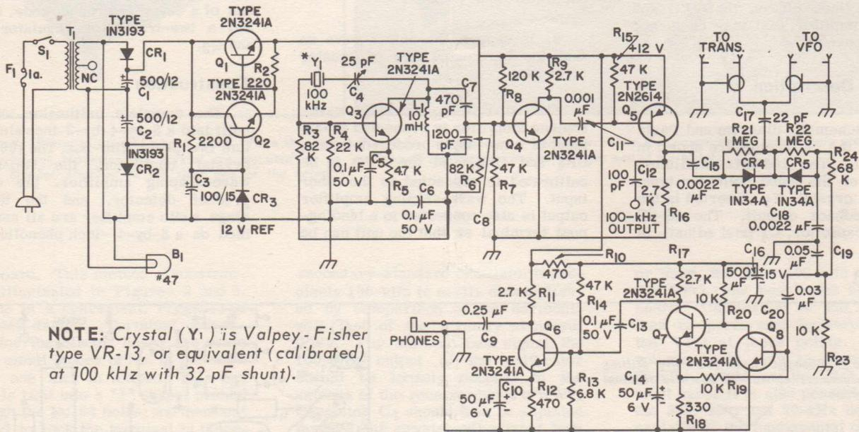
**NOTE:** Crystal (Y<sub>1</sub>) is Valpey-Fisher type VR-13, or equivalent (calibrated at 100 kHz with 32 pF shunt).
