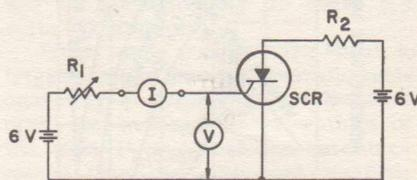
Figure 31: Test circuit used to determine gate-trigger-pulse requirements of thyristors.
