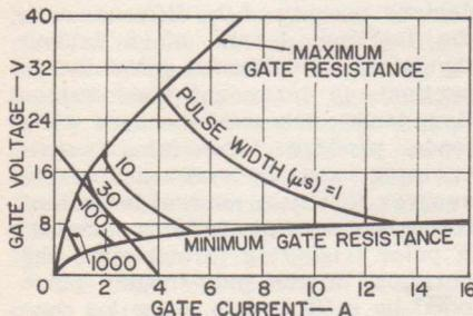
Figure 36: Forward gate characteristics of typical RCA SCR's showing load-line for a source of 20 volts and a required gate current of 1 ampere.
