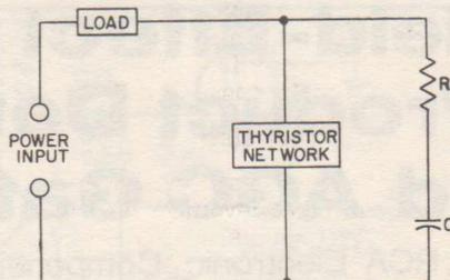
Figure 38: Diagram showing use of RC network for transient suppression in thyristor circuits.
