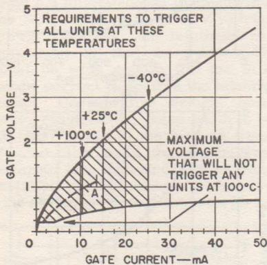
Figure 30: Gate-characteristics curves for a typical RCA SCR:
