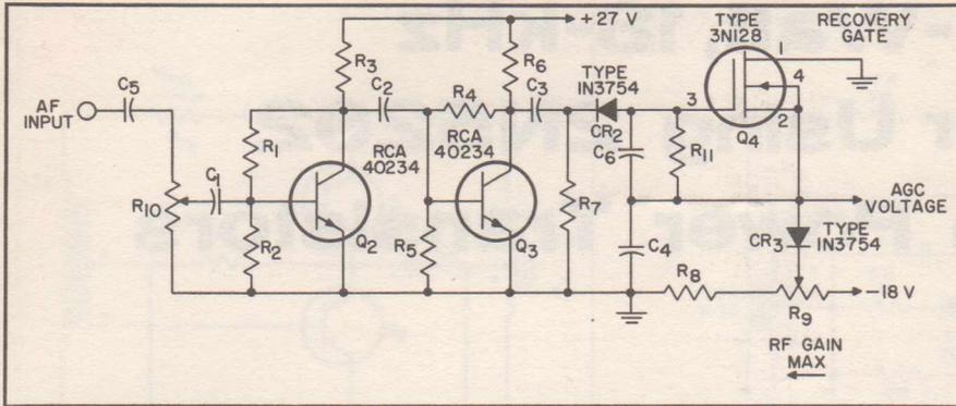
Figure 4: Schematic diagram of AGC system.
