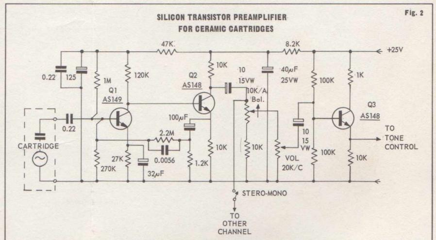
provide a smooth transition from one channel to the other. The insertion loss of this control is 3dB. When used in conjunction with the 'Stereo-Mono' switch, also provided at this point, a desirable silent transition of the effective sound source can be made from one speaker to the other, thus enhancing its use as described in the article "Phasing in Stereophonic Sound Systems" (Radiotronics May 1967).
