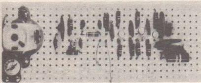
Figure 4 Layout of product-detector (left) and audio-AGC (right) components on vector board. Short wire in centre of board is the product-detector output; long-wire is the audio input for the AGC system.
