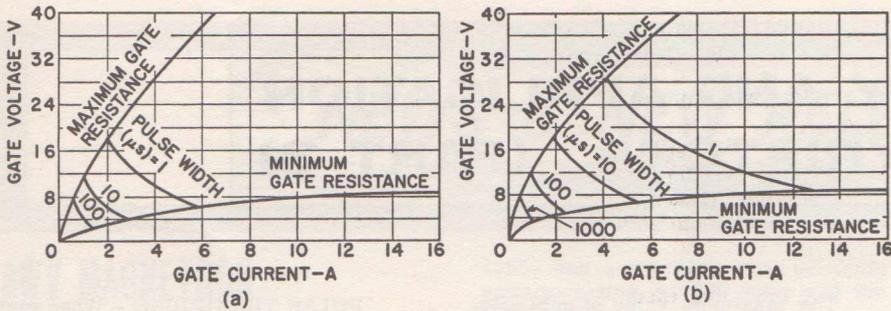
Figure 32: Forward-gate characteristics for pulse triggering of RCA SCR: (a) low-current types, (b) high-current types.
