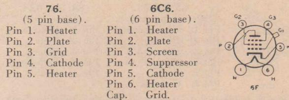
Type 76 is a general purpose triode while type 6C6 is an r-f pentode which may be connected as a triode (pins 2, 3 and 4 tied together to form the plate). Type 6C6 under transformer coupled conditions requires a decrease in bias from -13.5 volts to -8 volts, but in other respects the characteristics are fairly similar. Under resistance coupled conditions a change of bias resistor may or may not be necessary.
