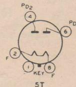
Types 5Y4-G and 5Y3-G are electrically identical, the only difference being in the base.
