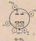
Type 5X4-G is electrically identical to type 5U4-G, but has a different number of pins in the base and different base connections. Apart from these differences in the base all other remarks apply as for type 5U4-G.
