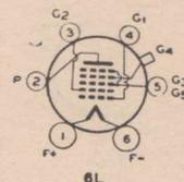
Type 15 is an indirectly heated 2-volt pentode, which is most commonly used as an autodyne converter. The circuit is similar to that used in a-c autodyne receivers.
