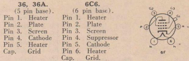
Type 36 is a screen grid r-f amplifier, while type 6C6 is a pentode r-f amplifier having higher gain and lower plate and screen currents. In most cases types 6C6 can be substituted for type 36 or for type 36A merely by making the necessary change in socket and connections.
