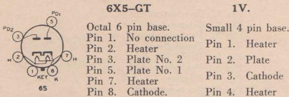
Type 1V is a half-wave indirectly heated rectifier having a heater current of 0.3 ampere, while type 6X5-GT is a full-wave indirectly heated rectifier, having a heater current of 0.6 ampere at 6.3 volts. The 6X5-GT may be used as a replacement for type 1V where the heater is supplied from a 6.3 volt source but not in AC/DC receivers.
