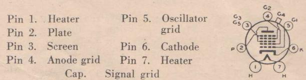
Type 2A7 is electrically identical to type 6A7, except for the heater rating. Type 2A7 has a heater rated at 0.8 ampere at 2.5 volts, while type 6A7 is rated at 0.3 ampere at 6.3 volts.
