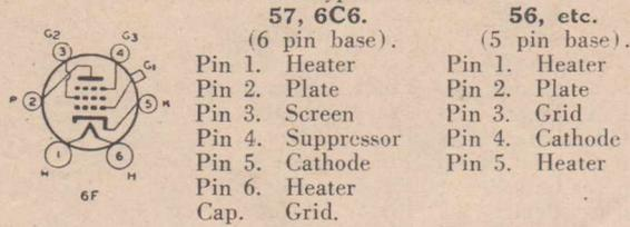
Type 56 is a general purpose triode while types 57 and 6C6 are r-f pentodes which may be used as triodes by connecting together pins 2, 3 and 4 as the plate. Types 57 or 6C6 connected as a triode require a lower bias than type 56 (-8 instead of -13.5 volts). In other respects their characteristics are very similar although the stage gain with types 57 or 6C6 will be higher.
