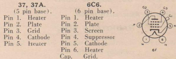
Type 37 is a general purpose triode while type 6C6 is an r-f pentode which may be connected as a triode to give characteristics somewhat similar to those of type 37. For triode operation Pins 2, 3 and 4 should be connected together to form the plate while the grid connection will go to the top cap.
