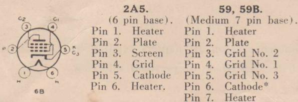
\*No connection in the case of type 59B which is directly heated.
