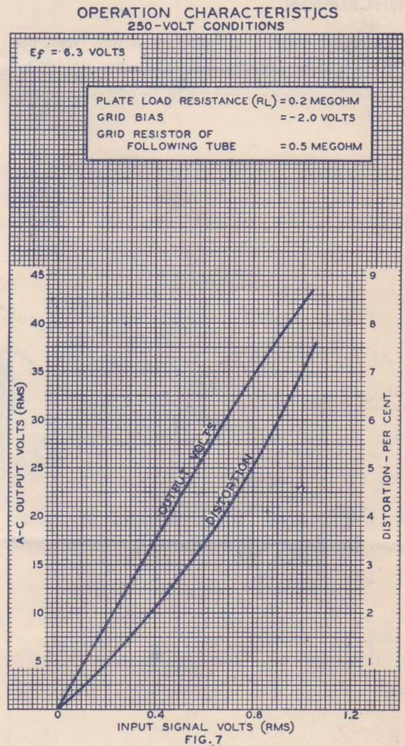
gain and distortion requirements. For most radio receiver applications, a bias of  $-2.0$  volts and a plate load resistance ( $R_L$ ) of 0.2 megohm are suitable.
