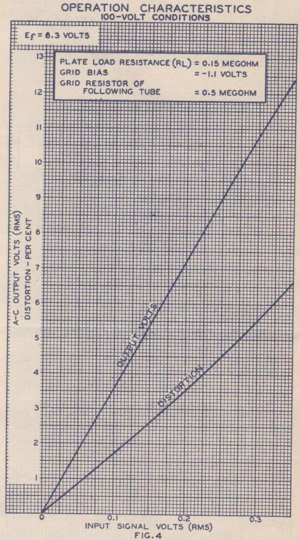
reasonably high signal voltages may be applied at low plate voltages, where the bias required for Class A operation is small.
