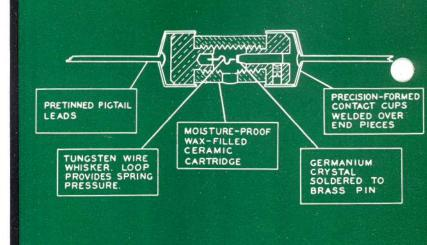
Cross sectional view showing crystal construction details.
