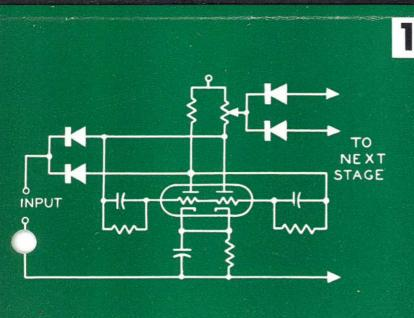
Sylvania germanium crystals are useful as coupling diodes in applications such as this trigger circuit.
