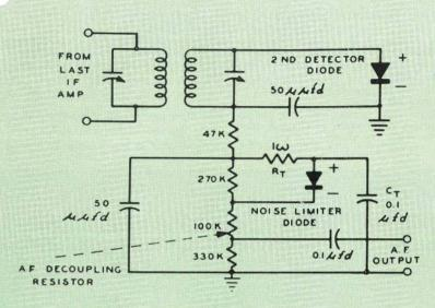
COMBINED NOISE LIMITER AND SECOND DETECTOR
