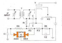
modulation receivers. The circuit is self adjusting to the average level of the received signal, and sharply clips impulse noise components which exceed a certain amplitude relative to it. Using a type 1N54 high reverse resistance crystal as a series clipper element, and a general purpose type 1N34 as a shunt clipper element, this circuit requires few components and little space, yet provides an unusually high degree of impulse noise suppression. 🖕 .
