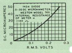
Voltage Calibration Curve for Low-Z Crystal Voltmeter Circuit using a Weston Model 301 0-200 D. C. Microammeter.
