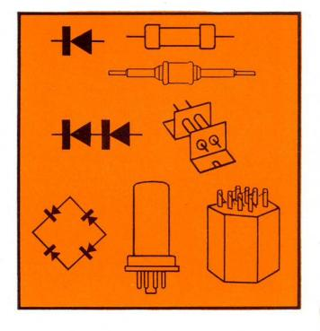
matched for use in balanced circuits for full-wave rectification, modulation, demodulation or ratio detection. The component diodes are matched for similar values of forward resistance under conditions typical of those in actual use. Resistances are maintained sufficiently high in the back direction to insure a good front-to-back ratio. The Sylvania Type 1N35 duo-diode permits compact packaging and easy portability of balanced circuits.
