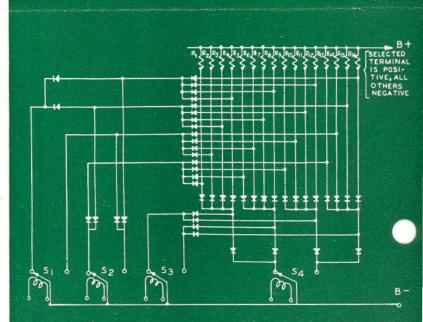
The Crystal Diode Matrix as a high speed selector switch provides another important use for the Sylvania germanium diode family.
