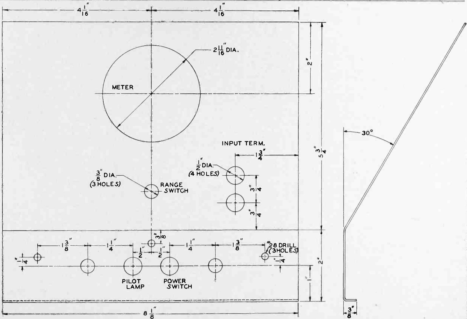
Fig. 3. Front Panel Layout.
