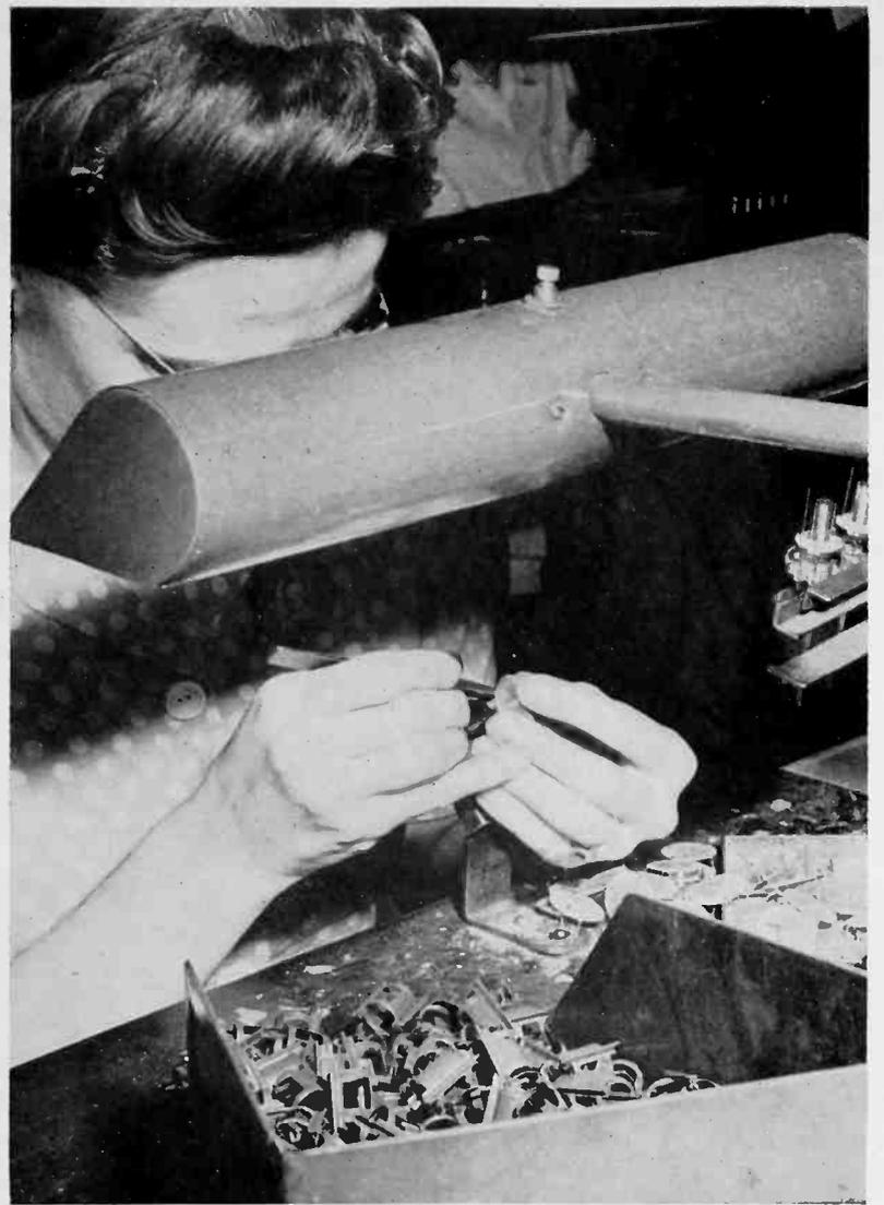
Next, the plate and top mica are put in position.
