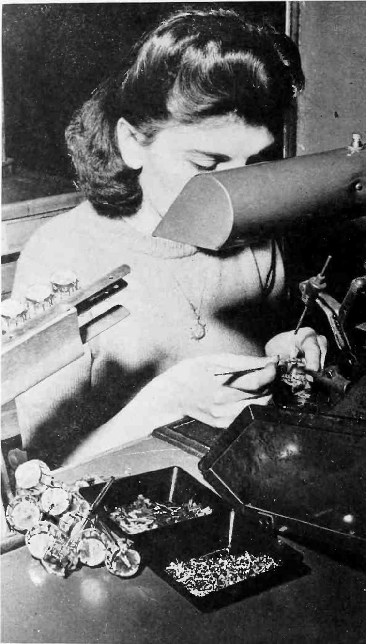
The first operator starts with a stem assembly, welds on a few connecting tabs, the bottom shield and mica, then passes it to the girl on her right.
