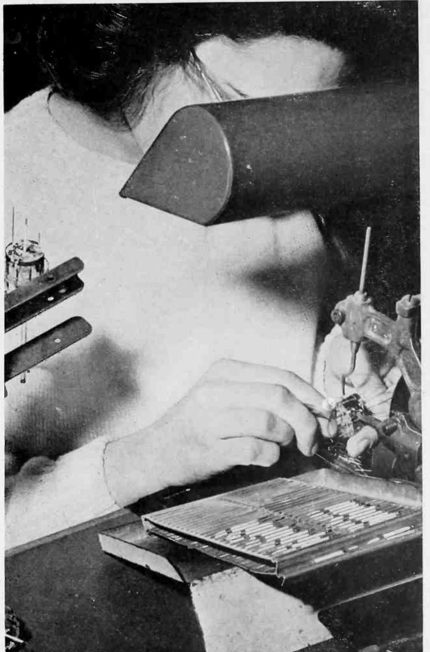
This operator welds the cathode and heater assembly in place, adds one mount support rod and the plate connector.
