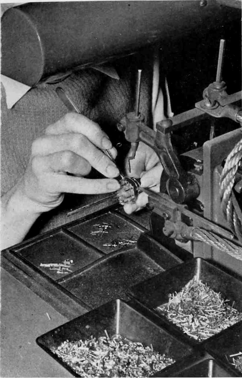
These unwelded parts are now all spot-welded in place with tiny "jumpers" of nickel plated steel ribbon (shown in the square boxes) connecting each element to the proper lead.
