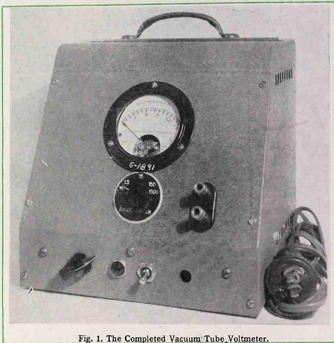
Fig. 1. The Completed Vacuum Tube Voltmeter.
