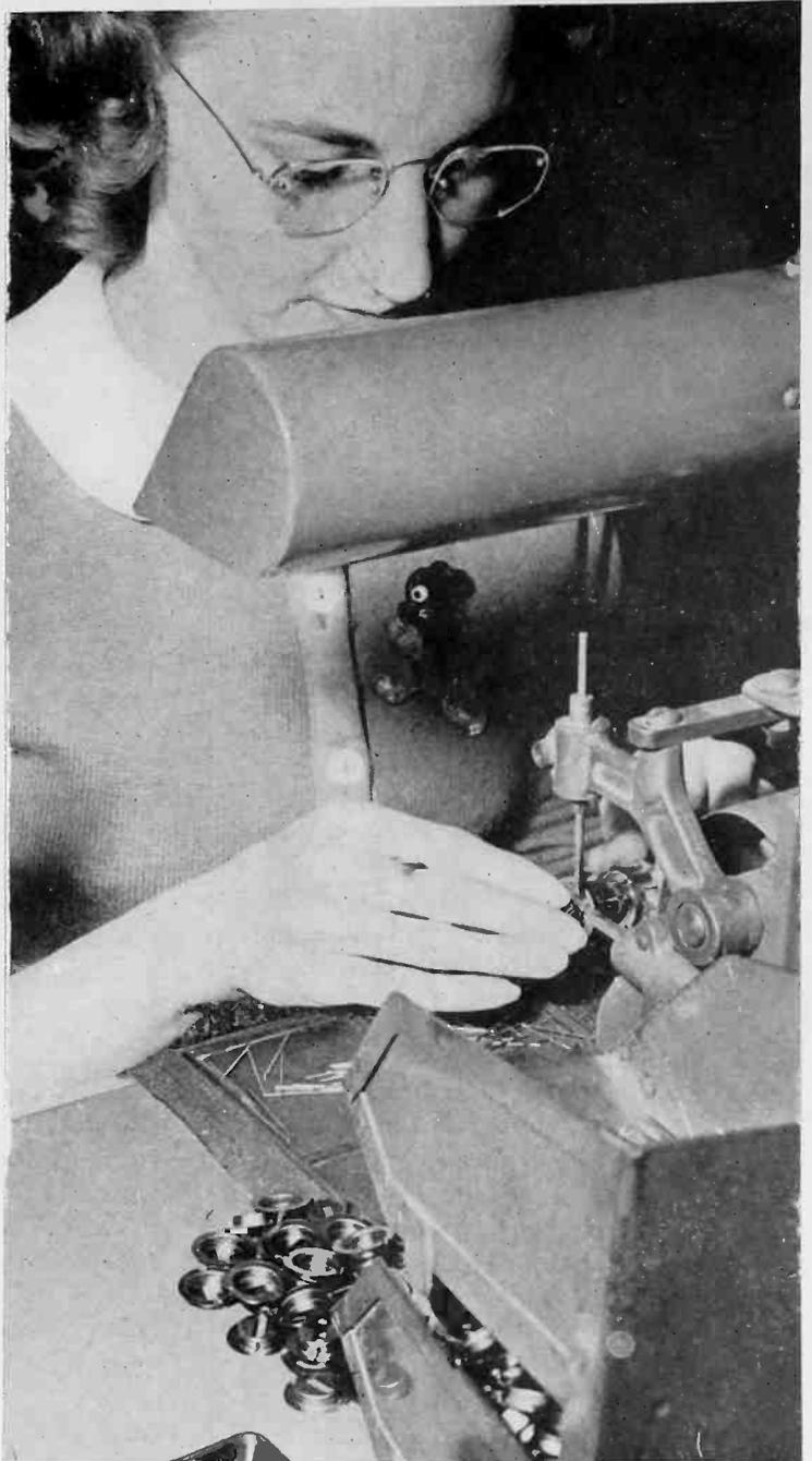
The top shield is now put in position and welded. The last mount support rod is also added.
