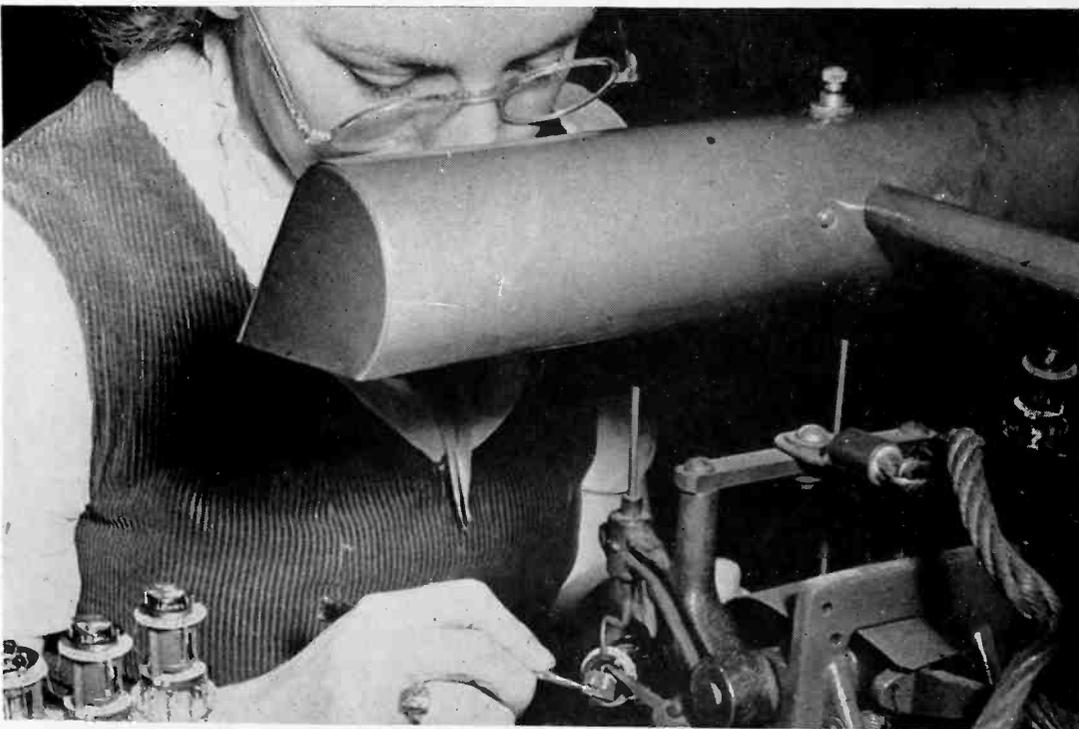
The last operator adds the getter flag and gives the complete mount a final inspection before it is taken to the sealing and exhaust machine. This team of operators complete about 180 mounts per hour.
