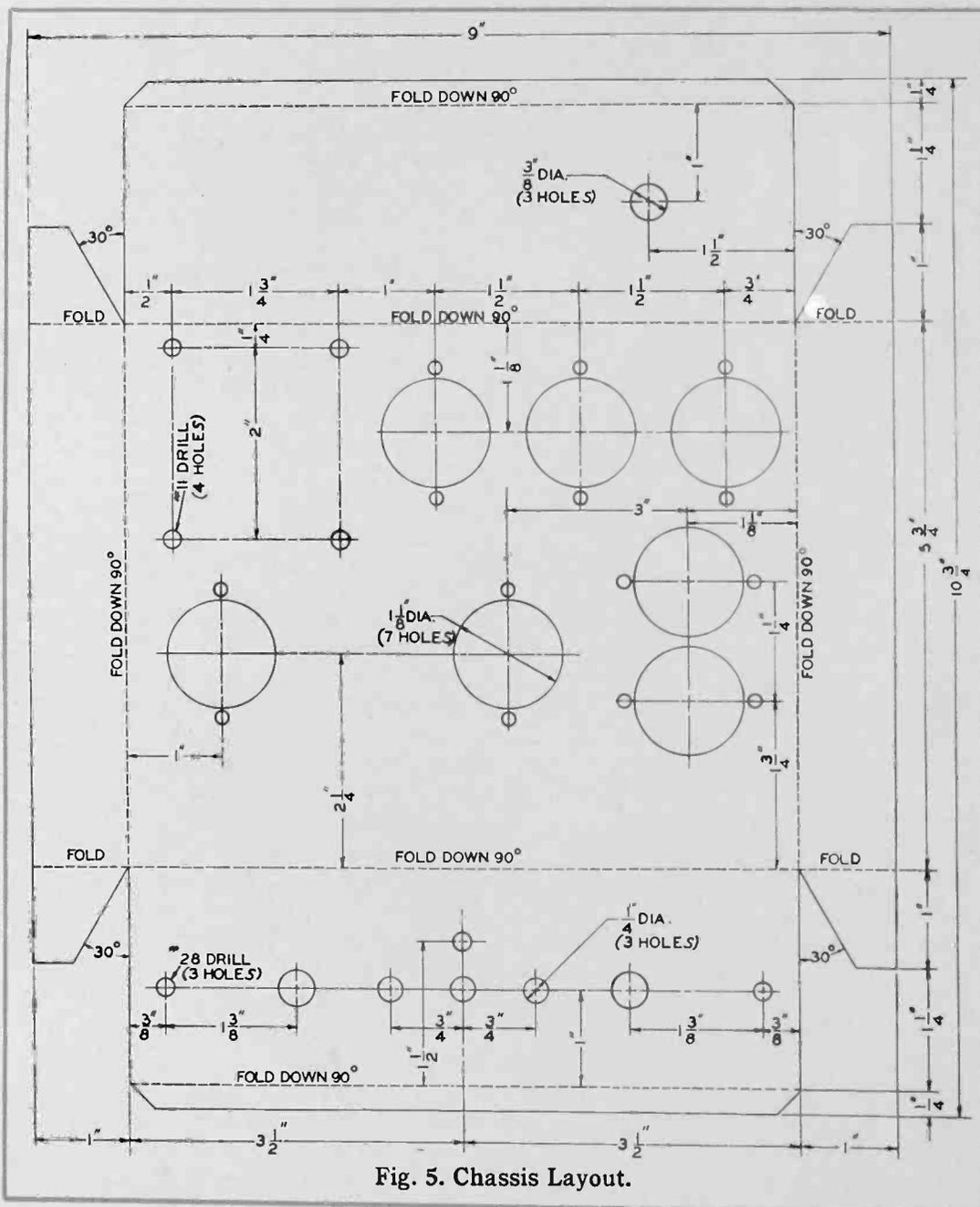
Fig. 5. Chassis Layout.
