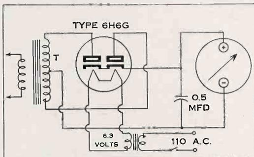
I used a Stancor Output Transformer No. 3856 (T) as the 6 taps are a convenient adjustment for different outputs. The meter I had was a 150-volt Triplett 1000-ohm per volt meter with taps at 3 and 7.5 volts but these were not used. The condenser, which should have a paper dielectric, should be rated for 200 volts at least and is required only to keep the A-C ripple from damaging the meter.
