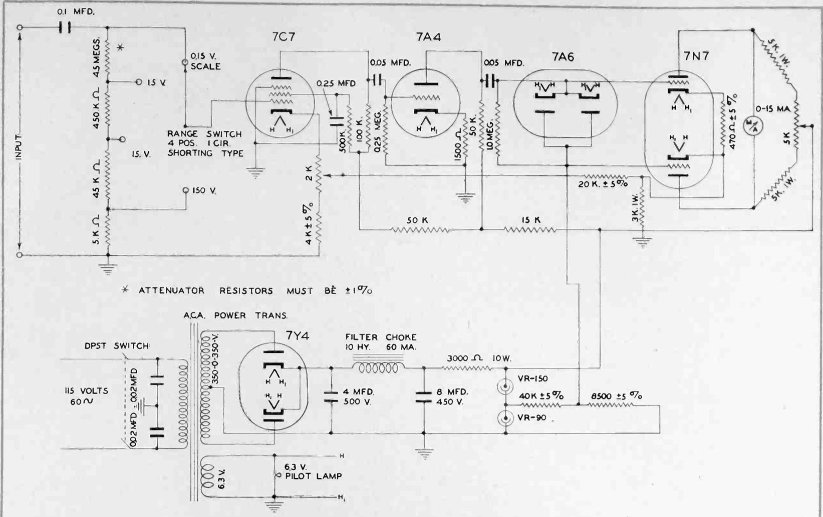
Fig. 2. Schematic Circuit Diagram of Sylvania VTVM.
