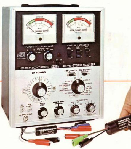
**FM RF Coverage:** 87 to 109 Megahertz; unmodulated, MPX or 400 Hz sine modulation.
