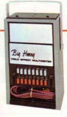
DC Volts: 0-0.3, 1, 3, 10, 30, 100, 300 1KV, 3KV, full scale, positive and negative. Zero center ranges: All positive and negative, 0.15, 0.5, 1.5, 5, 15, 50, 150, 500, 1.5KV. Input resistance: 15 megohms shunted by 58 pf. Accuracy: 1.5%. AC rejection: 30DB minimum.
