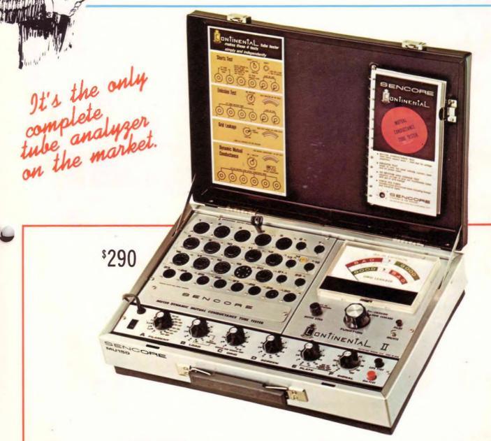
Mutual conductance test: 5,000 hertz square wave under actual amplifying conditions. The tube is harnessed up in the circuit, unlike other testers that are vanishing from the market that use the tube to do its own rectification.
