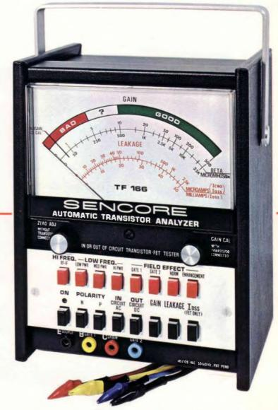
**Transistor Tests:** In or out of circuit for gain. Out of circuit for leakage tests only. Gain measured as good or bad or in Beta. Leakage (Icbo) measured in microamps.
