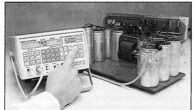
Fig. 1: Paralled banks of high value, high voltage capacitors can exceed the design limits of your Z Meter. Always test these capacitors one at a time.
