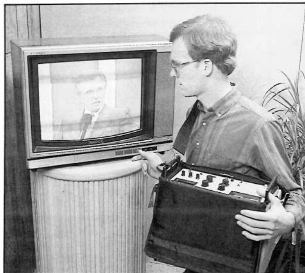
Fig. 1: Trust your CHANNELIZER to prove whether the cable system is causing a hum problem.
