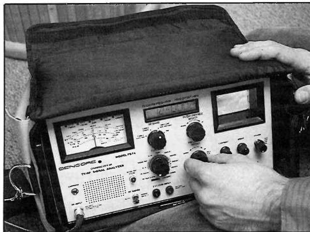
Fig. 2: The analog and digital meters quickly show you that the signal level and frequency are correct.
