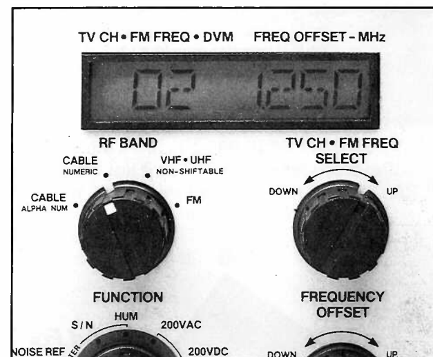
Figure 2: The Channelizers let you manually tune in 50 kHz steps to any cable channel from 5 to 495 MHz.
