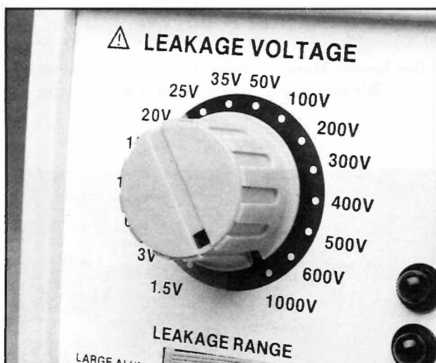
Fig. 7: Find leakage in capacitors, SCRs, triacs, or hi-pot applications with the LC101 leakage voltage extending all the way up to 1000 volts.
