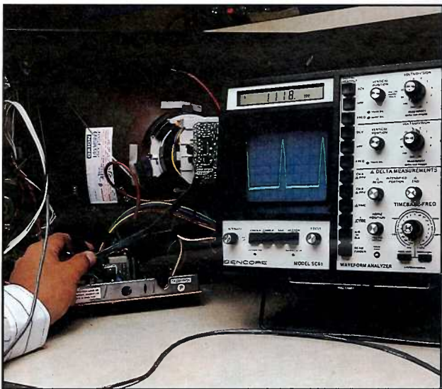
Fig. 7: The 3000 volt peak-to-peak (or 2000 volt DC) measuring range of the SC61 lets you measure any signal; patented circuits protect the input for any attenuator setting.
