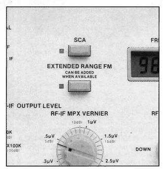
Fig. 13: The SG80's SCA signal lets you dynamically test and set SCA traps. The Extended Range FM button allows for later updates if and when new FM modulation schemes are accepted.
