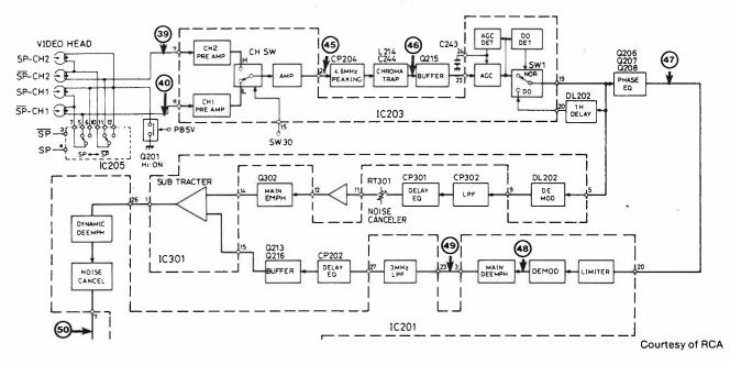
Fig. 1: You can use your Sencore block diagram to locate corresponding test points on any manufacturers' block diagram—as is shown above on the RCA VLPG25HF block diagram.
