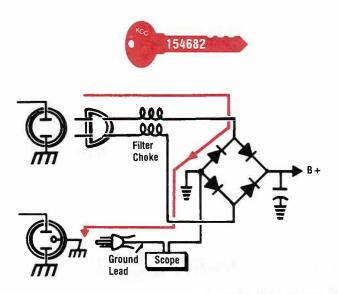
Fig. 2: Connecting a ground lead to a bridge rectifier chassis without using an isolation transformer will short out half the power supply.
