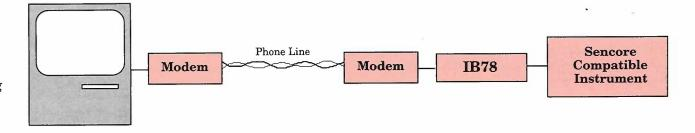
Fig. 2: Use your Sencore instrument for remote location testing or automatic monitoring with modems and a dial-up phone line.
