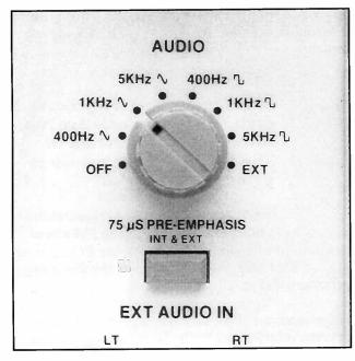
Fig. 16: The internal audio generator produces low distortion sinewaves, and harmonically-rich square waves for fast, reliable testing. Standard 75 microsecond pre-emphasis can be added when needed.
