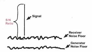
Fig. 9: The SG80 provides very low background noise, allowing you to make accurate sensitivity and S/N tests on low-noise receivers. Other generators have higher noise levels, which causes the tests to be in error.
