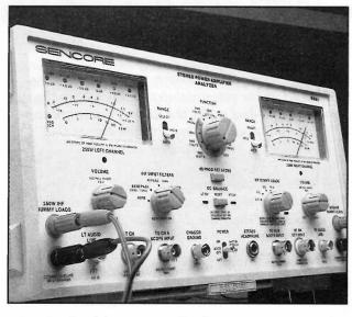
Fig. 4: Analog meter displays let you monitor audio levels or balance without the frustration of bouncing digital displays.
