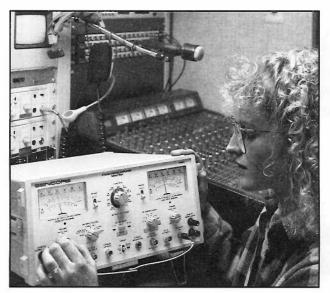
Fig. 3: The portable PA81 is ready to go with you on any service call to help you monitor signals or track problems down.
