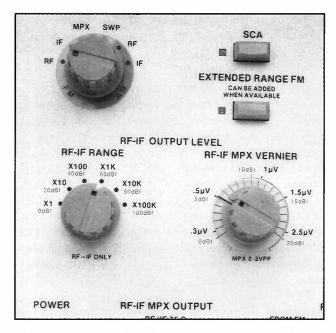
Fig. 4: The SG80's microprocessor-controlled attenuator is calibrated in both microvolts and dBf (dB referenced to a femtowatt) to match all manufacturers' specifications.
