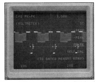
Fig. 6: Multiple readings can be complicated, and some readings disappear for certain setups, making even more confusion—they take your mind off your circuit.
