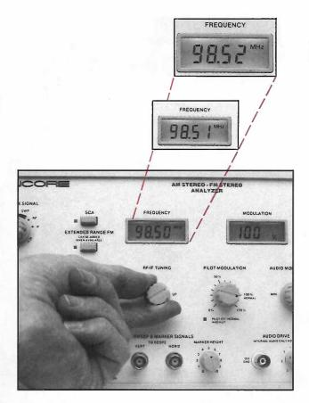
Fig. 8: Pressing the tuning knob moves the SG80 tuner to fine tuning steps of 10 kHz (0.01 MHz) for tests of the automatic tuning circuits.
