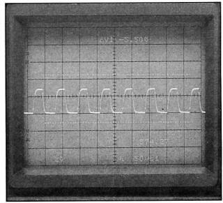
Fig. 2: Manual cursors don't follow the signal, so the reading remains the same if the signal changes amplitude—or disappears altogether.
