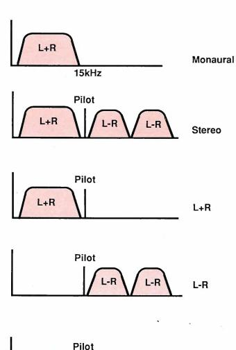
Fig. 15: Each setting of the AM & FM MPX MODE switch produces a different set of modulation conditions to dynamically test each part of the stereo decoder.
