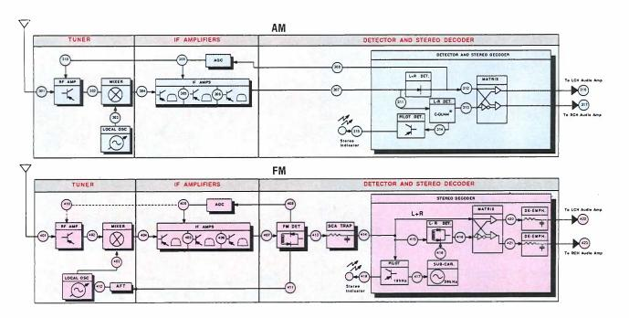
Fig. 3: The SG80 makes AM and FM troubleshooting look alike, by supplying the signals needed to test or align any stage from the antenna to the output.
