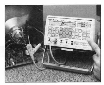
Fig. 4: The LC102 finds inductors with shorted turns using the exclusive in- or out-of-circuit Ringer Test.
