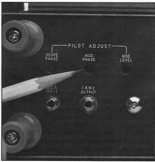
Fig. 11: Other FM stereo generators have phase adjustments which affect separation. The patented Sencore system holds proper phases all the time, without controls which can drift.
