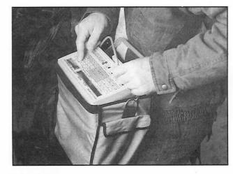
Fig. 6: The portable LC102 AUTO-Z lets you extend your testing capabilities to areas where a 120V wall outlet isn't available.
