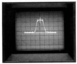
Fig. 17: Only the SG80 lets you tune the center marker of the sweep system to whatever frequency you need to match the circuits under test. Here, a center-marker frequency of 10.65 MHz matches the fixed-tuned IF stages.
