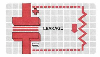
Fig. 2: Leakage develops when the capacitor has an internal parallel resistance. The LC102 tests for leakage with voltages up to 1000 volts.
