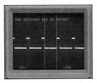
Fig. 4: Competitive scopes give errors when the horizontal or vertical vernier controls are "uncalibrated."
