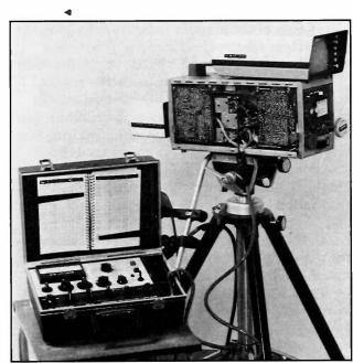
Fig. 4: Test and restore camera vidicons using the CR70 "BEAM BUILDER" without the hassle of removing the vidicon from the camera.
