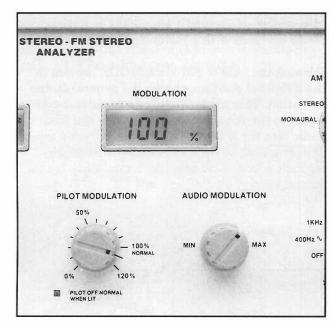
Fig. 14: The SG80 has separate modulation controls for the stereo pilot and the audio signal. The digital modulation meter indicates the total modulation, for reliable tests every time.
