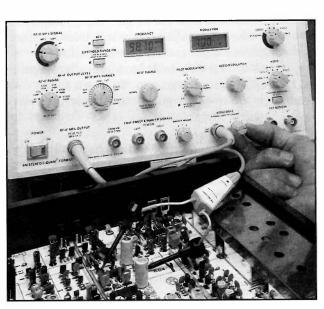
Fig. 19: The SG80 substitute signals "swamp" out the signal in the circuit, so you don't have to disconnect components when troubleshooting.
