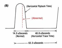
Fig. 3: Tuning capacitors (A) determine the horizontal flyback pulse timing. A shorter flyback pulse, (B) allows the horizontal output transistor to overheat.
