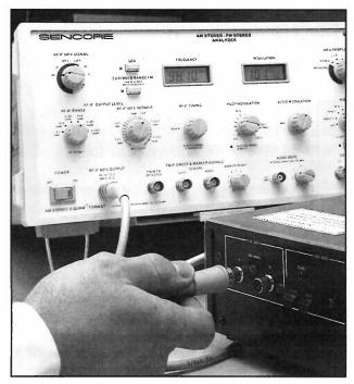
Fig. 5: The 75 ohm output of the SG80 connects directly to the receiver input, without needing matching pads or conversion formulas.
