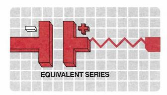
Fig. 3: Capacitor ESR is the resistance of its leads and dielectric. The LC102 automatically calculates capacitor ESR and displays it on the LCD readout.
