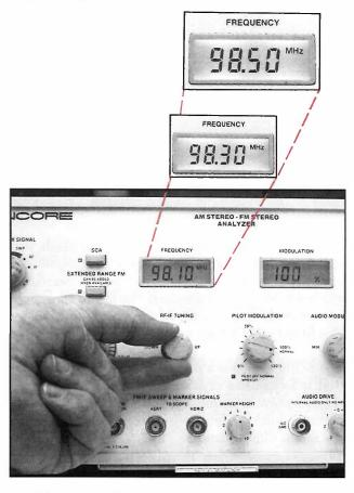
Fig. 7: The SG80 starts at the IHF test frequency of 98.1 MHz, and tunes one channel at a time as you turn the knob.
