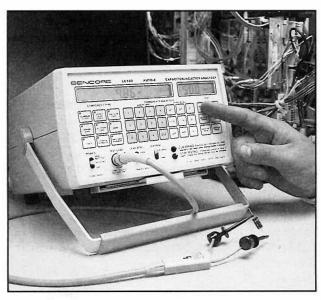
Fig. 5: The LC102's memory capabilities and GOOD/BAD readings are like having a standards engineer with you at all times.
