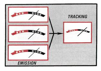
Fig. 3: The exclusive tracking memory circuit will store each projection CRT's beam current for up to 20 minutes. This allows you to show the customer which CRT needs to be restored.
