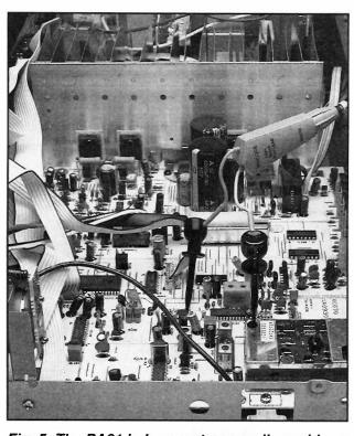
Fig. 5: The PA81 helps you trace audio problems down to the component so you can avoid swapping boards or shotgunning parts.
