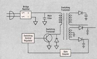
Fig. 1: A typical switched mode power supply contains a switching transformer and several filter capacitors that the LC102 can dynamically analyze.
