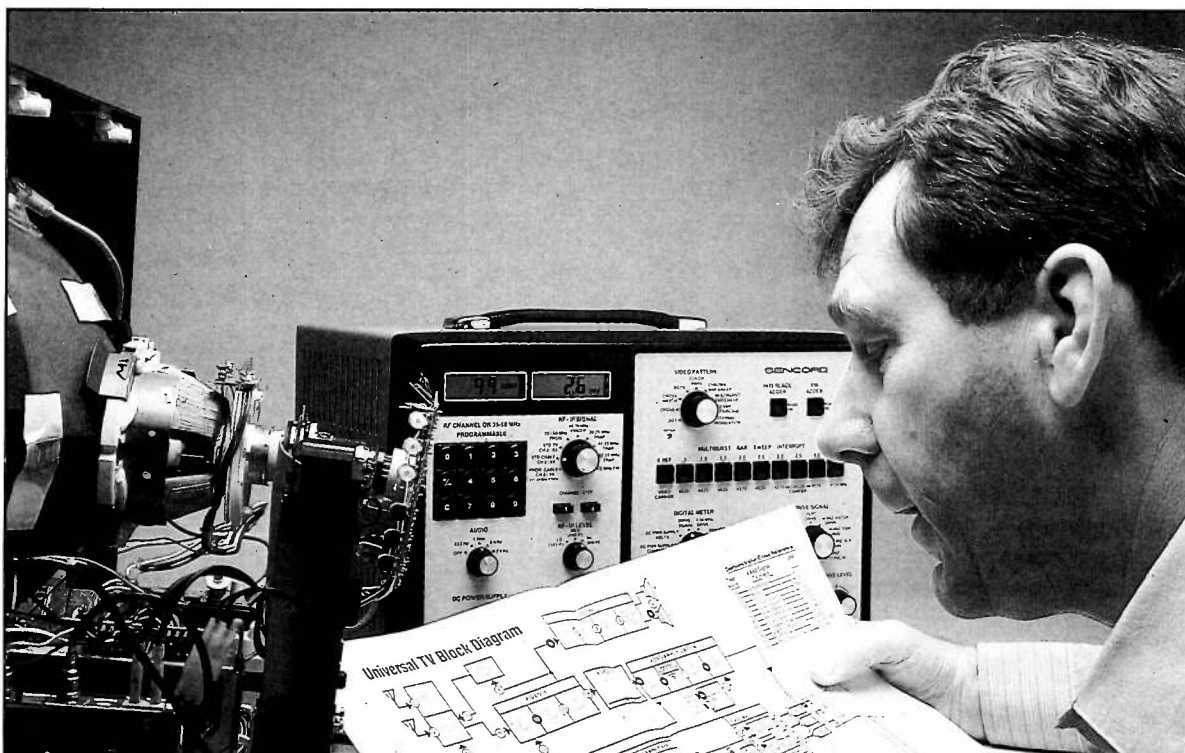
Fig. 2: The functional block diagram helps you isolate the trouble in the set you are testing.
