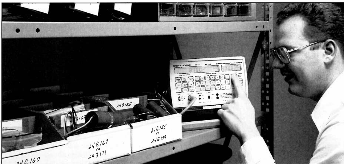
Fig. 6: Capacitors can develop leakage just sitting on the shelf. Use the LC102 AUTO-Z to detect and reform these capacitors.
