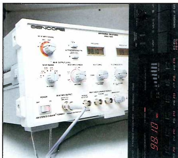
Fig. 2: The signal strength meter gave a quick indication the receiver had poor sensitivity.
