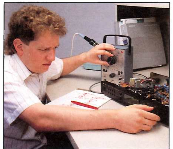
Fig. 6: Analog tuned generators drift in frequency and often require periodic retuning of the generator frequency.
