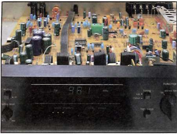
Fig. 3: Even though the front panel display on the receiver reads the correct frequency, it does not prove that the receiver is tuned to the correct station.
