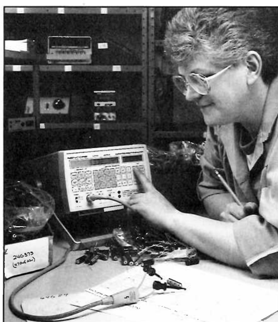
Fig. 3: The LC102 gives a decisive "GOOD" or "BAD" indication so any worker can use it with no chance of error.
