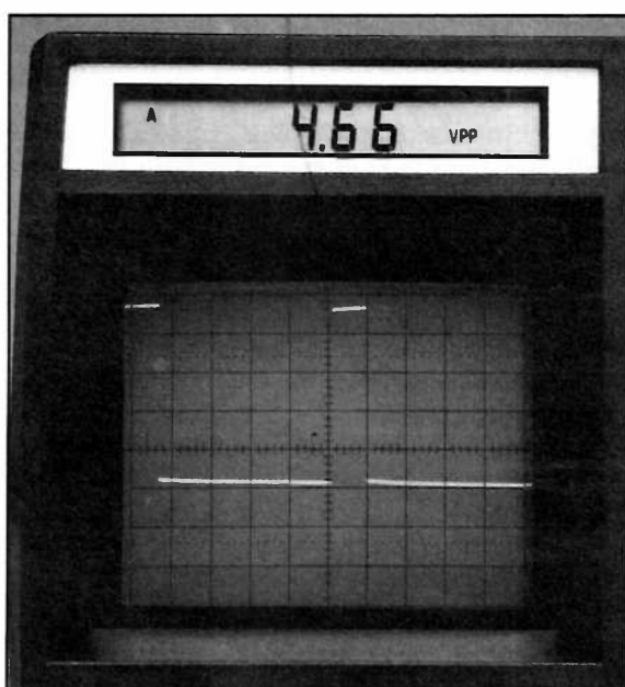
Fig. 10: Some servo problems will cause the PWM to go to maximum or minimum correction. If so, it may show pure DC, or a very narrow pulse, as shown here.
