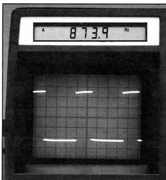
Fig. 9: When the pulse width modulator normally corrects for variations in tape motion, the output shows horizontal movement. Loading a motor by lightly touching a pulley with your finger should cause the pulse width to change.
