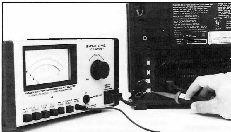
Fig. 1: To make a safety leakage test with your PR57, simply plug the chassis into the POWERITE® and touch the probe to all exposed metal surfaces.
