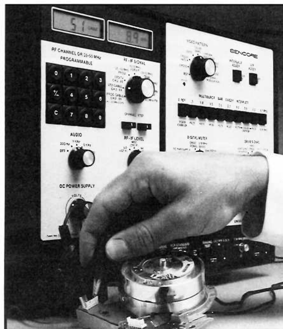
Fig. 7: You can confirm that each set of motor windings works by momentarily pulsing each with the VA62A power supply. If the motor turns part of a revolution, the coils are working.
