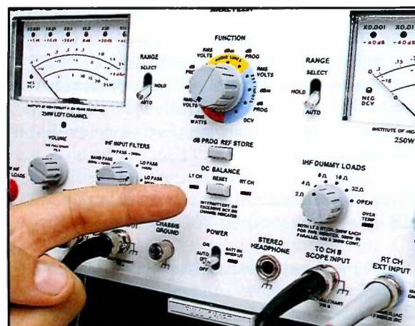
The PA81 Stereo Power Amplifier Analyzer program-mable dB function takes the calculations out of many radio tests.
