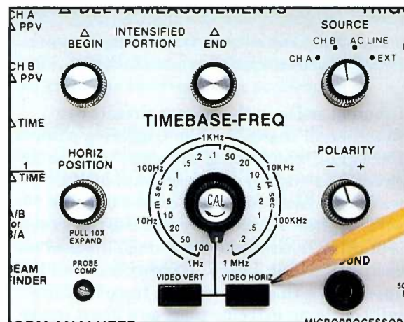
The video preset positions on the SC61 let you sync onto video waveforms at the vertical or horizontal rate with the push of one button.
