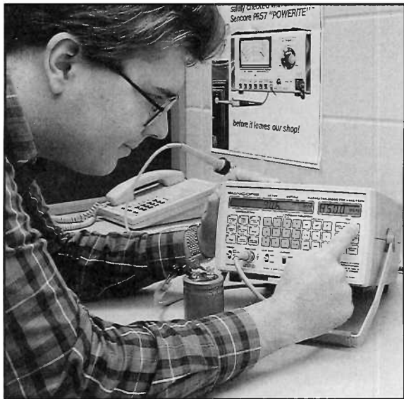
The LC102 Auto-Z tests electrolytics for all capacitor failures and automatically tells you if the capacitor is GOOD or BAD.
