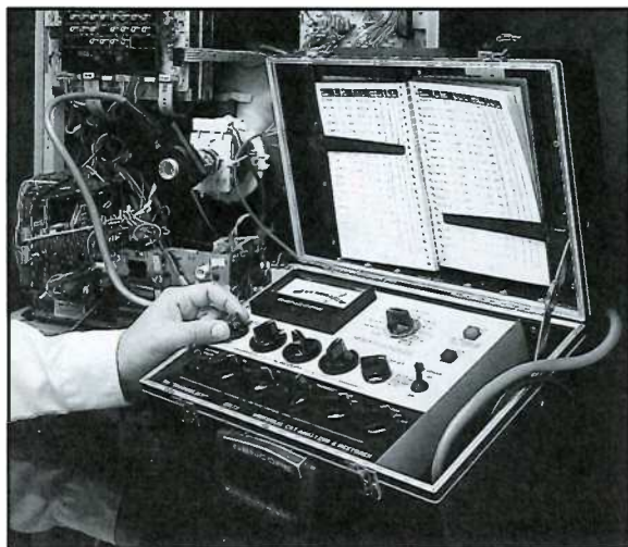
Use your CR70 Beam Builder to analyze the condition of the television's most expensive part (the CRT) without mistakes.
