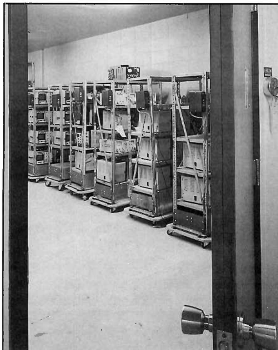
The "Shake 'n Bake" room weeds out any unit that would fail within the first month's use. We find the problems so you won't have to.
