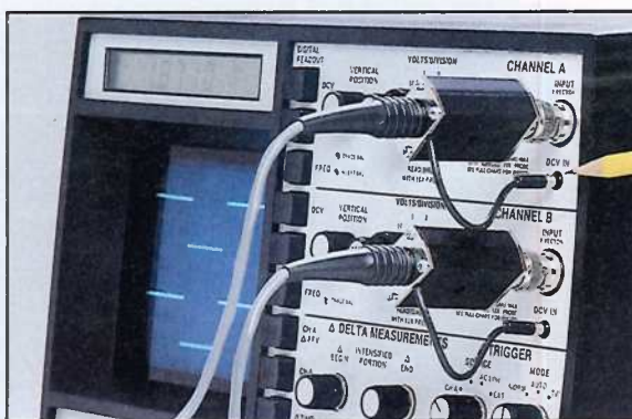
Fig. 5: The SC61's exclusive DC signal path lets you instantly switch from AC to DC digital readings, no matter where you have the input coupling switch set. This lets you move through power supply testing quickly.
