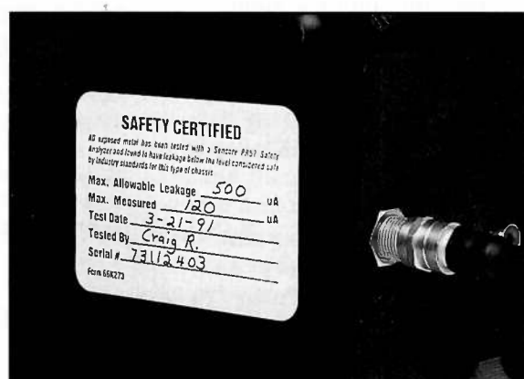
Figure 2: The safety leakage sticker tells your customer you have checked his equipment for shock potential due to leakage.
