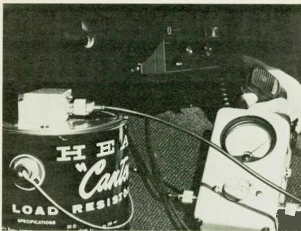
Fig. 19—Built-in CB41 dummy load eliminates external load for accurate RF power tests.
