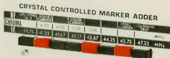
Sencore generators feature easy-to-use pushbutton markers with marker frequency listed on front panel.
