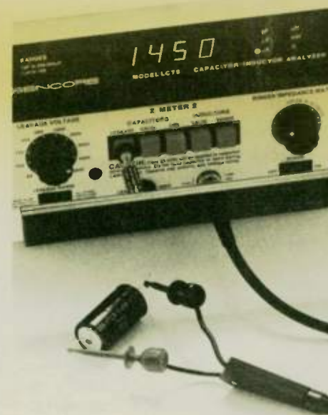
Fig. 8: Simply use the supplied push button holder to latch the Leakage button to attempt to reform leaky electrolytic capacitors.
