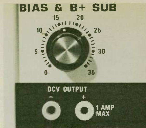
Fig. 47—Well-filtered supply provides positive or negative voltage (by just reversing leads) for four big circuit checks and uses.
