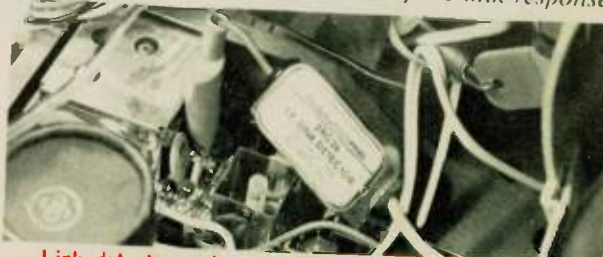
Link detector probe connected for link alignment of Admiral K-10 chassis.
