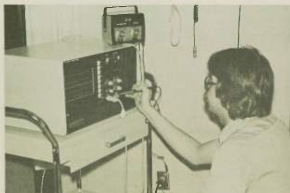
Fig. 12—Low, low 200 microAmp range measures medical and OSHA leakage currents with ease and accuracy.
