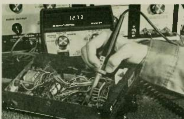
Fig. 13—Isolation switch in the probe isolates the test lead capacity to prevent upsetting critical oscillator circuits during tests.
