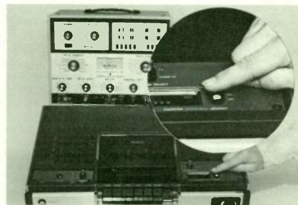
Fig. 25—The VA48 patterns may be recorded on a known good deck for a playback reference. Use the deck's digital counter to allow the desired section of the tape to be located.
