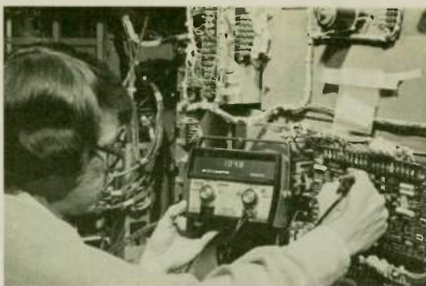
Fig. 2—The DVM37 can be used in high power motor and RF fields that would render analogs and other DVMs useless.
