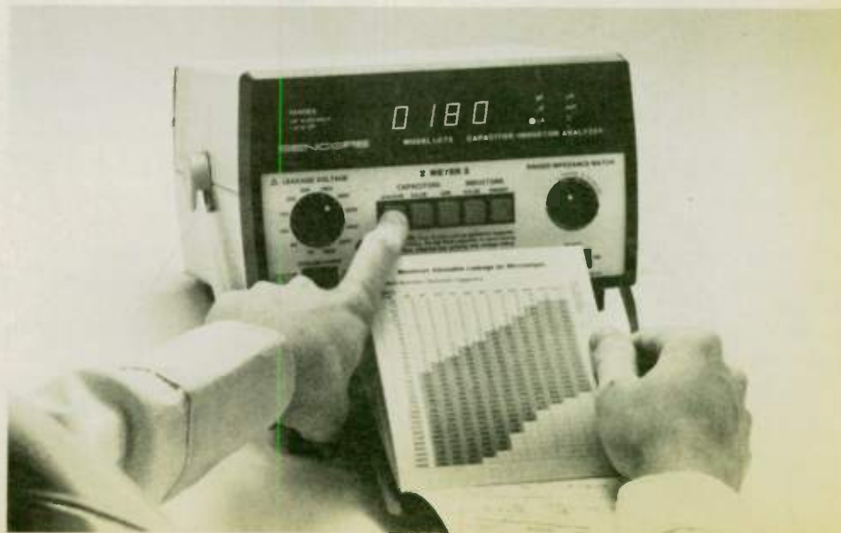
Fig. 4: Simply look at the pull chart to find how much leakage to allow for any capacitor value and voltage rating.
