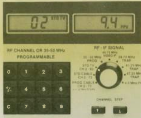
Fig. 5: The programmable function lets you program any shift, up to 9.75 MHz (plus or minus) by entering the shift into the keyboard.
