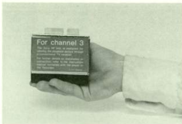
Fig. 24—The RF modulator is used to produce an output signal to feed directly to a standard TV set. This stage is not generally intended to be repaired.
