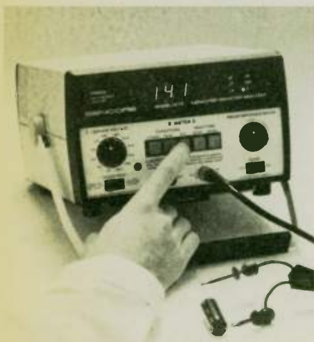
Fig. 7: Simply press the ESR button on the "Z2" and read the resistance directly in ohms to isolate ESR problems.
