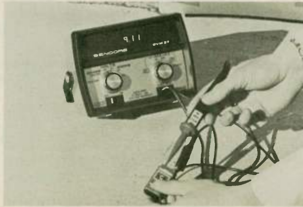
Fig. 11—Here's the proof that the DVM37 keeps on working after a ten-foot drop when other DVMs are shattered.
