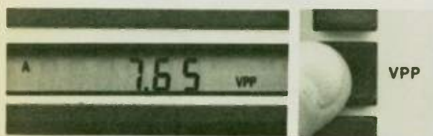
Fig. 5: Measure AC volts up to 100 MHz on either channel automatically at the push of a button.
