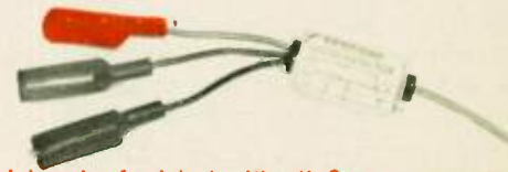
Special probe furnished with all Sencore generators provides detector probe and isolation probe in one.
