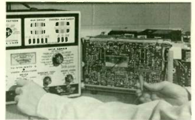
Fig. 39—The peak-to-peak reading signal tracing meter is especially handy when the signal amplitude is more important than the waveshape.
