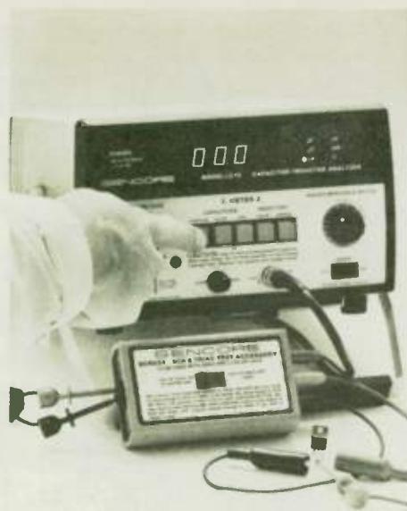
Fig. 11: The low-cost SCR224 adapts the "Z2" to test SCRs and TRIACs, accurately and easily.
