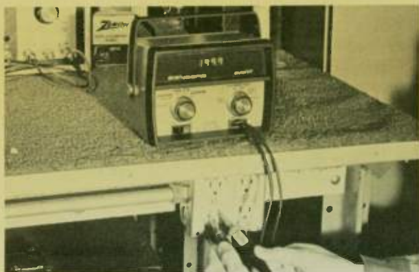
Fig. 8—The DVM37 simply winks at 120 Volts AC line voltage applied on the 200 Ohm range because of built-in diode protection.
