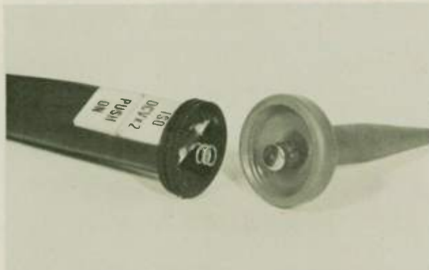
Fig. 9—Current ranges are fully protected against overloads above two Amps with a handy fuse in the probe.
