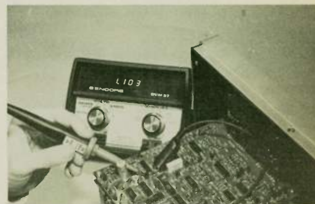
Fig. 14—Lo Power Ohms equips you to measure resistances in-circuit without unsoldering components or switching leads.
