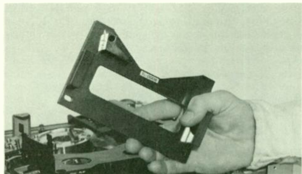
Fig. 27—Proper mechanical alignment requires the use of the special gauges and test jigs available from the deck manufacturer.
