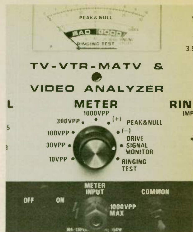
Fig. 41—Built-in peak-to-peak meter automatically monitors drive signal levels and can be used for signal tracing using external METER INPUT lead.
