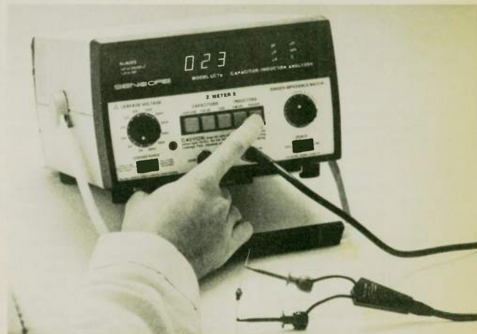
Fig. 10: The "Z2"'s Ringer test finds even a single shorted turn in an inductor by simply watching for a reading of 10 or larger on the display.
