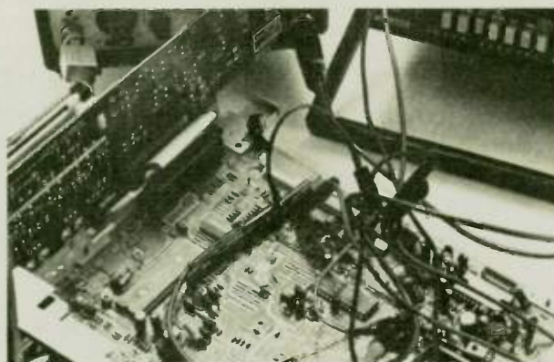
Fig. 2: Using additional leads often doubles the loading.
