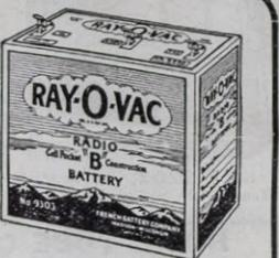
Type 9303. Twice the life of ordinary 45-volt types of medium size. For sets requiring more than 15 mils. 8x4½x7½ in. Shpg. wt., 10 lbs.
