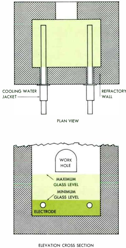
**ELECTRIC DAY TANK**, a small furnace, has two horizontal electrodes extending through a wall. This arrangement keeps electrodes fully immersed as workers take glass out of the tank.
