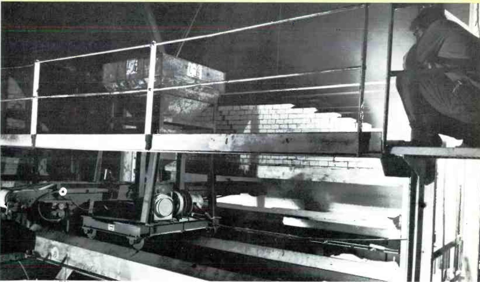
**BATCH CHARGER** for the continuous electric furnace at the Jeannette Glass Company travels along the side of the furnace.
