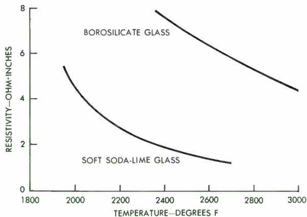
**ELECTRICAL RESISTIVITY OF GLASS** varies inversely with temperature, and it also depends on the chemical composition of the glass. This wide variation in resistivity encountered among various glasses and at various temperatures necessitates careful design of electric furnaces and their power supplies. The characteristics illustrated here are for a borosilicate glass (for ovenware) and a soda-lime glass (common container glass).
