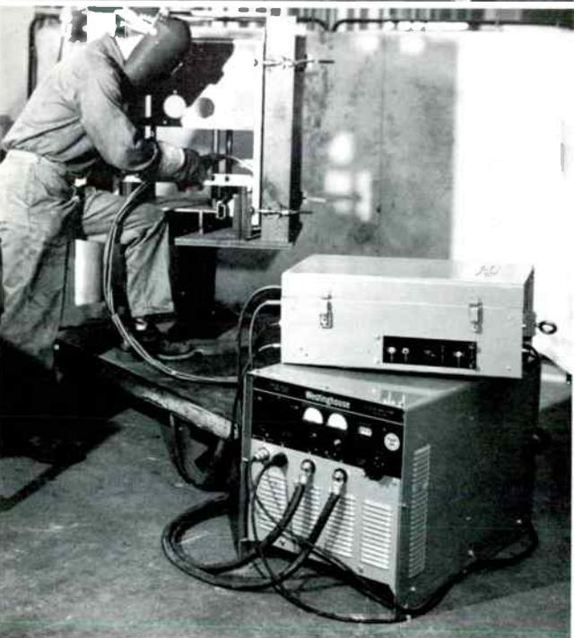
it reacts to a change in current in such a manner as to hold the current constant. Its effect is strictly dynamic, thus limiting only the rate of change of current and not the final steady-state value. A mechanical analogy of the dynamic reactor is the flywheel, which tends to level out what would otherwise be abrupt speed changes.
