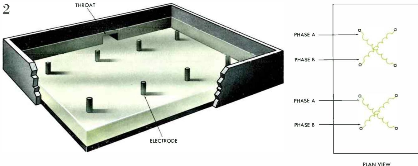
**TYPICAL ELECTRIC FURNACE** has eight vertical cylindrical electrodes (left). The electrodes are connected in a two-phase four-wire arrangement (right), an inherently square configu-
