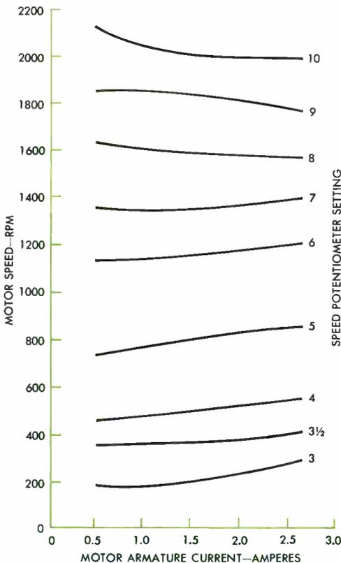
**SPEED REGULATION** with the type 902 thyristor drive in the *low* speed range (top) and the *high* range (bottom). Excellent control is provided over a range of seven to one or greater. The curves are based on the performance of a dc shunt-wound motor rated at 1/4 horsepower, 2.5 amperes, and 1725 rpm.
