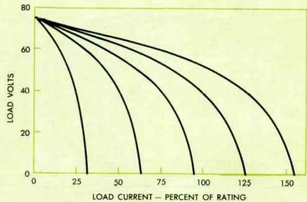
**CONSTANT-CURRENT DC WELDERS** have electrical characteristics as shown by these typical volt-ampere curves. Because the curves slope steeply in the working voltage range, a change in load voltage at a given machine setting produces only a relatively small current change.
