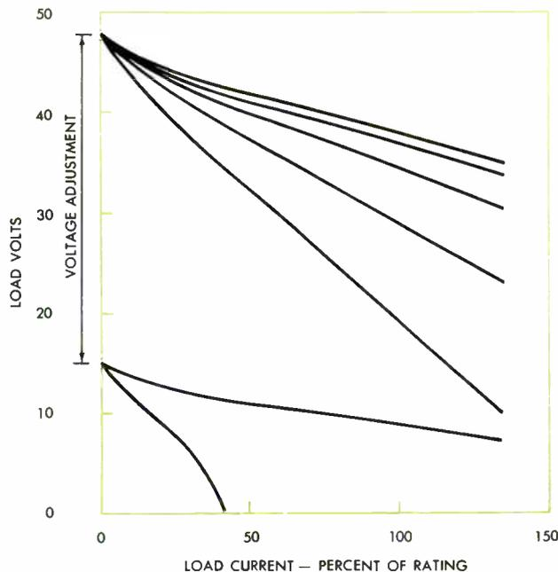
**CONSTANT-VOLTAGE DC WELDERS** have volt-ampere curves that are nearly flat. In some, the slope of the curves can be adjusted as shown. Voltage also is adjustable over a wide range.
