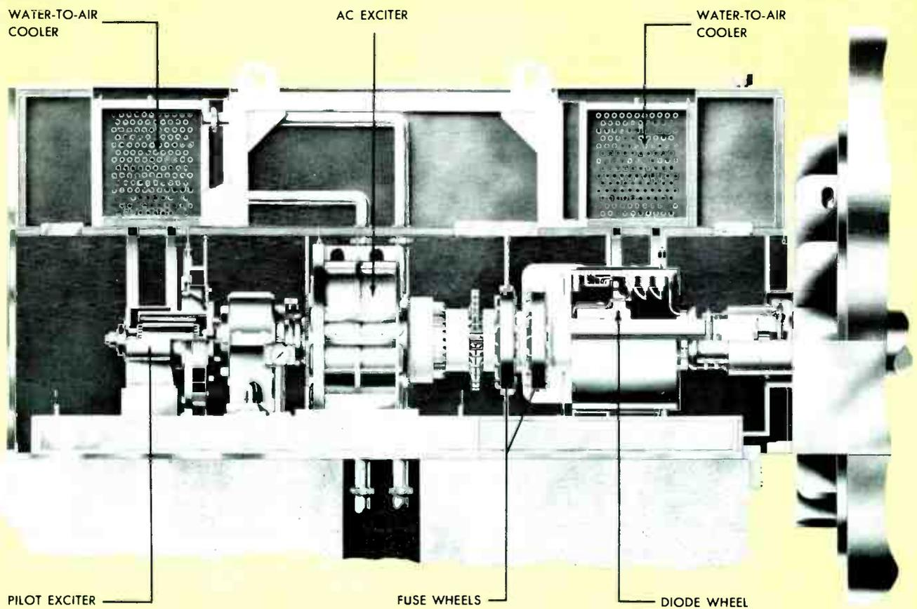
COMPONENT ARRANGEMENT of the brushless excitation system is shown in this artist's drawing of the 1350-kw unit.
