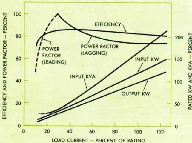
**AC ARC WELDERS** of the transformer type usually have capacitors for power-factor correction, giving electrical performance illustrated by these typical curves. Because the capacitors draw the same corrective kva under all load conditions, power factor increases with decreasing current output. Idling input is approximately 1.5 kva per 100 amperes of rating, and power factor is 100 percent leading.
