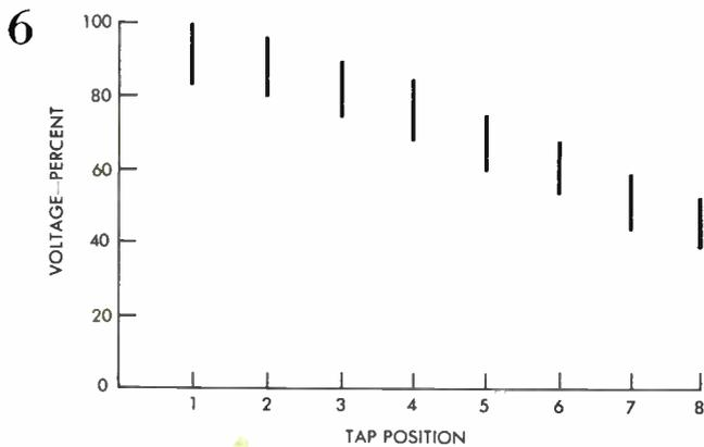
**VOLTAGE CONTROL** available at each transformer tap position by reactor adjustment overlaps that available at the adjacent positions. This reduces the amount of tap changing required.
