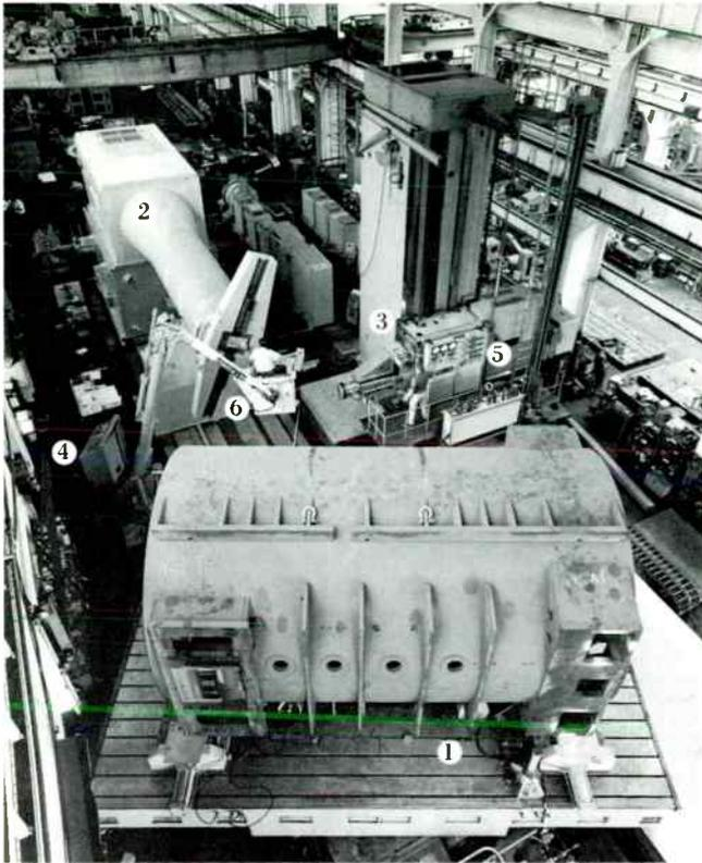
**MACHINING CENTER** for large generator frames (above) performs all machining operations at one work station. Its side unit (left) machines the sides of a frame, while its end unit (right) works on the two ends.
