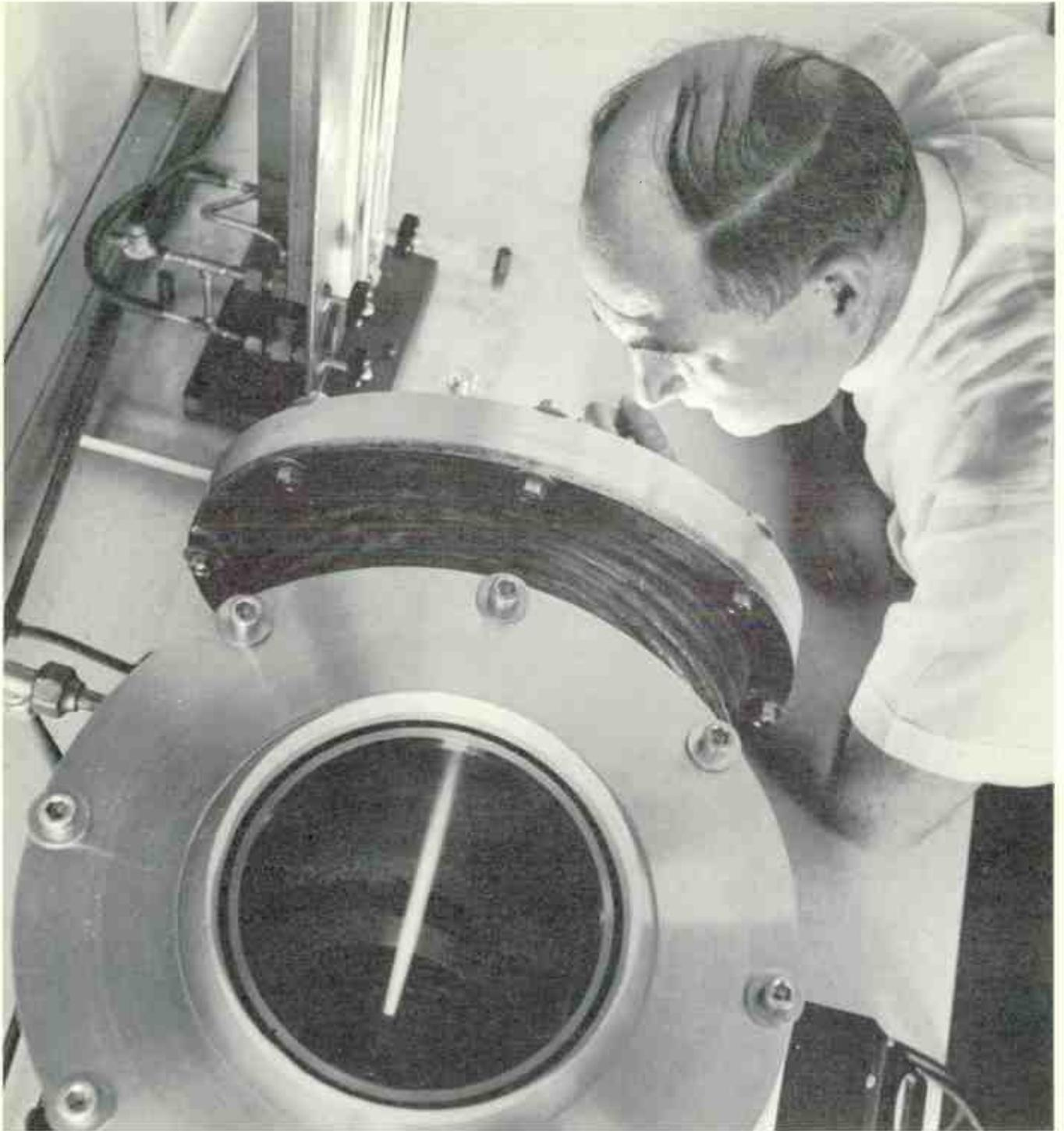
An arc plasma jet is being operated in a vacuum chamber here as part of an evaluation of its usefulness as an attitude-control device for space vehicles. The jet unit consists basically of a nozzle and two electrical terminals, between which an electric arc is maintained. When helium is fed into the arc, the great amount of heat imparted to it causes it to expand through the nozzle at supersonic velocity and thereby develop thrust. A heated cathode
