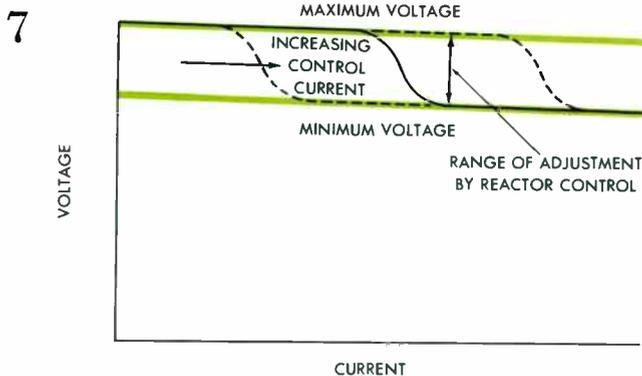
**VOLTAGE-CURRENT CHARACTERISTICS** of the furnace power supply for one transformer tap position. The two colored lines indicate maximum and minimum voltages available at this tap position. The solid line shows the characteristic for one specific setting of control current in the saturable reactor; other control-current settings would give the characteristics indicated by the dashed lines.
