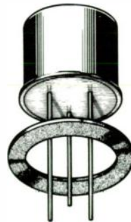
Figure 24 - A plastic ring used to space a transistor.
