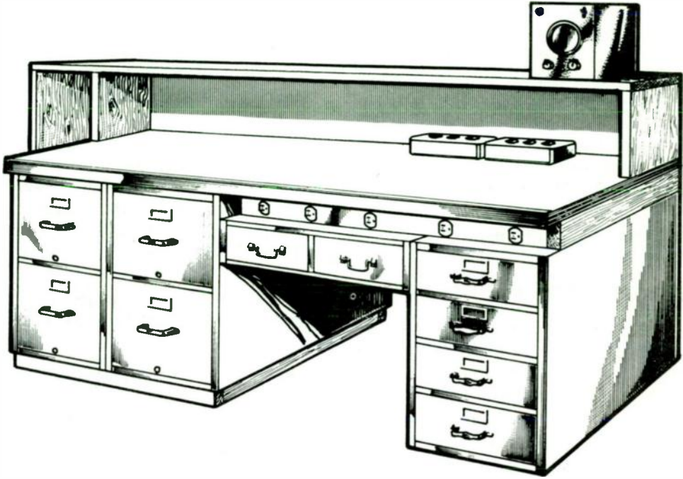
Figure 3 — One version of a work bench constructed from file cabinets and plywood.
