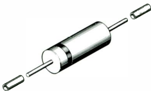
Figure 10 - Sleeving for a component's leads.
