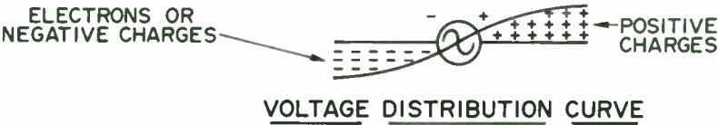
Figure 4 - Dipole antenna showing current and voltage distribution.
