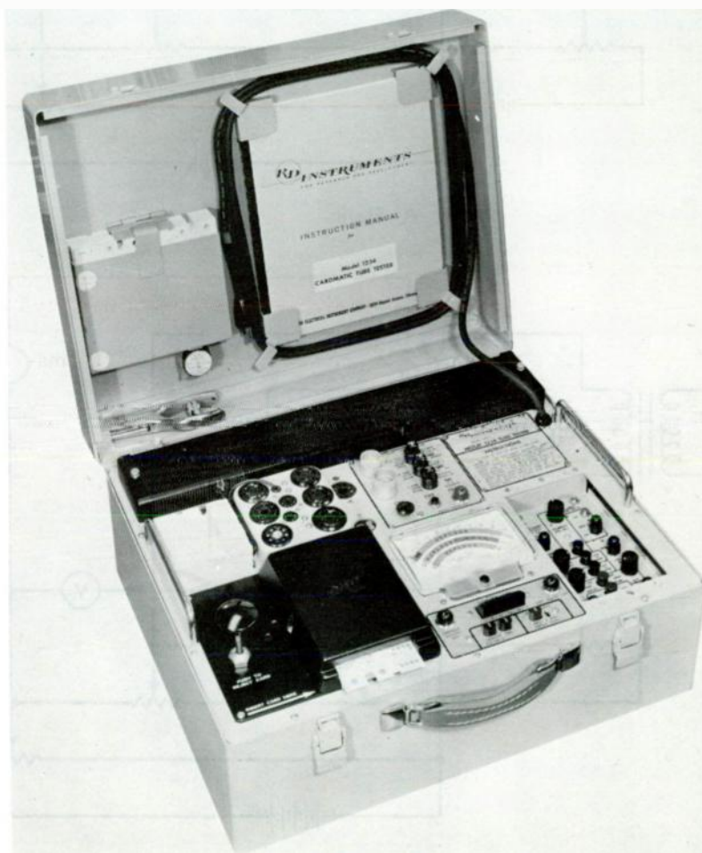
Figure 10 — Card-type mutual-conductance tube tester.
