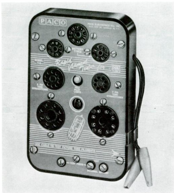
Figure 4 — Filament continuity tester.
