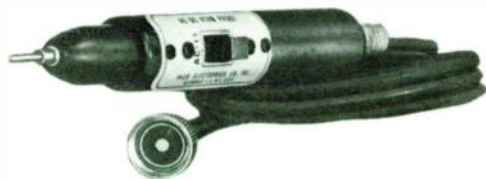
Figure 26 - VTVM single probe for AC, DC and ohms.
