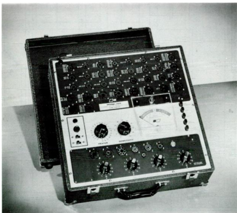
Figure 16 — Gm tester with minimum number of controls.
