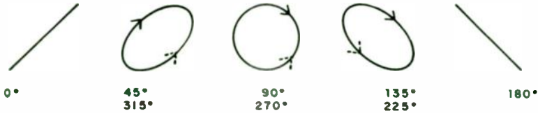
Figure 16 — Lissajous patterns show phase difference between two sine waves.
