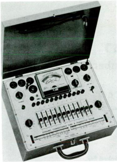
Figure 23 — Combination tube and transistor checker.
