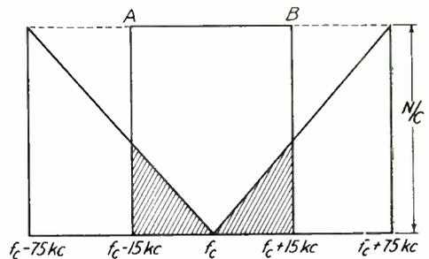
Fig. 24.—Noise-to-signal ratio for f.m. and a.m. systems.
