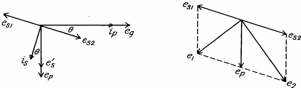
Fig. 40.—Vector phase relations above resonance in a discriminator circuit.
