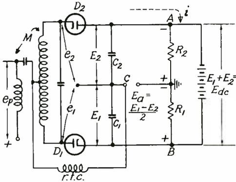
Fig. 47.—Basic circuit of ratio detector.
