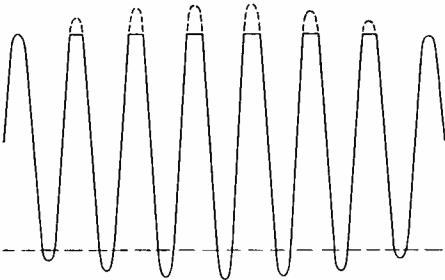
Fig. 31.—Appearance of wave after limiting.
