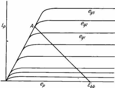
Fig. 30.—Plate family of characteristics showing limiting action owing to shape of curves.
