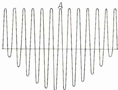
Fig. 34.—Representative appearance of the output wave of a limiter.
