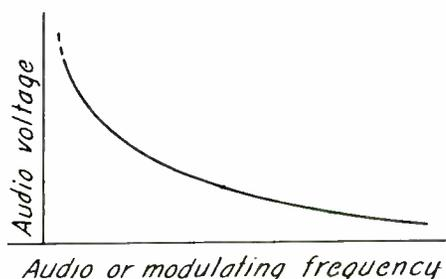
Fig. 5.—Audio-frequency response curve required to give f.m. in the Armstrong system.
