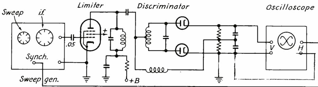
Fig. 43.—Test setup for visual adjustment of f.m. receiver.
