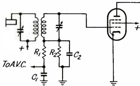
Fig. 35.—Method of obtaining a.v.c. from a limiter stage.
