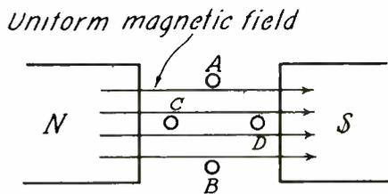
Fig. 3.—Generation of an a.c. wave by the rotation of a loop in a uniform magnetic field.
