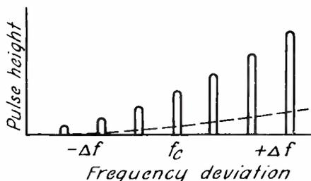
Fig. 56.—Relation between pulse amplitude and frequency deviation.
