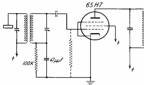
Fig. 32.—Limiter stage employing clipping in grid circuit.
