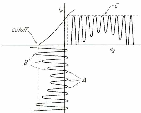
Fig. 33.—Appearance of grid input wave and plate current output wave in grid limiter.
