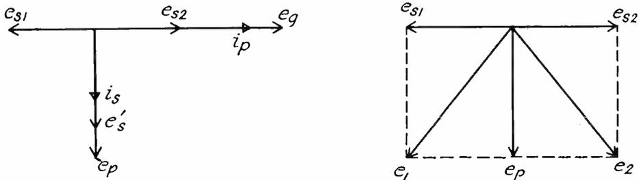
Fig. 39.—Vector phase relations at resonance in a discriminator circuit.
