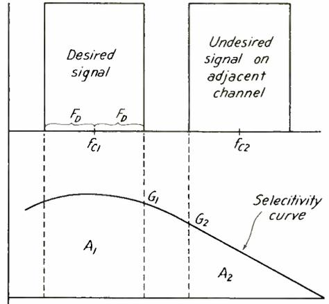
Fig. 26.—Effect of selectivity curve on two signals in adjacent channels.
