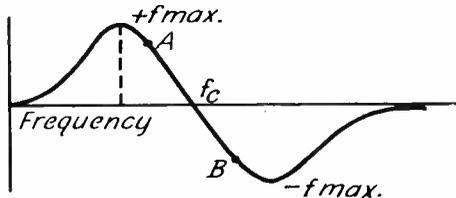
Fig. 42.—Discriminator characteristic: output versus frequency deviation.
