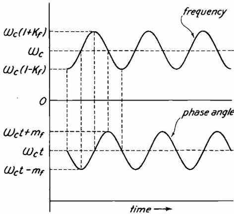
Fig. 4.—Relation between sinusoidal frequency variation and corresponding phase variation.
