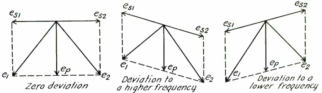
Fig. 48.—Vector diagrams showing phasing voltages for zero deviation, deviation to a higher frequency, and deviation to a lower frequency.
