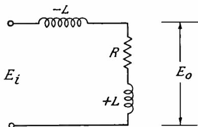
Fig. 9.—Theoretical preemphasis network required in an f.m. transmitter.
