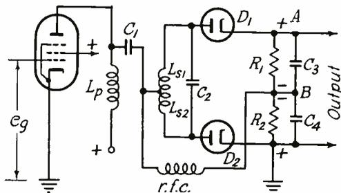
Fig. 38.—Typical discriminator circuit.
