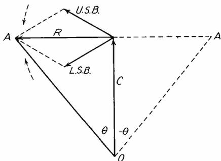
Fig. 14.—Combination of carrier vector with two first-order side bands to give approximate frequency modulation.
