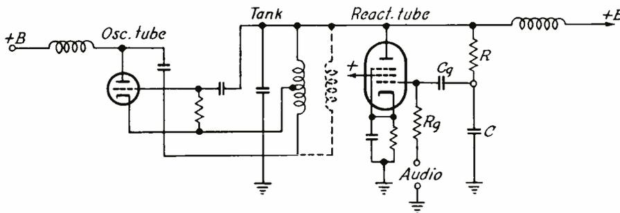
Fig. 6.—Reactance tube used as a shunt inductance to the tank circuit.
