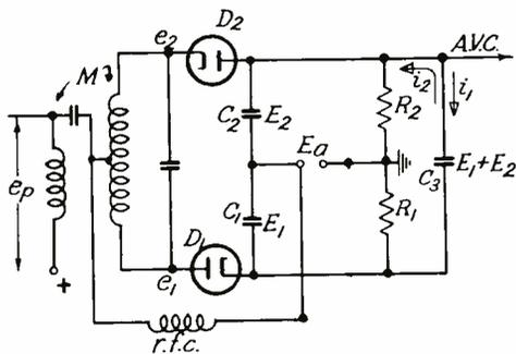
Fig. 51.—Use of a stabilizing capacitor  $C_3$  instead of a battery.
