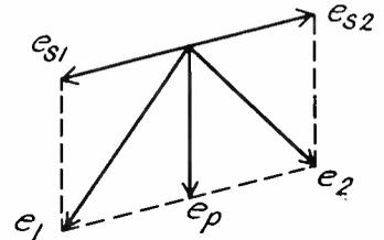
Fig. 41.—Vector phase relations below resonance in a discriminator circuit.
