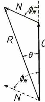
Fig. 22.—Vector diagram used to derive signal/noise ratio for f.m.
