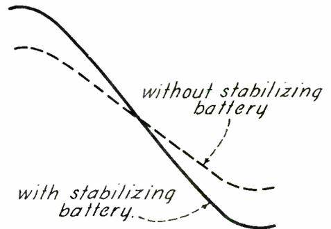
Fig. 50.—Effect of using a stabilizing battery.
