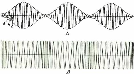
Fig. 1.—A.M. and F.M. waves.
