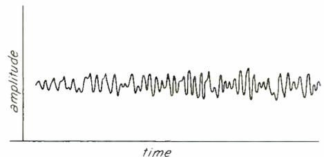
Fig. 20.—Picture of thermal noise, showing its random nature with time.
