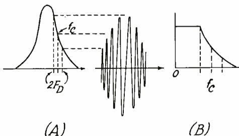
Fig. 37.—Use of resonant circuit and also cutoff portion of a band-pass filter to obtain a.m. from f.m.
