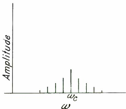
Fig. 11.—Frequency distribution and relative amplitudes of some of the side bands of a sinusoidally frequency-modulated wave.
