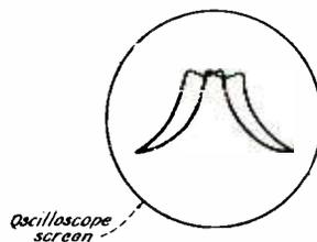
Fig. 45.—Appearance of i.f. resonance curves on oscilloscope screen.
