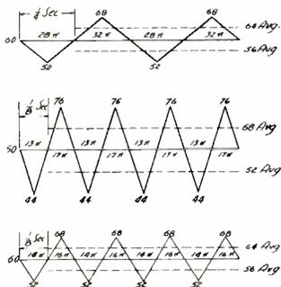
Fig. 3A. — Sawtooth frequency modulation at two deviation frequencies and rates.
