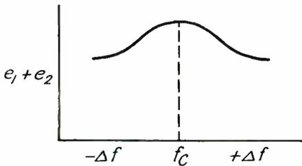
Fig. 49.—Variation in  $(e_1 + e_2)$  with frequency deviation  $\pm \Delta f$  from the carrier frequency  $f_c$ .
