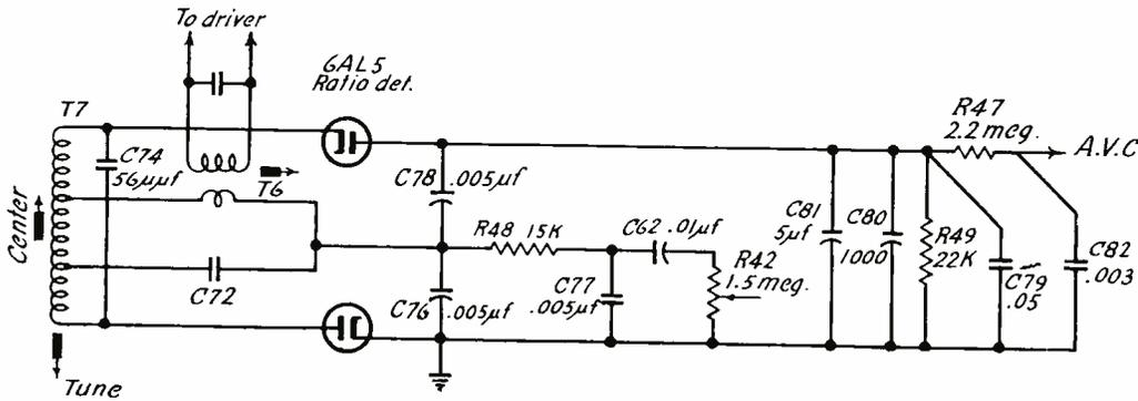
Fig. 58.—Ratio-detector circuit used in RCA Model 612V1 receiver.
