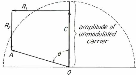
Fig. 15.—Combination of carrier, first-order, and second-order side bands.
