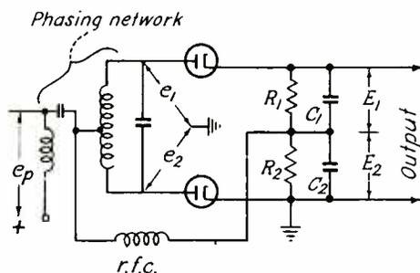
Fig. 46.—Discriminator circuit showing a.c. and d.c. voltages.
