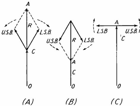
Fig. 12.—Representation of an amplitude-modulated wave by a carrier vector C, an upper side-band vector u. s. b., and a lower side-band vector, l. s. b.
