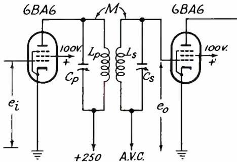
Fig. 28.—Typical i.f. stage of an f.m. receiver.
