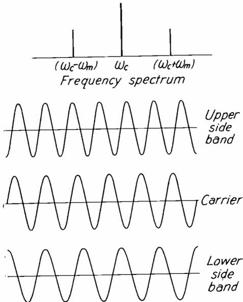
Fig. 2.—Side bands and carrier of an amplitude-modulated wave.
