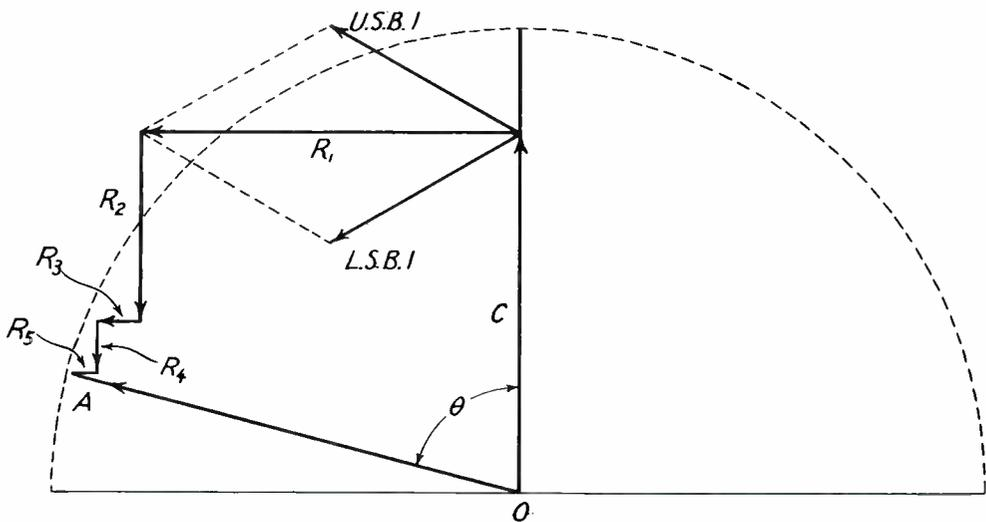
Fig. 16.—Combination of five pairs of side-band vectors with the carrier.
