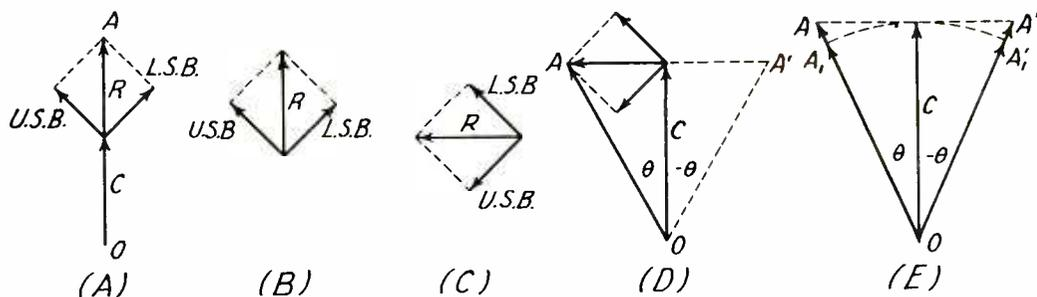
Fig. 18.—Successive steps in producing f.m. by means of the Armstrong method.
