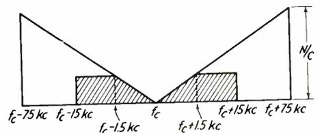
Fig. 25.—Noise-to-signal ratio when deemphasis is used.
