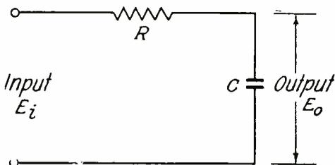
Fig. 8.—Standard deemphasis network for an f.m. amplifier.
