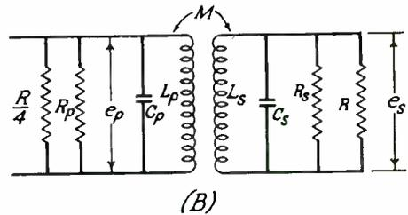
Fig. 52.—Elementary basic circuit of the ratio detector.
