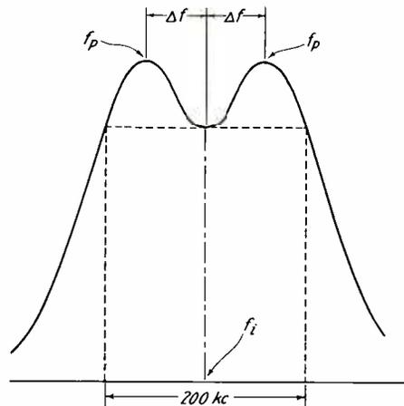
Fig. 29.—Peak half band width and total band width.
