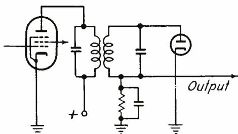
Fig. 36.—Elementary f.m. detector.
