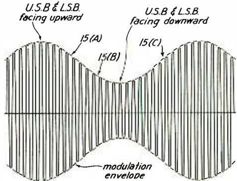
Fig. 13.—Modulated wave showing points on its envelope corresponding to Fig. 12(A), (B), and (C).
