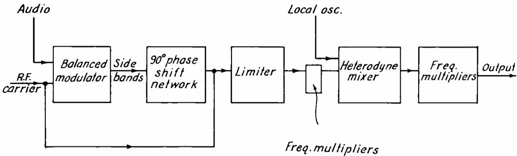
Fig. 17.—Block diagram of Armstrong system of frequency modulation.
