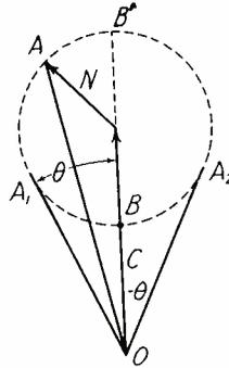
Fig. 21.—Combination of an unmodulated carrier and a noise component.
