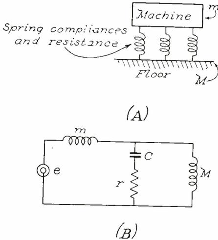
Fig. 25.--Electrical analogue of machine isolated from floor.
