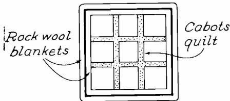
Fig. 29.--Arrangement of acoustic material in ventilating duct.
