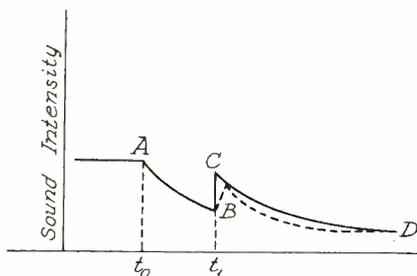
Fig. 8.--Discontinuous decay obtained for two coupled enclosures.
