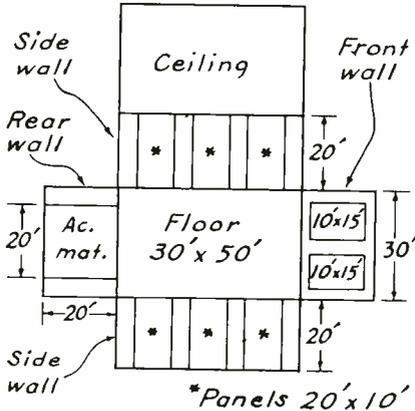
Fig. 4.--Arrangement of acoustic treatment in a studio.
