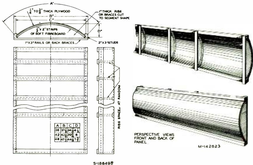
Fig. 16.—Constructional details of a polycylindrical wall.
