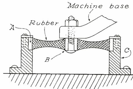
Fig. 26.--One form of vibration isolator.
