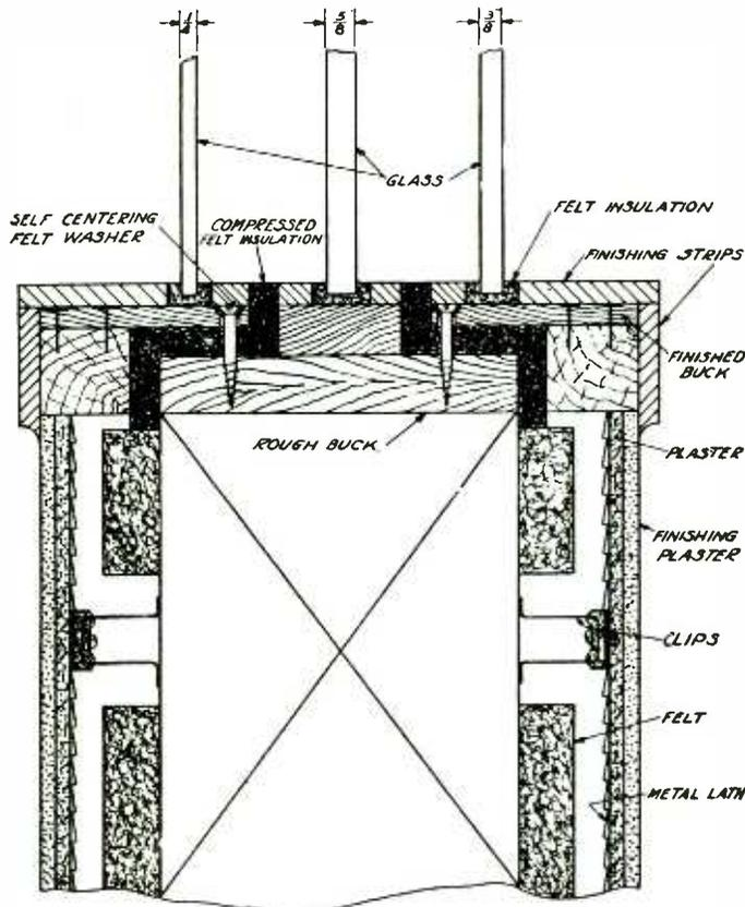
Fig. 10—Soundproof window construction.
