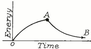
Fig. 2.--Growth and decay of sound energy in an enclosure.
