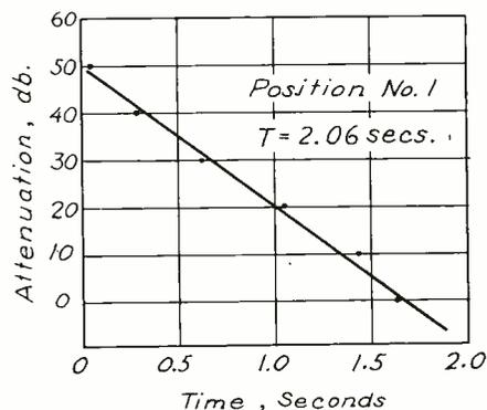
Fig. 19.—Relation between attenuation of a sound from a maximum level to some lower level, and corresponding elapsed time.
