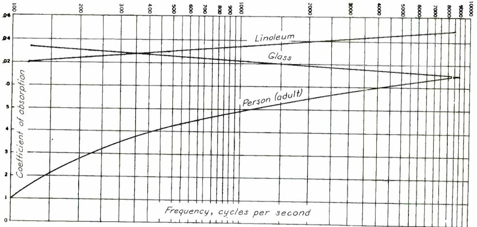
Fig. 37.--Absorption coefficients of various materials at different frequencies.
