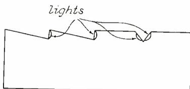
Fig. 12.--Break-up of ceiling to diffuse sound.
