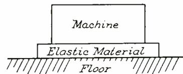
Fig. 24.--Use of elastic material to isolate machine vibration from floor.
