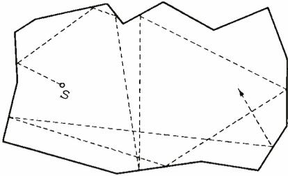
Fig. 11.-- Use of vee serrations in the walls of an auditorium to diffuse sound.
