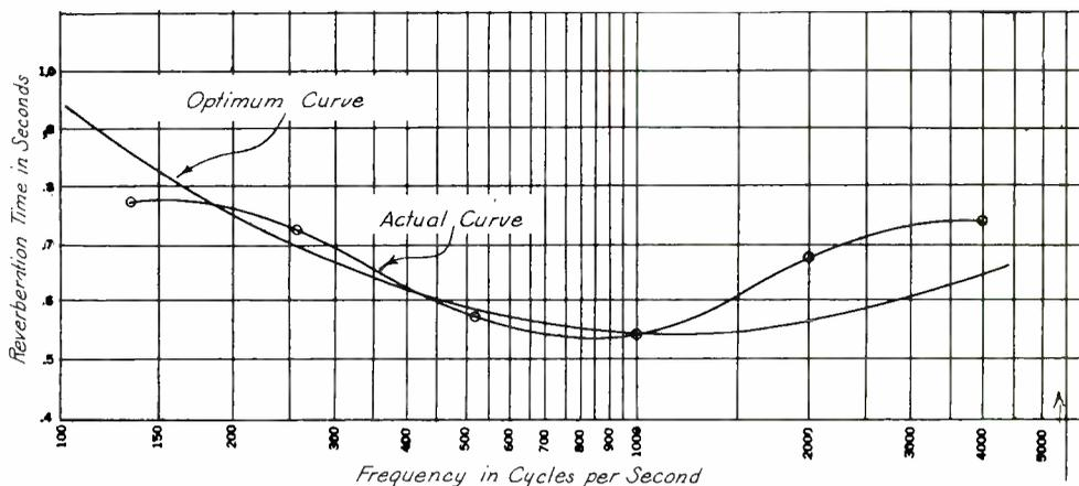
Fig. 39.--Calculated and optimum reverberation time for proposed studio.
