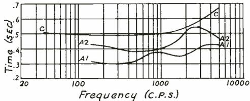
Fig. 34.--Actual and calculated reverberation time vs. frequency for WOR Studio 8.
