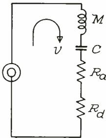
Fig. 15.—Electrical circuit equivalent to resonant wall.
