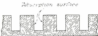
Fig. 21.--Showing how hole increase sound-absorbing surface.
