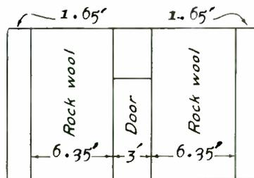
Fig. 38.--Rear wall of proposed studio, showing layout of acoustic material and door.
