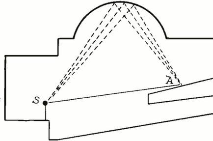
Fig. 10.--Focusing effect of a dome in an auditorium.
