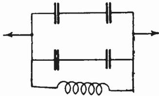
THE VOLTAGE RATING OF THIS COMBINATION WILL BE  $2 \times 100 = 200$  VOLTS WHICH EXCEEDS THE MAXIMUM EXPECTED VOLTAGE OF 150 VOLTS. NOTE THAT ONLY 2 AMPERES FLOWS THROUGH ANY ONE CONDENSER SO THE VOLTAGE DROP IS KEPT DOWN TO  $2 \times 1.414 \times 26.5 = 75$  VOLTS PEAK PER CONDENSER. THE TOTAL CAPACITY OF THE COMBINATION WILL BE 100  $\mu\text{F}$ .
