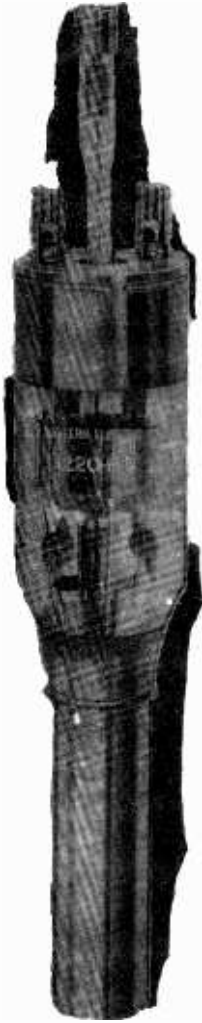
Fig. 8.—Type 220B—Filamentary water-cooled triode.
