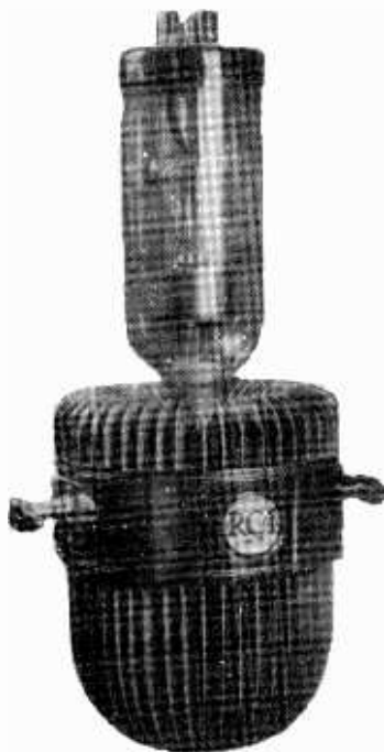
Fig. 6.—One of the standard metal-anode type tubes fitted with copper radiating fins for air cooling.
