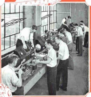
These students are receiving special instruction on balancing superheterodynes and making final efficiency tests with oscillators, output meters and modern test instruments of various kinds.
