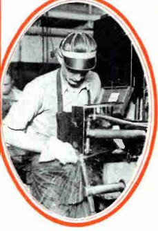
Spot welding of radio chassis.
