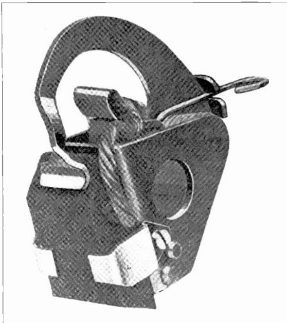
Fig. 19. Reaction-type brush holders keep the brush in place by the pressure of a "brush hammer", as shown on top of the brush in this view.
