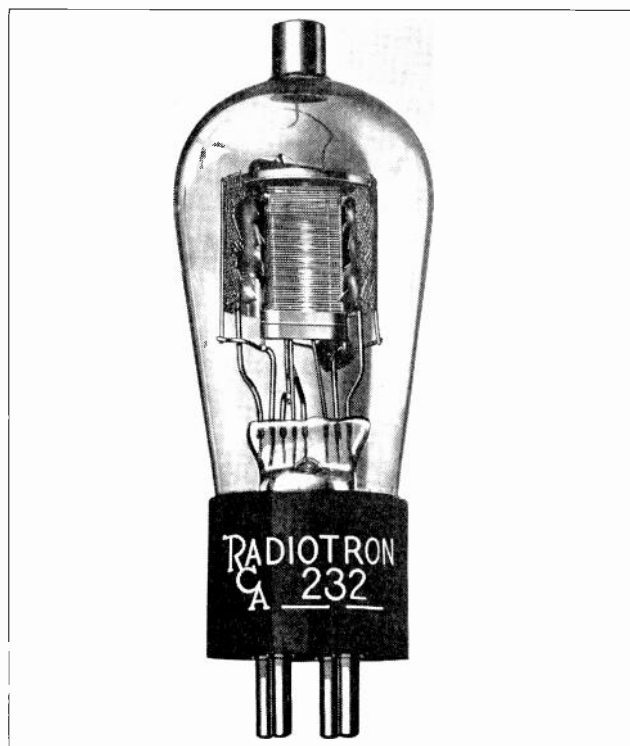
Fig. 59. This excellent photograph shows a vacuum tube with part of the outer screen grid and part of the plate removed, to clearly show the inner screen grid in its position between the control grid and plate. (Photo courtesy of R. C. A. Radiotron Co., Inc.)
