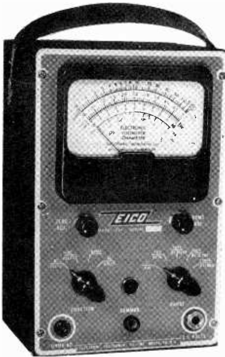
An electronic voltmeter with a high input resistance is needed to measure the voltages operative in an avc system.
