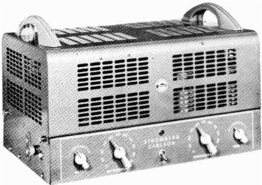
Portable phonograph and sound amplifier equipped with automatic volume expander circuit.
