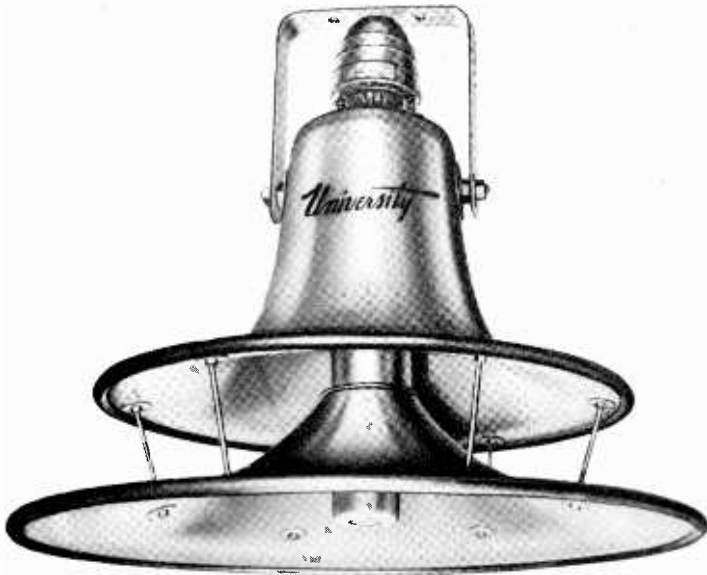
Radial Reflex Speaker consisting of reflex air column horns with radial deflectors, designed with a dispersion angle of 360^\circ for uniform sound distribution over wide areas.
