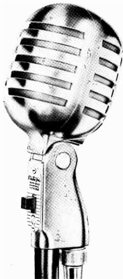
Crystal microphone with cardioid pickup characteristic. Equipped with screwdriver adjustment for changing from flat response to high-frequency boost.
