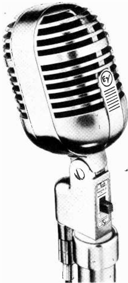
Dynamic microphone with a cardioid wide-angle pickup and the greater part of the reflected sounds eliminated. Has a frequency response from 40 to 10,000 cycles per second.
