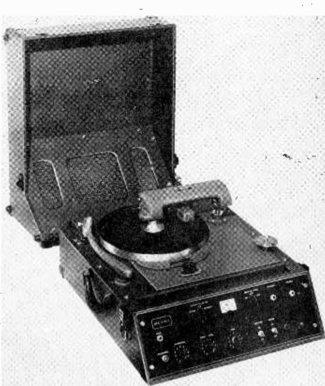
Recorder for 12-inch disks. Both the cutting arm and pickup arm can be seen. The pickup arm can be used also for 16-inch transcriptions.
