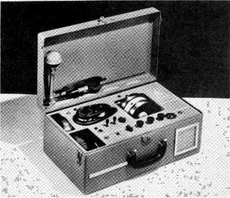
Portable magnetic wire recorder and reproducing unit.
